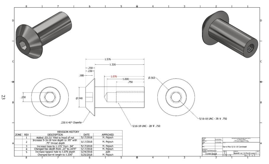
Figure A-3. 1.567-in. (40-mm) Long Barrel Nut with Cone Head Design
