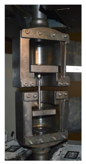
Figure 2. Tensile Test Setup
