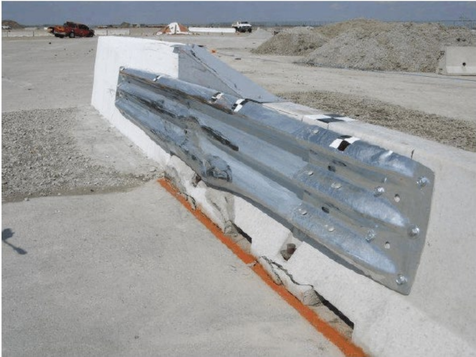
Figure 3. Concrete Height Transition Details after MASH Test 3-21
