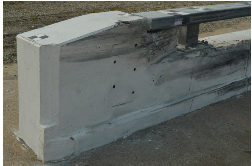
Figure 109. End Post, Tapered End, and Rail and Post No. 23 Damage, Test No. MNCBR-2
