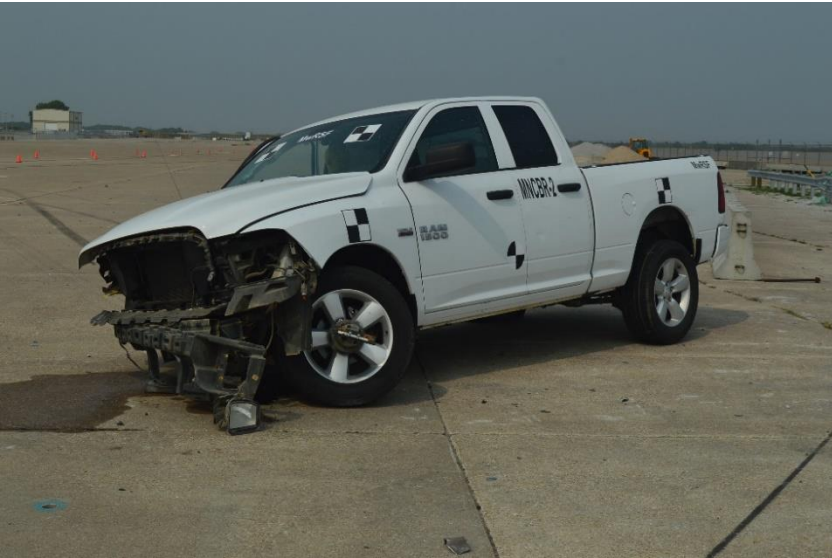
Figure 115. Vehicle Damage, Test No. MNCBR-2
