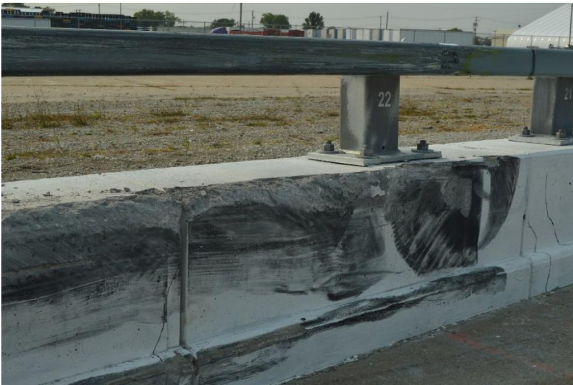
Figure 104. Concrete Gouging and Spalling, Test No. MNCBR-2
