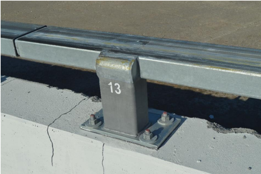
Figure 81. Rail and Post Damage, Post No. 13, Test No. MNCBR-1
