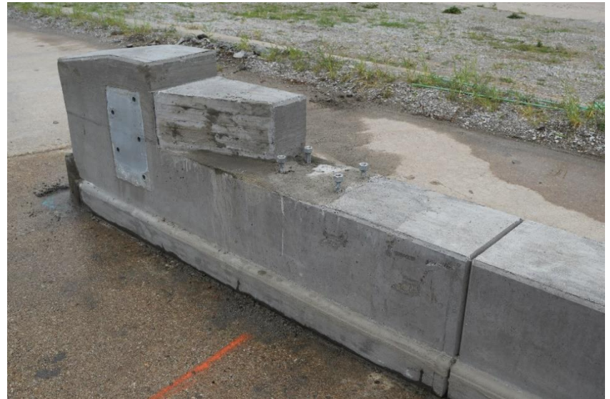
Figure 39. New Concrete Tapered End Installation, Test Nos. MNCBR-1, MNCBR-2, and MNCBR-3
