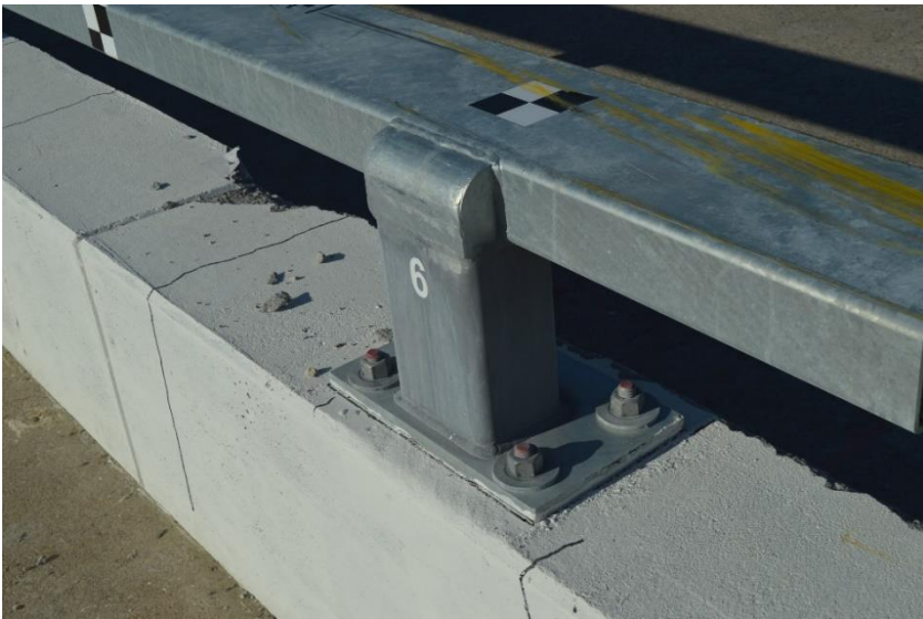
Figure 76. Rail and Post Damage, Post No. 6, Test No. MNCBR-1
