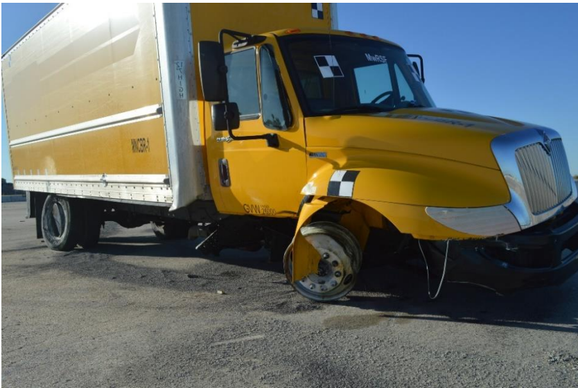
Figure 87. Vehicle Damage, Test No. MNCBR-1
