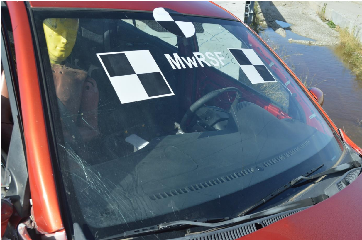
Figure 145. Windshield Damage (Post-Test), Test No. MNCBR-3
