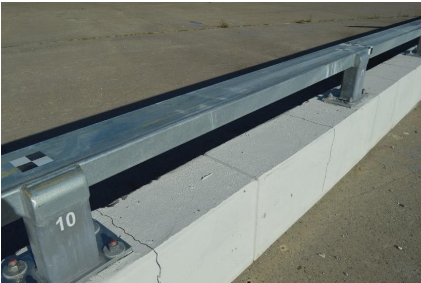
Figure 83. Rail and Post Damage, Post Nos. 11 and 10, Test No. MNCBR-1
