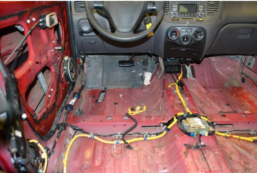
Figure 143. Vehicle Floor Pan Damage, Test No. MNCBR-3
