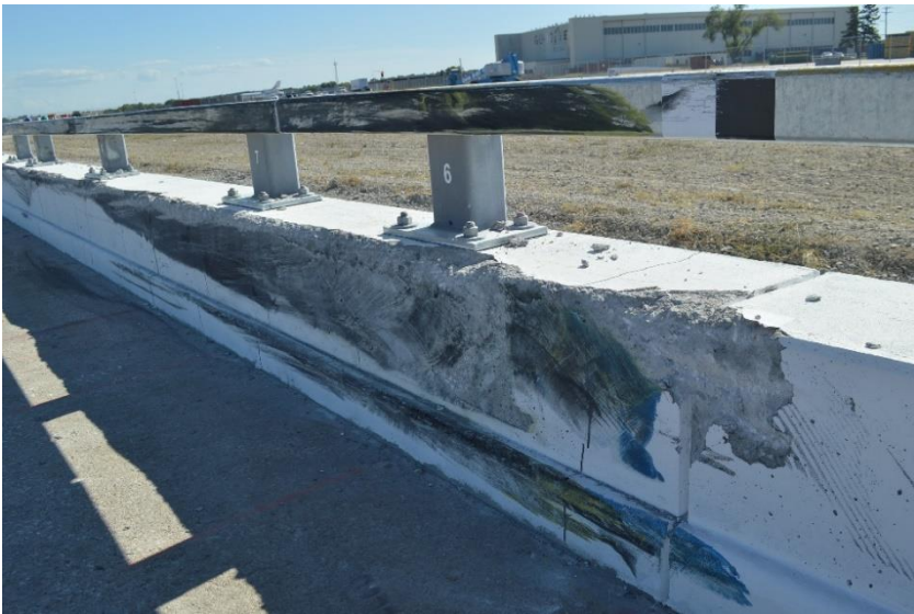
Figure 70. Concrete Gouging and Spalling, Test No. MNCBR-1
