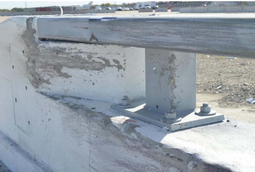
Figure 136. Rail and Post No. 4 Damage, Test No. MNCBR-3
