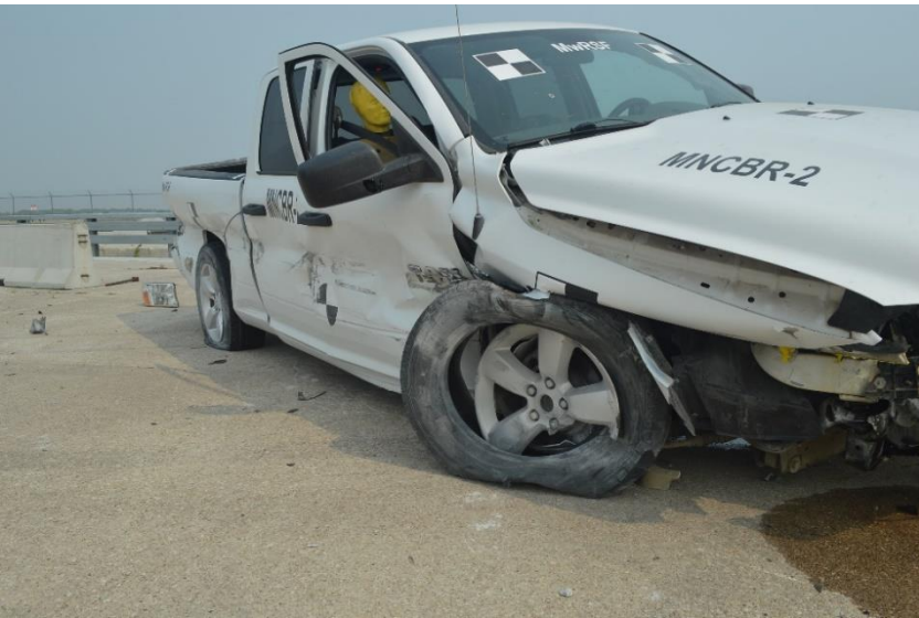
Figure 114. Vehicle Damage, Test No. MNCBR-2
