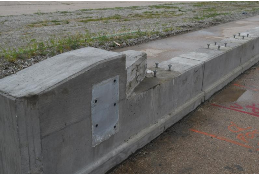
Figure 39. New Concrete Tapered End Installation, Test Nos. MNCBR-1, MNCBR-2, and MNCBR-3
