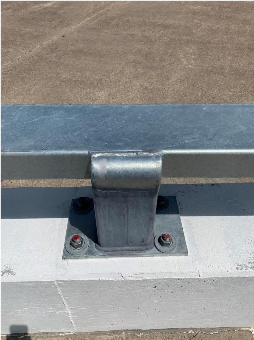
Figure 45. Post Assembly, Test Nos. MNCBR-1, MNCBR-2, and MNCBR-3
