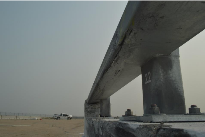
Figure 106. Rail and Post No. 22 Damage, Test No. MNCBR-2
