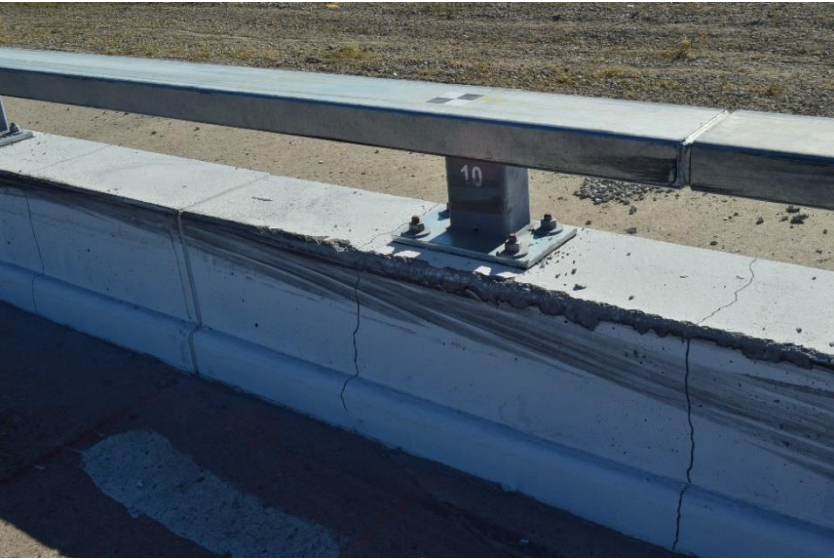
Figure 72. Rail and Post Damage, Test No. MNCBR-1
