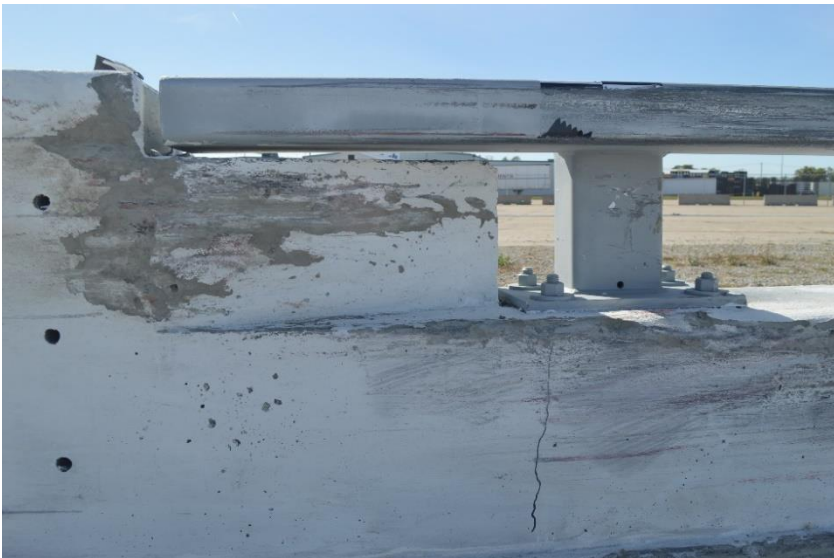
Figure 137. Rail and Post No. 4 Damage, Test No. MNCBR-3
