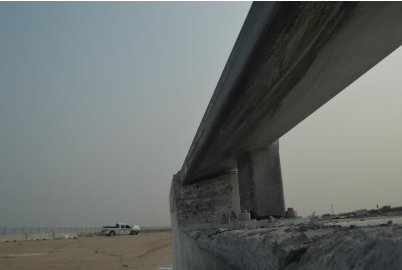
Figure 108. Rail and Post No. 23 Damage, Test No. MNCBR-2
