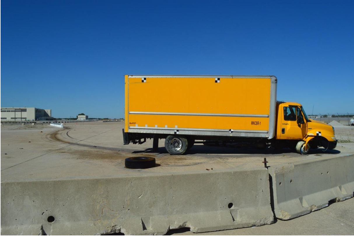
Figure 67. Vehicle Final Position and Trajectory Marks, Test No. MNCBR-1.
