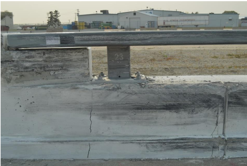
Figure 107. Rail and Post No. 23 Damage, Test No. MNCBR-2
