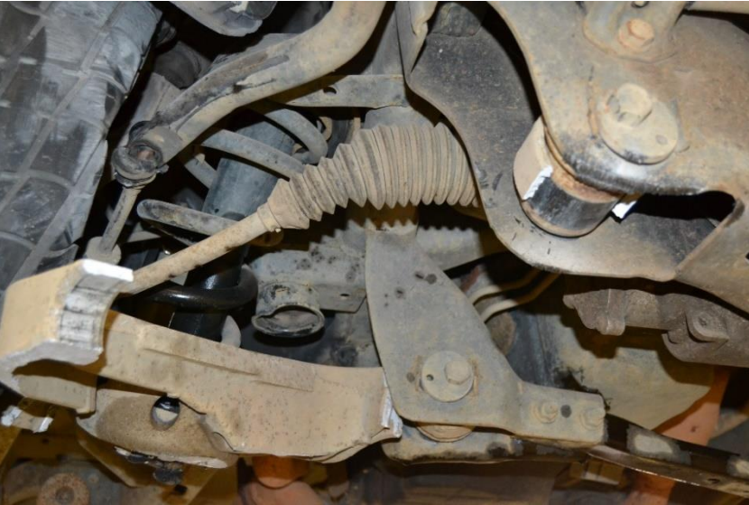
Figure 121. Undercarriage Damage, Test No. MNCBR-2
