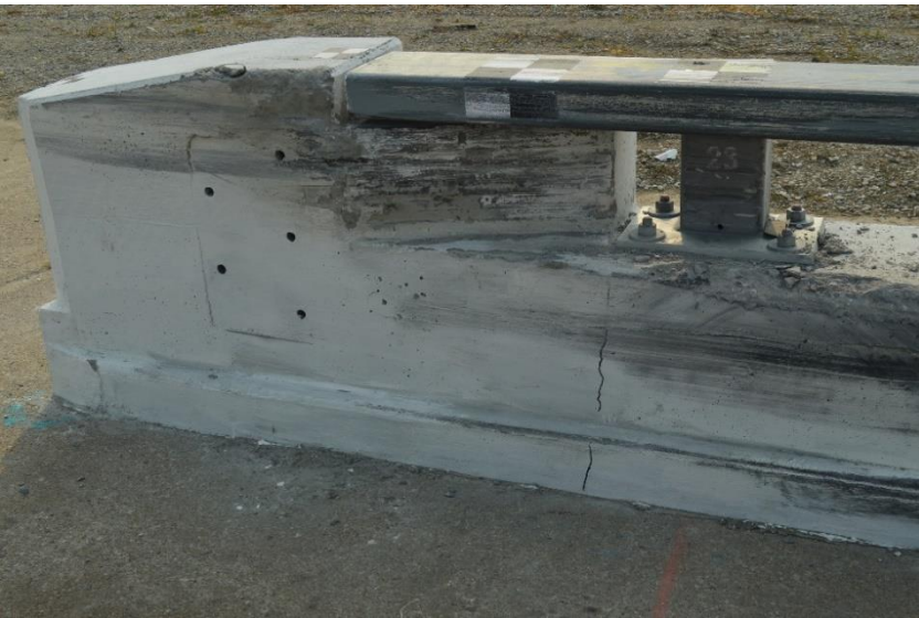
Figure 109. End Post, Tapered End, and Rail and Post No. 23 Damage, Test No. MNCBR-2
