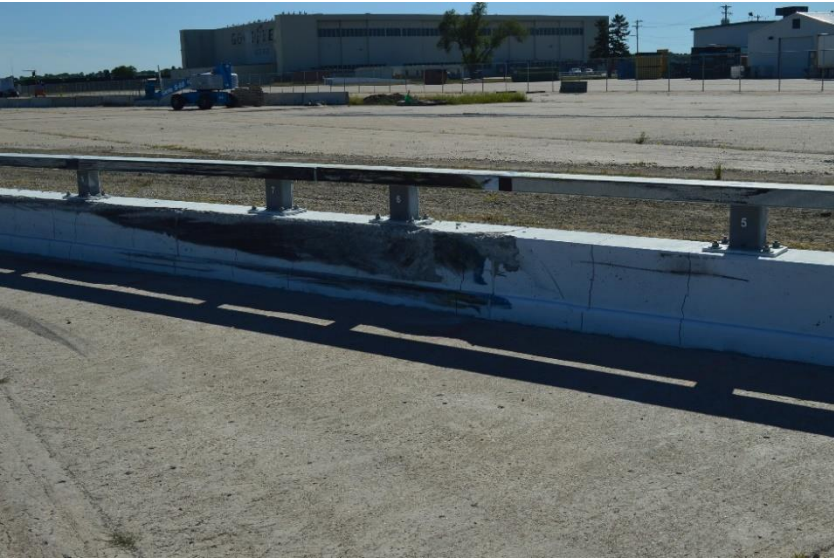
Figure 69. System Damage, Test No. MNCBR-1
