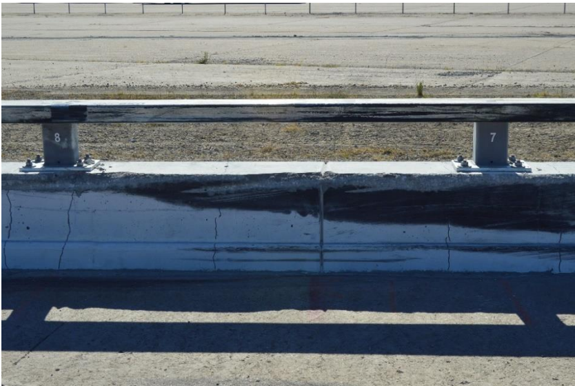
Figure 71. Concrete Gouging and Spalling, Test No. MNCBR-1
