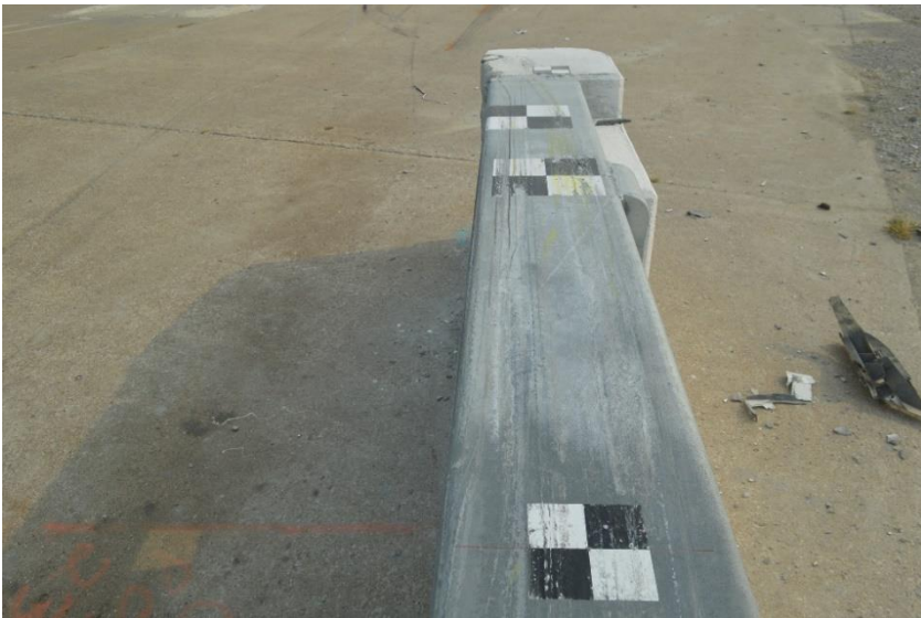
Figure 111. End Post, Tapered End, and Rail Damage, Test No. MNCBR-2
