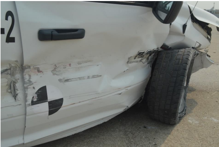
Figure 117. Vehicle Damage, Test No. MNCBR-2
