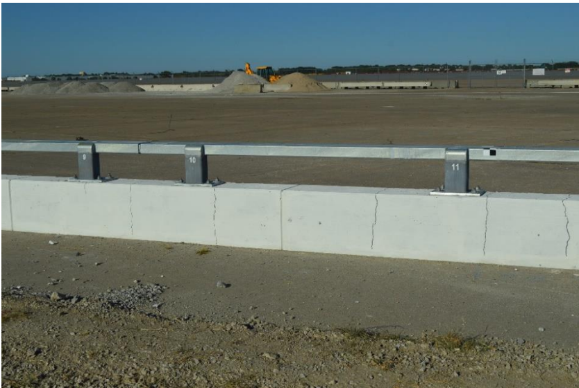
Figure 82. Rail and Post Damage, Post Nos. 12 and 11, Test No. MNCBR-1
