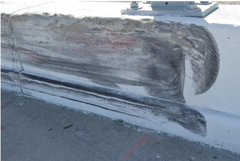
Figure 134. Concrete Gouging, Test No. MNCBR-3
