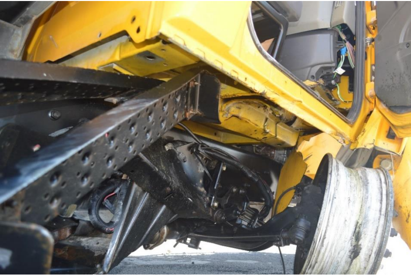
Figure 88. Undercarriage Damage, Test No. MNCBR-1
