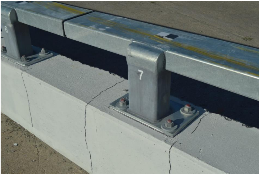
Figure 75. Rail and Post Damage, Post No. 7, Test No. MNCBR-1
