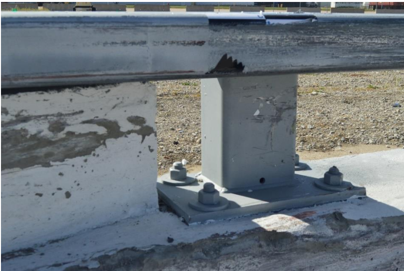
Figure 138. Rail and Post No. 4 Damage, Test No. MNCBR-3
