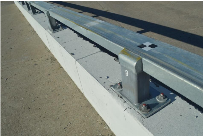
Figure 84. Rail and Post Damage, Post Nos. 10 and 9, Test No. MNCBR-1
