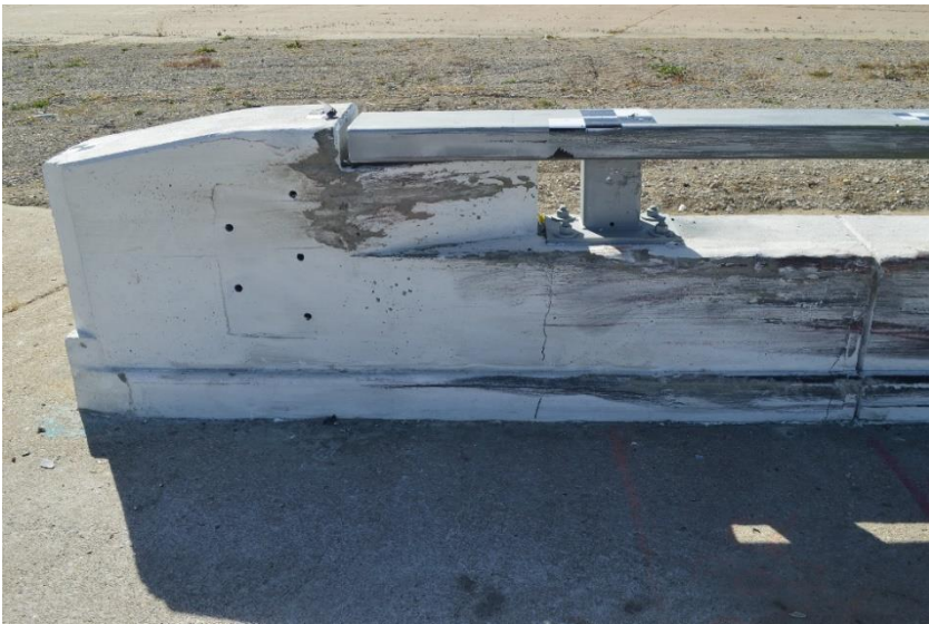
Figure 135. Concrete Gouging, Test No. MNCBR-3
