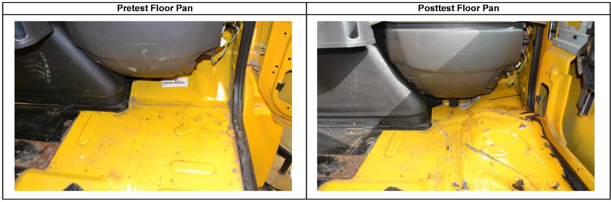
Figure C-2. Floor Pan Deformation Data – Set 2, Test No. MNCBR-1
