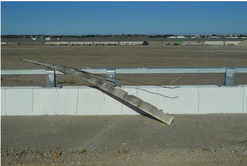
Figure 79. Vehicle Debris on Bridge Railing, Test No. MNCBR-1
