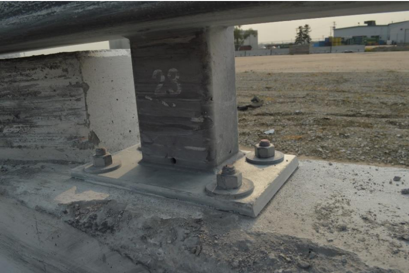
Figure 110. Post No. 23 Damage, Test No. MNCBR-2
