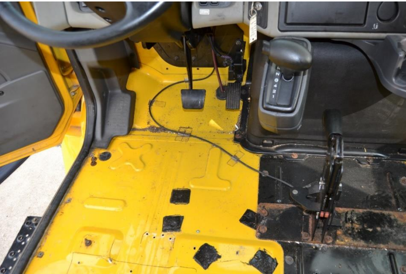
Figure 90. Vehicle Floor Pan Damage, Test No. MNCBR-1
