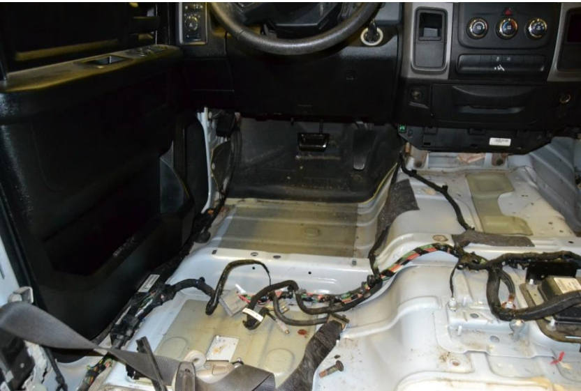
Figure 119. Vehicle Floor Pan Damage, Test No. MNCBR-2
