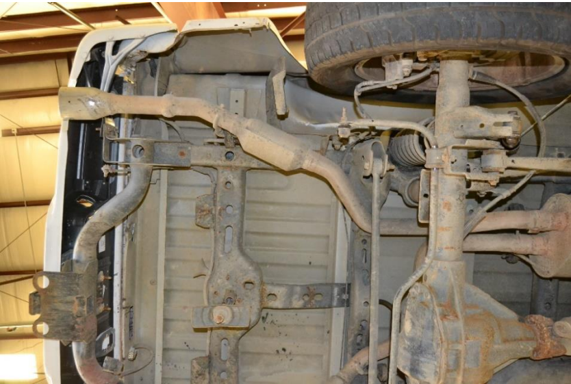
Figure 120. Undercarriage Damage, Test No. MNCBR-2
