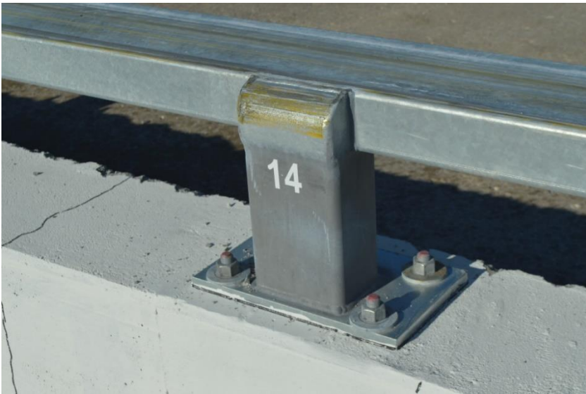
Figure 80. Non-Traffic Side Rail and Post Damage, Post No. 14, Test No. MNCBR-1
