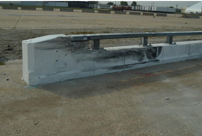
Figure 102. System Damage, Test No. MNCBR-2
