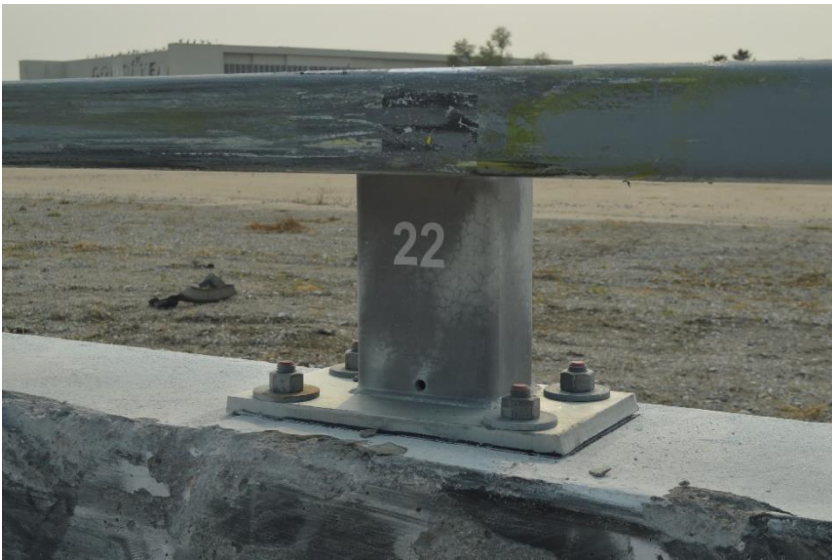
Figure 105. Rail and Post No. 22 Damage, Test No. MNCBR-2
