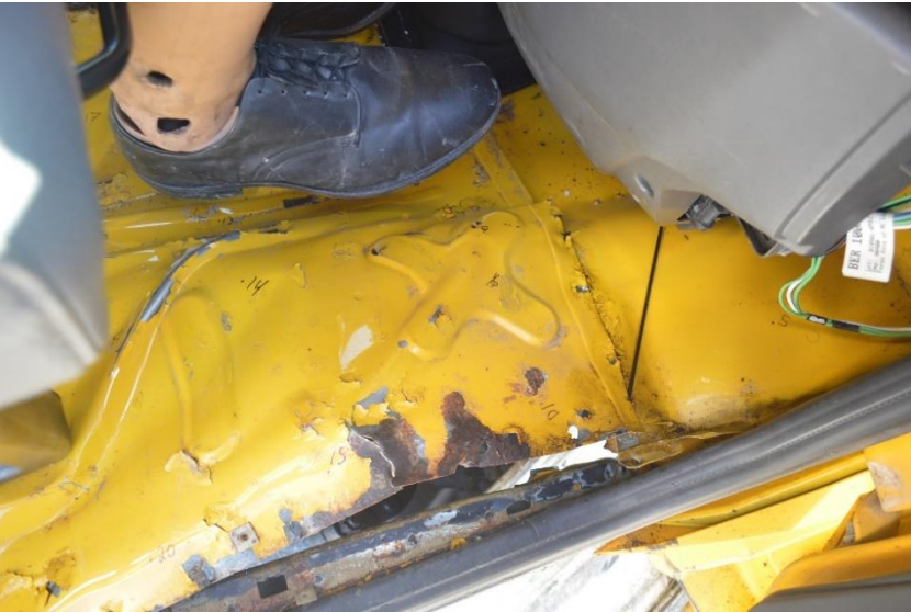
Figure 89. Vehicle Floor Pan Damage, Test No. MNCBR-1
