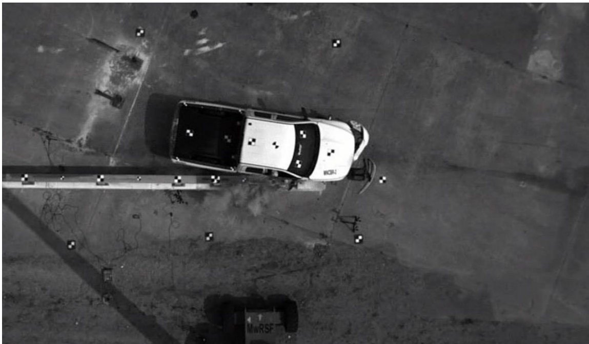
Figure 123. Overhead View of Head Ejection During Impact Event, Test No. MNCBR-2
