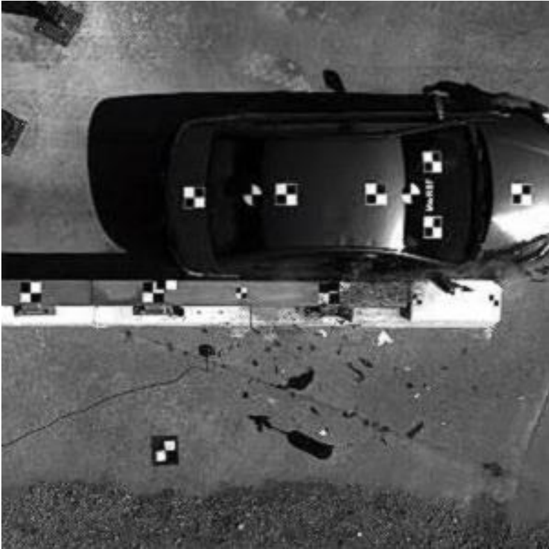
Figure 148. Overhead View of Head Ejection During Impact Event, Test No. MNCBR-3
