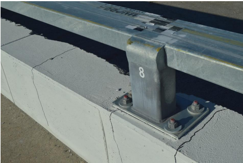
Figure 74. Rail and Post Damage, Post No. 8, Test No. MNCBR-1
