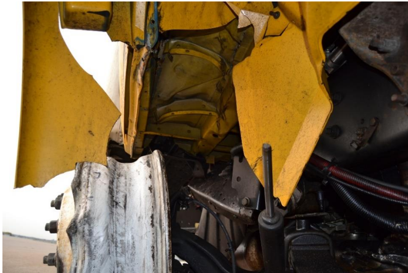
Figure 91. Undercarriage Damage, Test No MNCBR-1
