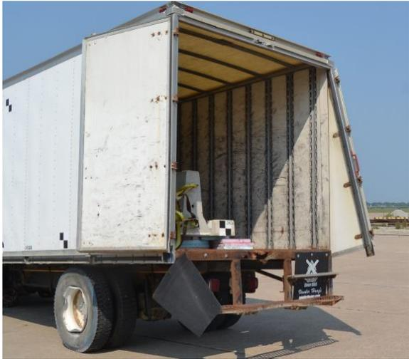
Figure 54. Rear Vehicle Damage, Test No. 4CBR-1
