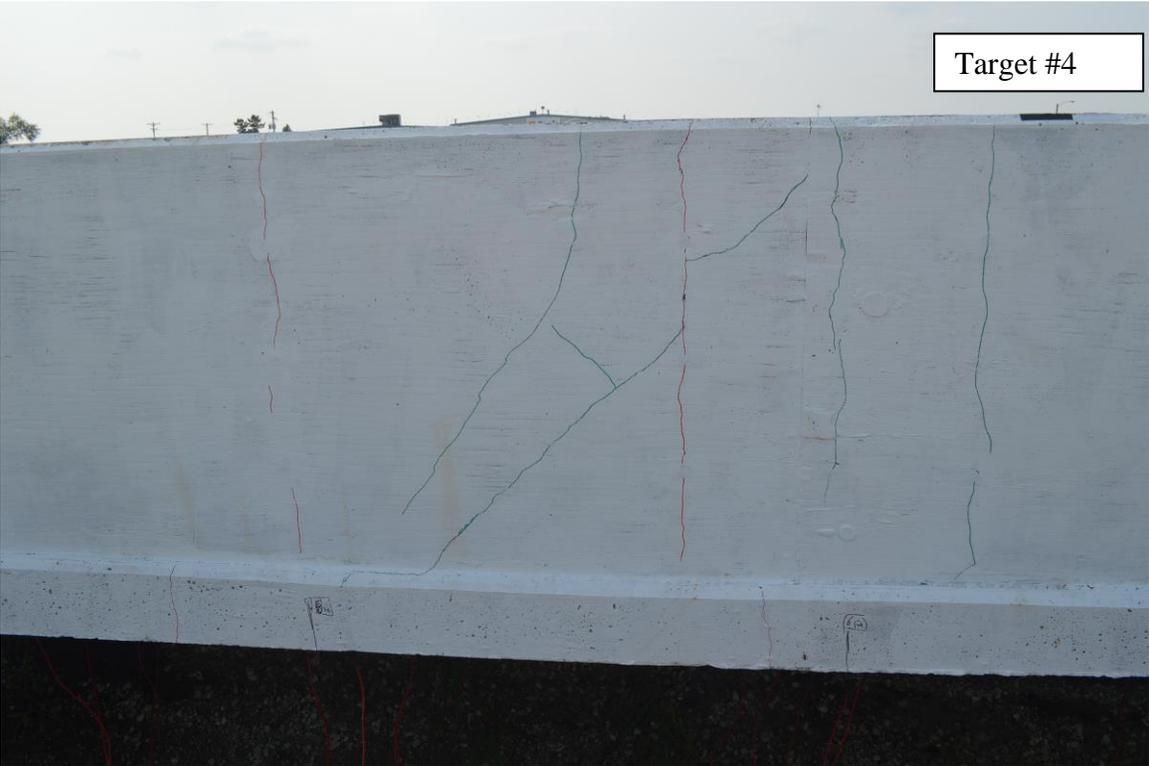
Note: Red lines are shrinkage cracks present before testing. Green lines are cracks from impact.
