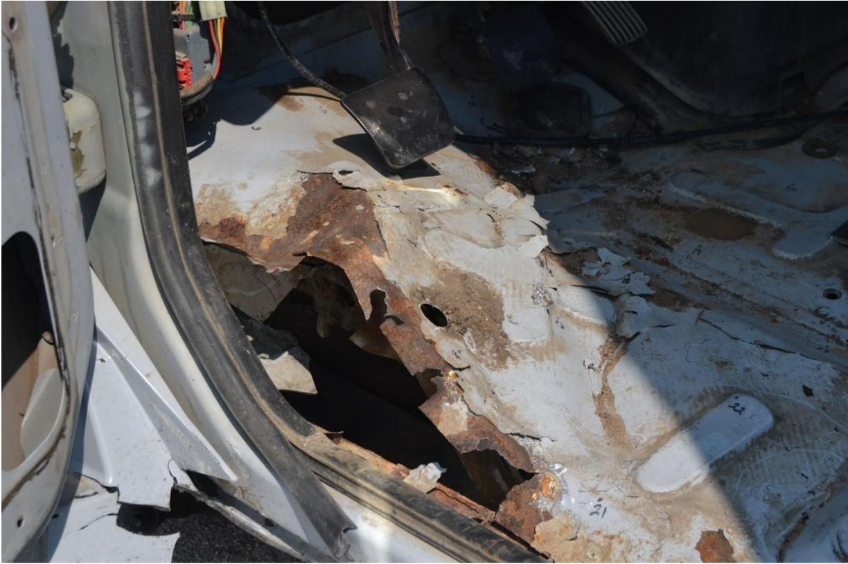
Figure 56. Post-Test Floor Pan Photos, Test No. 4CBR-1
