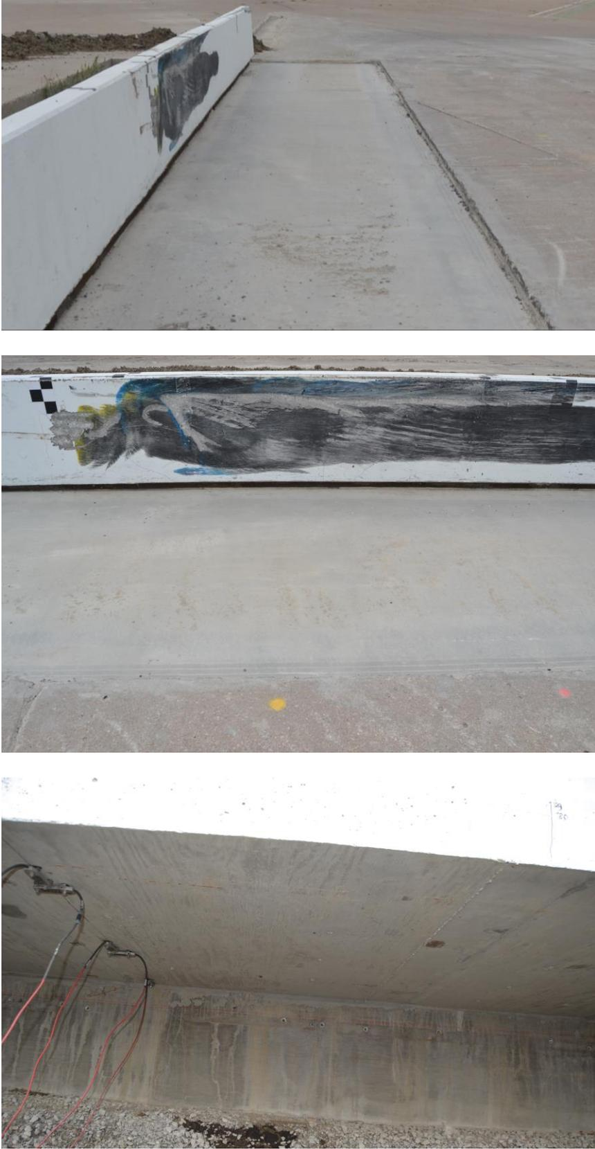
Figure 50. Deck Damage, Test No. 4CBR-1
