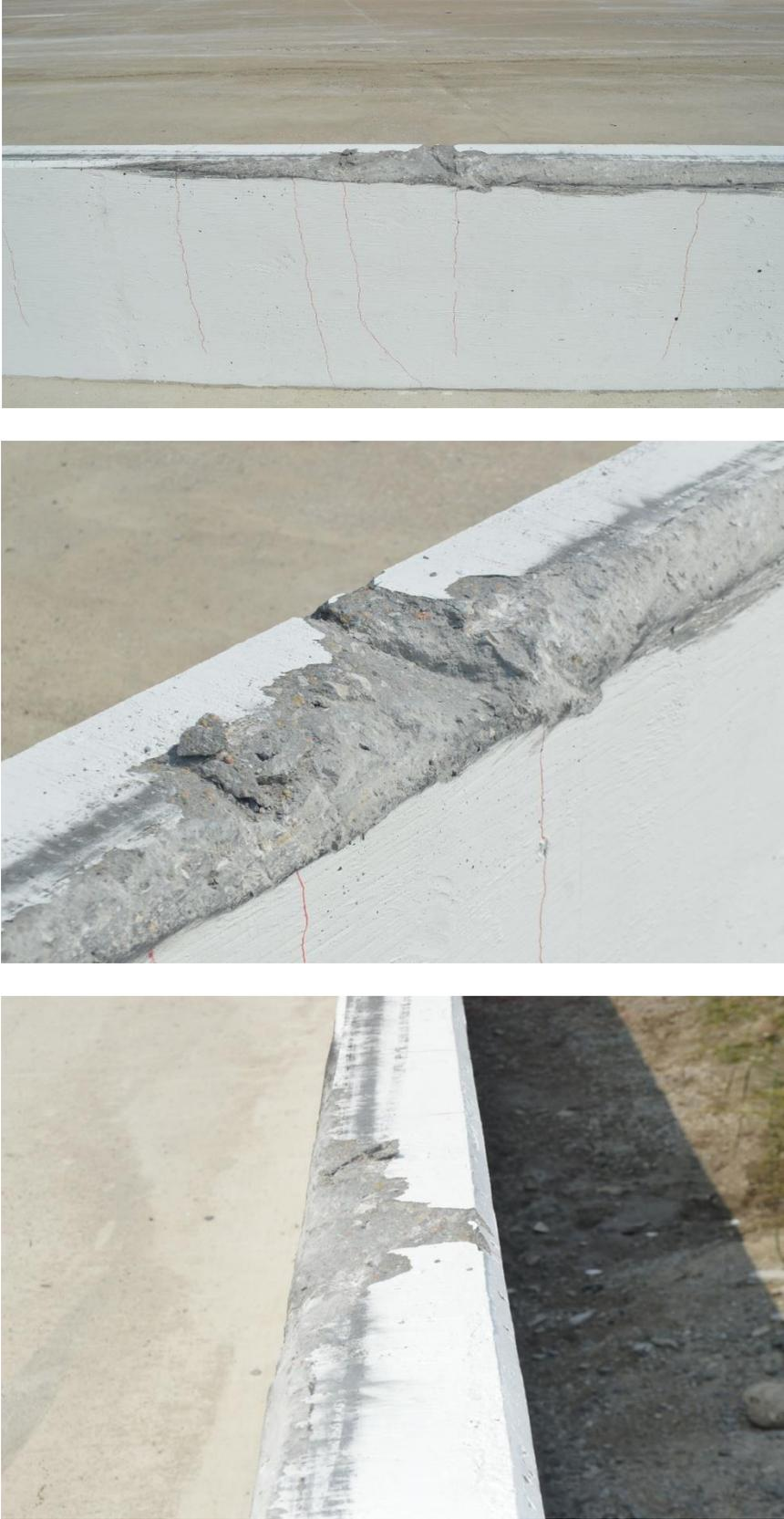
Figure 48. System Damage, Downstream Gouge Details, Test No. 4CBR-1
