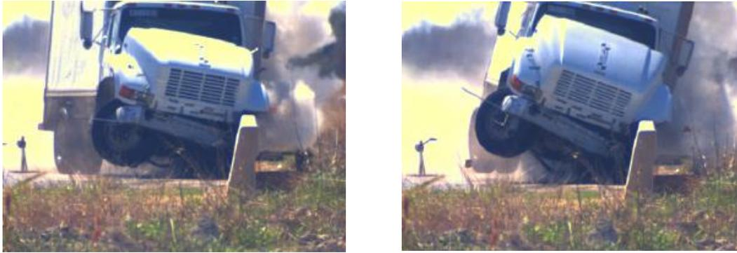
Figure 4. SUT Stability in TL-4 Test with 36-in. Tall Barrier [9]
