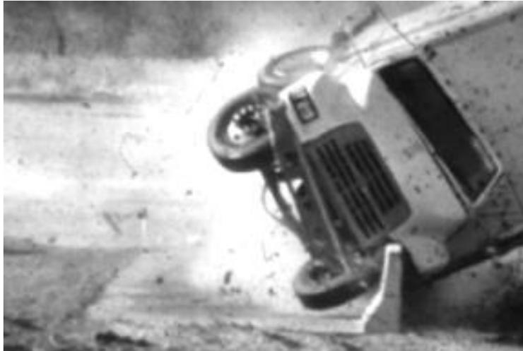
Figure 2. SUT Rollover in TTI TL-4 Test with 32-in. Tall Barrier [5]
