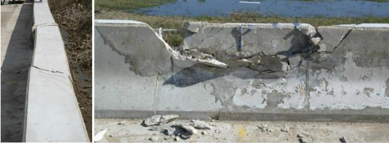
Figure 6. Punching Shear Failures of Concrete Barriers [29]
