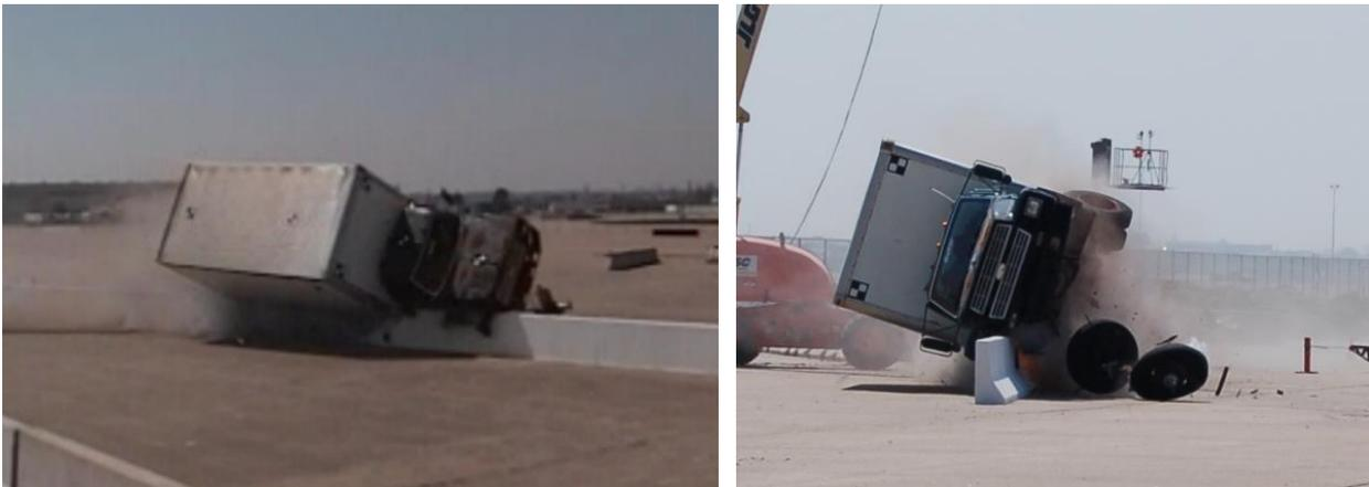
Figure 1. SUT Rollover in MwRSF TL-4 Test with 32-in. Tall Barrier [4]
