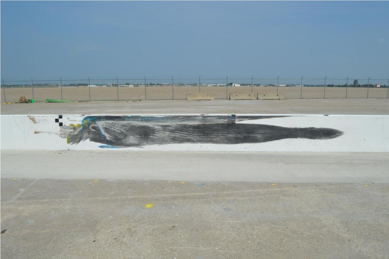
Figure 47. Overall System Damage, Test No. 4CBR-1
