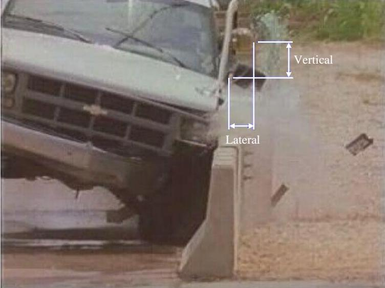
Figure 12. Measurement of Head Ejection Envelope [7]
