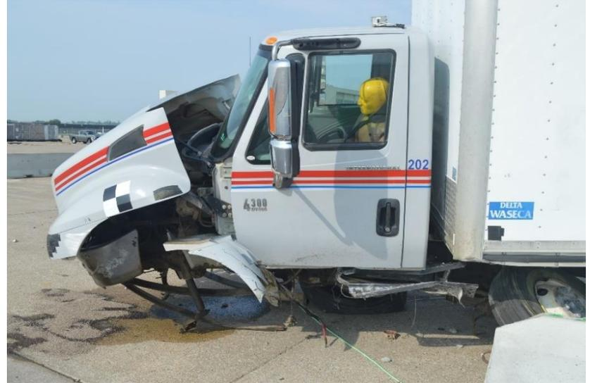
Figure 53. Left- and Right-Side Vehicle Damage, Test No. 4CBR-1
