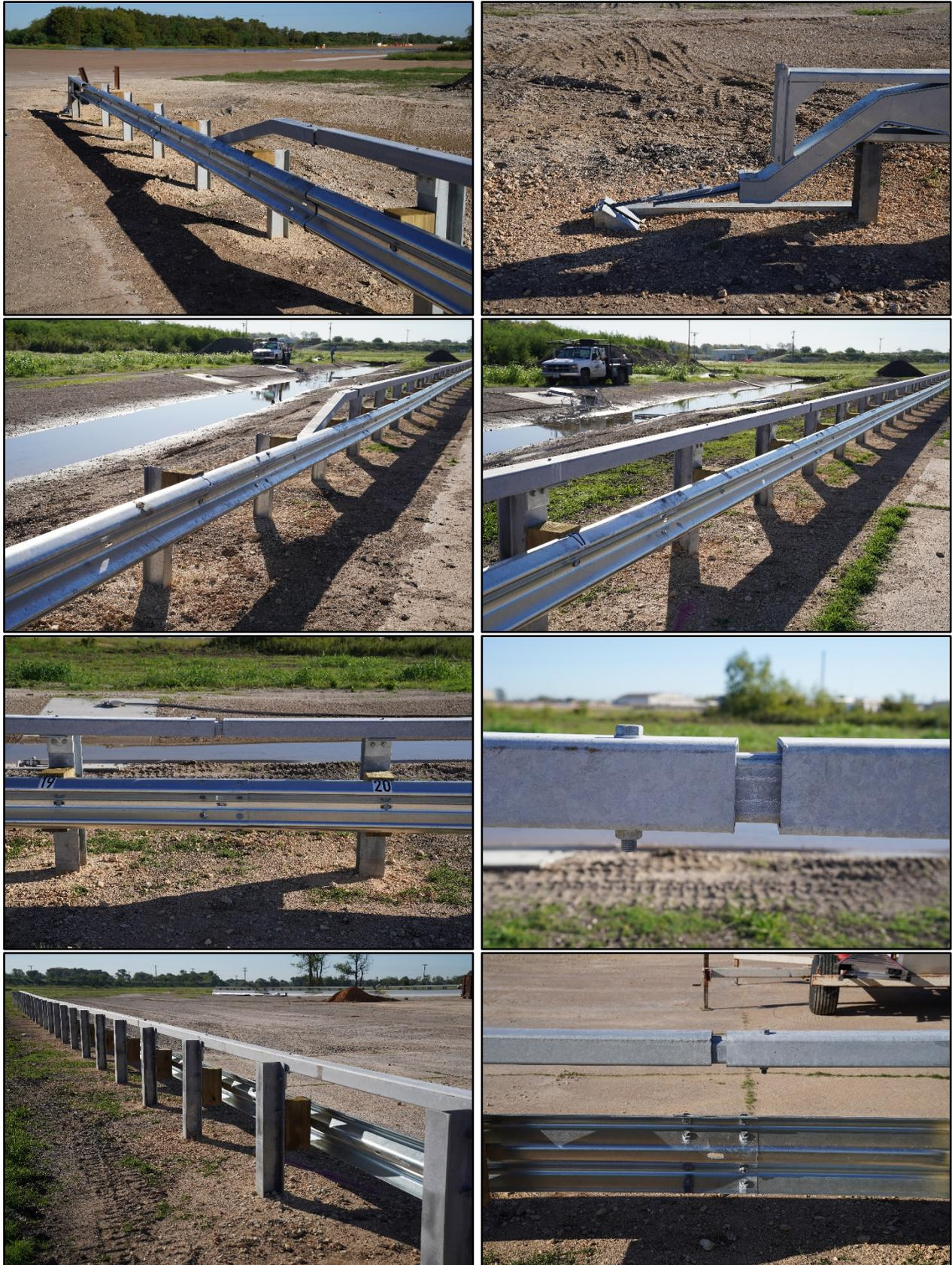
**Figure 3.2. MASH TL-4 Guardrail System prior to Testing.**
