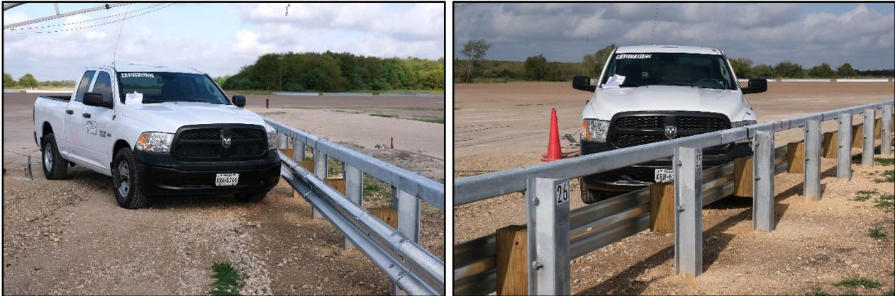
**Figure 8.1. Guardrail System/Test Vehicle Geometrics for Test No. 440190-01-2.**
