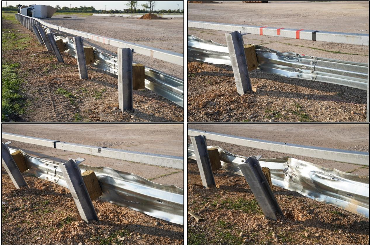
**Figure 6.5. Field Side of Guardrail after Test No. 440190-01-1.**
