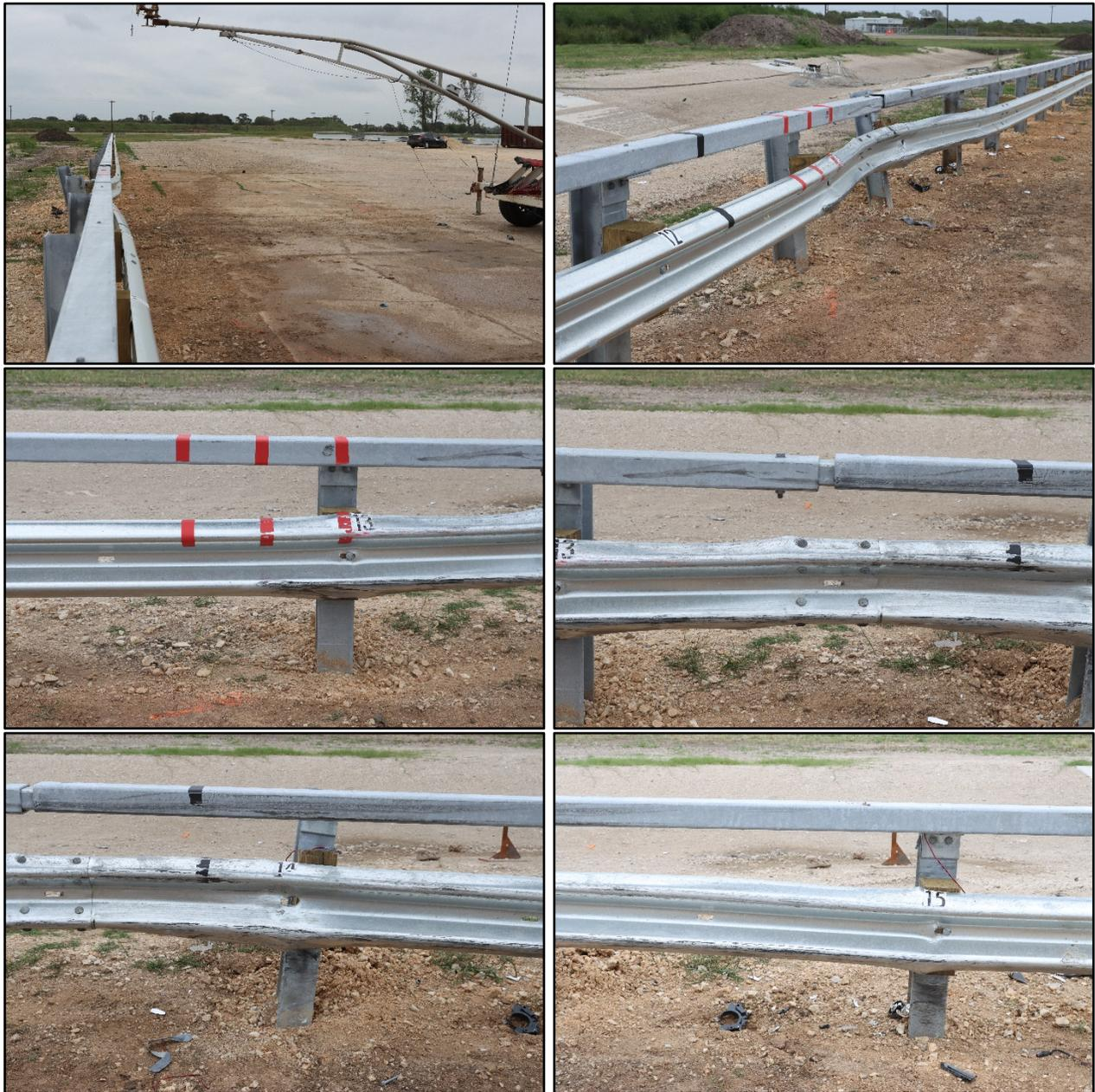
**Figure 7.3. Guardrail after Test No. 440190-01-3.**
