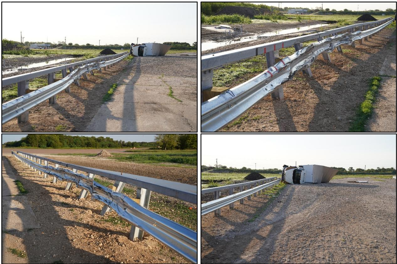
**Figure 6.3. Guardrail after Test No. 440190-01-1.**
