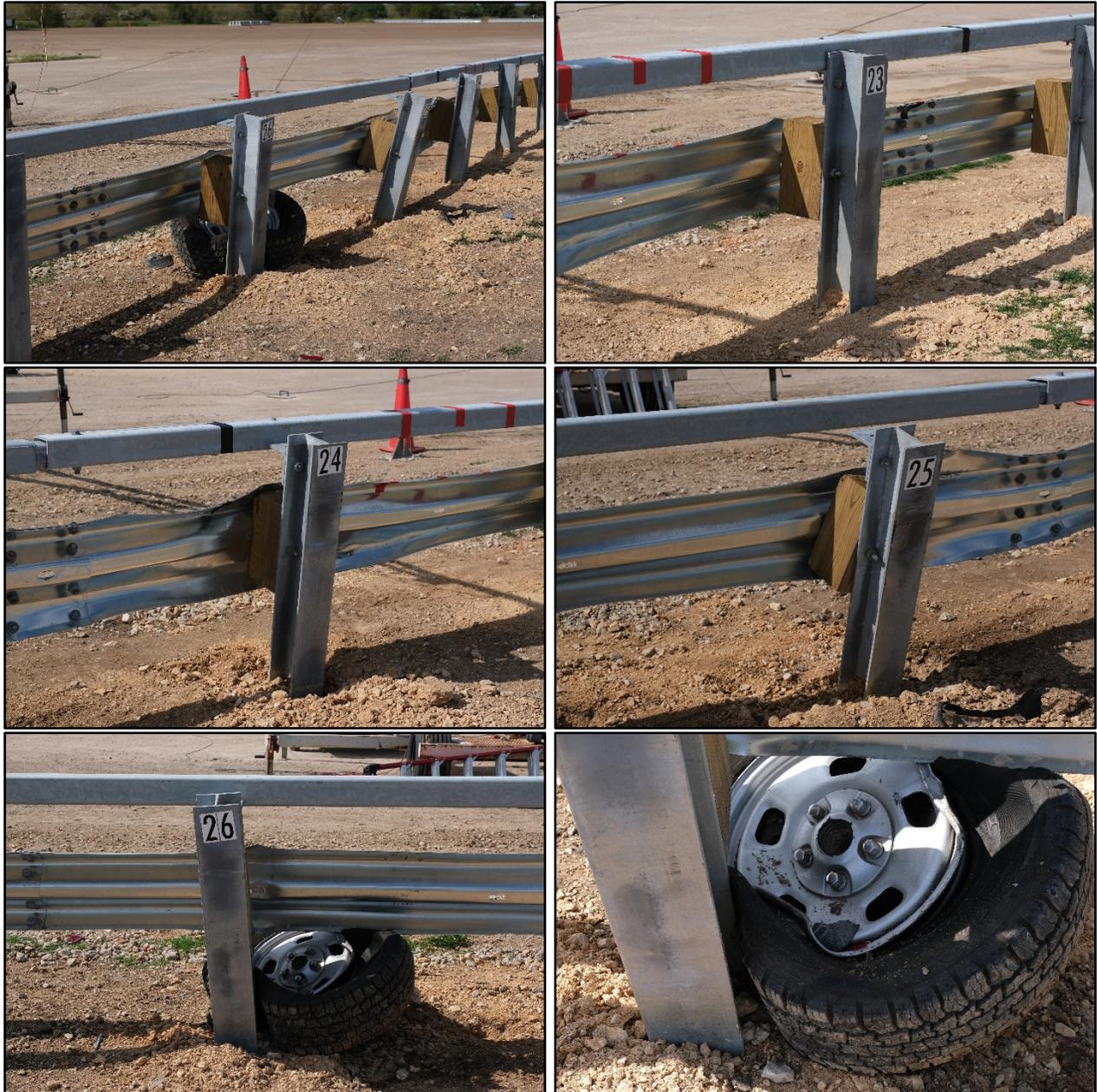
**Figure 8.4. Field Side of Guardrail after Test No. 440190-01-2.**
