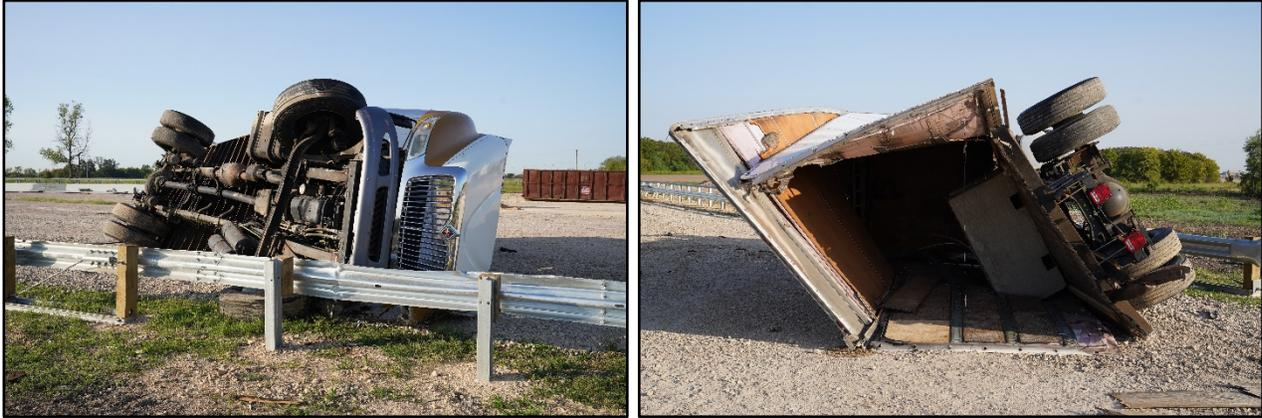
**Figure 6.6. Test Vehicle after Test No. 440190-01-1.**
