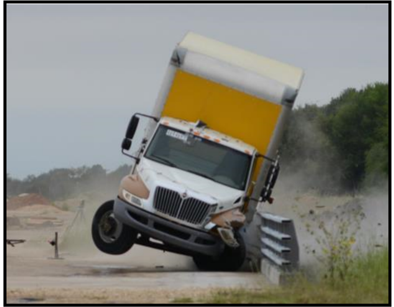
Crash test of MASH Test 4-12 on the TxDOT C1W Bridge Rail.
