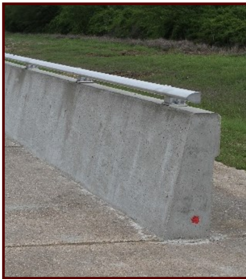
Image of the tested barrier design with bridge railing from MASH Test 3-11.
