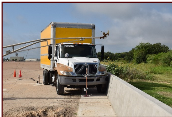
Image of single unit truck at CIP of the Moment Slab Foundation.
