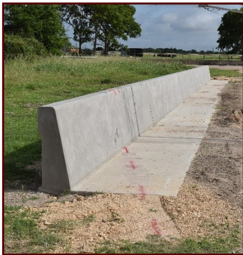
Image of the Moment Slab Foundation installed at the testing site.
