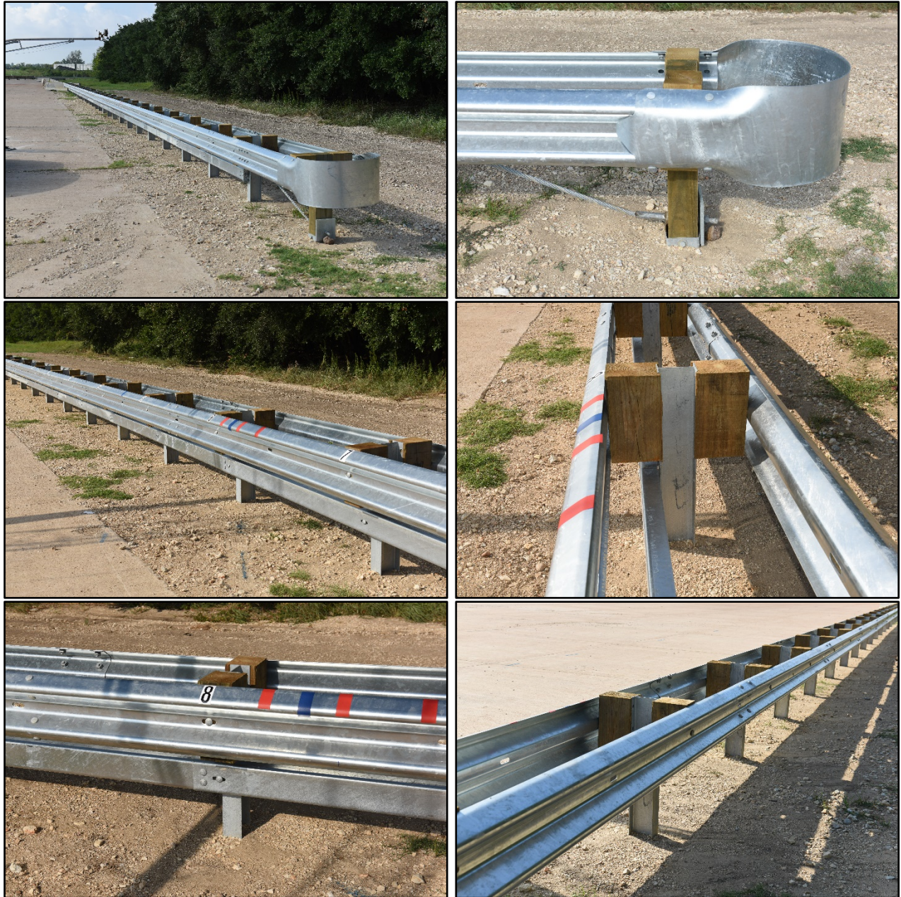
Figure 2.2. W-Beam Median Barrier with Rub Rail Prior to Testing.
