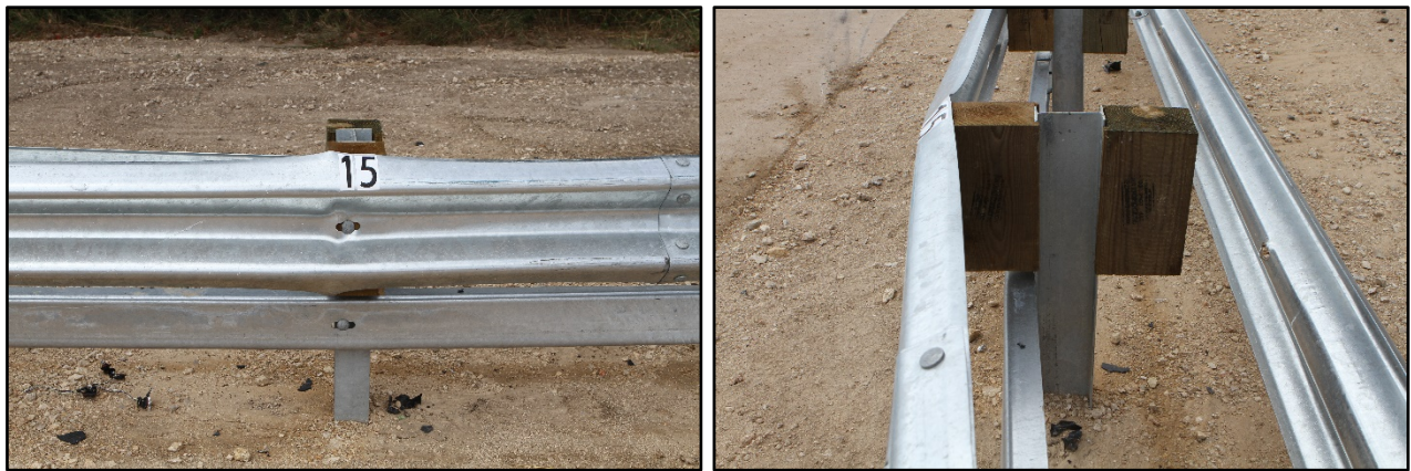
Figure 6.8. Median Barrier after Test No. 611971-03-2.
