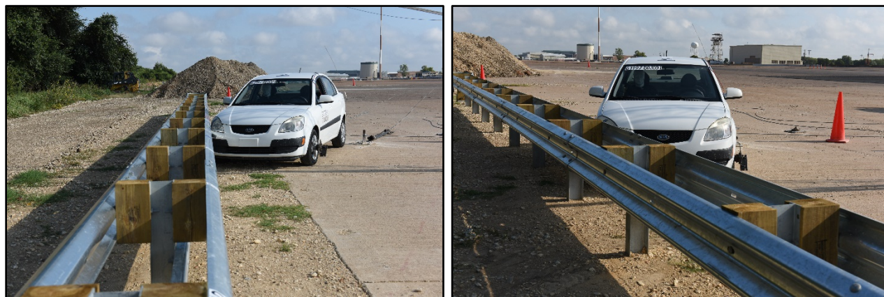
Figure 5.1. Median Barrier/Test Vehicle Geometrics for Test No. 611971-03-1.
