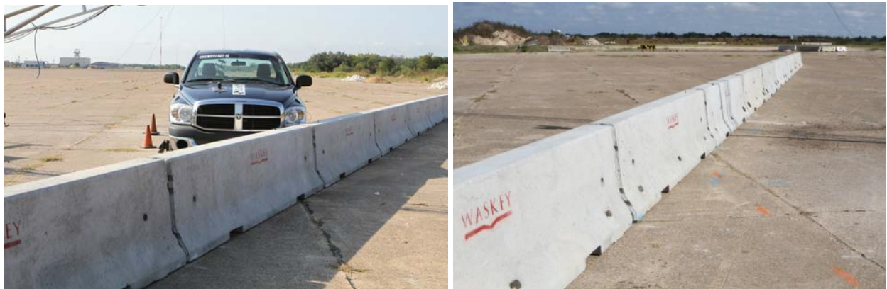
Figure 20. Test installation of free-standing to pinned-down concrete barrier transition installed on concrete pavement.
