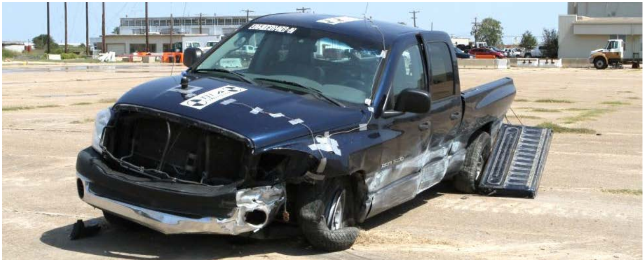
Figure 21. Test installation after crash testing.
