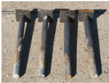
Figure 13. Anchoring pins after the test.
