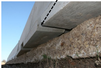
Figure 12. Barrier deflection and damage after the crash test.
