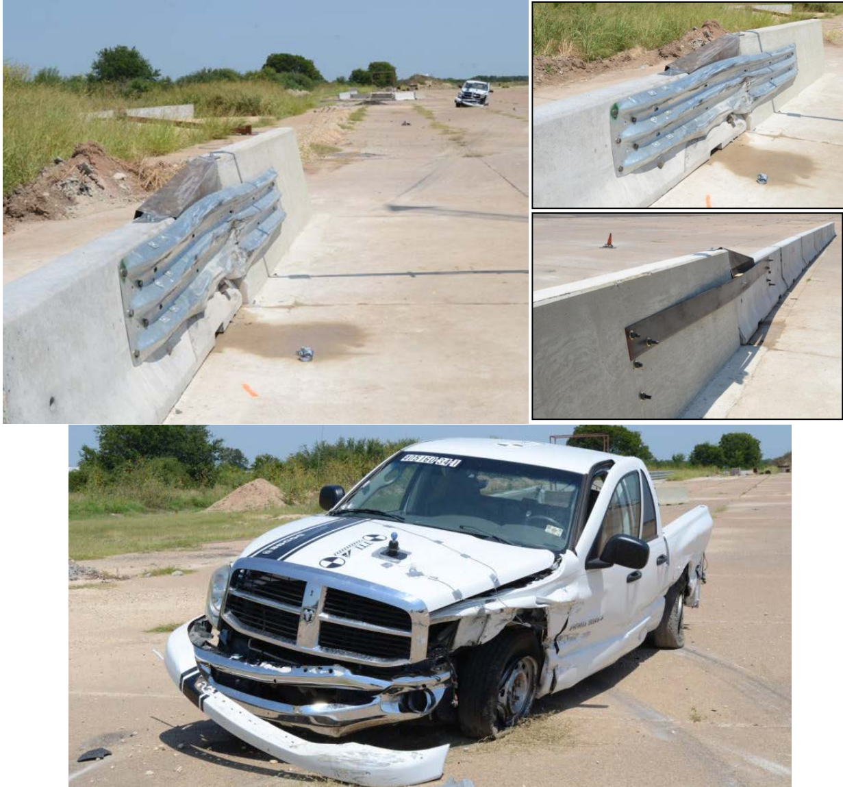
Figure 25. Transition test installation after crash testing.
