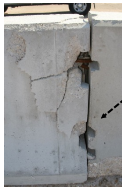
Figure 12. Barrier deflection and damage after the crash test.
