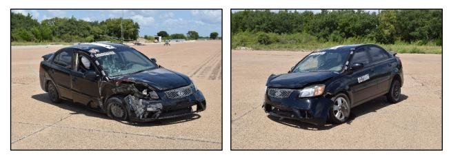
Figure 6.4. Test Vehicle after Test No. 469689-2-1.
