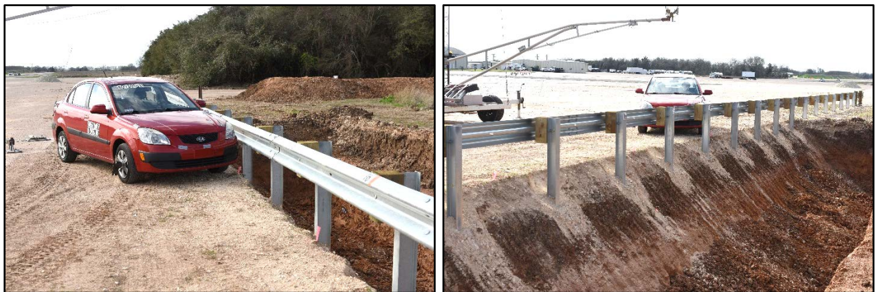
Figure 2.2. Guardrail on 1H:1V Slope/Test Vehicle Geometrics for Test No. 609301-01-1.
