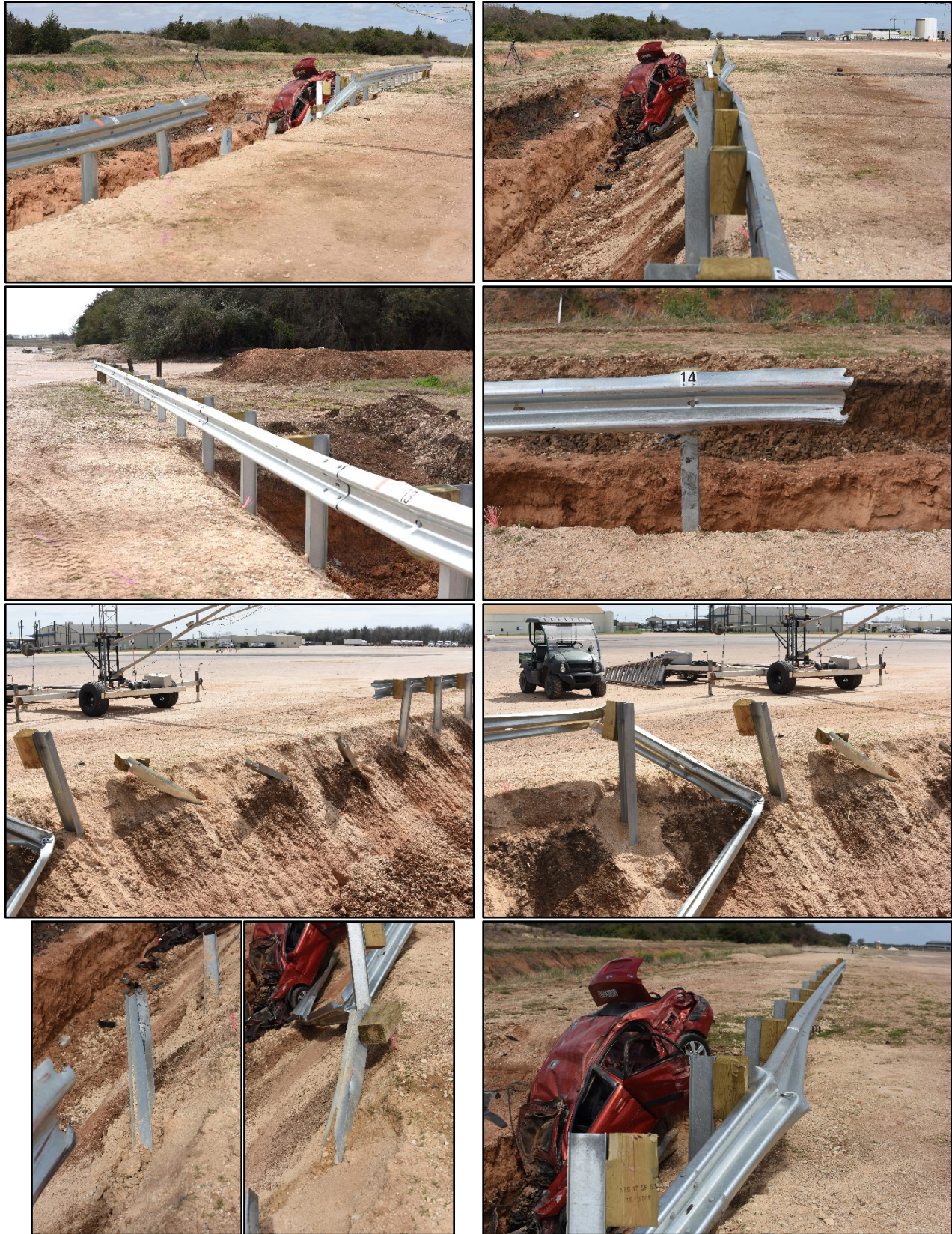
Figure 2.3. Guardrail on 1H:1V Slope after Test No. 609301-01-1.
