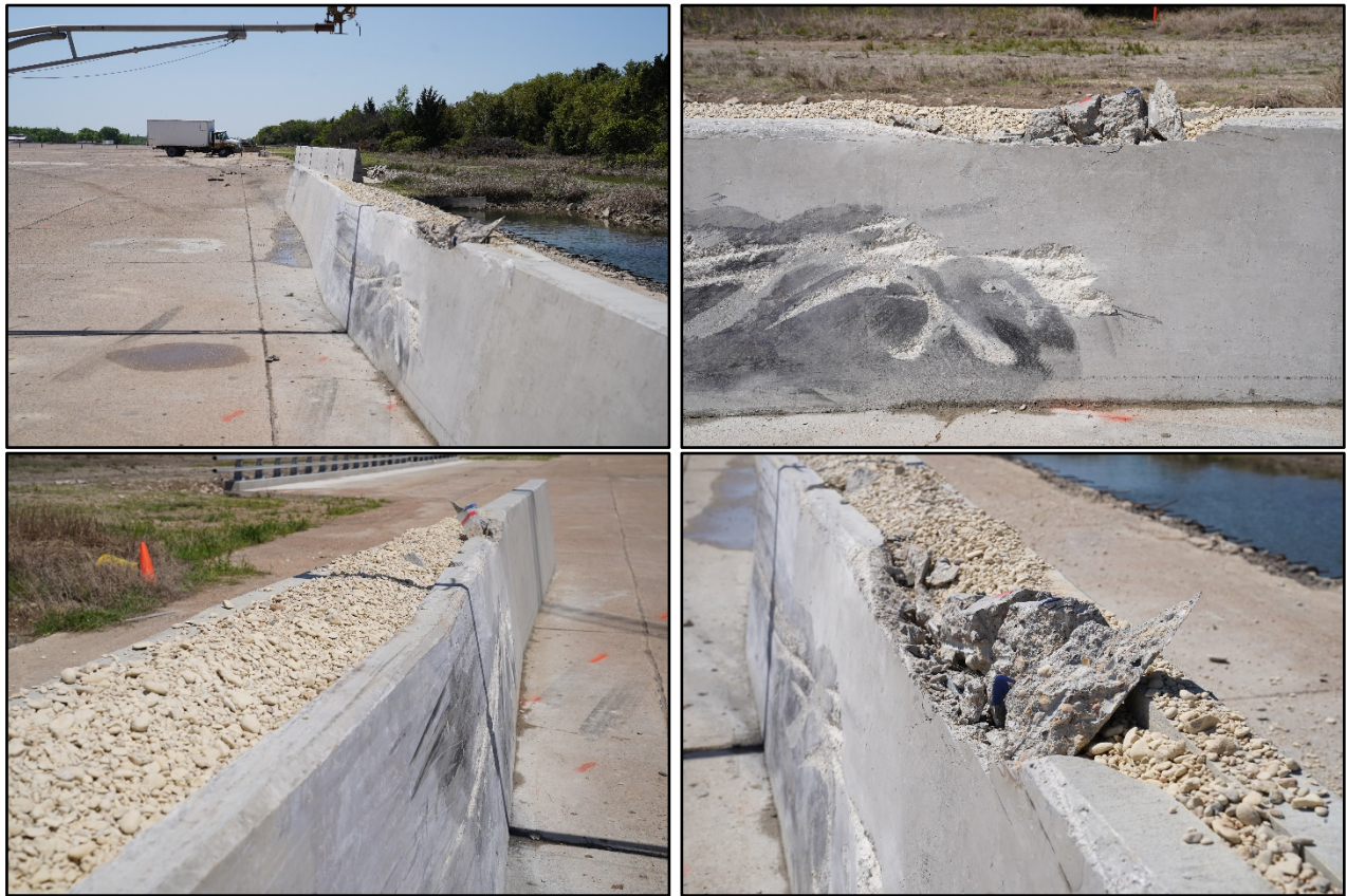
Figure 8.3. Barrier System after Test No. 611901-05-1.
