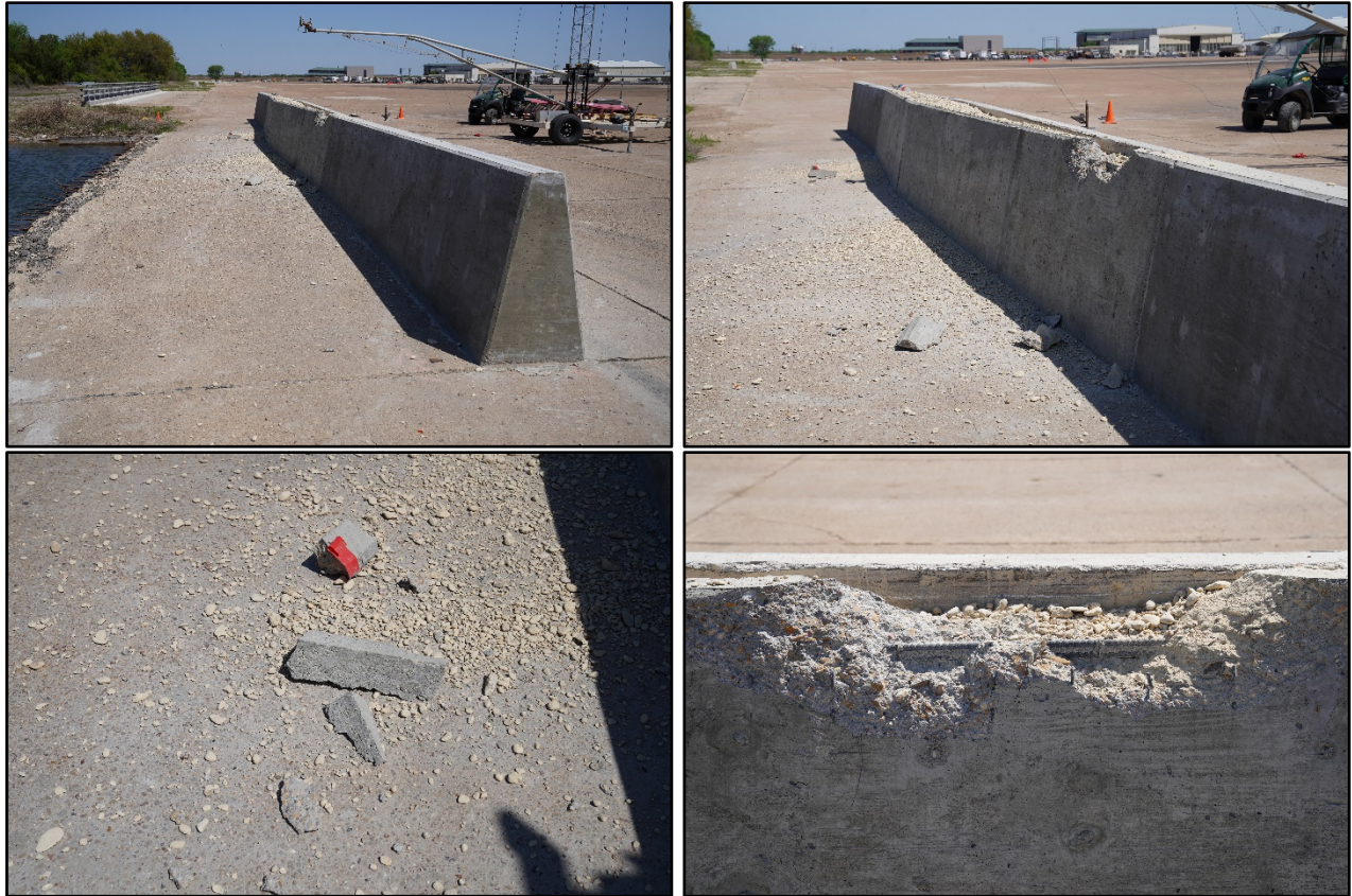
Figure 8.4. Field Side of Barrier System after Test No. 611901-05-1.
