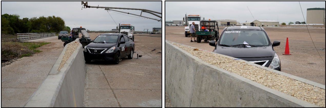
Figure 6.1. Barrier System/Test Vehicle Geometries for Test No. 611901-03-1.
