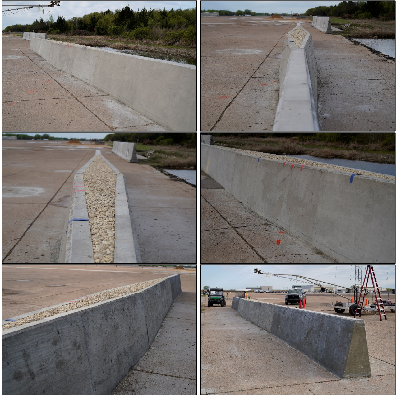
Figure 3.2. Critical Flare Concrete Barrier System prior to Testing.
