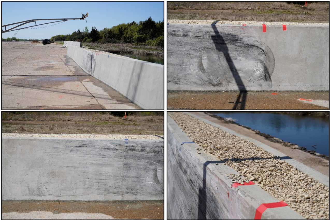
Figure 7.3. Barrier System after Test No. 611901-04-1.
