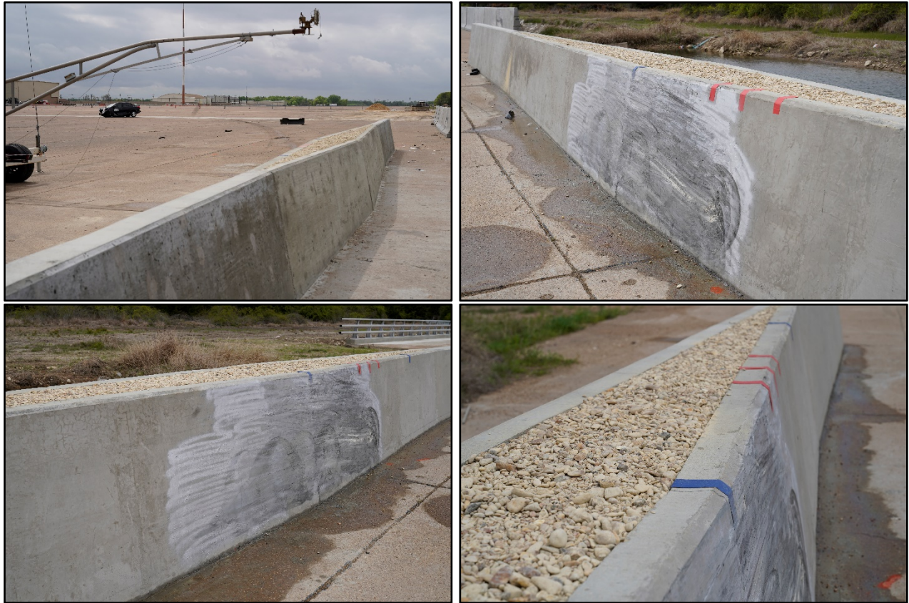
Figure 6.3. Barrier System after Test No. 611901-03-1.
