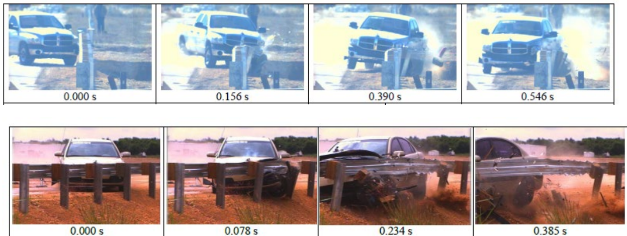
Figure 1.7. Sequential of MASH Tests 3-11 and 3-10 of the Guardrail on 2H:1V Slope System.
