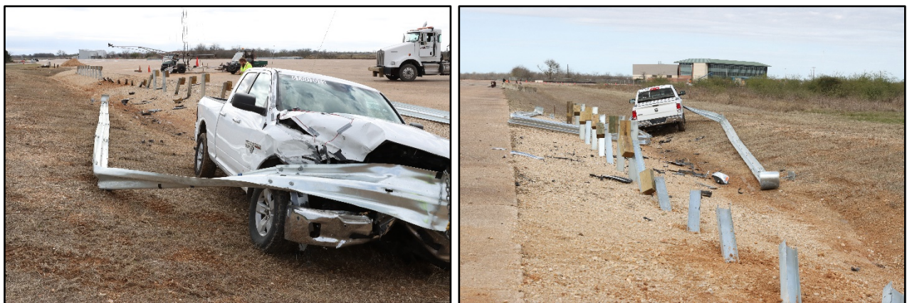
Figure 8.3. Guardrail after Test No. 613011-01-2.
