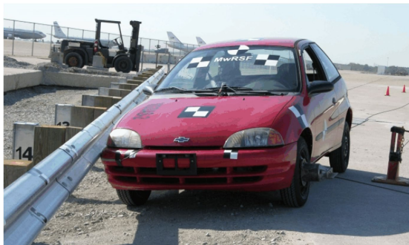
Figure 1.3. NCHRP Report 350 Small Car at Impact Point of MSG Guardrail on 8H:1V Slope (MwRSF Report TRP-03-188-08).
