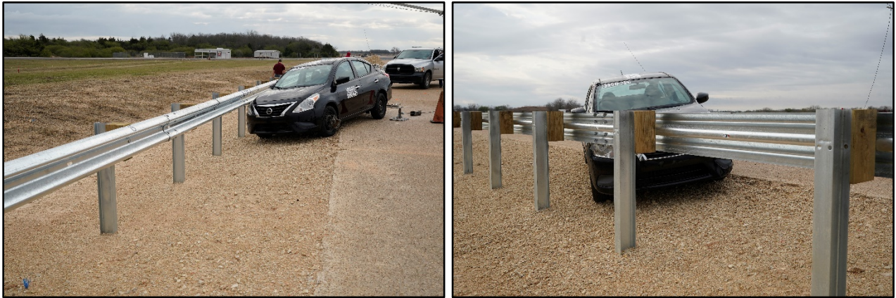
Figure 7.1. Guardrail/Test Vehicle Geometrics for Test No. 613011-01-1.
