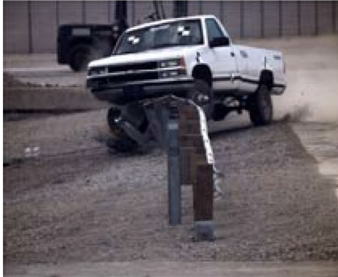
Figure 1.4. Pickup Truck almost Overriding MSG Guardrail on 8H:1V Slope (MwRSF Report TRP-03-188-08).
