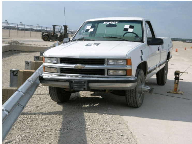
Figure 1.2. NCHRP Report 350 Pickup Truck at Impact Point of MSG Guardrail on 8H:1V Slope (MwRSF Report TRP-03-188-08).
