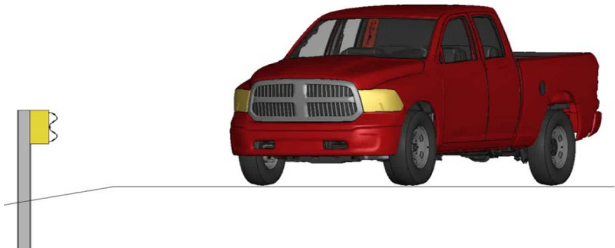
Figure 3.7. Truck Setting with Option 1 W-Beam Guardrail with 24-inch Offset.
