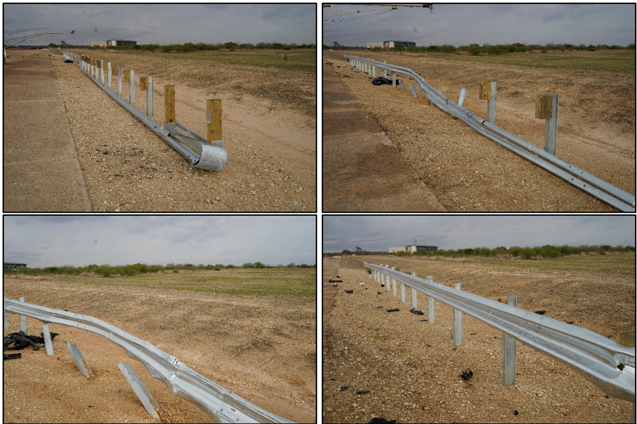
Figure 7.3. Guardrail on 6H:1V Slope after Test No. 613011-01-1.
