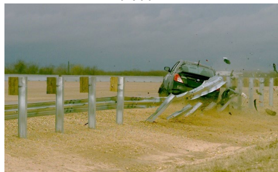
Figure D.2. Sequential Photographs for Test No. 613011-01-1 (Rear View).
