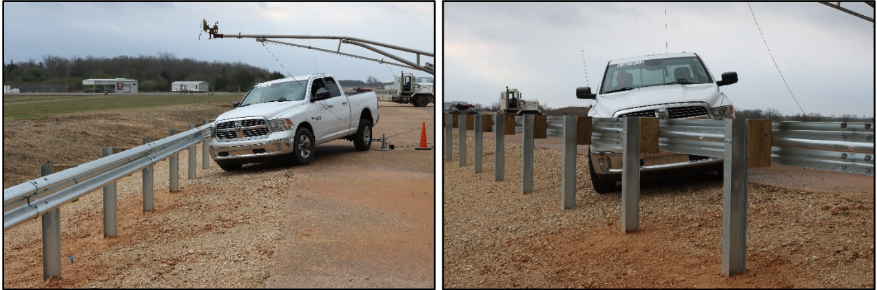
Figure 8.1. Guardrail/Test Vehicle Geometrics for Test No. 613011-01-2.
