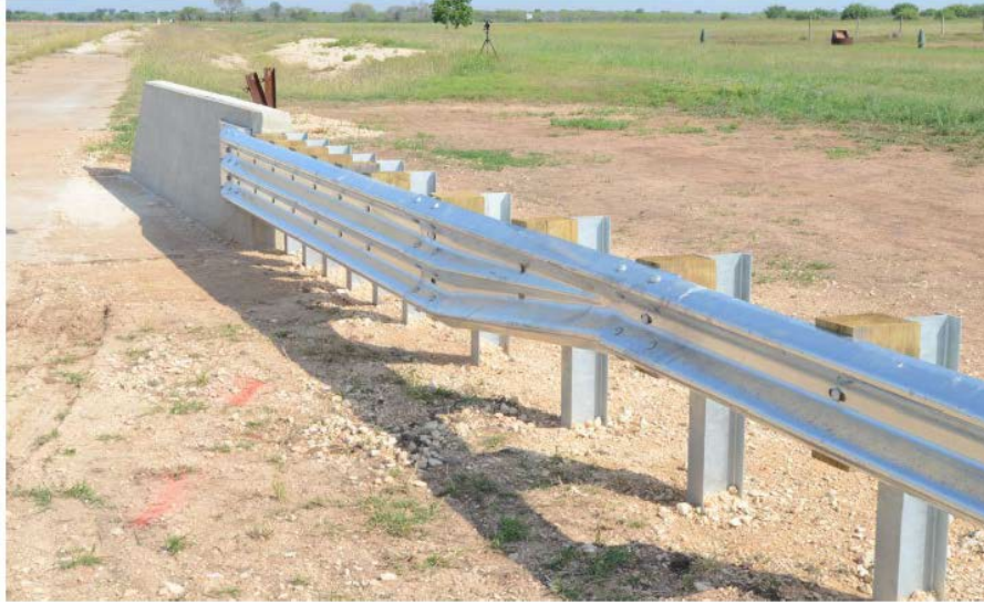
Figure 2.2. Simplified Thrie Beam transition without Curb and Rubrail.
