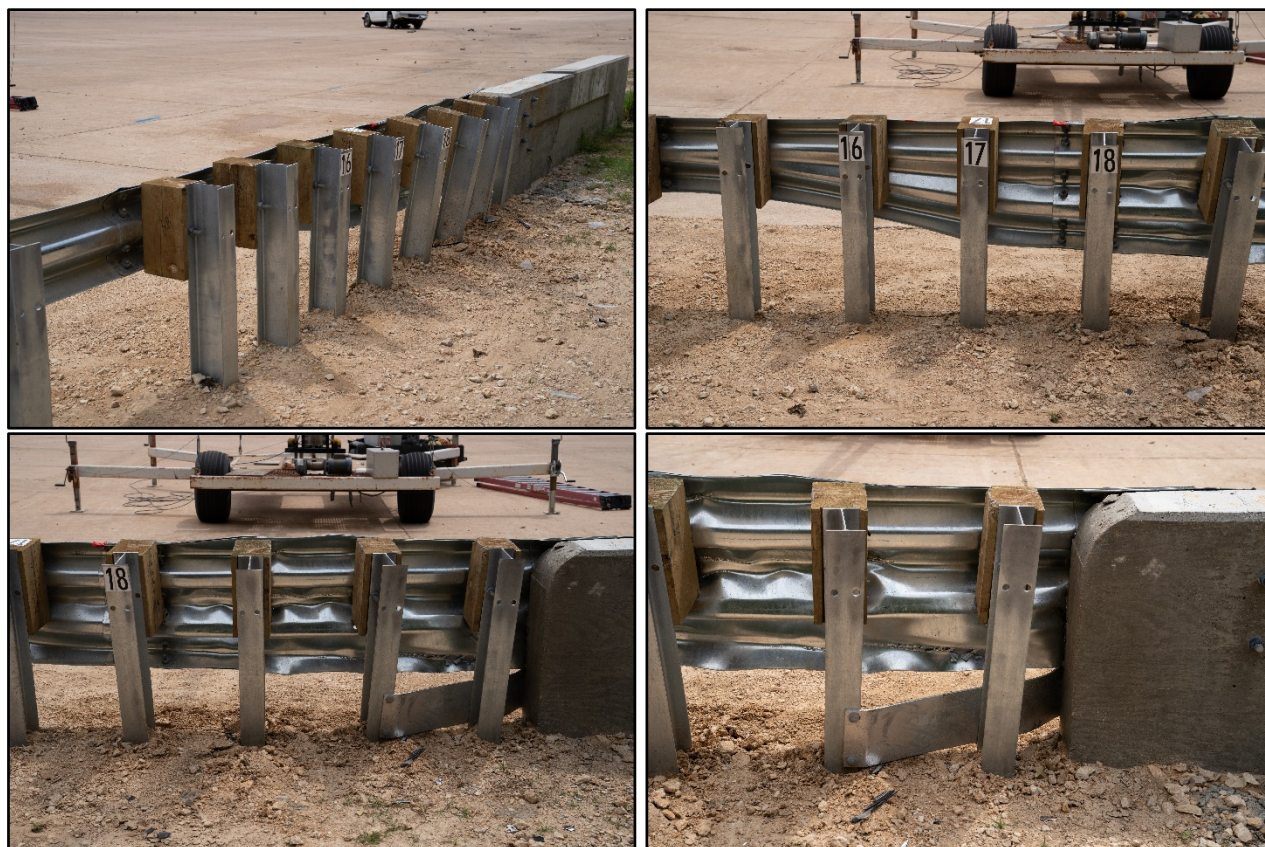
Figure 7.4. Field Side of Transition after Test No. 613121-01-1.
