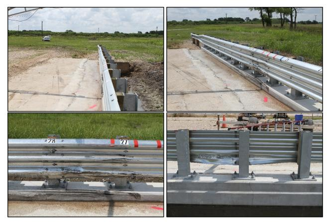
Figure 6.3. Bridge Rail Retrofit after Test No. 615131-01-1.
