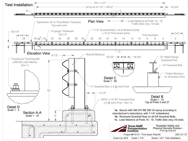
Q:\Accreditation-17025-2017\EIR-000 Project Files\615131 - Thrie-Beam Bridge Rail Development - Williams\Drafting, 615131\615131 Drawing Figure 2.1. Details of Thrie Beam Bridge Rail Retrofit.
