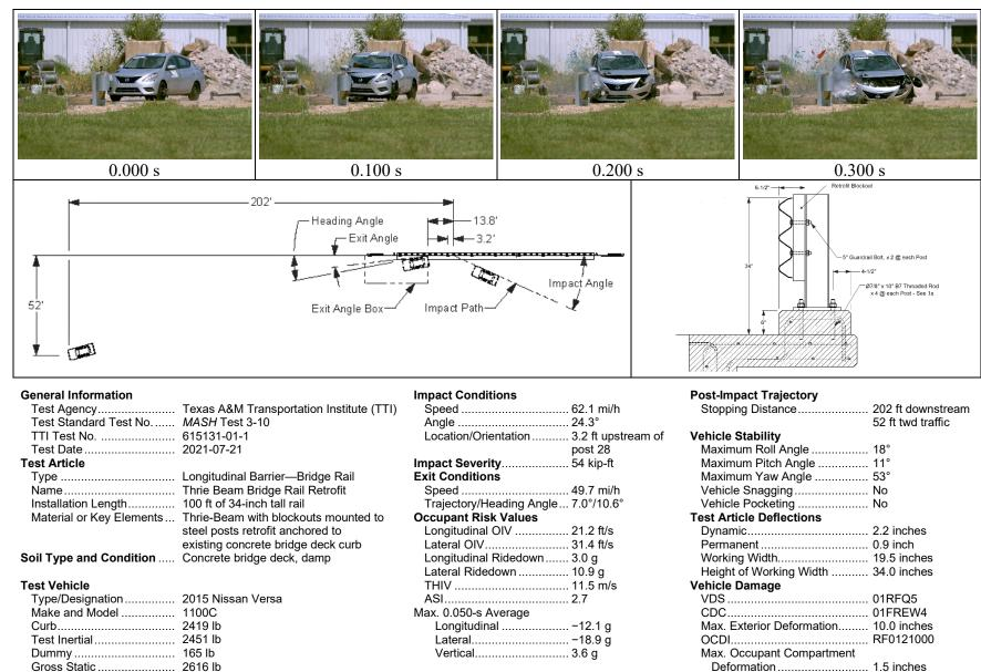
Figure 6.6. Summary of Results for MASH Test 3-10 on Thrie Beam Bridge Rail Retrofit.
