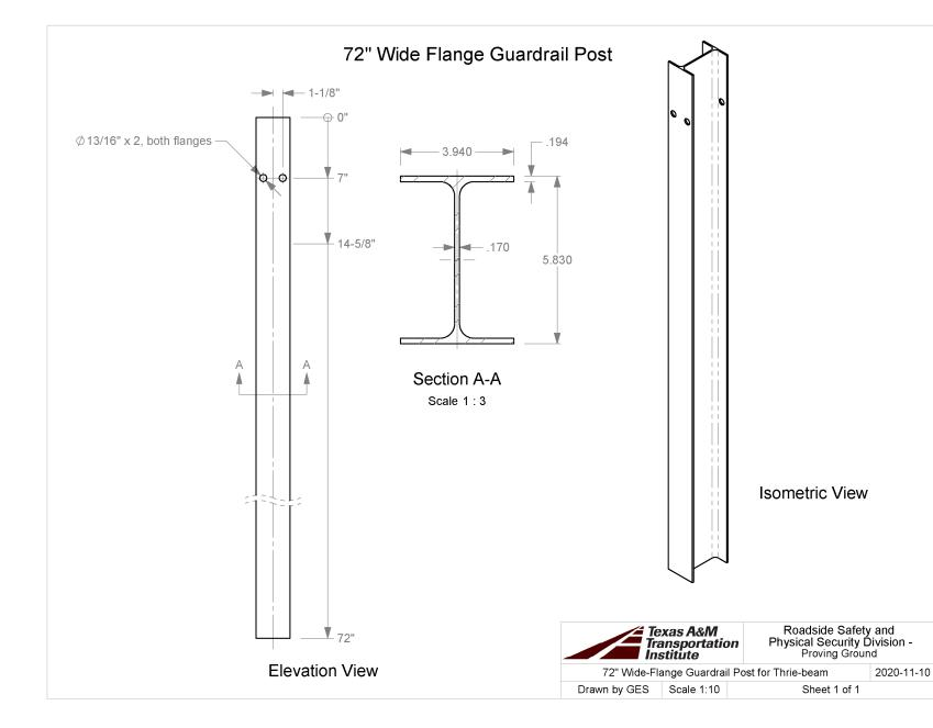
T:\Drafting Department\Solidworks\Standard Parts\Guardrail Parts and Subs\Guardrail Drawings\Post, 72" Wide Flange for W-beam
