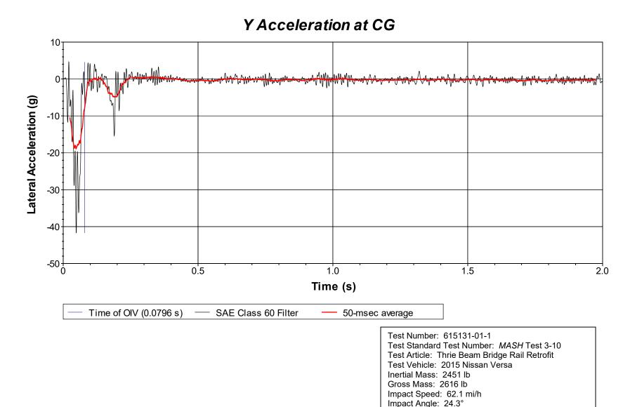
Figure E.5. Vehicle Lateral Accelerometer Trace for Test No. 615131-01-1 (Accelerometer Located at Center of Gravity).
