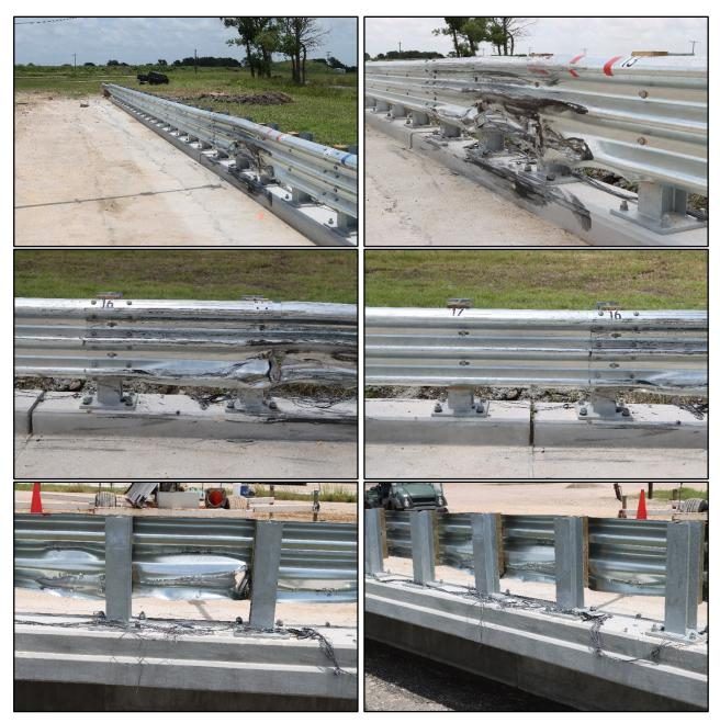
Figure 5.3. Bridge Rail Retrofit after Test No. 612131-01-2.
