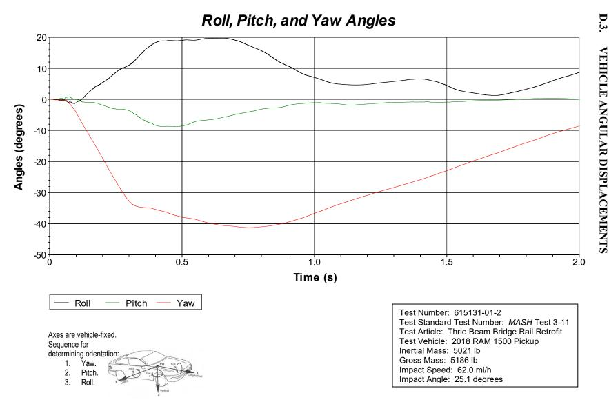
Figure D.3. Vehicle Angular Displacements for Test No. 615131-01-2.
