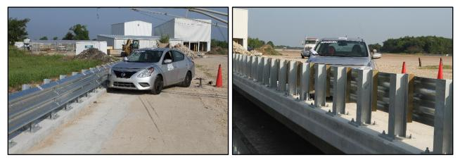
Figure 6.1. Bridge Rail Retrofit/Test Vehicle Geometrics for Test No. 615131-01-1.
