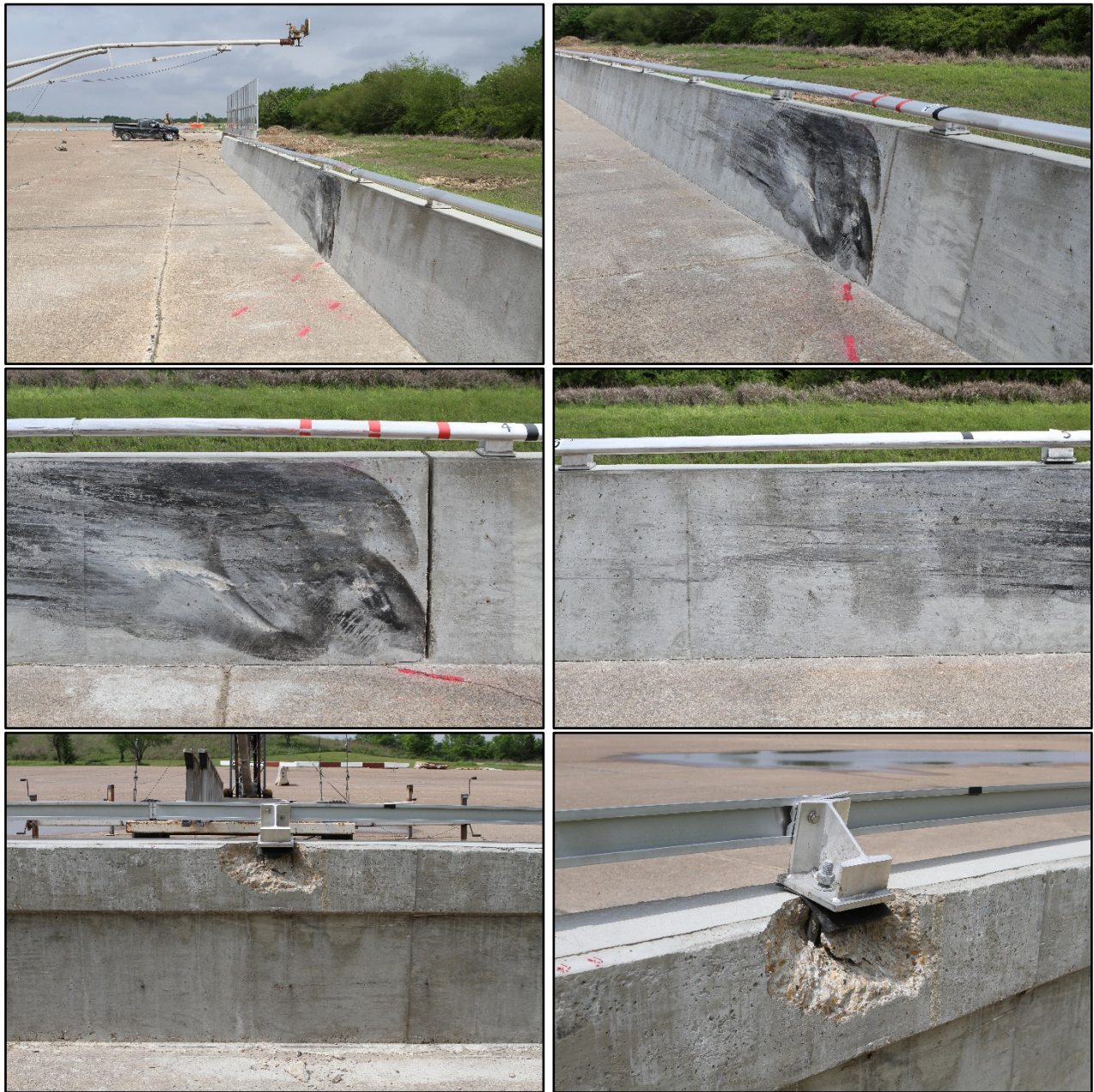
Figure 5.3. Bridge Rail after Test No. 611971-02-1.
