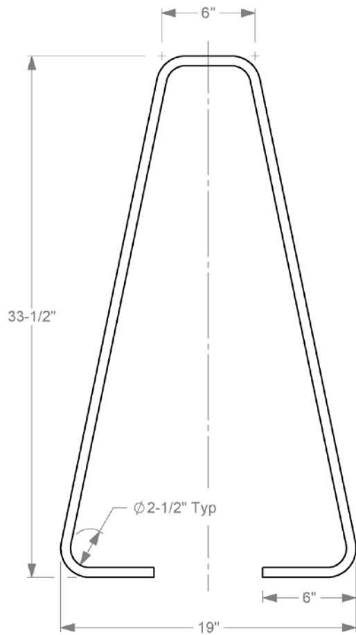
5R-bar Ø5/8" Grade 60 Rebar
