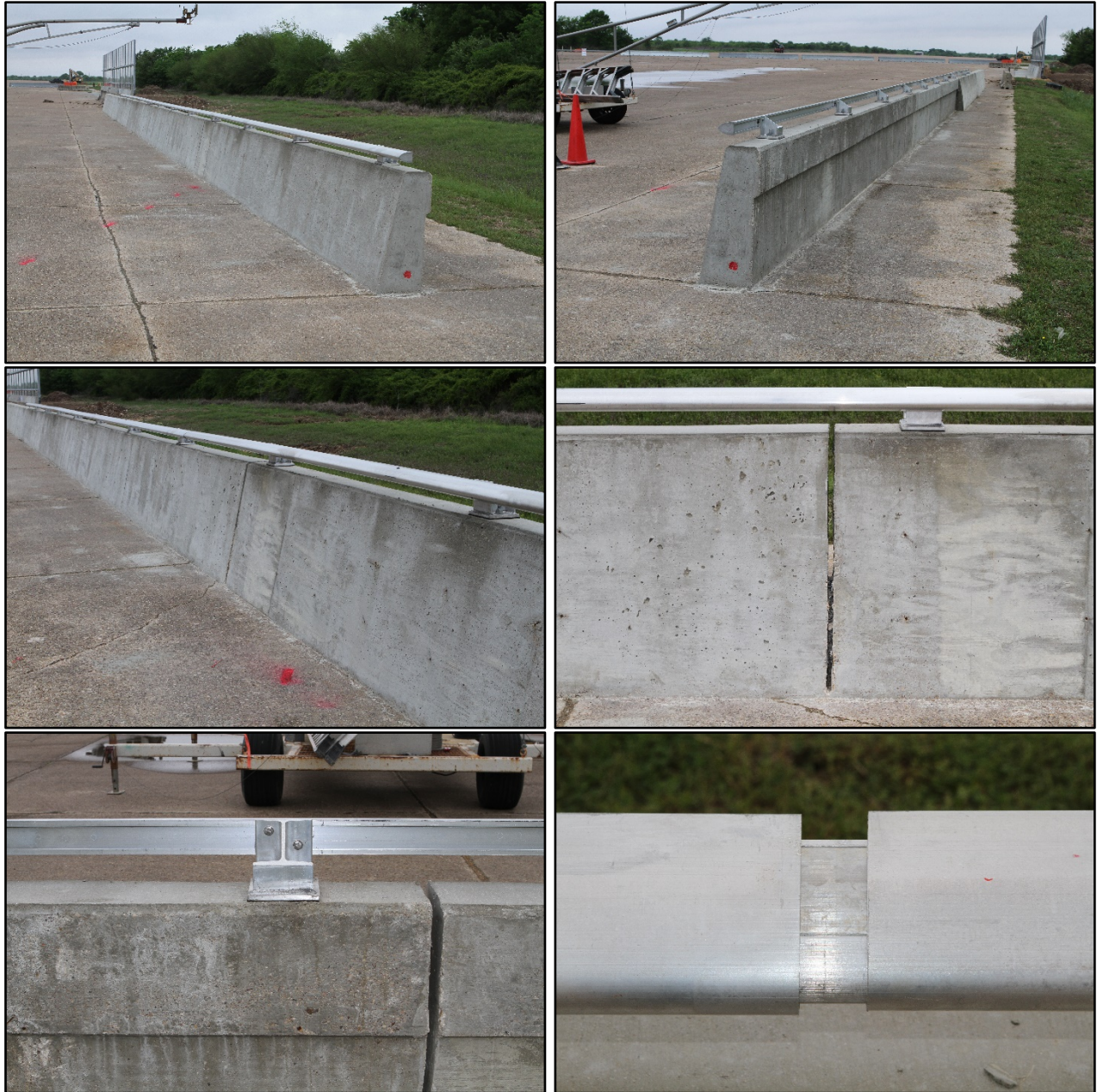
Figure 2.2. 42-inch Tall Combination Traffic-Pedestrian-Bicycle Bridge Rail System prior to Testing.
