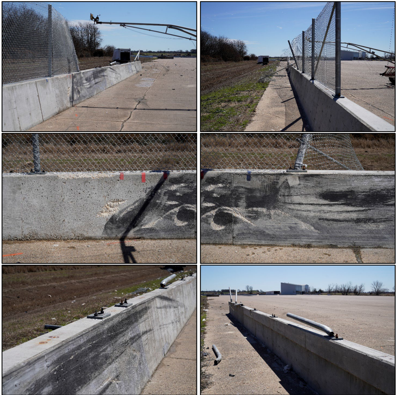
Figure 5.5. CMB after Test No. 613131-03-2.
