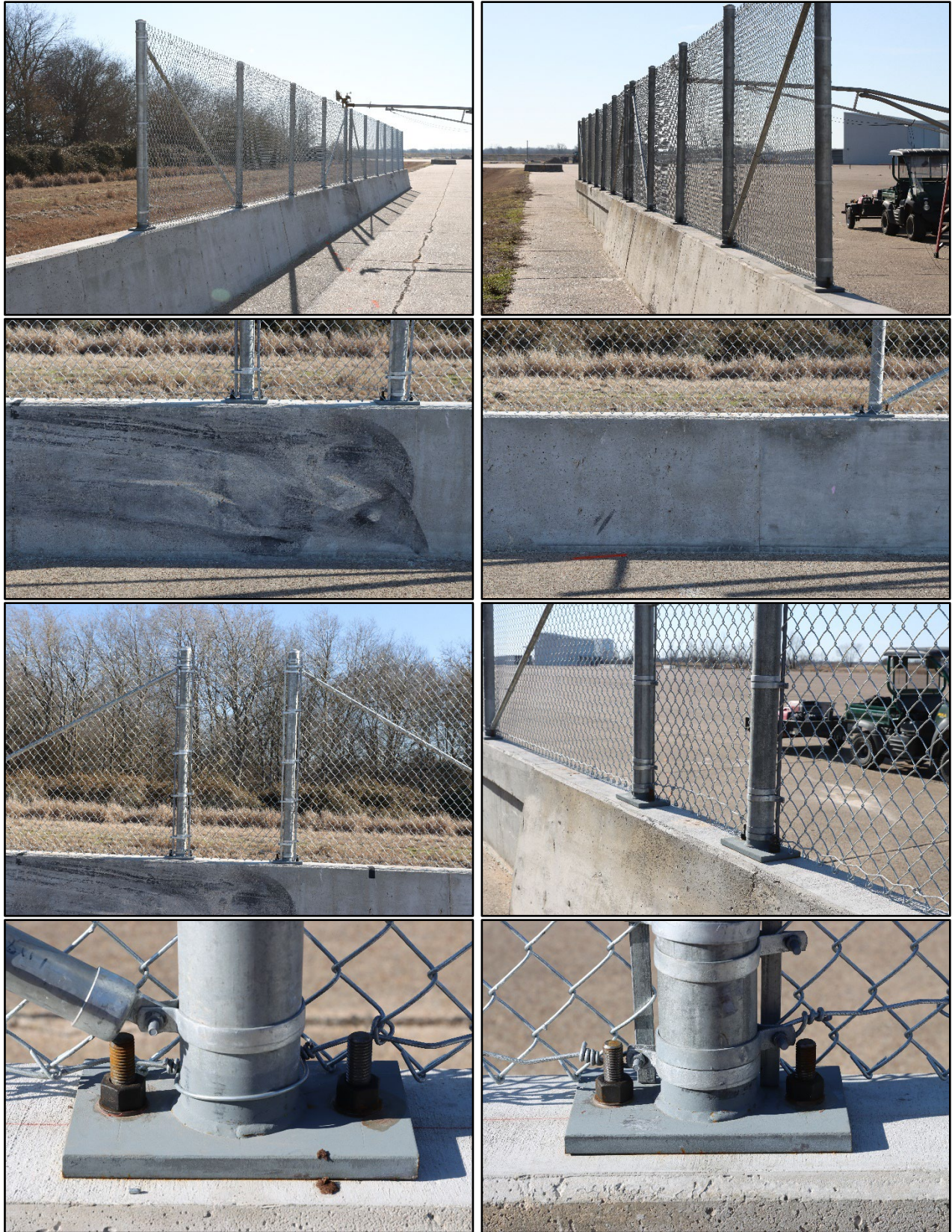
Figure 5.2. CMB with Fence Mounted on Top prior to Test No. 613131-01-2.
