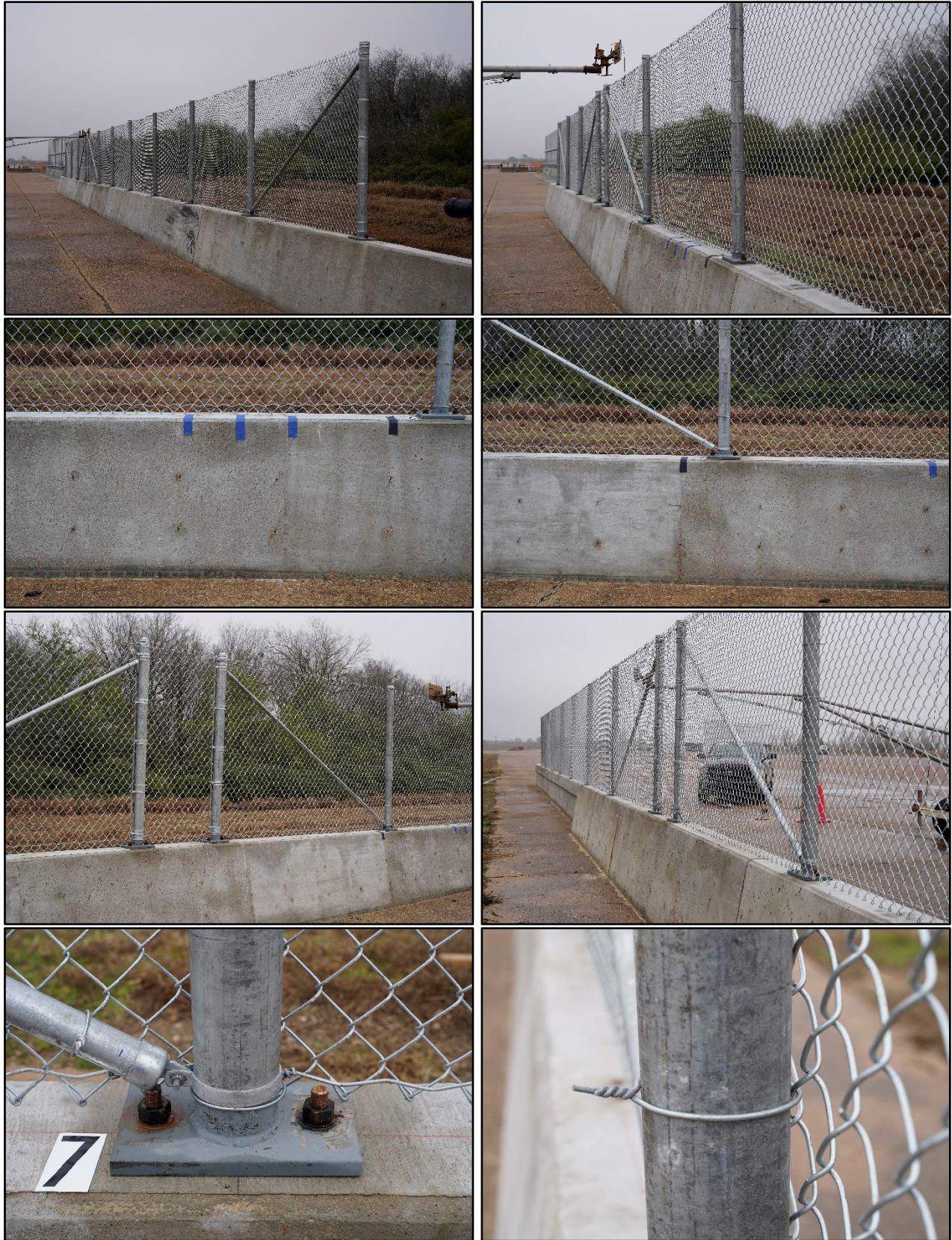
Figure 4.2. CMB with Fence Mounted on Top prior to Test No. 613131-01-1.
