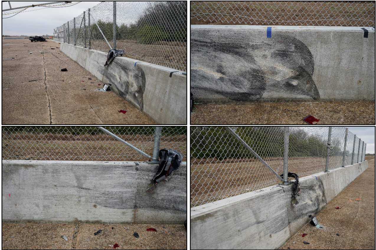
Figure 4.5. CMB after Test No. 613131-03-1.
