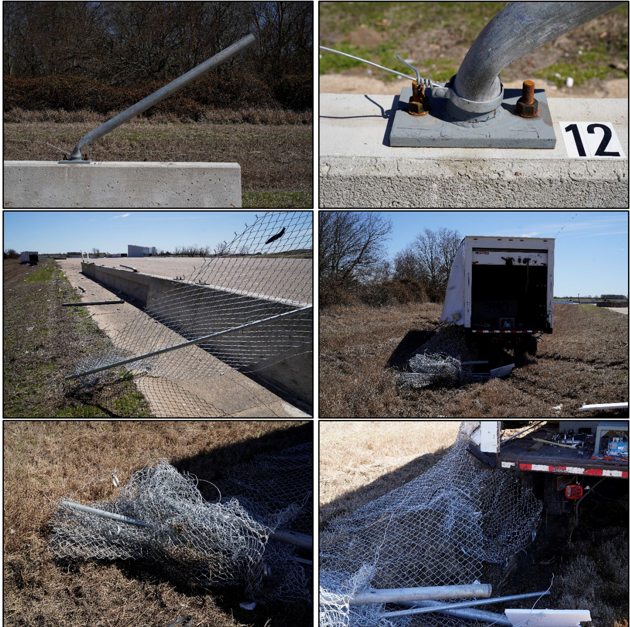
Figure 5.7. Post 12 and Separated Chain Link Fence after Test No. 613131-03-2.
