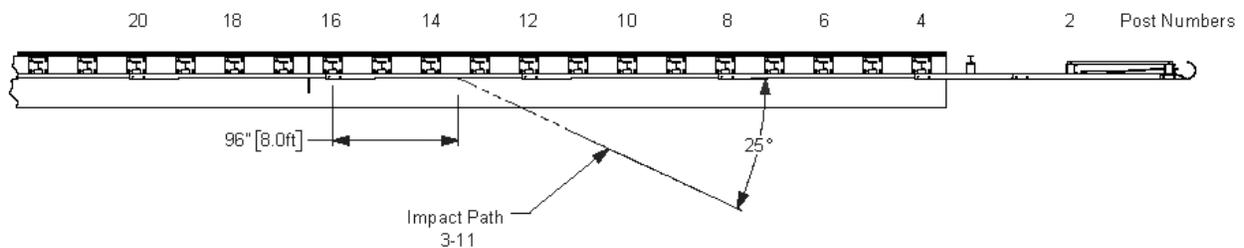
**Figure 3.2. Target CIP for *MASH* Test 3-11 on Thrie Beam Bridge Rail Retrofit.**
