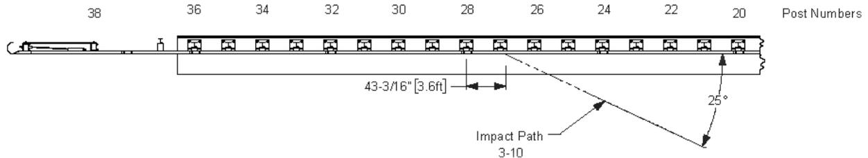
**Figure 3.1. Target CIP for *MASH* Test 3-10 on Thrie Beam Bridge Rail Retrofit.**
