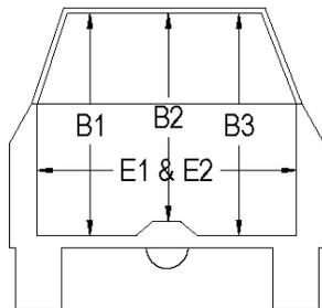
**OCCUPANT COMPARTMENT DEFORMATION MEASUREMENT**
