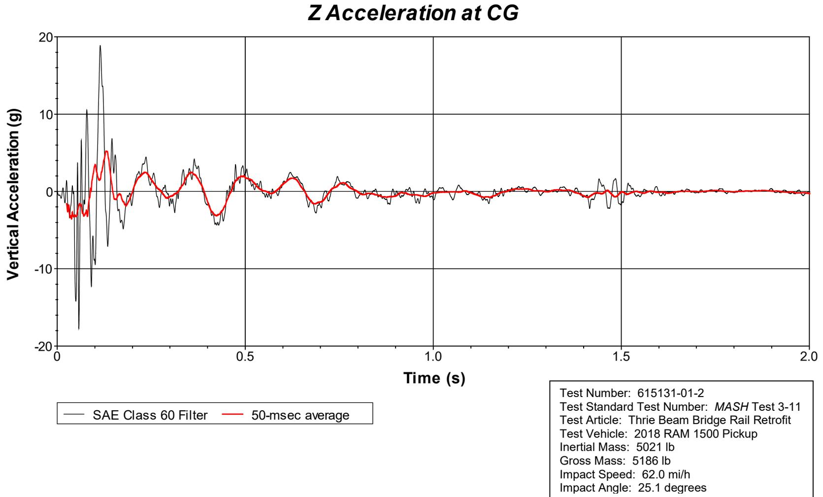
**Figure D.6. Vehicle Vertical Accelerometer Trace for Test No. 615131-01-2
