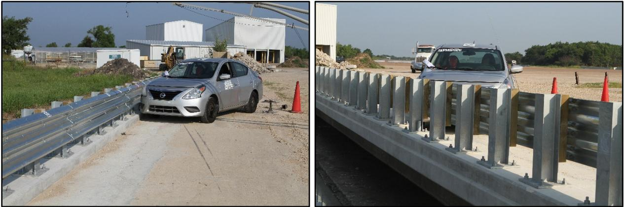
**Figure 6.1. Bridge Rail Retrofit/Test Vehicle Geometrics for Test No. 615131-01-1.**
