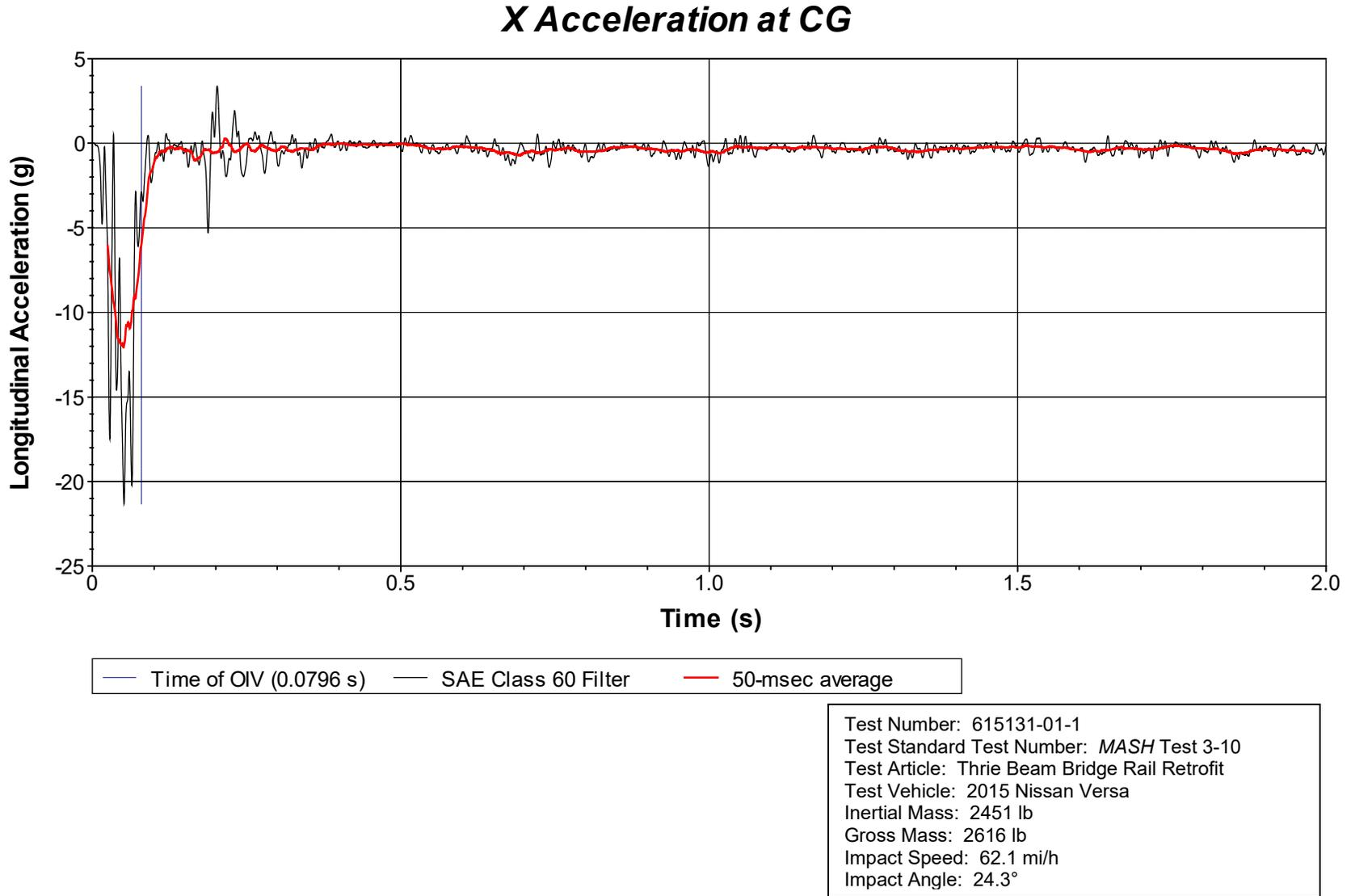
**Figure E.4. Vehicle Longitudinal Accelerometer Trace for Test No. 615131-01-1 (Accelerometer Located at Center of Gravity).**
