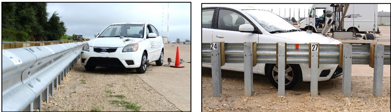
Figure 4.3. Guardrail/Test Vehicle Geometrics for Test No. 610211-01-1.
