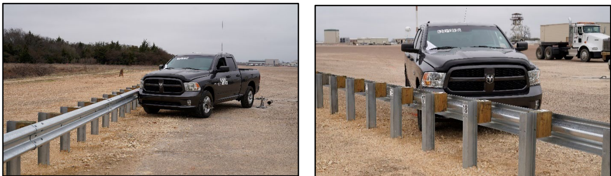
Figure 5.19. Guardrail/Test Vehicle Geometrics for Test No. 610211-01-6.
