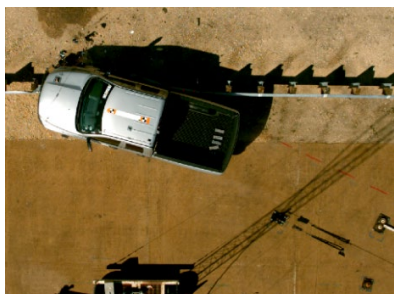
Figure 5.13. Top View Comparison of Failed MASH Test 3-11 Simulation.
