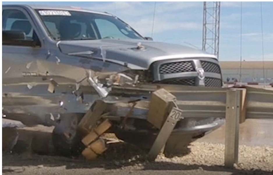
Figure 5.9. Rear View of Rail Rupture.
