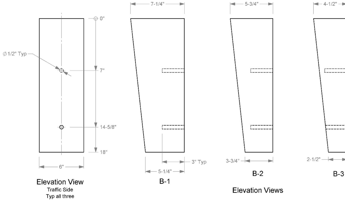
**6a.** Timber blockouts are treated with a preservative in accordance with AASHTO M 133 after all cutting and drilling.
