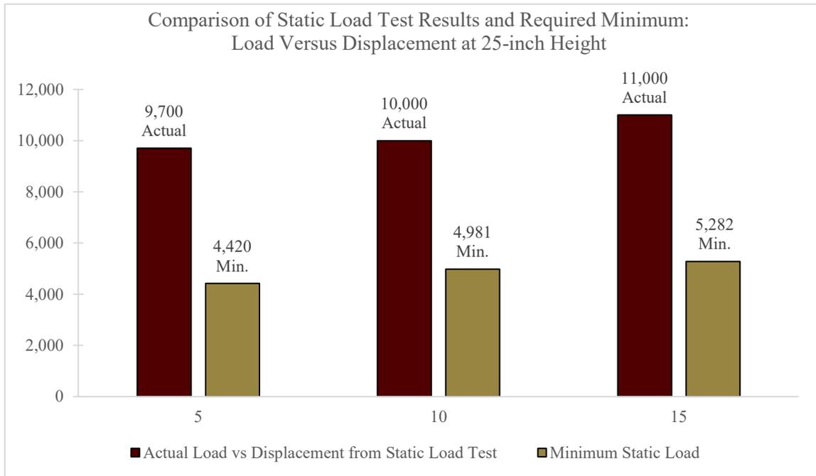
**Figure B.1. Test Day Static Soil Strength Documentation for Test No. 616391-01-1.**
