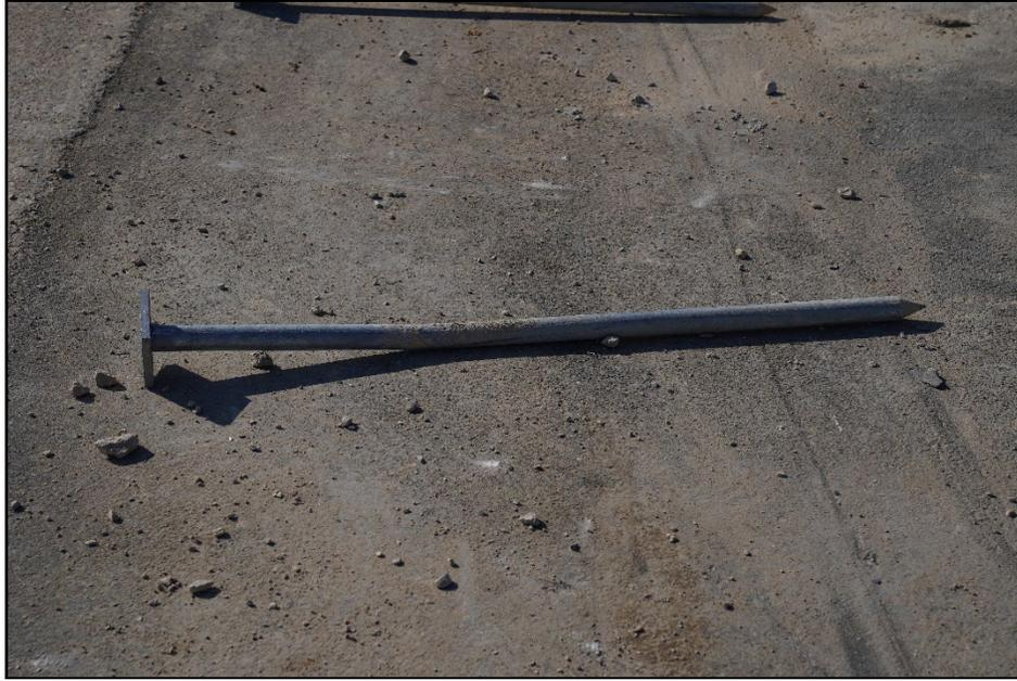
**Figure 7.11. Damage to the Middle Anchor Pin 616391-01-2.**
