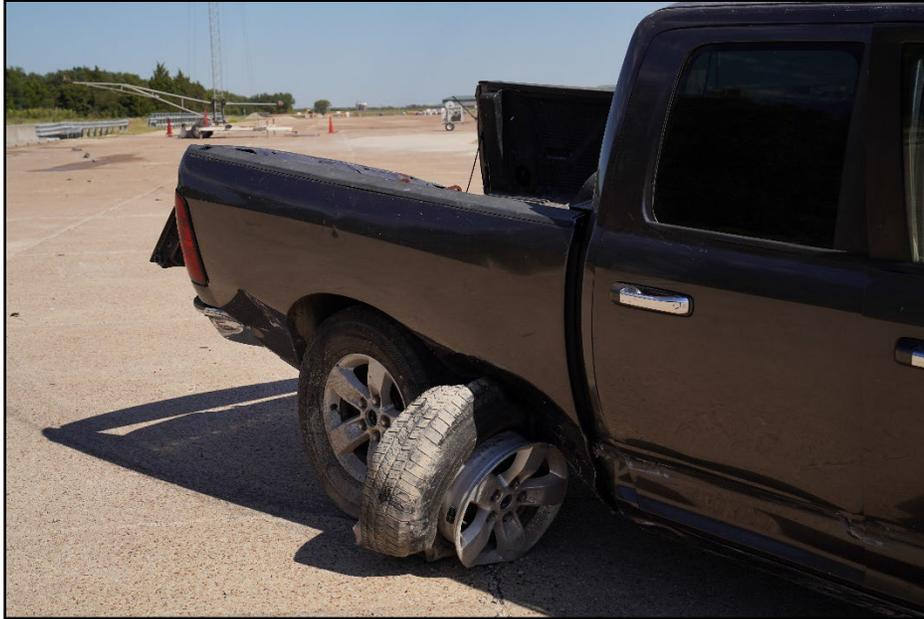
**Figure 7.15. Rear Impact Side of Test Vehicle after Test 616391-01-2.**
