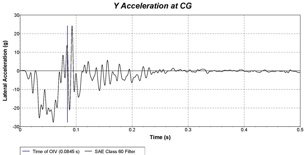
**Figure C.9. Vehicle Lateral Accelerometer Trace for Test No. 616391-01-1 (Accelerometer Located at Center of Gravity).**
