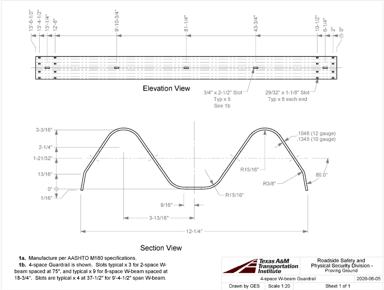
T:\Drafting Department\Solidworks\Standard Parts\Guardrail Parts and Subs\Guardrail Drawings\W-Beam Guardrail
