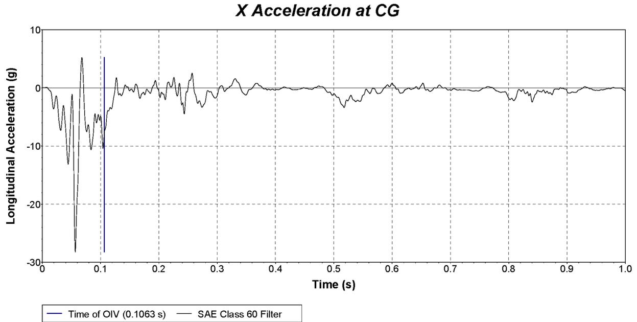
**Figure C.8. Vehicle Longitudinal Accelerometer Trace for Test No. 616391-01-2
