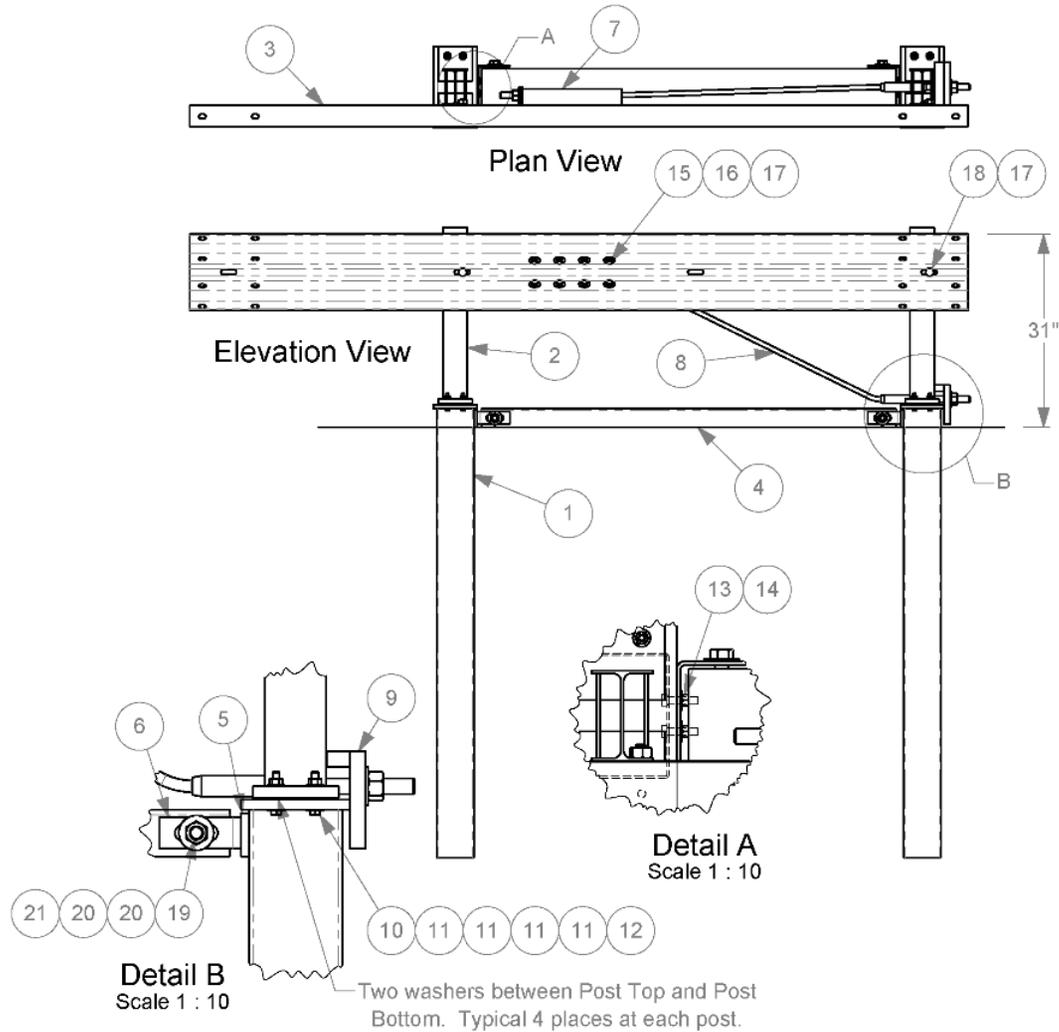
1a. 7/16" x 2-1/2" Bolts are ASTM A449. All other Bolts are ASTM A307. All Nuts (except Recessed Guardrail Nuts) are ASTM A563A unless otherwise indicated.
