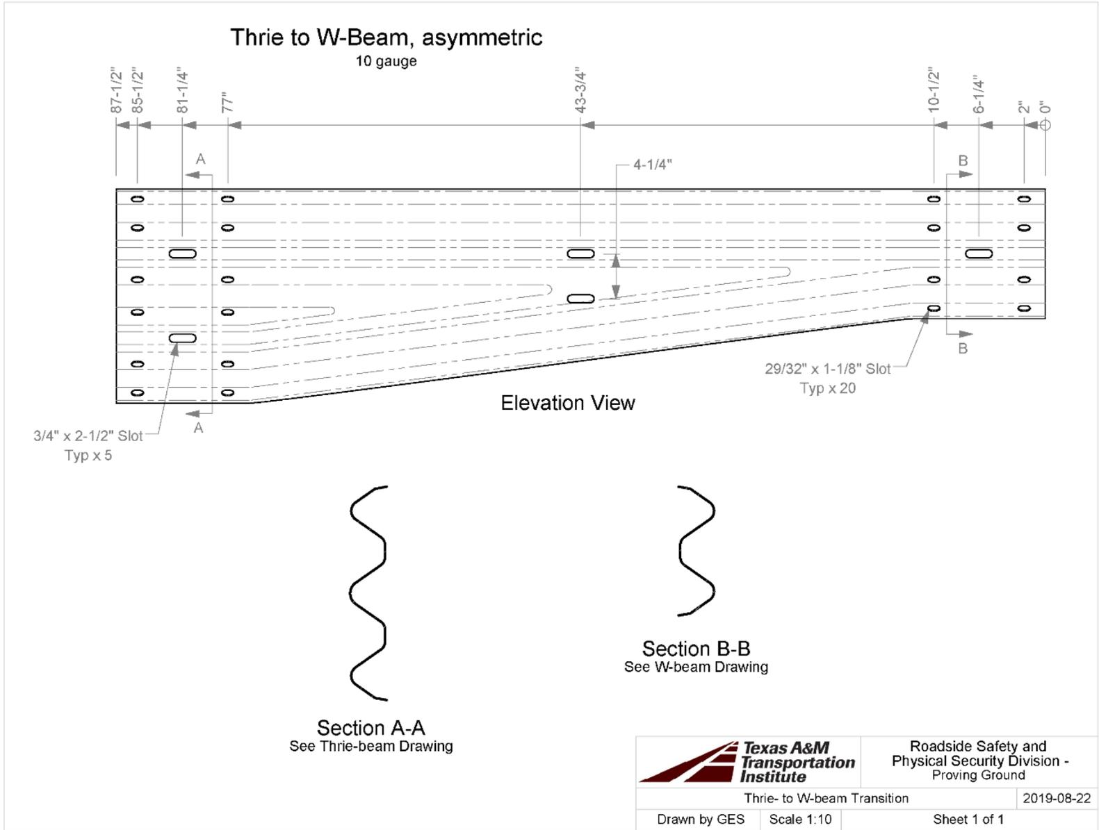
T:\Drafting Department\Solidworks\Standard Parts\Guardrail Parts and Subs\Guardrail Drawings\Thrie to W-Beam, asymmetric
