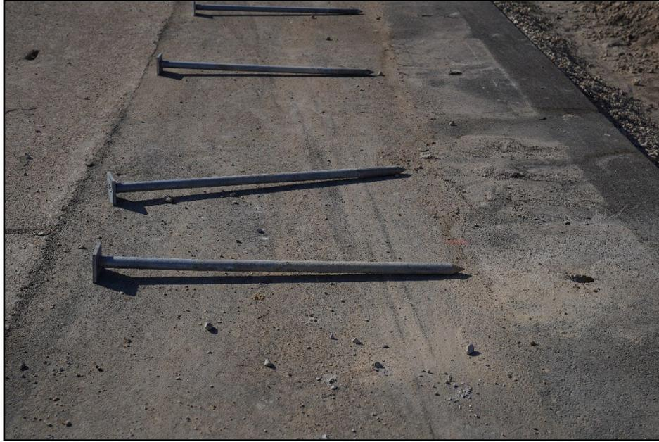
**Figure 7.13. Damage to the Downstream Anchor Pins 616391-01-2.**
