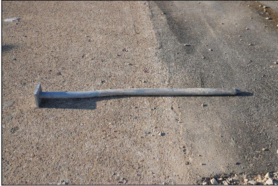
**Figure 6.9. Damage to the Upstream Anchor Pin 616391-01-1.**
