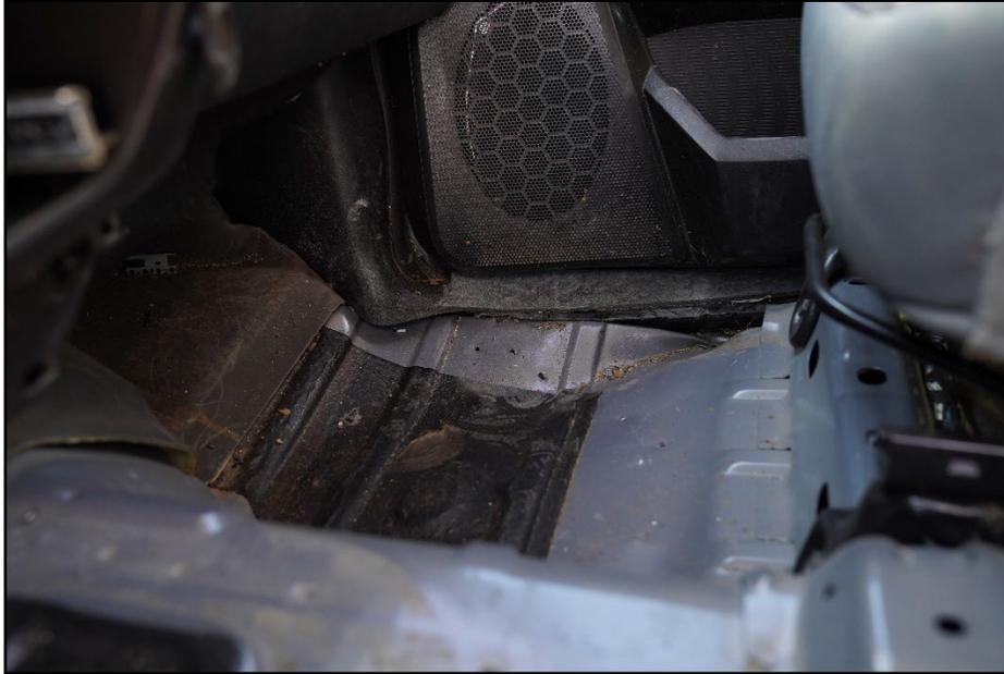
**Figure 7.17. Interior of Test Vehicle on Impact Side after Test 616391-01-2.**
