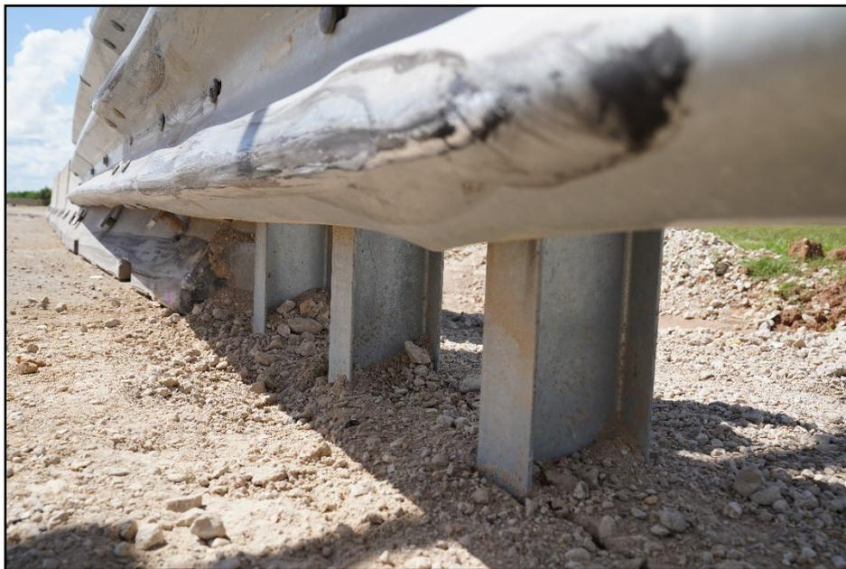
**Figure 6.6. Transition after Test at Grade Near the Impact Point 616391-01-1.**
