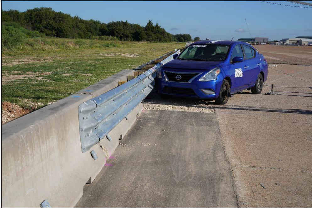
**Figure 6.1. Transition/Test Vehicle Geometrics for Test 616391-01-1.**
