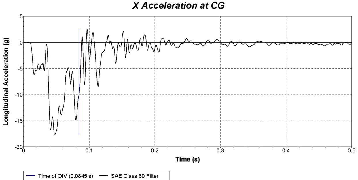
**Figure C.8. Vehicle Longitudinal Accelerometer Trace for Test No. 616391-01-1 (Accelerometer Located at Center of Gravity).**
