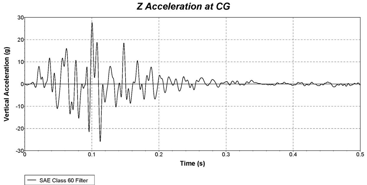
**Figure C.10. Vehicle Vertical Accelerometer Trace for Test No. 616391-01-1 (Accelerometer Located at Center of Gravity).**
