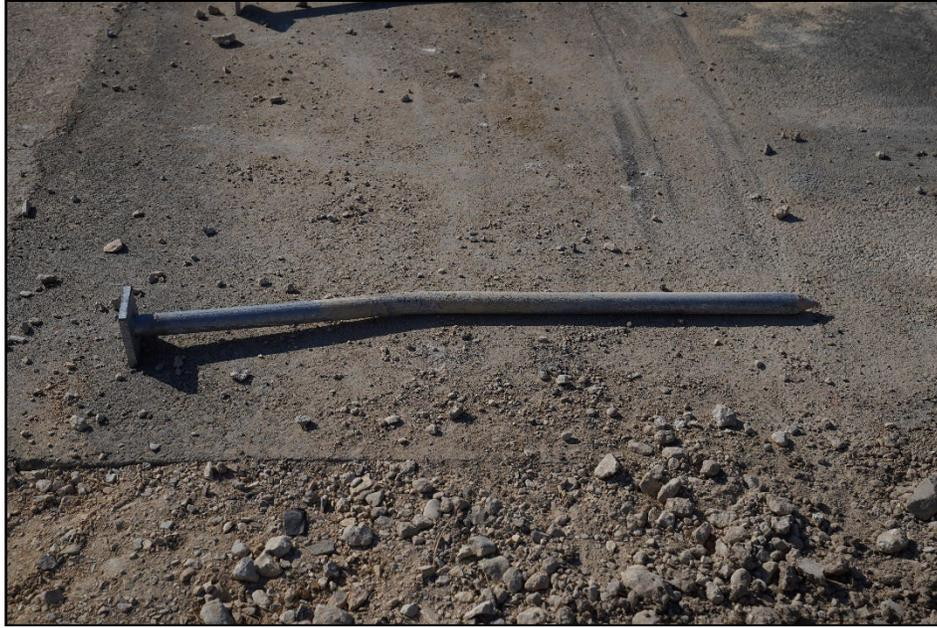
**Figure 7.9. Damage to the Upstream Anchor Pin 616391-01-2.**
