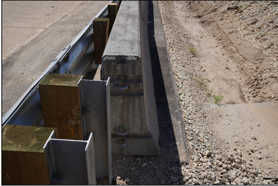
**Figure 6.7. Transition after Test In-line with Portable Concrete Barrier 616391-01-1.**
