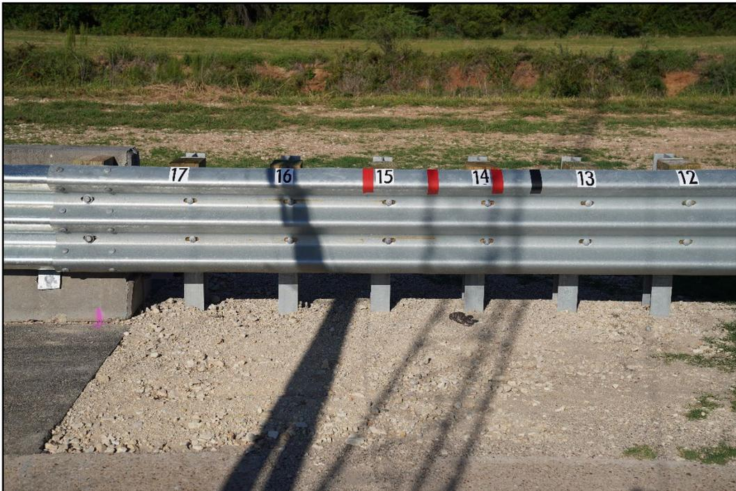
**Figure 3.3. Transition prior to Testing.**
