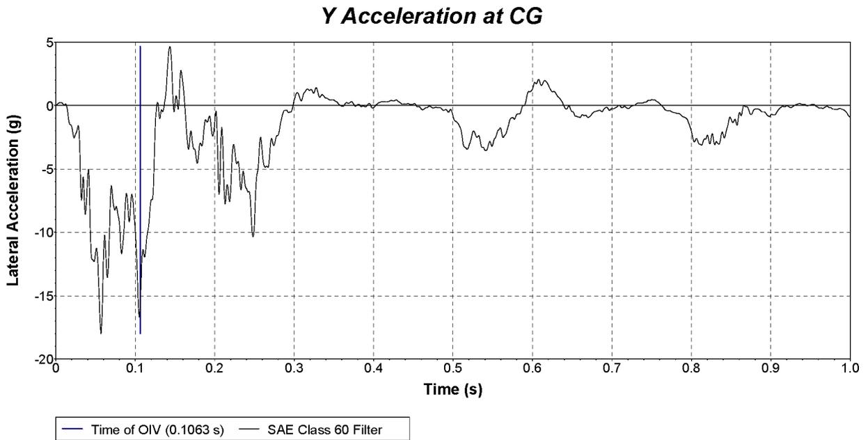
**Figure D.9. Vehicle Lateral Accelerometer Trace for Test No. 616391-01-2
