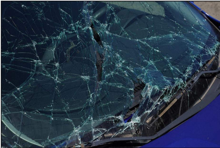
**Figure 6.15. Windshield Deformation of the Test Vehicle after Test 616391-01-1.**
