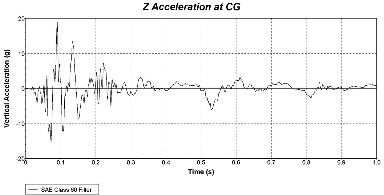
**Figure D.10. Vehicle Vertical Accelerometer Trace for Test No. 616391-01-2
