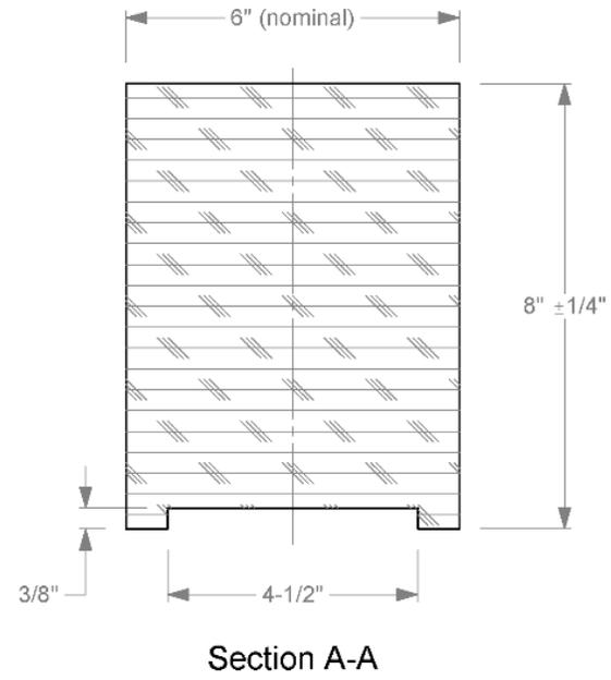
1a. Timber blockouts are treated with a preservative in accordance with AASHTO M 133 after all cutting and drilling.
