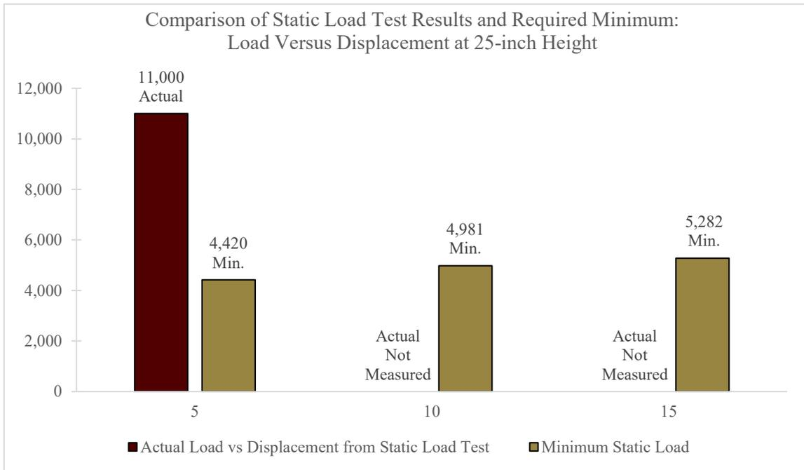
**Figure B.2. Test Day Static Soil Strength Documentation for Test No. 616391-01-2.**
