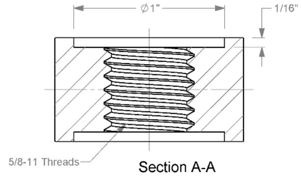
1a. Material is ASTM A 563 Grade A.
