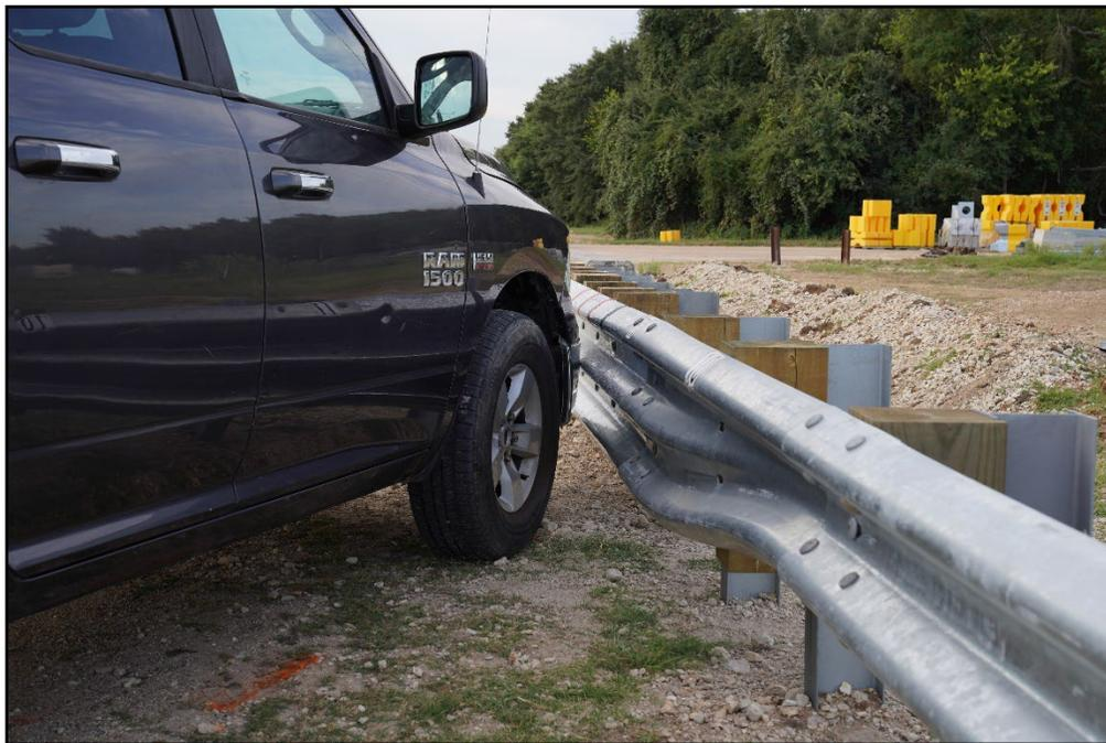
**Figure 7.2. Transition/Test Vehicle Impact Location 616391-01-2.**
