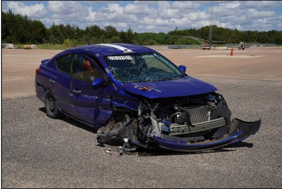
**Figure 6.14. Impact Side of Test Vehicle after Test 616391-01-1.**
