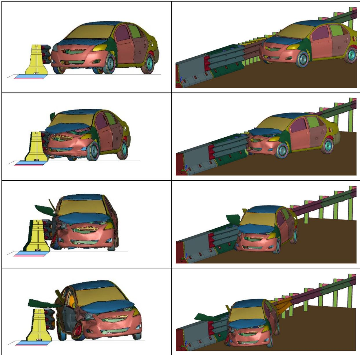
**Figure 2.6. Simulation Results of MASH Test 3-20 with Small Passenger Car.**
