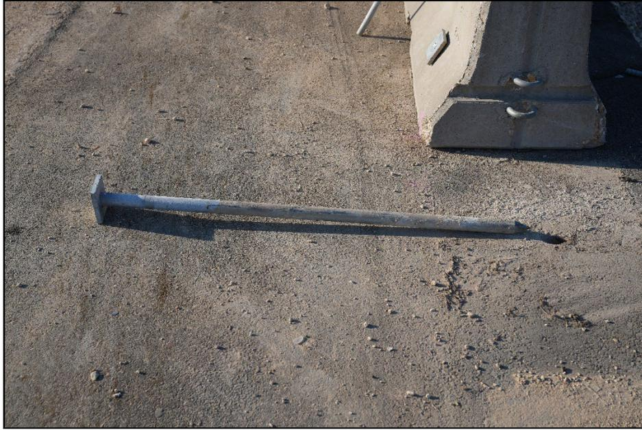
**Figure 6.13. Damage to the Downstream Anchor Pin 616391-01-1.**
