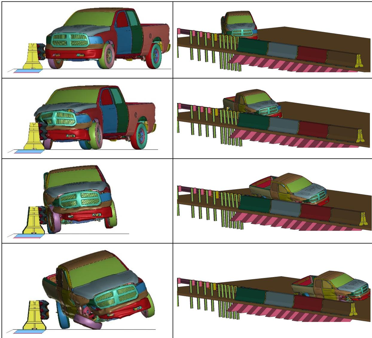
**Figure 2.5. Simulation Results of MASH Test 3-21 with Pickup Truck.**
