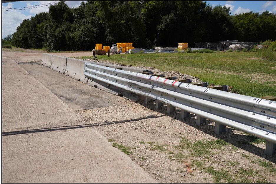
**Figure 6.5. Transition after Test at Impact Location 616391-01-1.**
