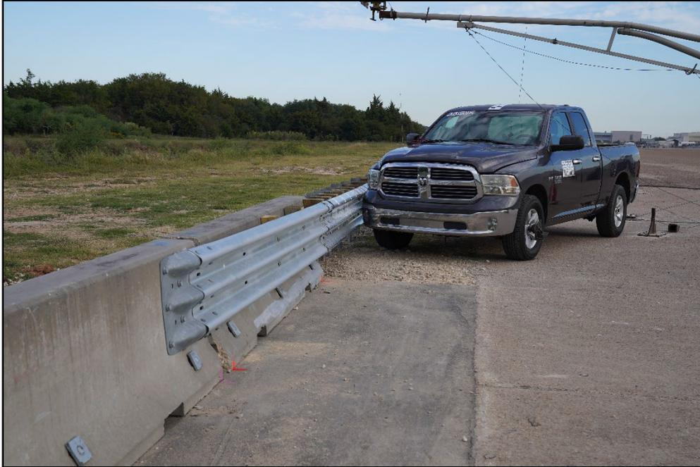
**Figure 7.1. Transition/Test Vehicle Geometrics for Test 616391-01-2.**
