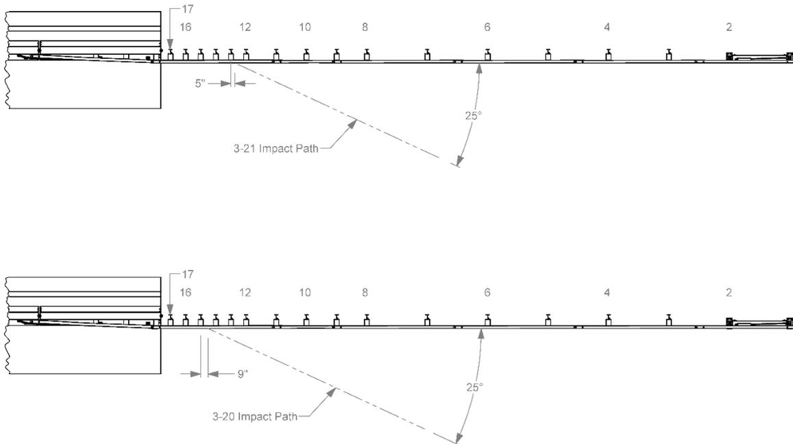
**Figure 4.1. Target CIP for *MASH* TL-3 Tests on Transition.**
