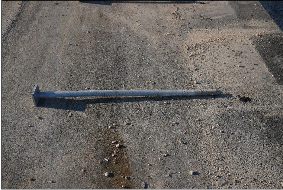
**Figure 6.11. Damage to the Middle Anchor Pin 616391-01-1.**
