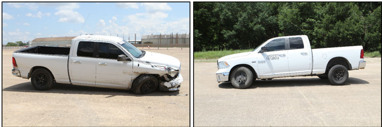
Figure 6.6. Test Vehicle after Test No. 614341-01-1.
