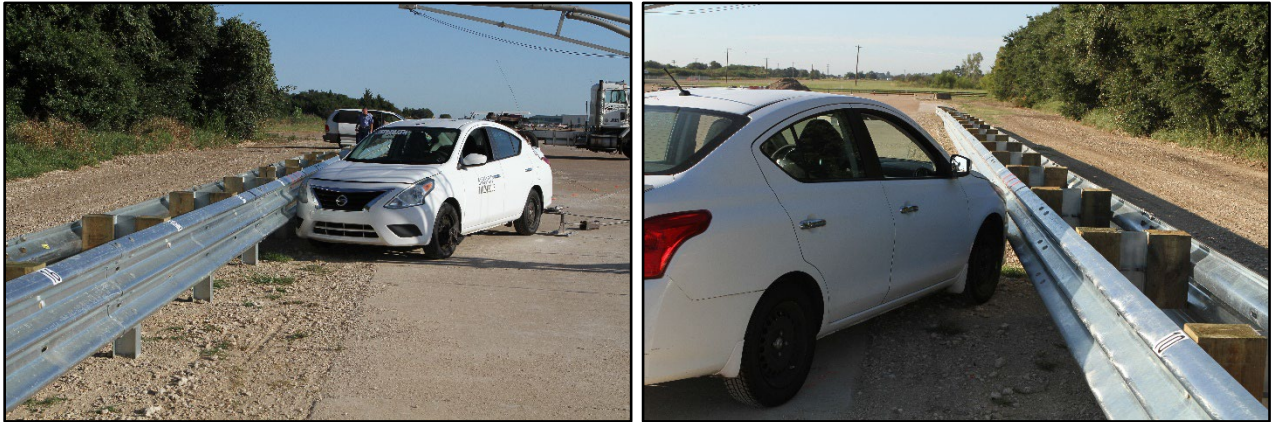
Figure 7.3. Median Thrie-beam System/Test Vehicle Geometrics for Test No. 614341-01-2.
