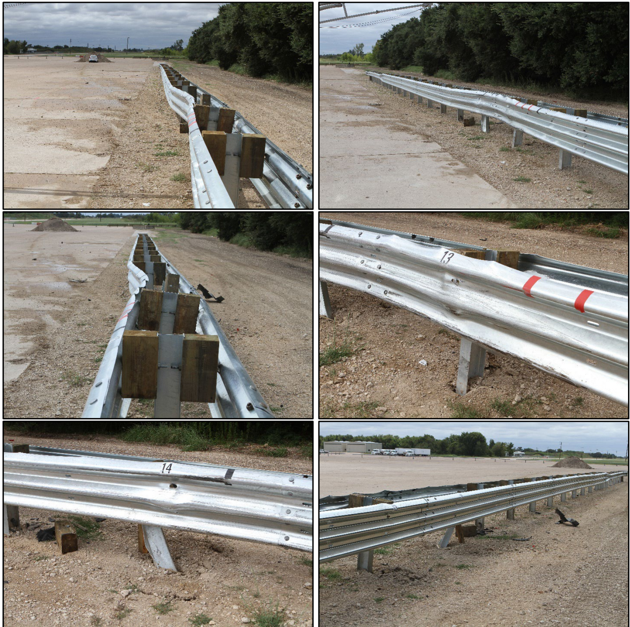
Figure 7.5. Median Thrie-beam System after Test No. 614341-01-2.
