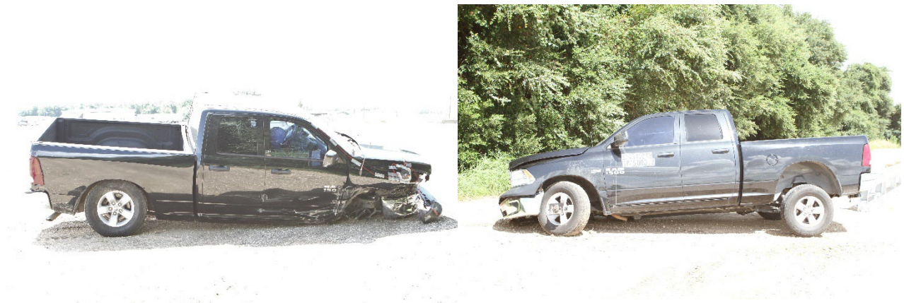
Figure 6.12. Test Vehicle after Test No. 614341-01-3.
