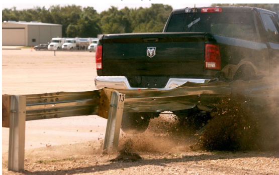
Figure E.2. Sequential Photographs for Test No. 614341-01-3 (Rear View).
