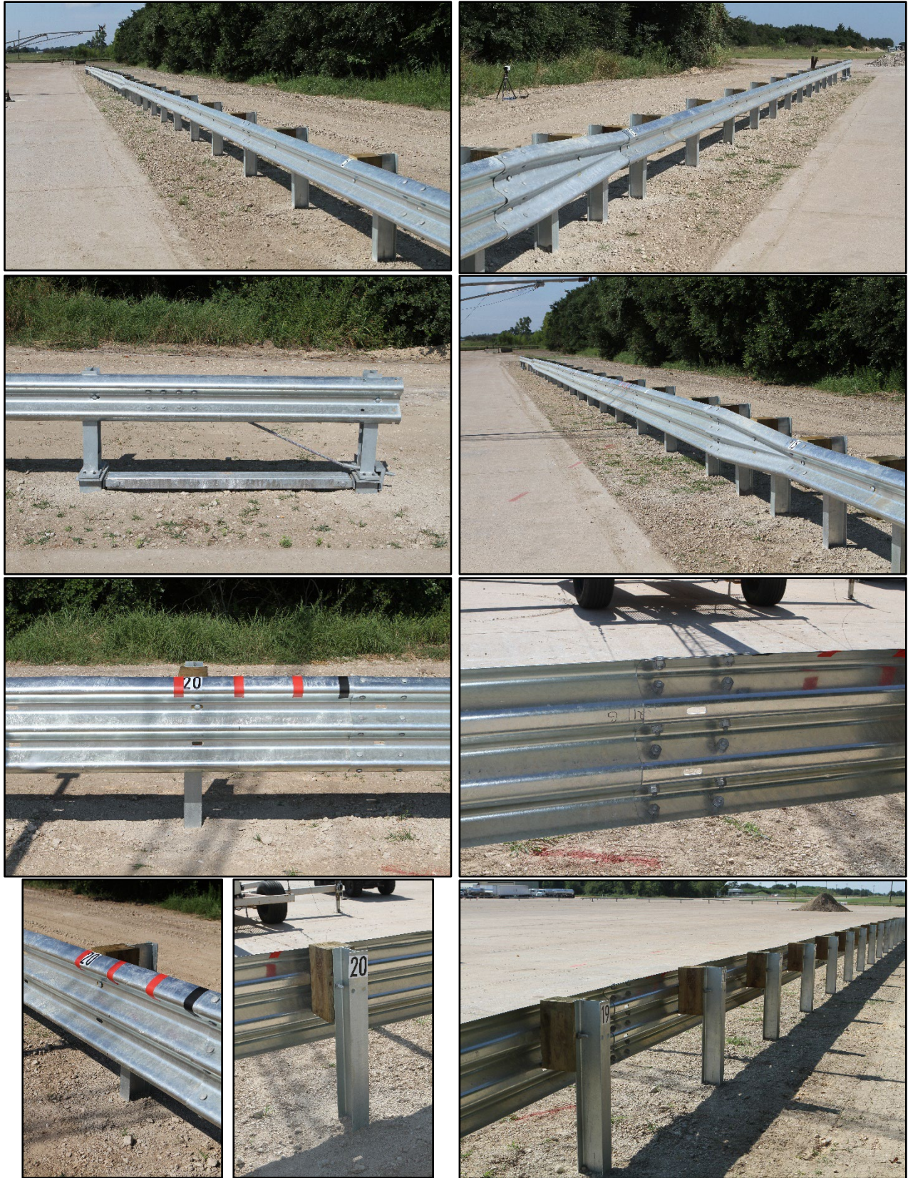
Figure 6.2. Roadside Thrie-beam System prior to Testing.
