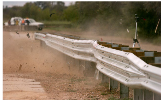
Figure G.2. Sequential Photographs for Test No. 614341-01-2 (Rear View).
