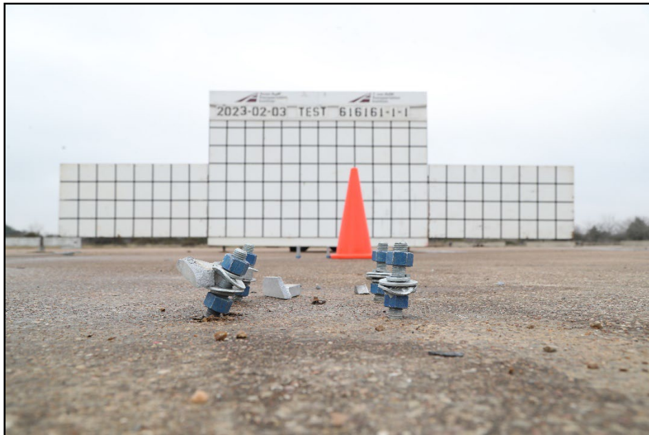
Figure 5.6. Crashworthy Enhanced Highway Sign Assemblies after Test at the Anchor Bolts 616161-01-1.
