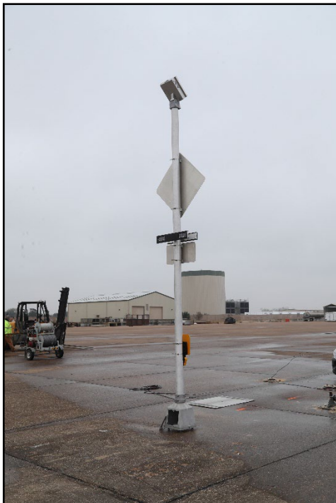
Figure 2.3. The Rear of the Crashworthy Enhanced Highway Sign Assemblies prior to Testing.
