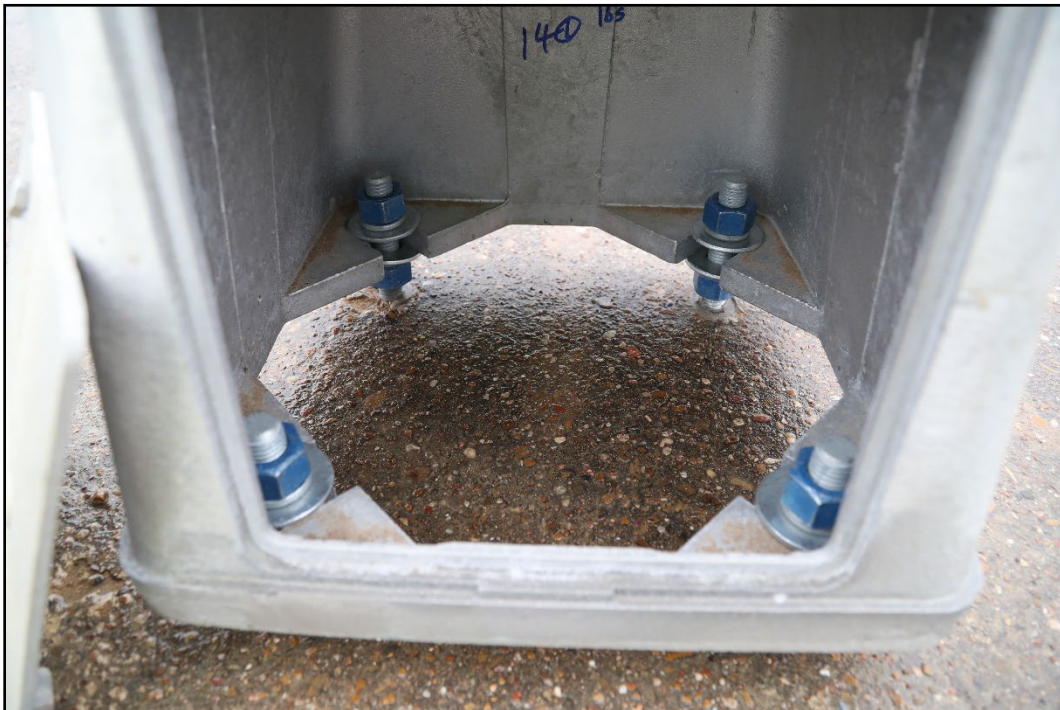
Figure 2.7. The Anchor System of the Crashworthy Enhanced Highway Sign Assemblies prior to Testing.
