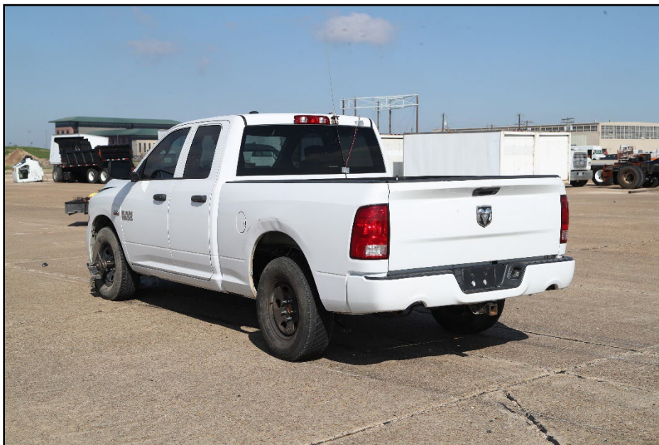
Figure 6.8. Rear Impact Side of Test Vehicle after Test 616161-01-2.
