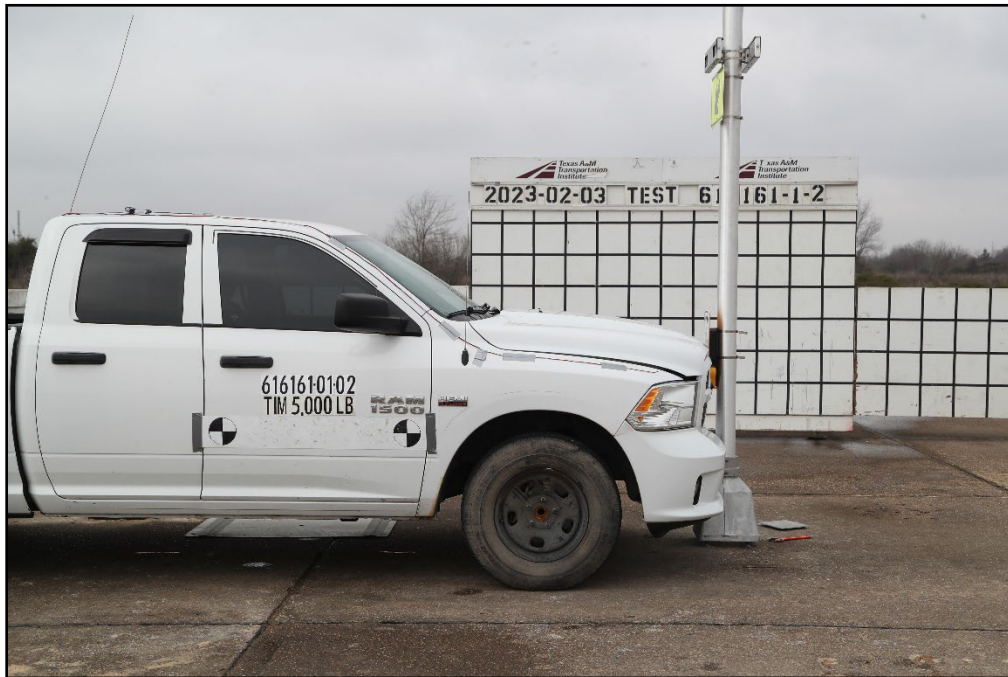
Figure 6.2. Crashworthy Enhanced Highway Sign Assemblies/Test Vehicle Impact Location 616161-01-2.
