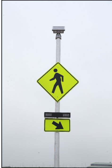
Figure 2.4. The Top Portion of the Crashworthy Enhanced Highway Sign Assemblies prior to Testing.
