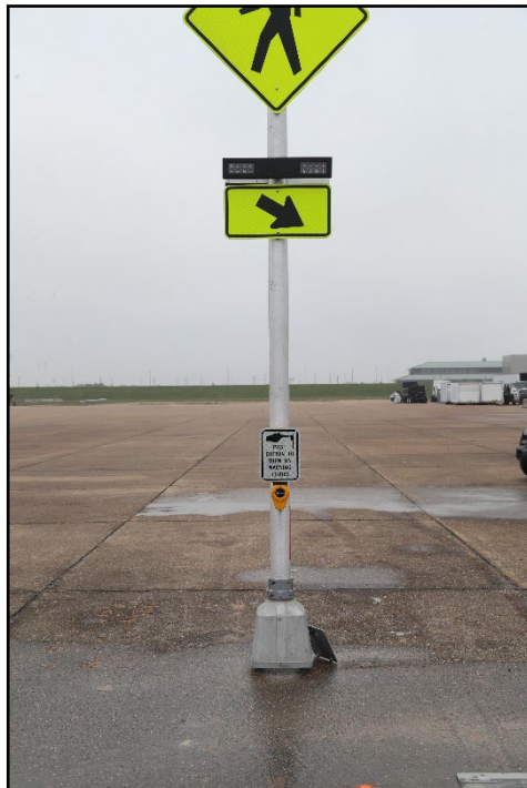
Figure 2.5. The Lower Portion of the Crashworthy Enhanced Highway Sign Assemblies prior to Testing.
