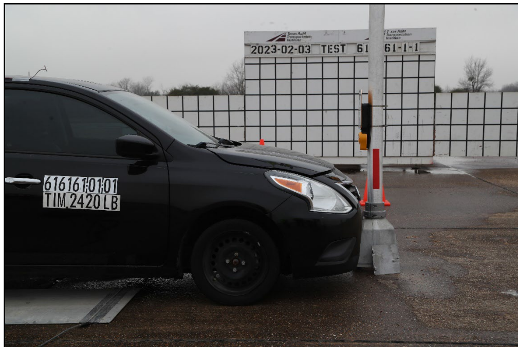
Figure 5.2. Crashworthy Enhanced Highway Sign Assemblies/Test Vehicle Impact Location 616161-01-1.
