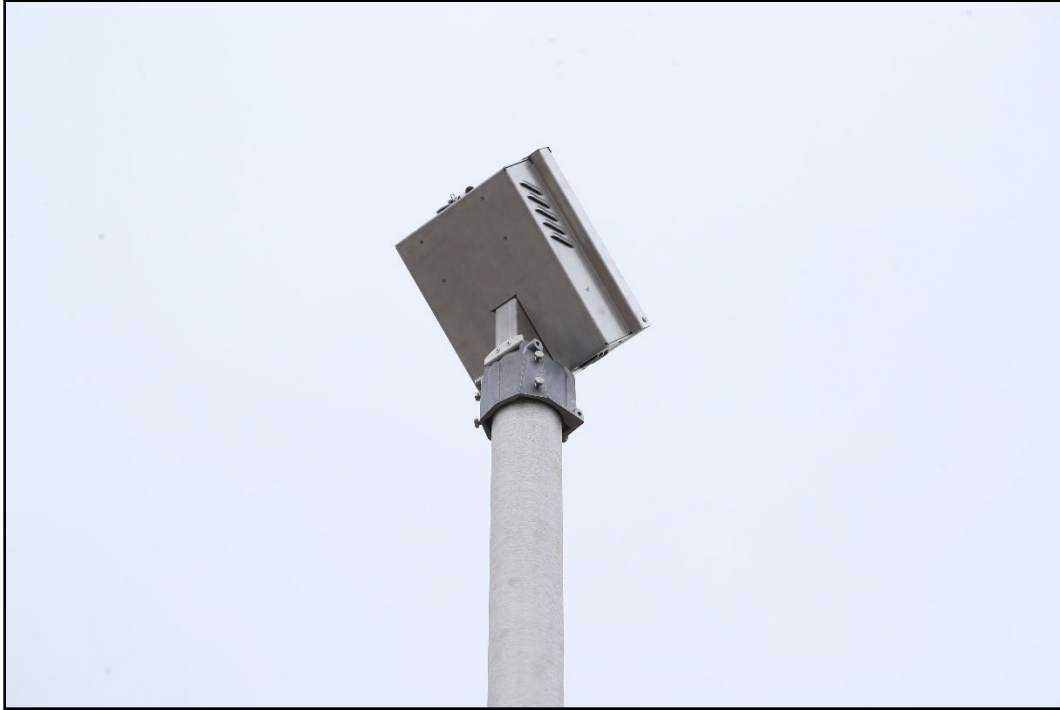
Figure 2.6. Rear of the Solar Panel on the Crashworthy Enhanced Highway Sign Assemblies prior to Testing.
