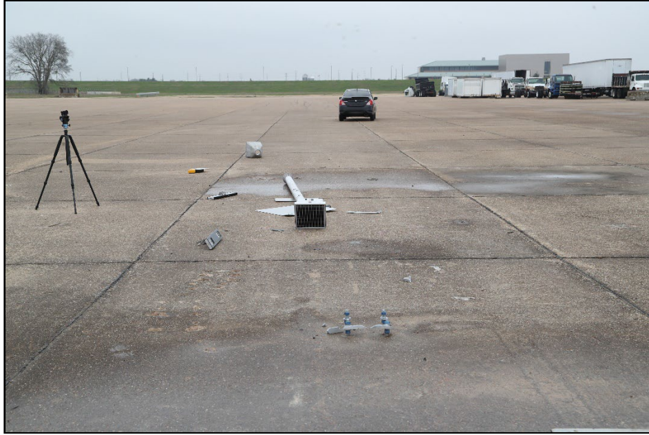
Figure 5.5. Crashworthy Enhanced Highway Sign Assemblies after Test at Impact Location 616161-01-1.
