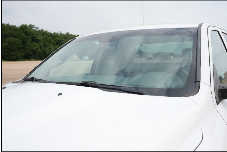
Figure 6.8. Roof and Windshield of Test Vehicle after Test 616011-01-6.
