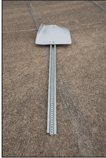
Figure 5.6. U-Channel Sign Support System at its Landing Location after Test 616011-01-5.
