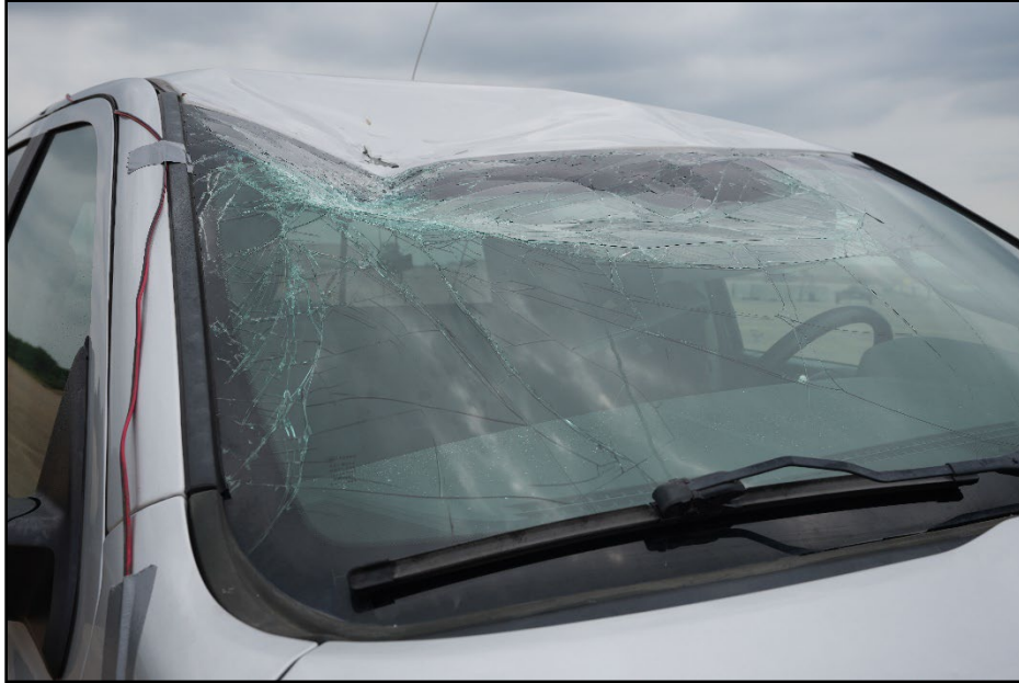
Figure 5.8. Roof and Windshield of Test Vehicle after Test 616011-01-5.
