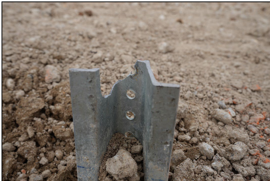
Figure 6.5. U-Channel Sign Support System at Impact Location after Test 616011-01-6.
