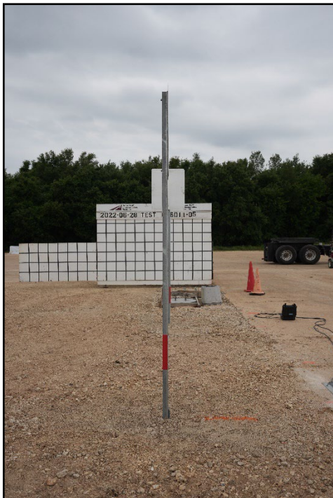
Figure 2.3. Right Angle View of the U-Channel Sign Support System prior to Testing.
