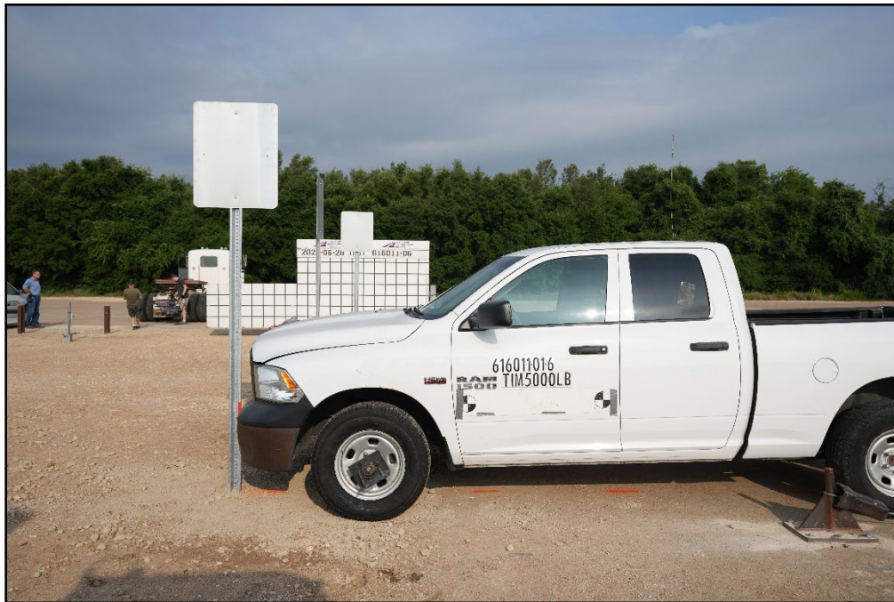
Figure 6.2. U-Channel Sign Support System/Test Vehicle Impact Location 616011-01-6.
