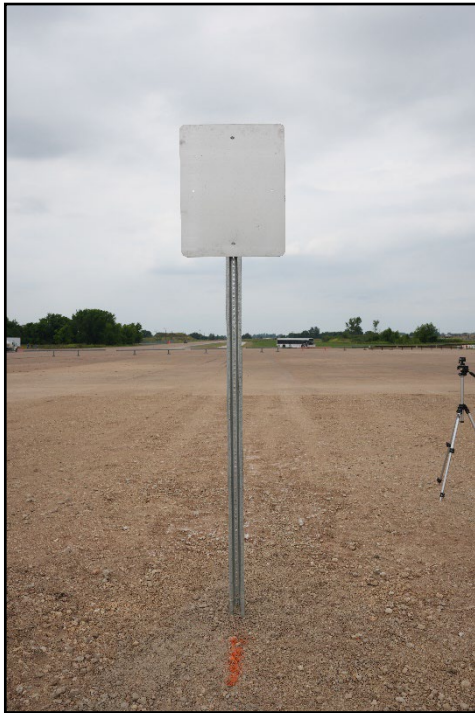
Figure 2.2. U-Channel Sign Support System prior to Testing.
