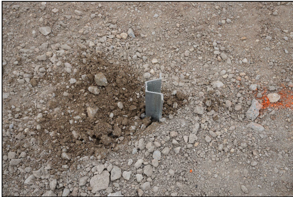
Figure 5.5. U-Channel Sign Support System at Impact Location after Test 616011-01-5.
