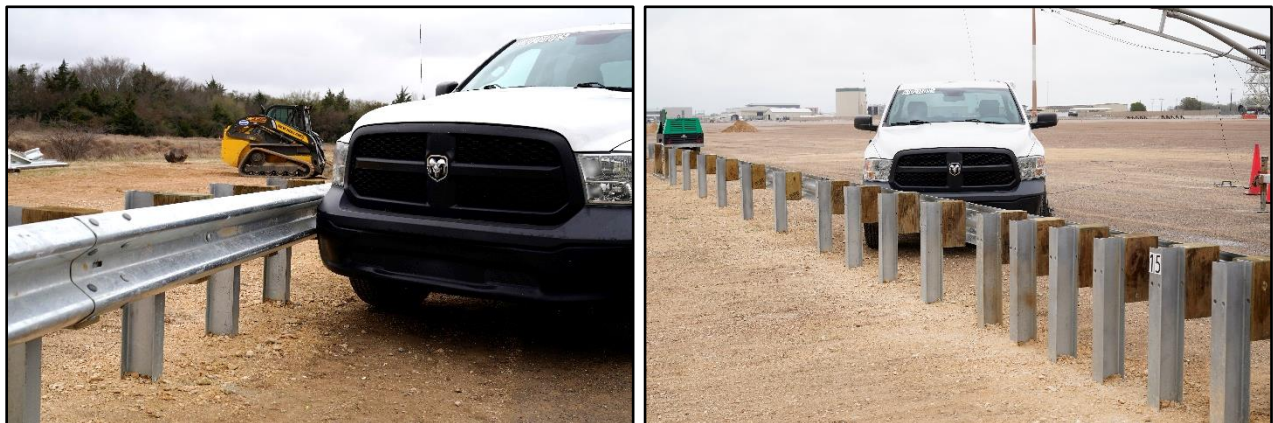
Figure 6.18. Transition/Test Vehicle Geometrics for Test No. 610211-01-5.
