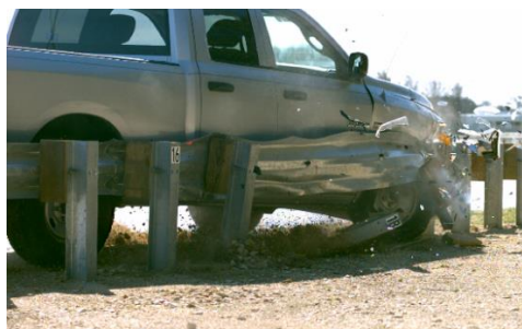
Figure 5.12. Rear View Comparison of Failed MASH Test 3-11 Simulation.
