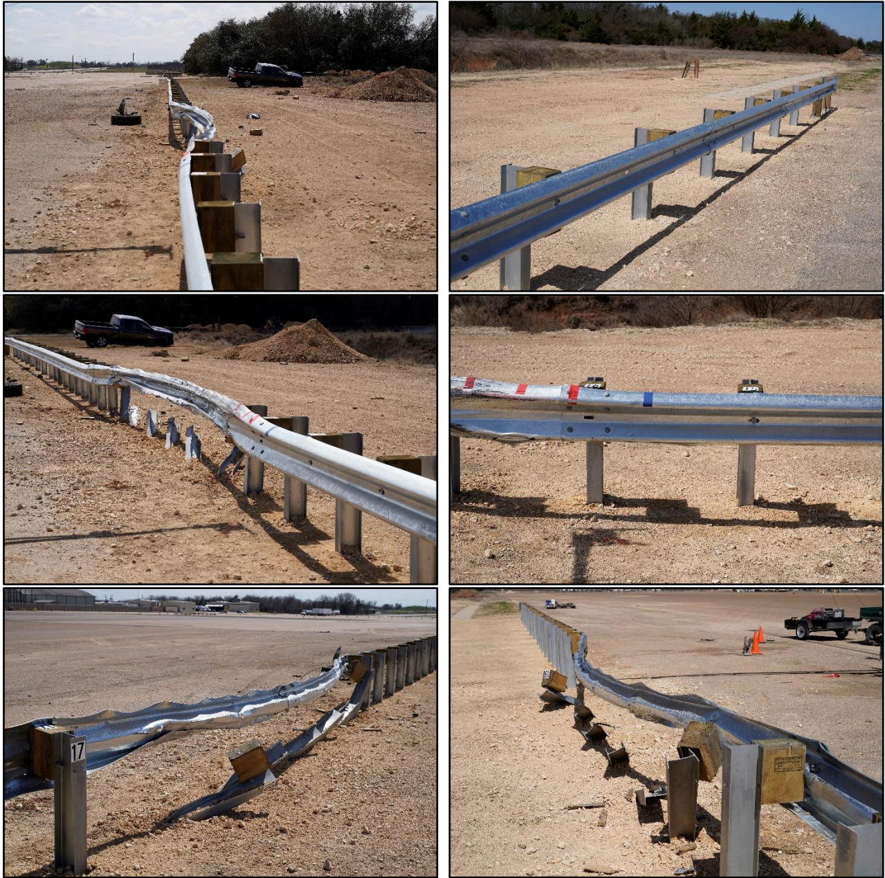
Figure 5.21. MGS with half Post Spacing and Shortened Blockouts after Test No. 610211-01-6.
