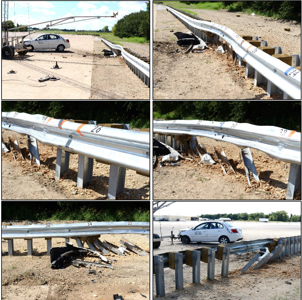
Figure 4.5. MGS with Quarter Post Spacing after Test No. 610211-01-1.
