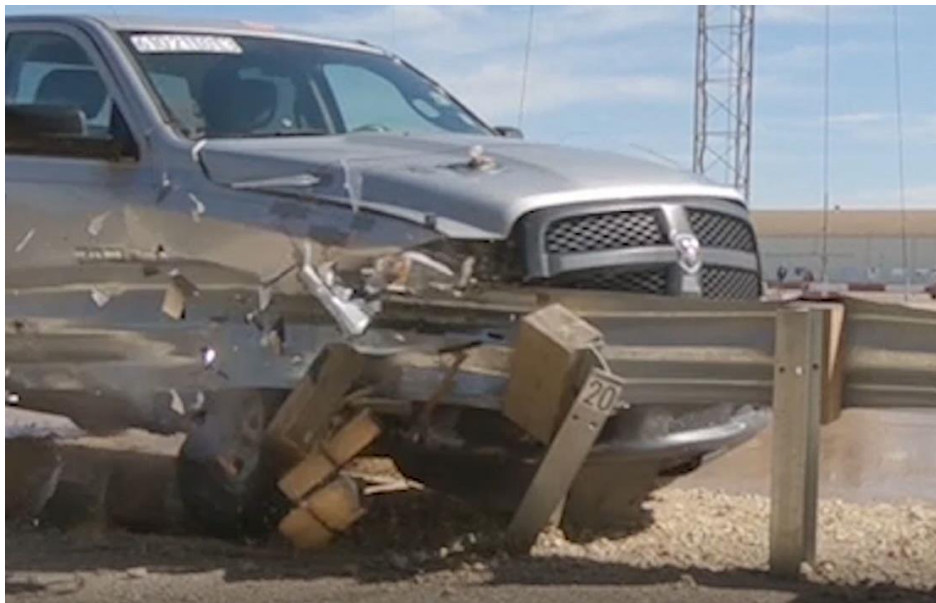
Figure 5.9. Rear View of Rail Rupture.
