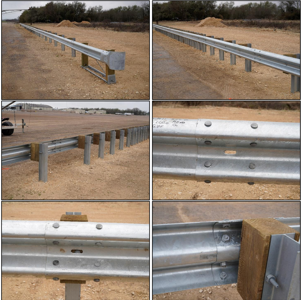
Figure 6.17. MGS with Longer Transition from Full to Quarter Post Spacing prior to Testing.
