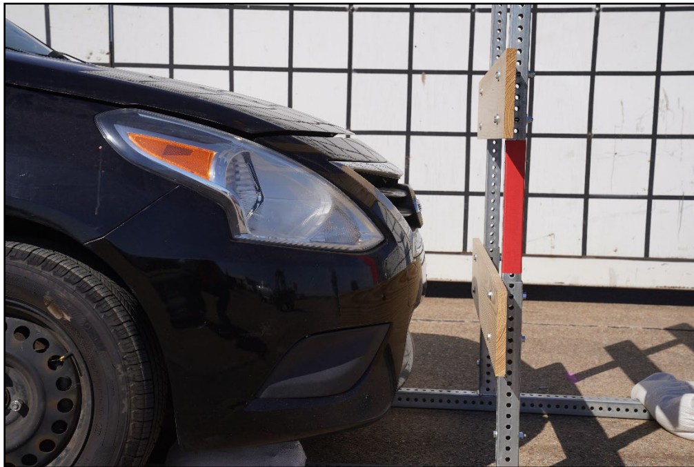
Figure 8.2. Type III Barricade with Mounted Sign/Test Vehicle Impact Location 616411-01-2.
