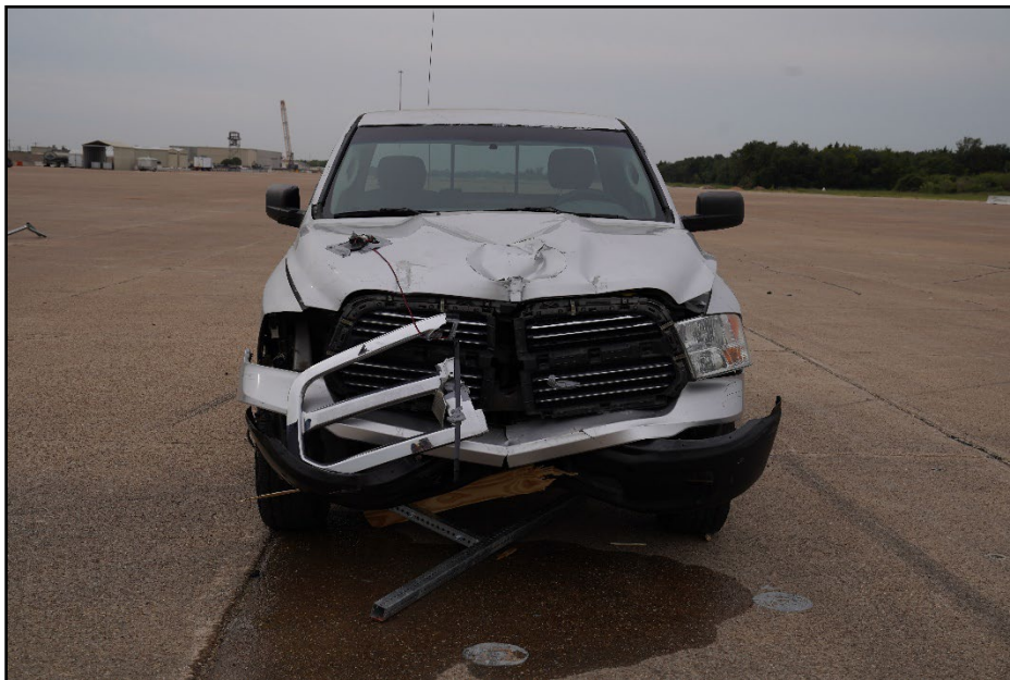
Figure 10.7. Impact Side of Test Vehicle after Test 616411-01-4.
