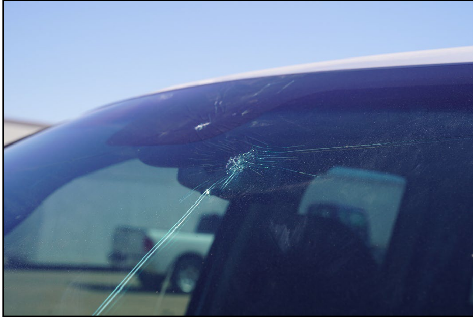
Figure 9.8. Windshield of Test Vehicle after Test 616411-01-3.
