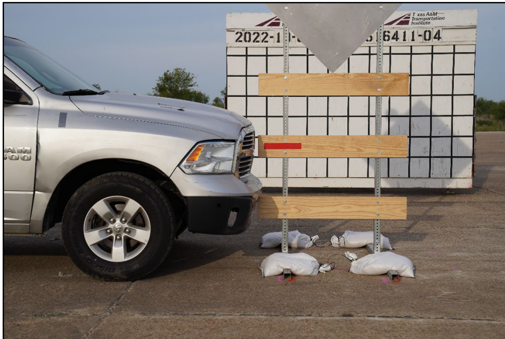
Figure 10.2. Type III Barricade with Mounted Sign/Test Vehicle Impact Location 616411-01-4.
