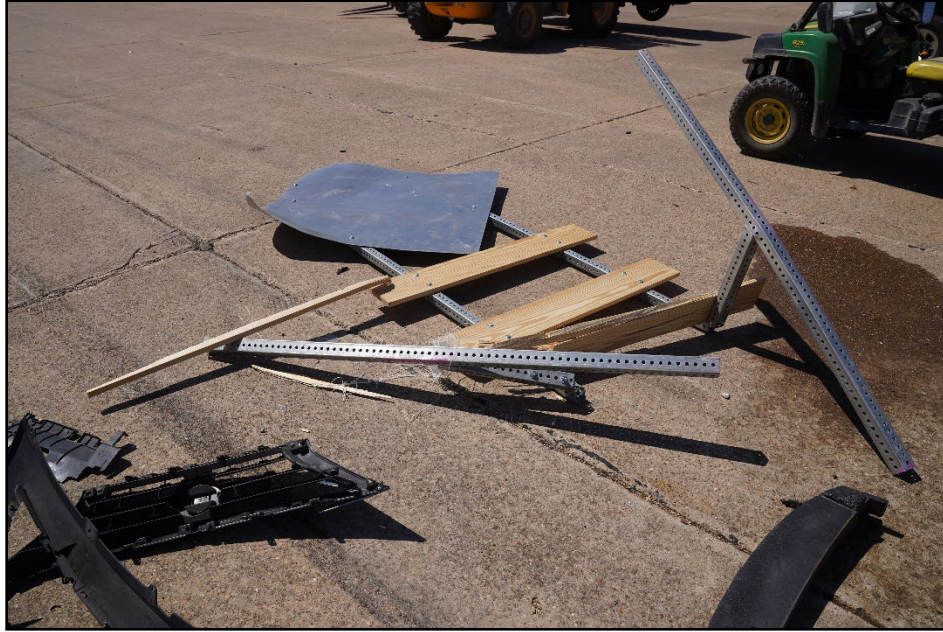
Figure 8.6. Type III Barricade with Mounted Sign after Test After Being Removed from the Vehicle 616411-01-2.
