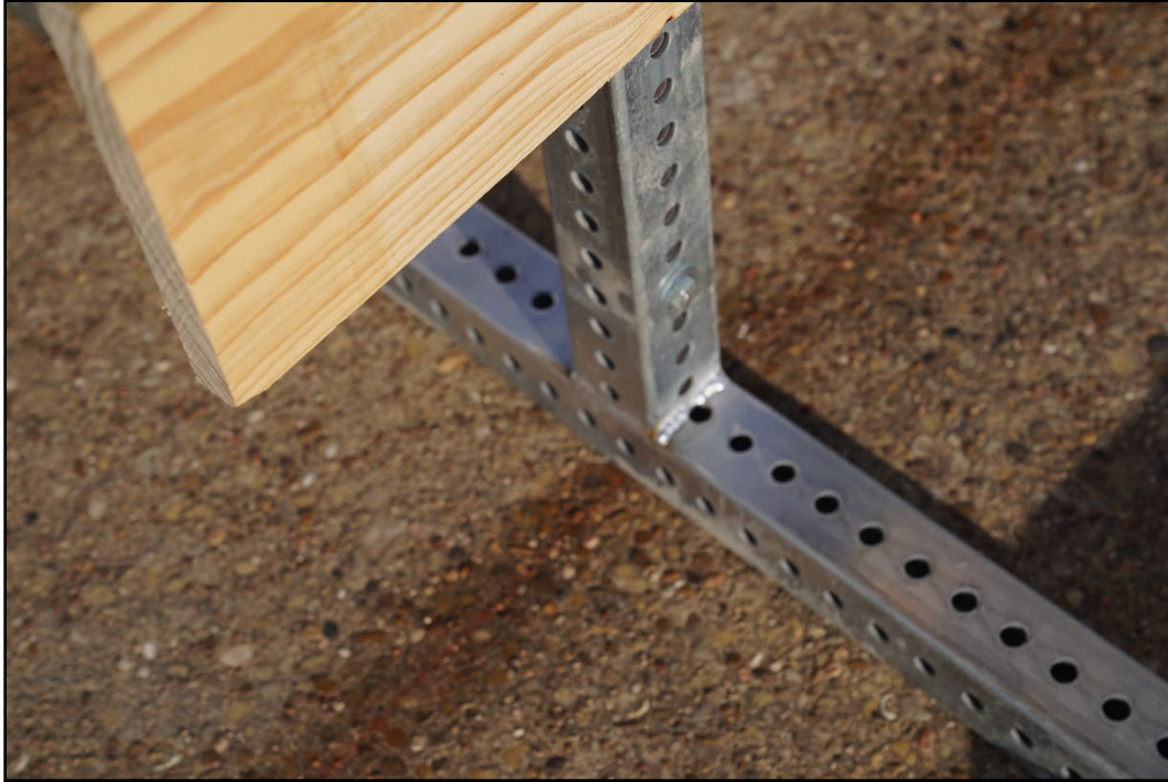
Figure 4.4. Base of Type III Barricade with Mounted Sign prior to Testing.
