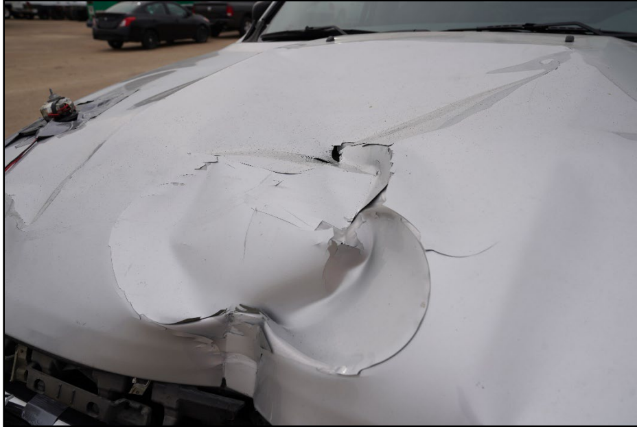
Figure 10.8. Test Vehicle Hood Damage after Test 616411-01-4.
