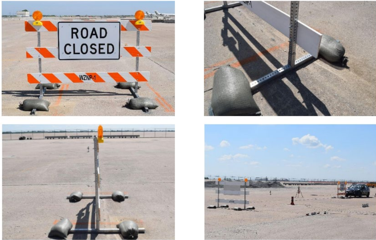
Figure 2.12: Non-proprietary Type III Barricade (6)
