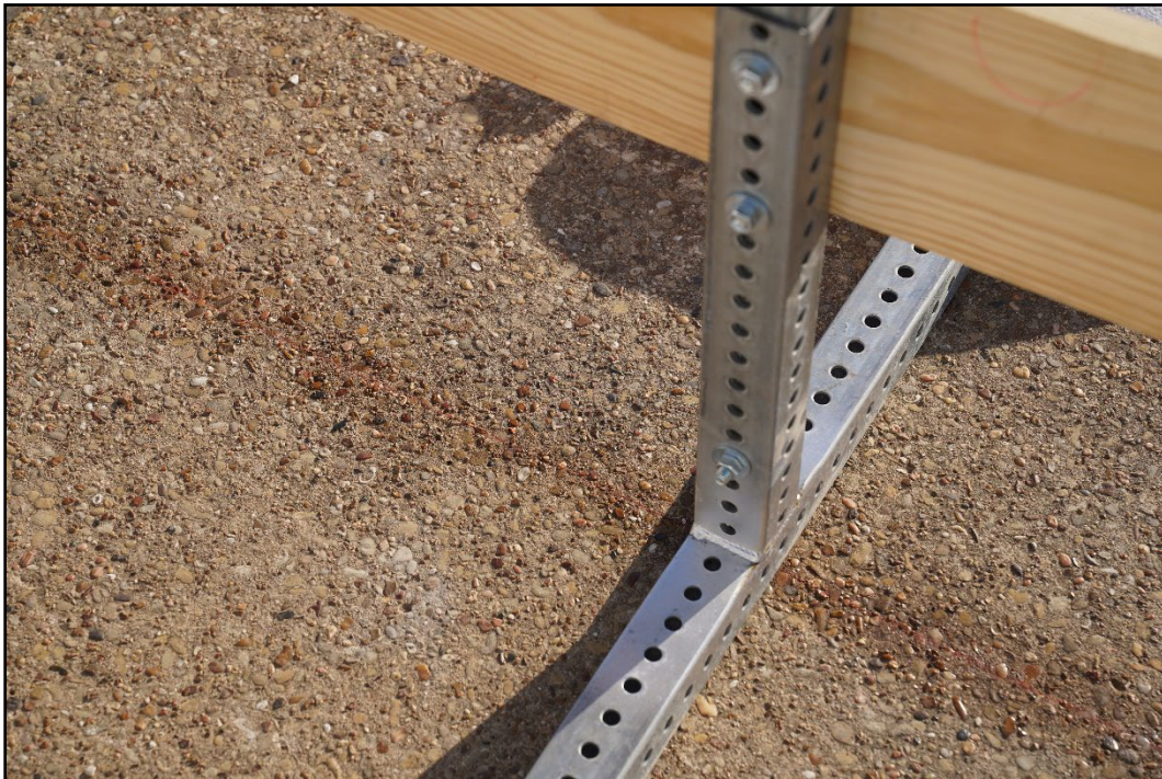
Figure 4.5. Rear View of the Base of the Type III Barricade with Mounted Sign prior to Testing.
