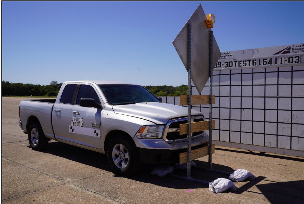
Figure 9.1. Type III Barricade with Mounted Sign/Test Vehicle Geometrics for Test 616411-01-3.
