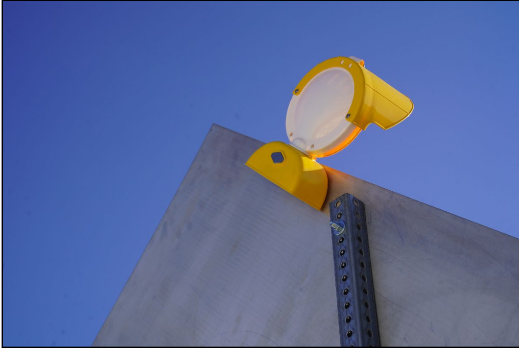
Figure 4.6. Rear View of the Flashing Light on the Type III Barricade with Mounted Sign prior to Testing.
