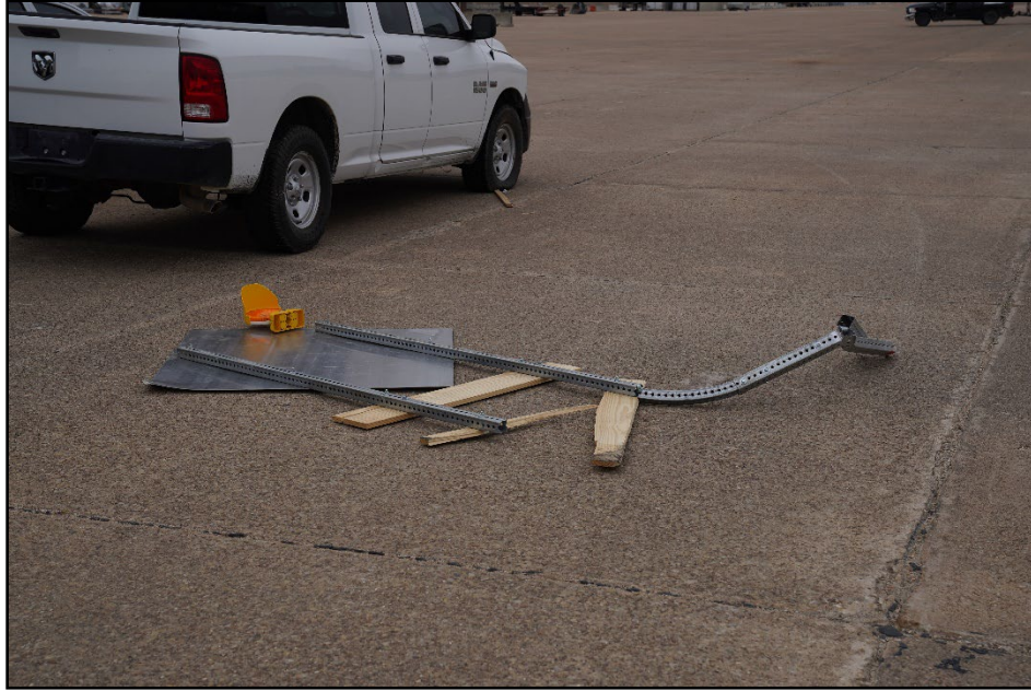
Figure 10.6. Type III Barricade with Mounted Sign after Test at its Final Resting Location 616411-01-4.
