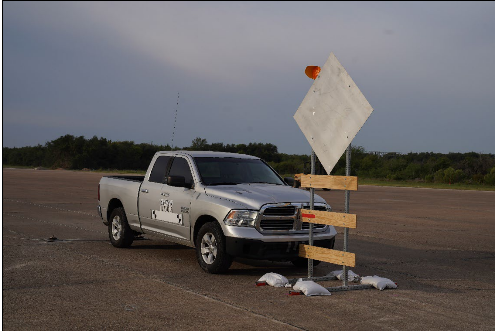
Figure 10.1. Type III Barricade with Mounted Sign/Test Vehicle Geometrics for Test 616411-01-4.
