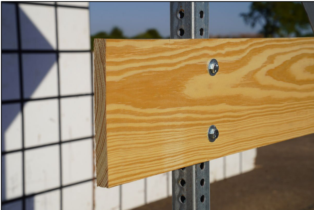
Figure 4.7. Pine Board and Hardware on the Type III Barricade with Mounted Sign prior to Testing.
