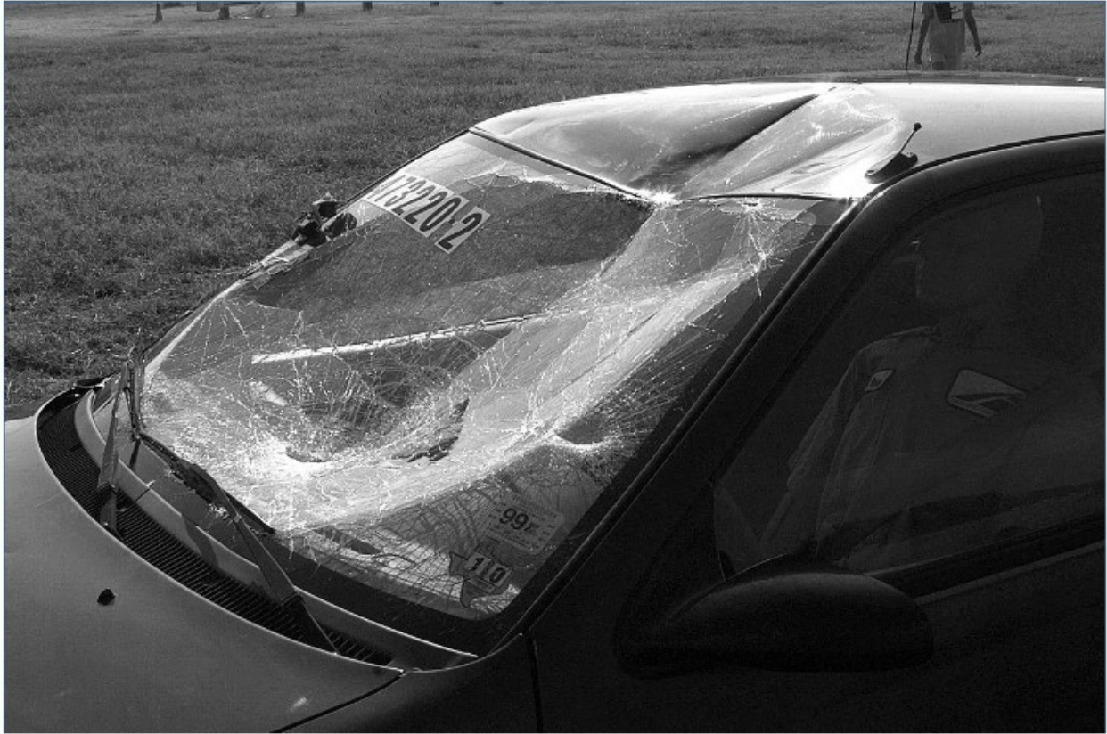
Figure 2.11: Windshield Damage to Vehicle from New Jersey Type III PVC Barricade Testing (5)
