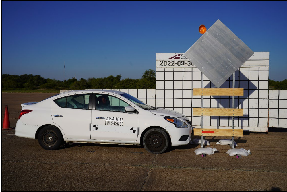
Figure 7.1. Type III Barricade with Mounted Sign/Test Vehicle Geometrics for Test 616411-01-1.
