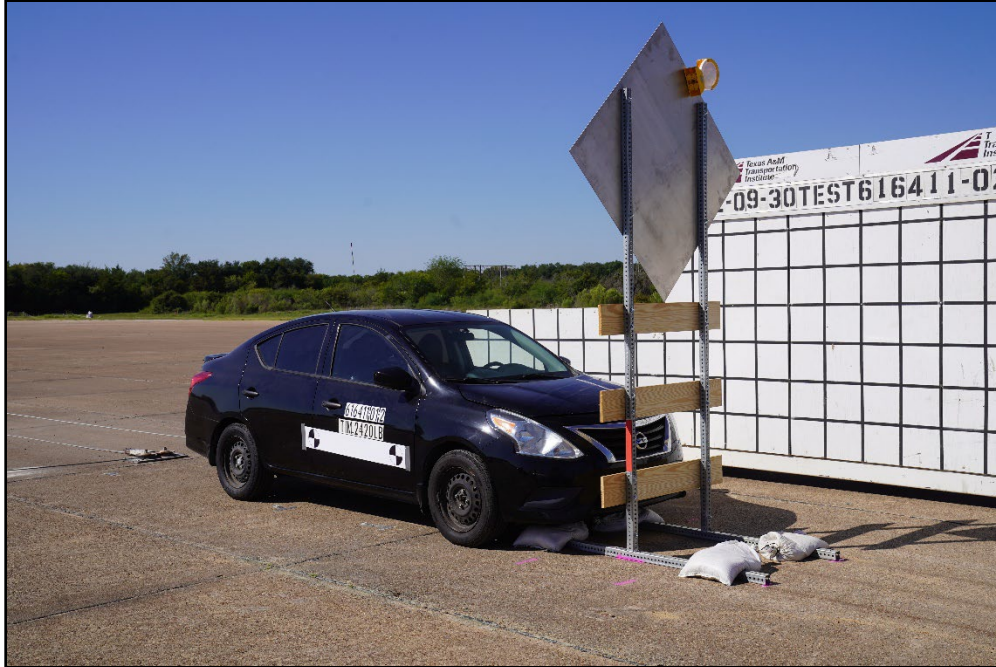
Figure 8.1. Type III Barricade with Mounted Sign/Test Vehicle Geometrics for Test 616411-01-2.
