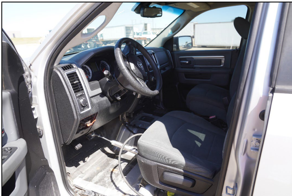
Figure 9.9. Overall Interior of Test Vehicle after Test 616411-01-3.
