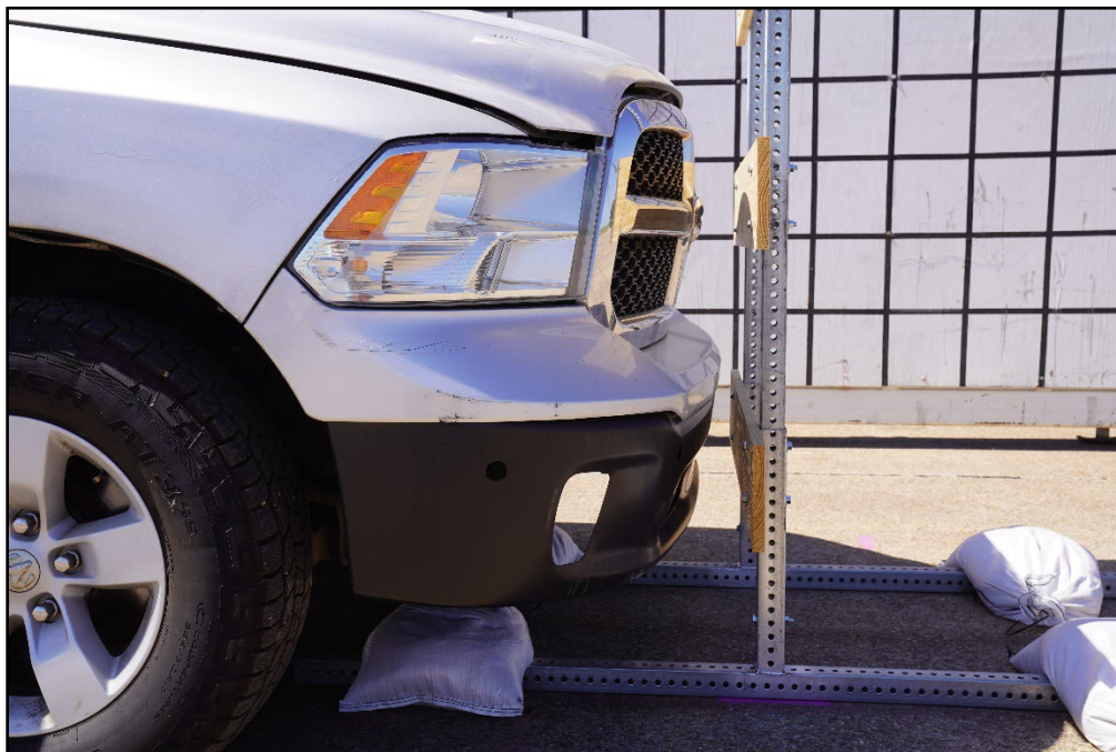
Figure 9.2. Type III Barricade with Mounted Sign/Test Vehicle Impact Location 616411-01-3.
