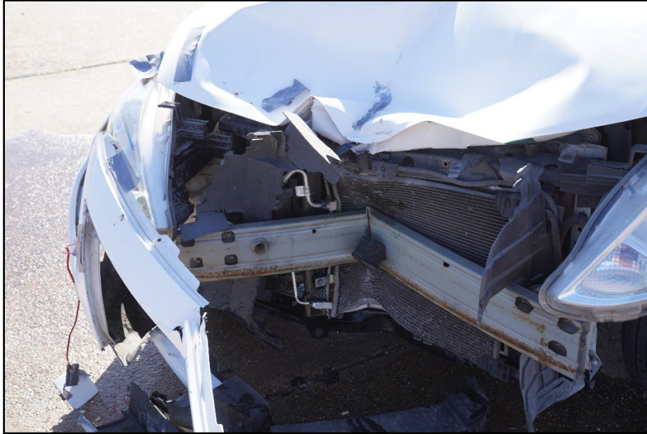
Figure 7.8. Front Bumper of Test Vehicle after Test 616411-01-1.
