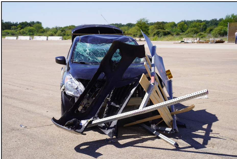
Figure 8.7. Impact Side of Test Vehicle after Test 616411-01-2.
