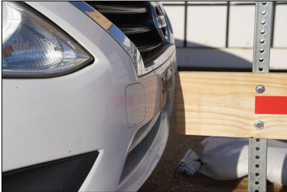
Figure 7.2. Type III Barricade with Mounted Sign/Test Vehicle Impact Location 616411-01-1.
