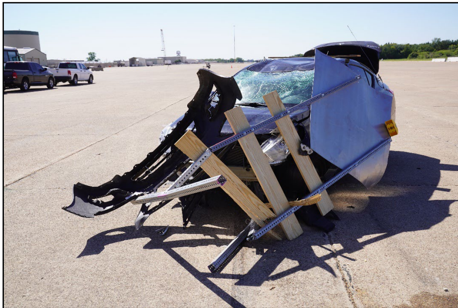
Figure 8.5. Type III Barricade with Mounted Sign after Test 616411-01-2.
