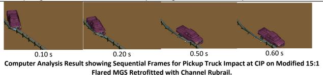
After crash testing and computer analysis, Project 609971 ultimately recommended crash testing a modified and retrofitted MGS system with a 15:1 flare using regular post spacing, shorter blockouts (6-inch X 8-inch X 10-inch), C6X8 rubrail centered at 12-inches from ground, and a steel non-flared terminal (such as a SoftStop) to minimize chances of anchor failure in future testing.
