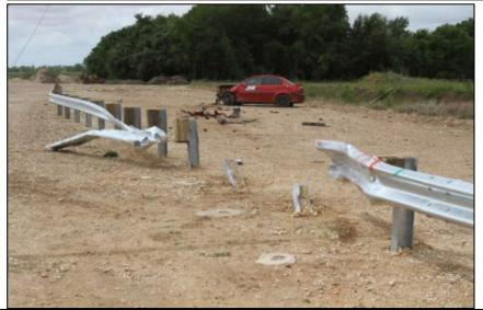
• 11:1 flared MGS system with pickup truck – failed, containment problem due to failed anchor
