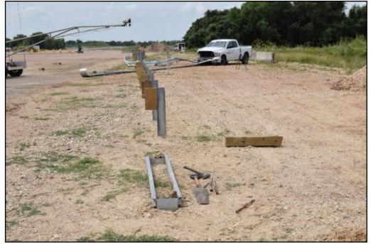
• 11:1 flared MGS section with non-flared MGS sections at the end of the system (shortened flared section) with a pickup truck – failed, ruptured rail
