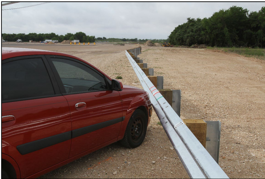
Figure 5.2. MGS Guardrail with Flare/Test Vehicle Impact Location for Test 609971-01-1.
