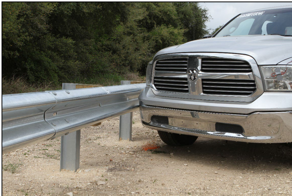
Figure 7.2. MGS Guardrail with Flare/Test Vehicle Impact Location for Test 609971-03-2.
