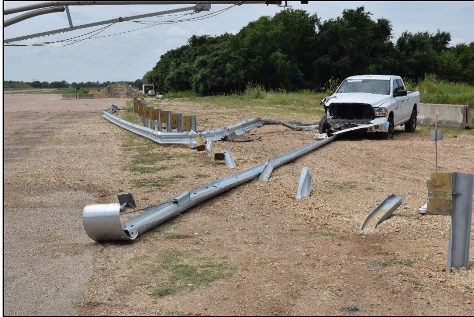
Figure 6.5. MGS Guardrail with Flare after Test at Impact Location for Test 609971-03-1.
