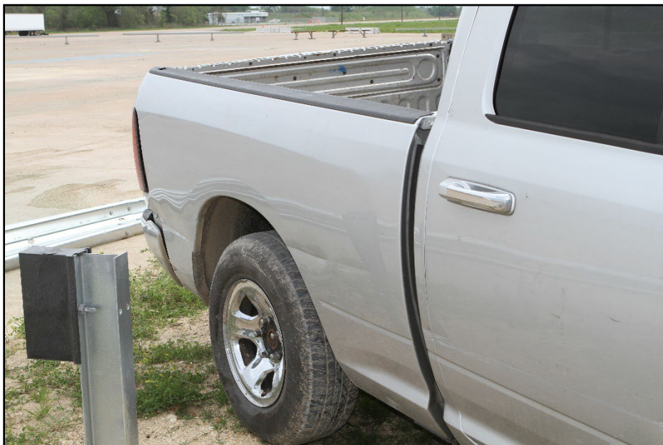
Figure 7.8. Rear Impact Side of Test Vehicle after Test 609971-03-2.
