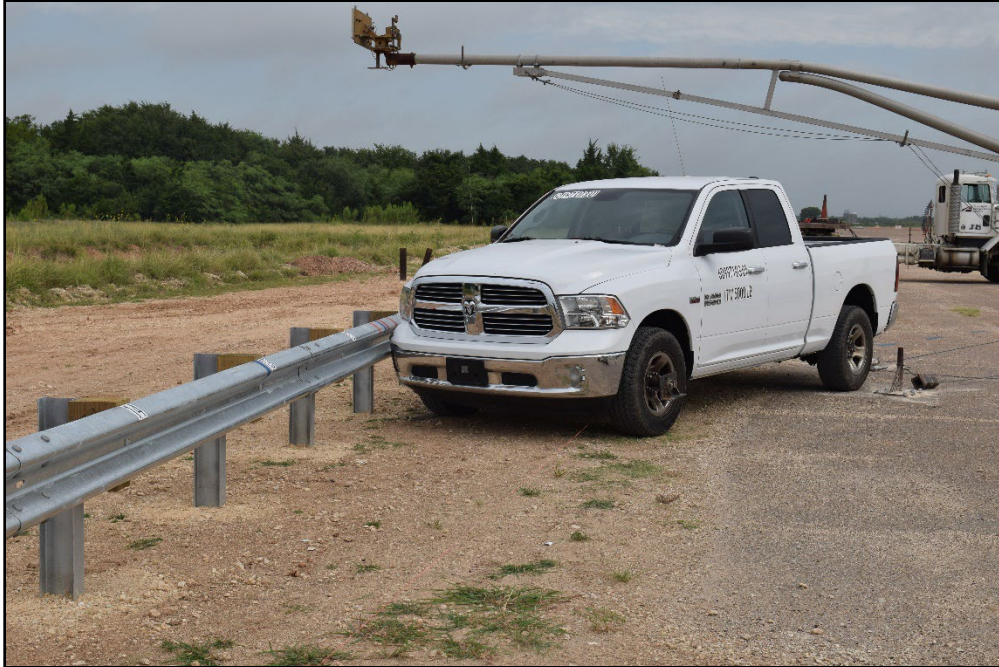
Figure 6.1. MGS Guardrail with Flare/Test Vehicle Geometrics for Test 609971-03-1.
