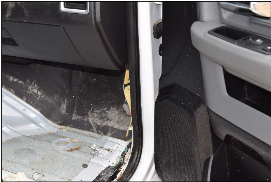
Figure 6.10. Interior of Test Vehicle on Impact Side after Test 609971-03-1.
