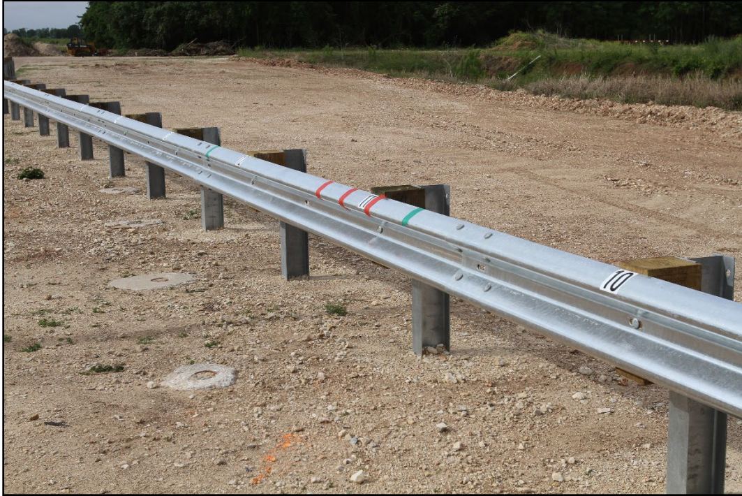
Figure 2.4. MGS Guardrail with 7:1 Flare at Impact prior to Testing.
