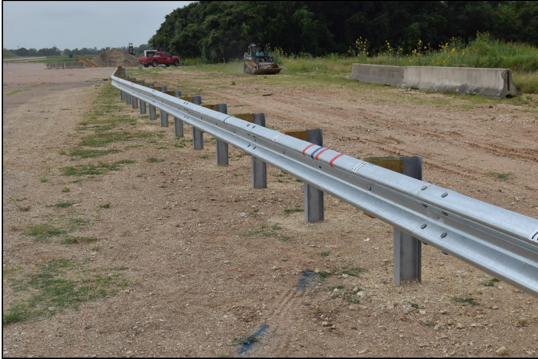
Figure 2.9. MGS Guardrail with 11:1 Flare at Impact prior to Testing.
