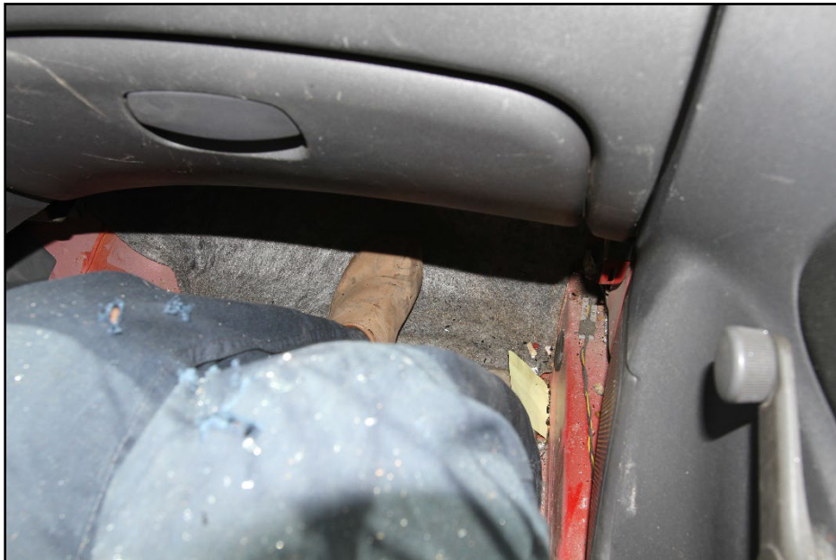
Figure 5.10. Interior of Test Vehicle on Impact Side after Test 609971-01-1.
