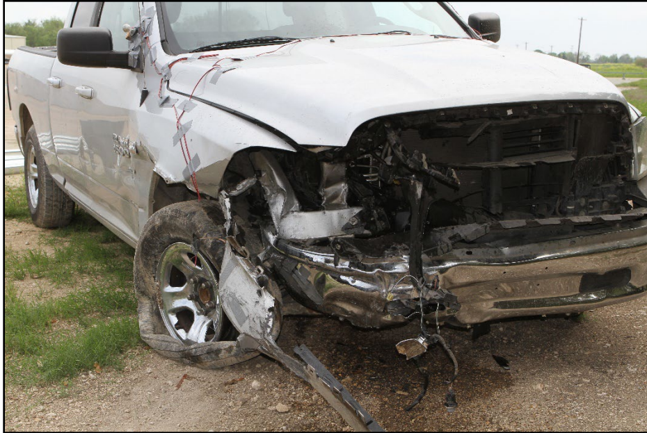
Figure 7.7. Impact Side of Test Vehicle after Test 609971-03-2.
