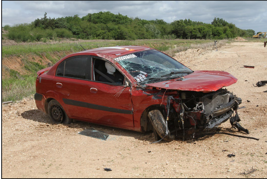
Figure 5.7. Impact Side of Test Vehicle after Test 609971-01-1.
