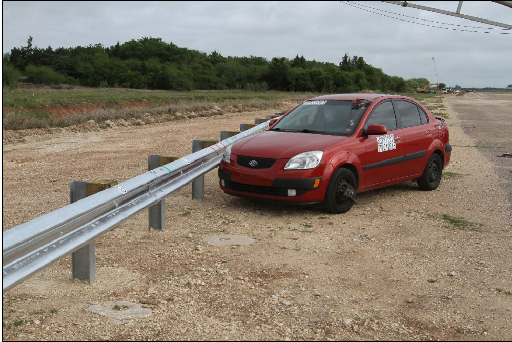
Figure 5.1. MGS Guardrail with Flare/Test Vehicle Geometrics for Test 609971-01-1.
