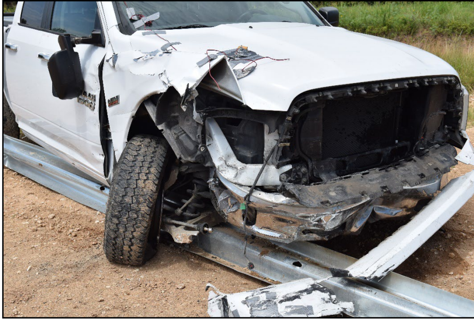
Figure 6.7. Impact Side of Test Vehicle after Test 609971-03-1.
