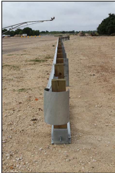
Figure 2.5. In-line View of the MGS Guardrail with 7:1 Flare prior to Testing.
