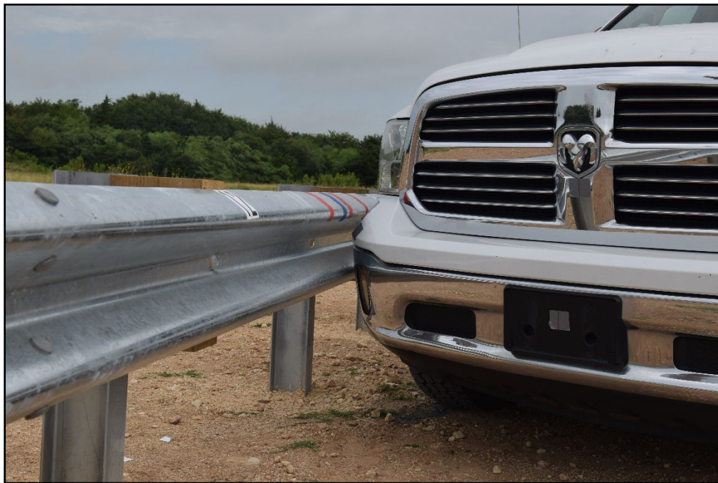
Figure 6.2. MGS Guardrail with Flare/Test Vehicle Impact Location for Test 609971-03-1.
