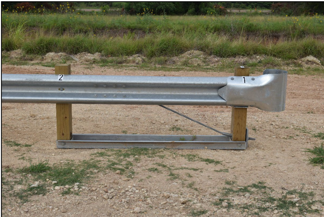
Figure 2.8. Upstream Terminal of the MGS Guardrail with 11:1 Flare prior to Testing.
