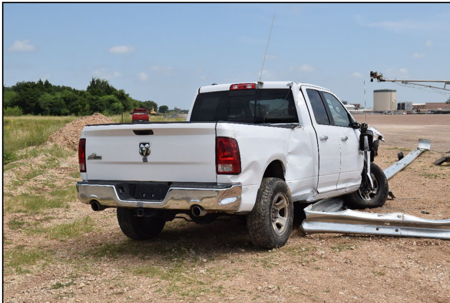
Figure 6.8. Rear Impact Side of Test Vehicle after Test 609971-03-1.
