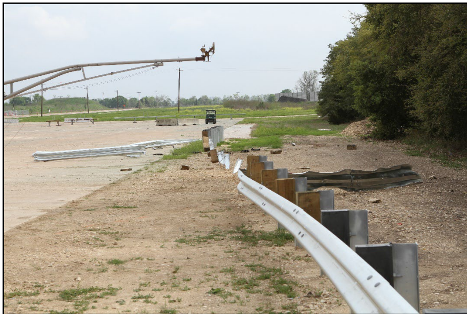
Figure 7.6. MGS Guardrail with Flare after Test 609971-03-2.
