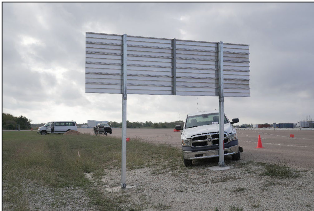
Figure 7.2. Large Sign Slip Base Support/Test Vehicle Impact Location 612261-05-2.
