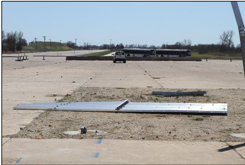
Figure 6.5. Large Sign Slip Base Support after Test at Impact Location 612261-04-1.
