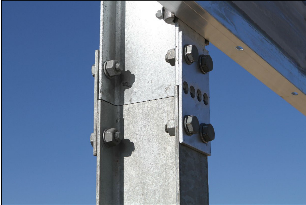
Figure 2.11. Front Plate of the Large Sign Slip Base Support Prior to Testing 612261-04-1.
