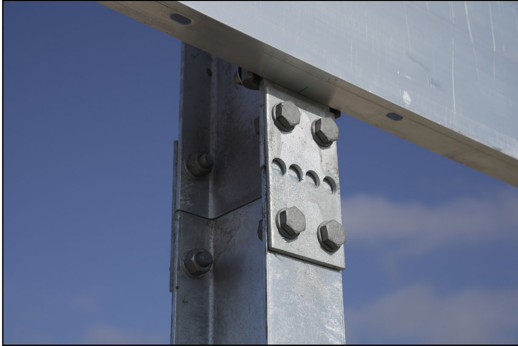
Figure 2.18. Front Plate of the Large Sign Slip Base Support on a Slope Prior to Testing 612261-05-2.
