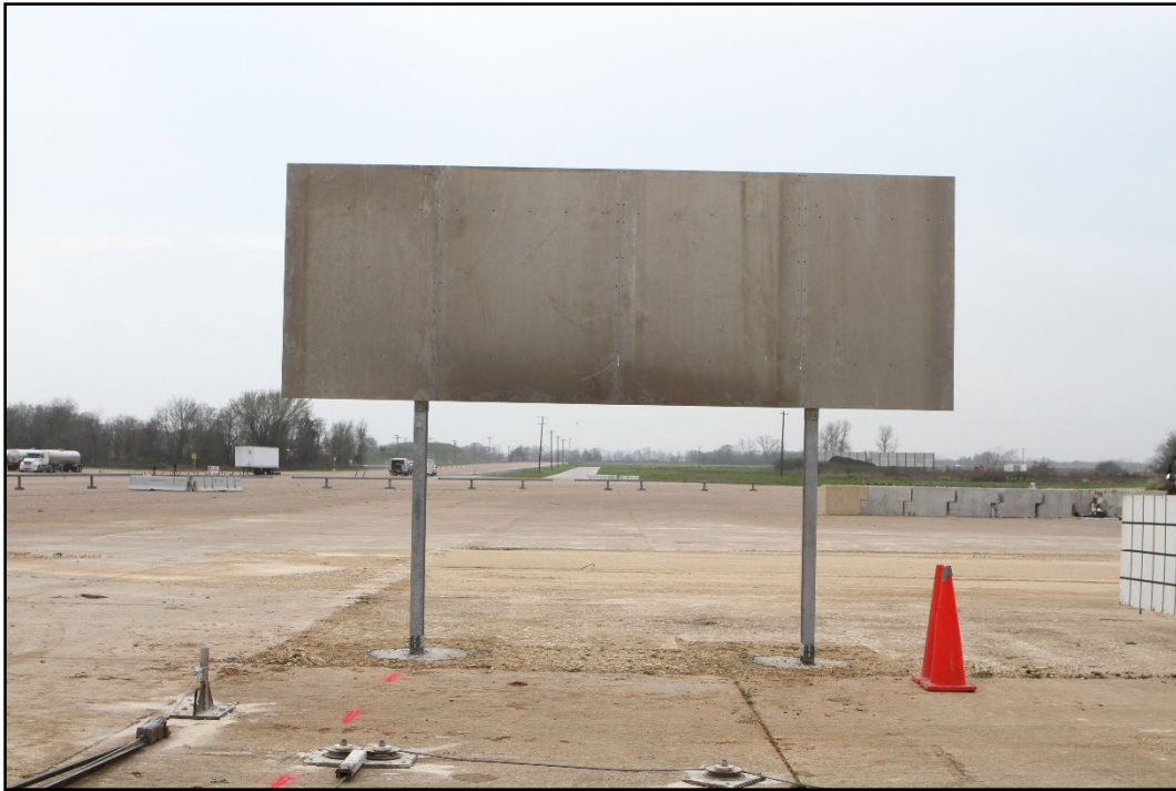
Figure 2.2. Large Sign Slip Base Support from the Impact Side Prior to Testing 612261-05-1.
