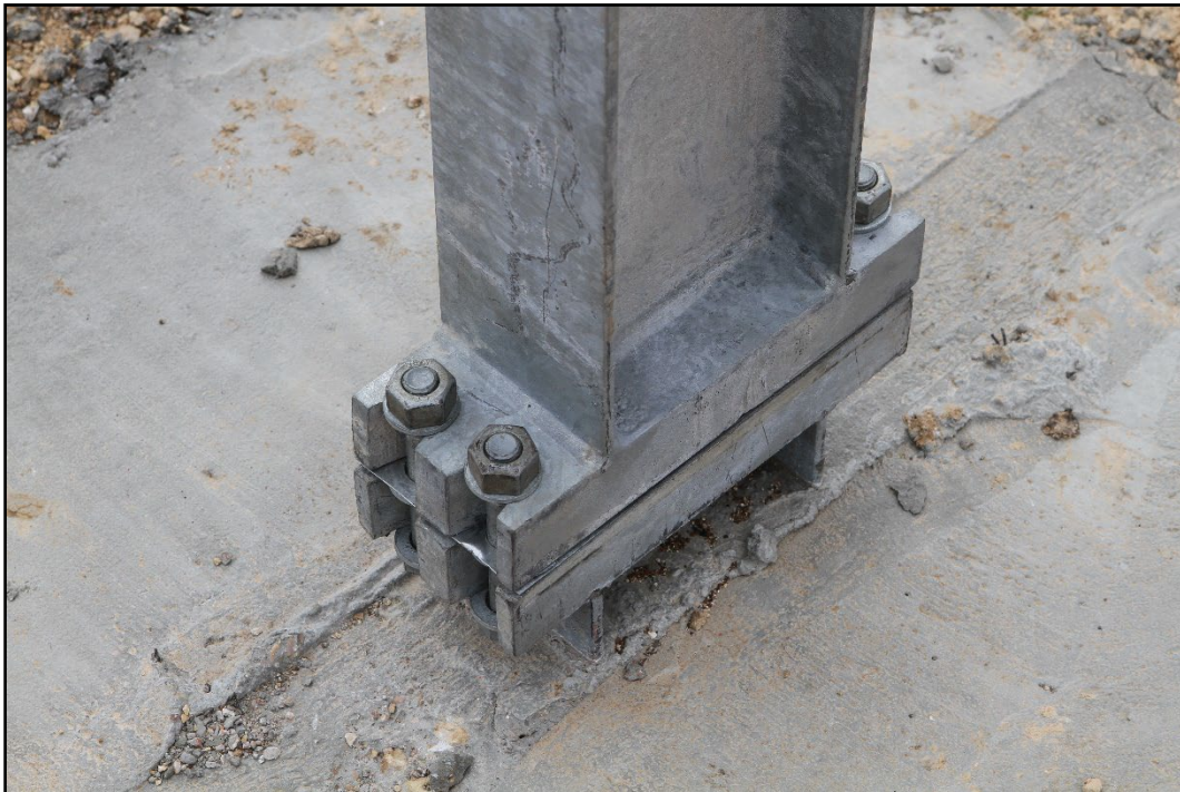
Figure 2.7. Opposite of the Impact Side of the Base of the Large Sign Slip Base Support Prior to Testing 612261-05-1.
