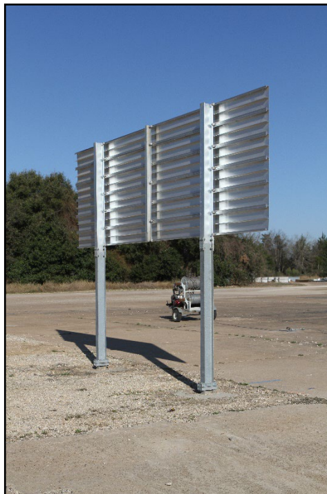
Figure 2.10. Large Sign Slip Base Support from Opposite of the Impact Side Prior to Testing 612261-04-1.
