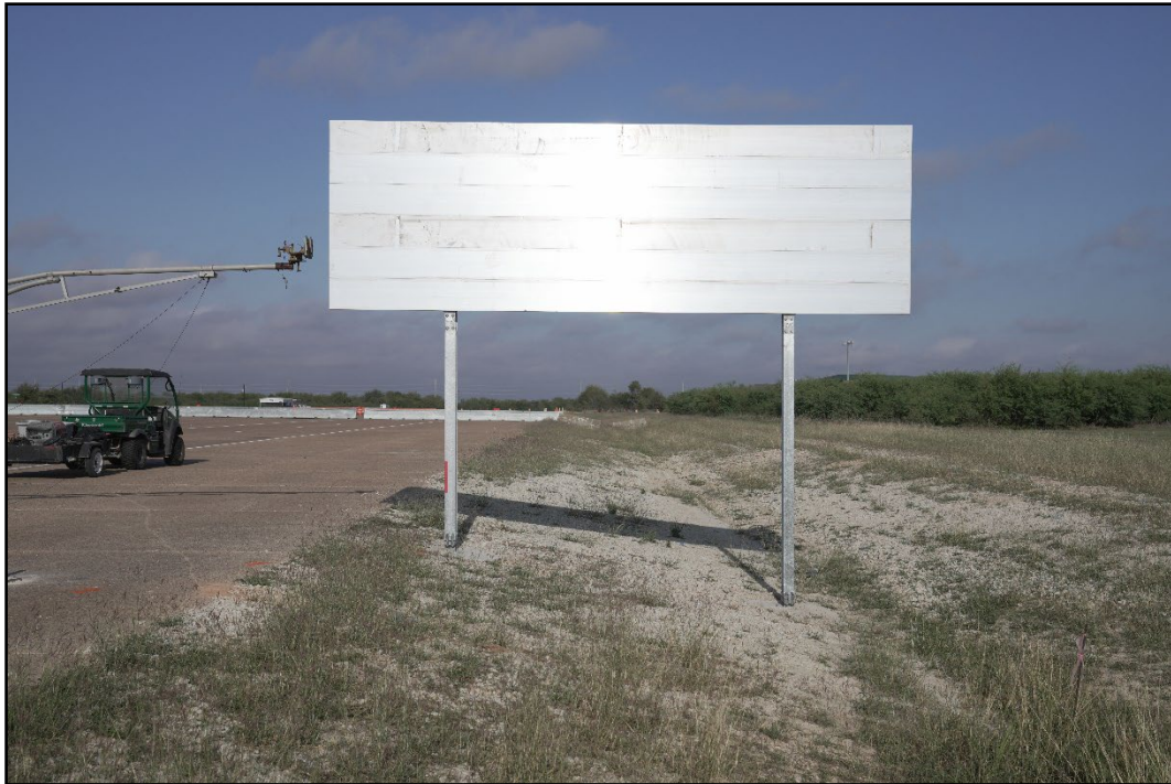
Figure 2.16. Large Sign Slip Base Support on a Slope Prior to Testing 612261-05-2.
