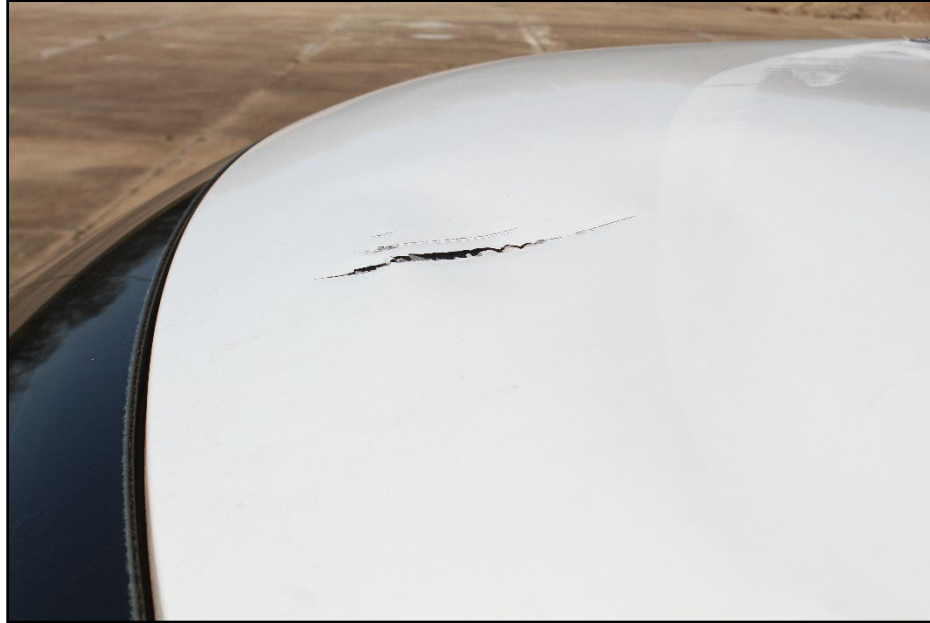
Figure 6.8. Roof Damage on Test Vehicle after Test 612261-04-1.
