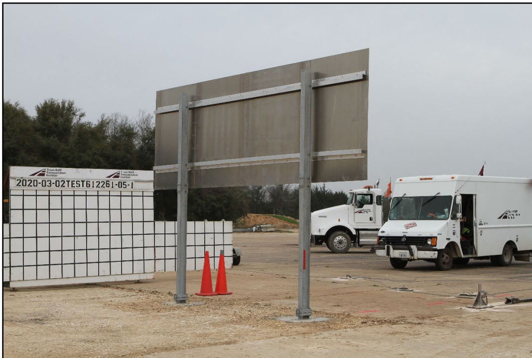
Figure 2.3. Large Sign Slip Base Support from Opposite of the Impact Side Prior to Testing 612261-05-1.
