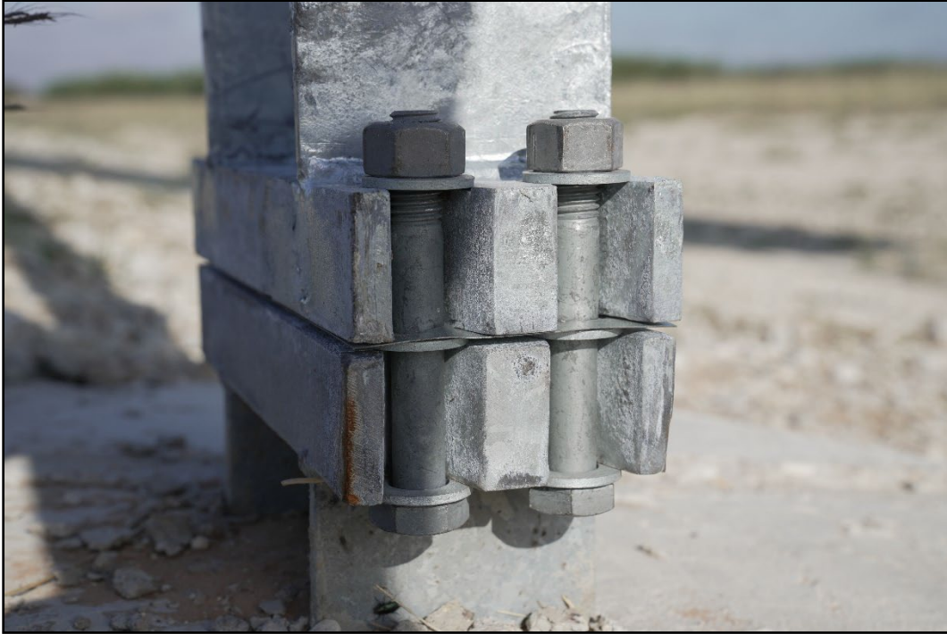
Figure 2.20. Front View of the Base of the Large Sign Slip Base Support on a Slope Prior to Testing 612261-05-2.
