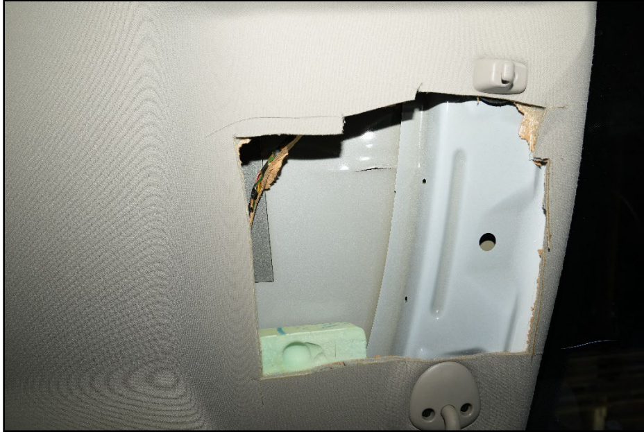
Figure 6.10. Interior of Test Vehicle Roof on Impact Side after Test 612261-04-1.
