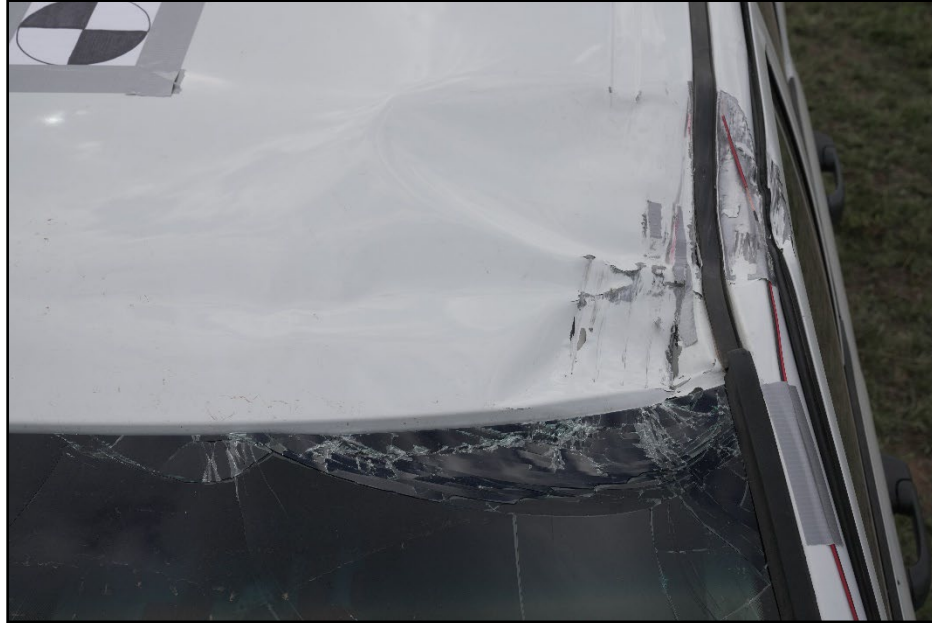
Figure 7.9. Roof of Test Vehicle after Test 612261-05-2.
