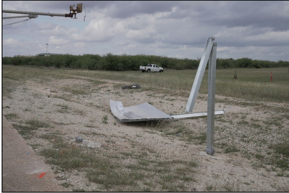
Figure 7.5. Large Sign Slip Base Support after Test at Impact Location 612261-05-2.
