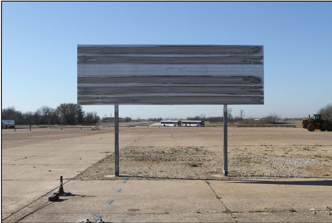
Figure 2.9. Large Sign Slip Base Support from the Impact Side Prior to Testing 612261-04-1.
