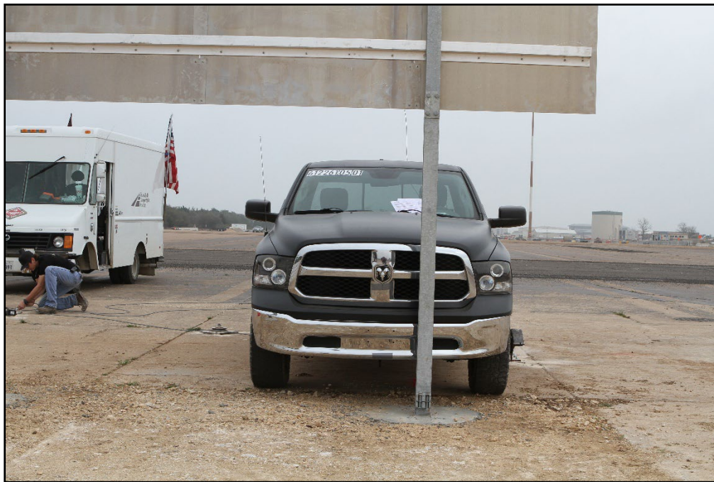
Figure 5.2. Large Sign Slip Base Support/Test Vehicle Impact Location 6122561-05-1.
