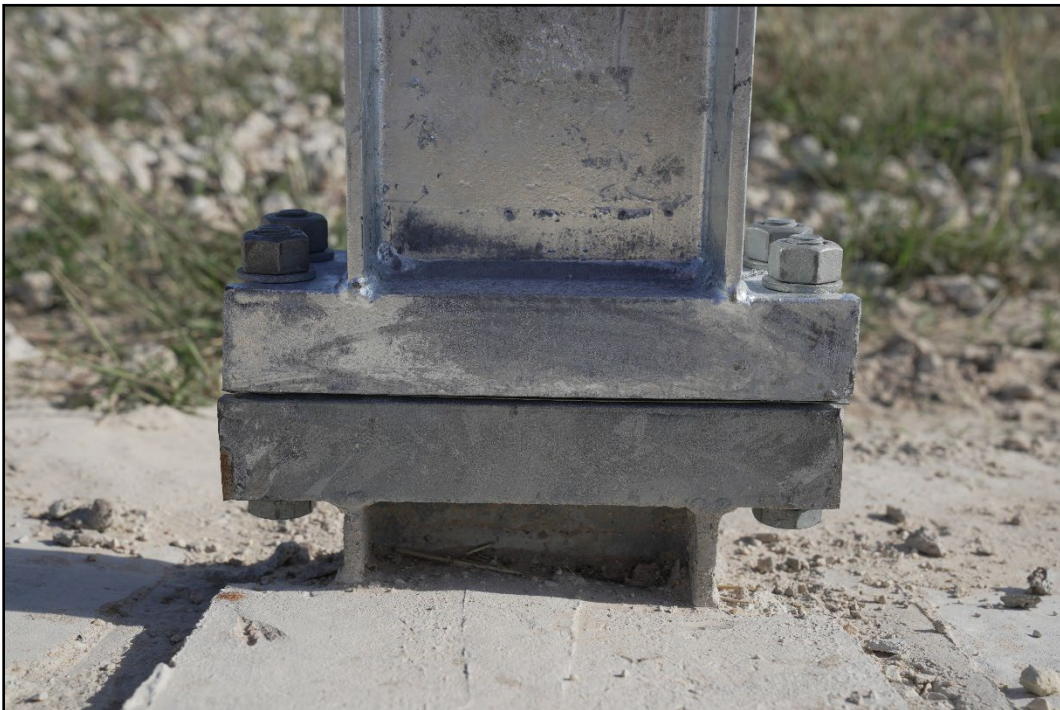
Figure 2.21. Side View of the Base of the Large Sign Slip Base Support on a Slope Prior to Testing 612261-05-2.
