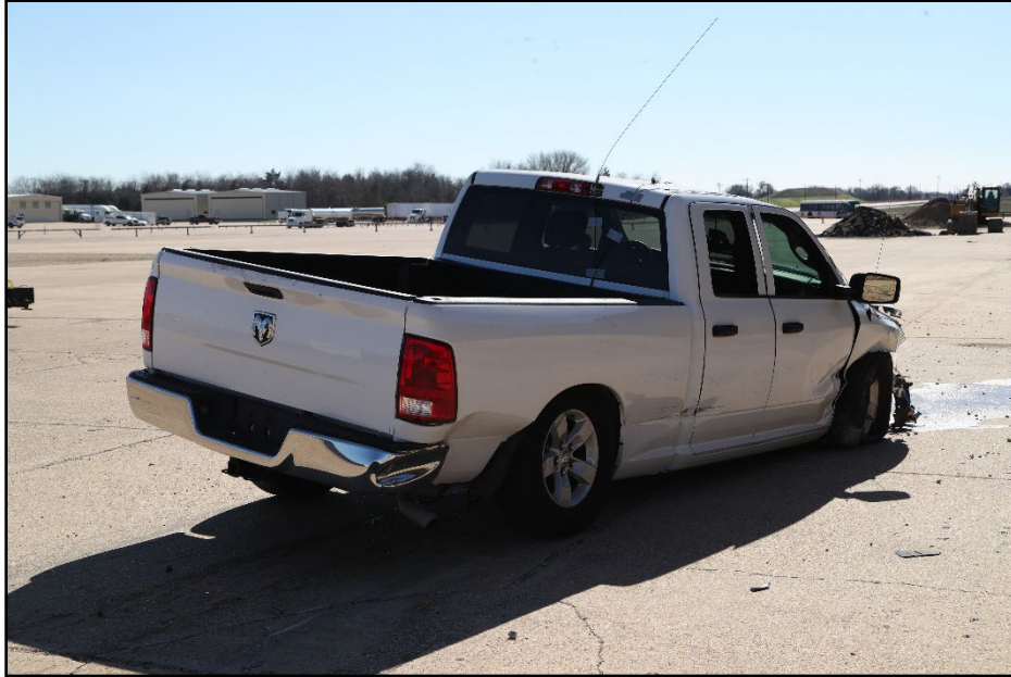
Figure 8.8. Rear Impact Side of Test Vehicle after Test 615251-01-1.
