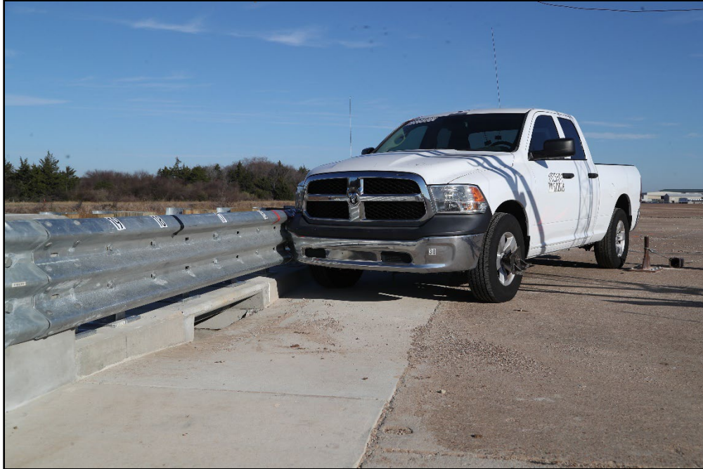
Figure 8.1. Transition with Storm Drain Inlet/Test Vehicle Geometrics for Test 615251-01-1.
