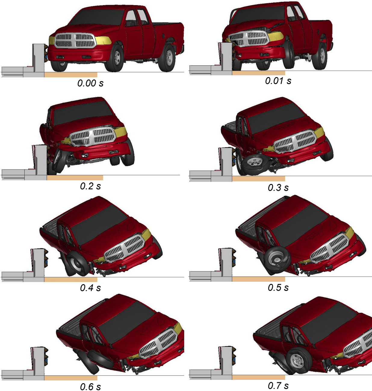
Figure 4.7. Sequential Images of Truck Impacting the Transition System with 40-inch Inlet Offset at Upstream End of the Inlet (IP3).
