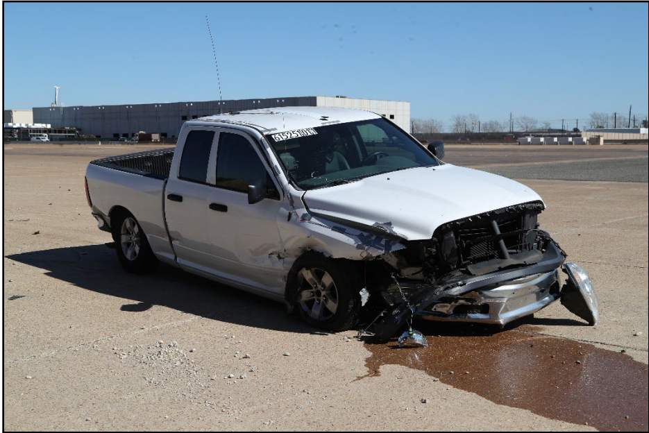
Figure 8.7. Impact Side of Test Vehicle after Test 615251-01-1.
