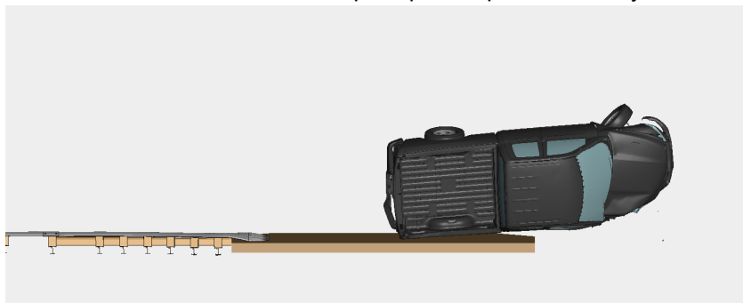
d. Time = 0.420 seconds: pickup truck loses contact with parapet
