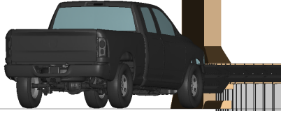
a. Time = 0.025 seconds: pickup truck impacts thrie beam
