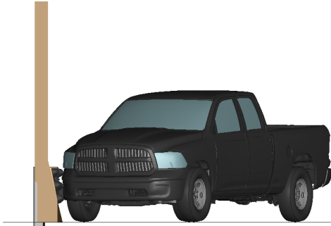
a. Time = 0.025 seconds: pickup truck impacts thrie beam
