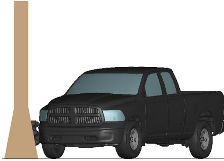
a. Time = 0.025 seconds: pickup truck impacts thrie beam
