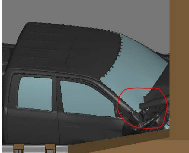
Figure 3.10. Corner of Hood Intruding into Windshield after Hood Contact with Tall Wall.
