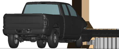
b. Time = 0.060 seconds: pickup truck impacts end of extended parapet
