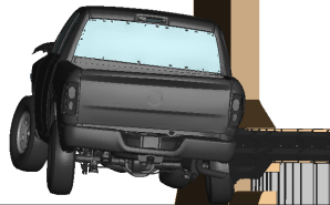
c. Time = 0.215 seconds: pickup truck parallel with system
