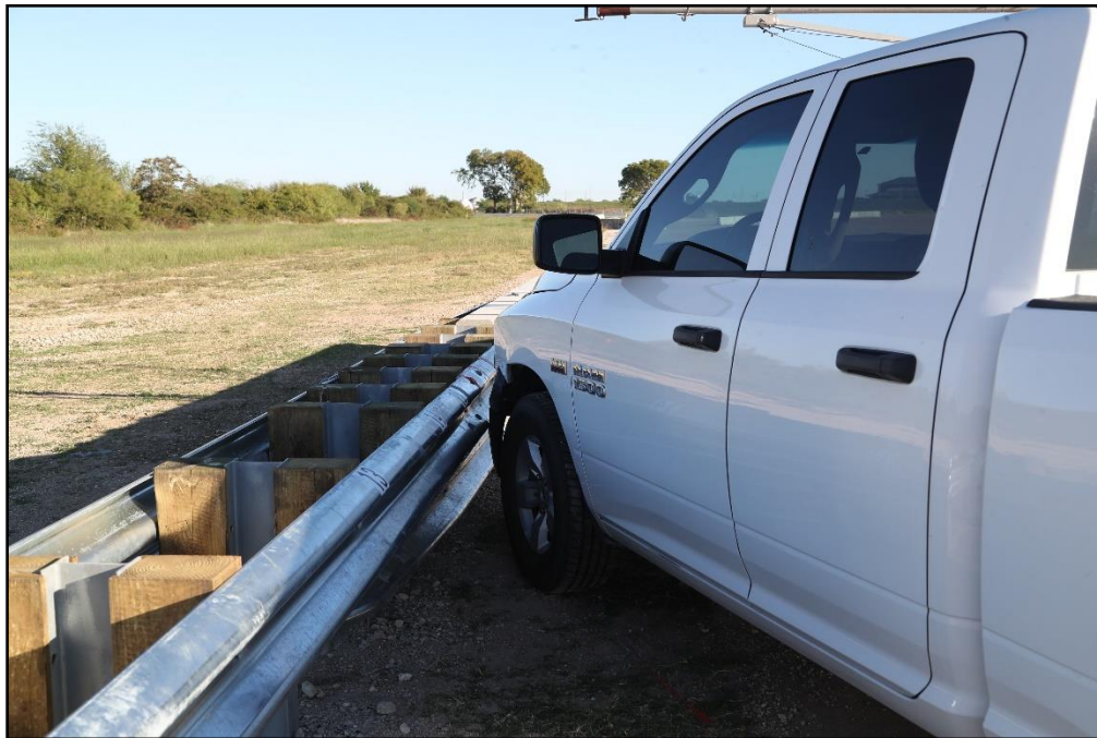
Figure 6.2. Median Guardrail Transition to Median F-Shape Barrier/Test Vehicle Impact Location for Test 618851-01-1.
