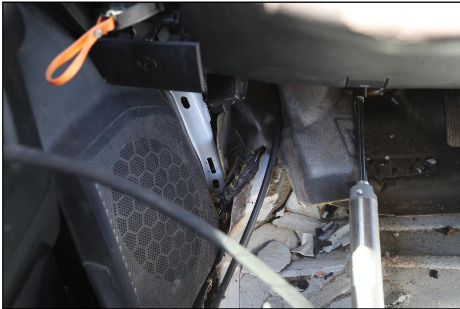
Figure 6.10. Seam Separation on Impact Side after Test 618851-01-1.
