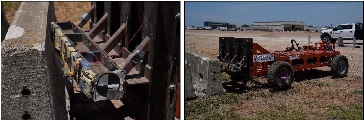
Figure 2.11. Bogie Test Vehicle after Test No. 619441-01-3.
