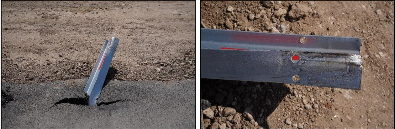
**Figure 2.12. Post after Test No. 619441-01-4.**
