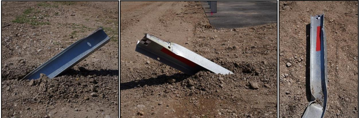
**Figure 2.4. Soil Embedded Post after Test No. 619441-01-1.**
