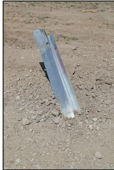
Figure 2.6. Soil Embedded Post after Test No. 619441-01-8.
