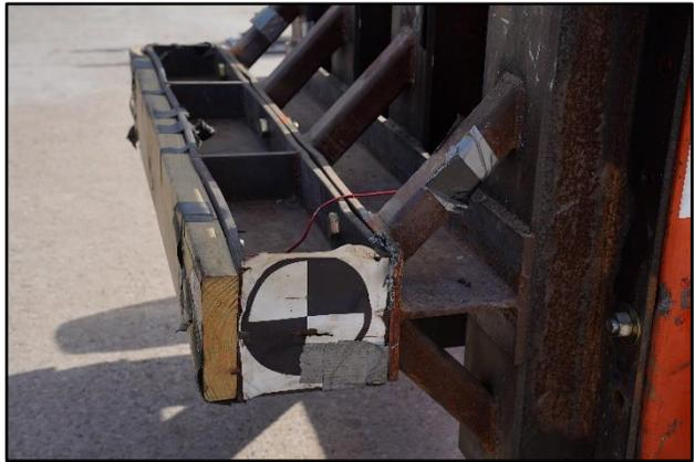
**Figure 2.3. Bogie Test Vehicle before Test No. 619441-01-1.**
