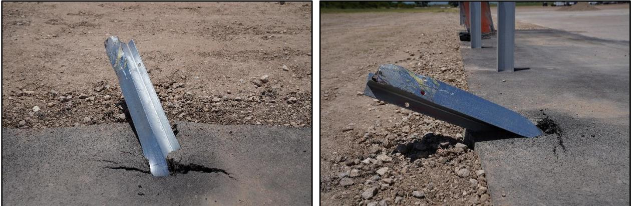
Figure 2.10. Post after Test No. 619441-01-3.
