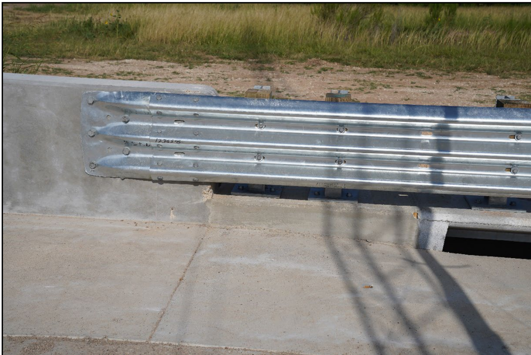
Figure 2.3. TL-3 Transition with a Storm Drain Inlet at the Transition prior to Testing.
