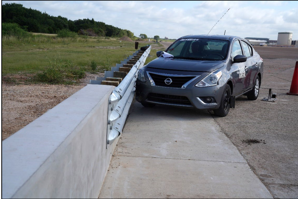
Figure 5.1. TL-3 Transition with a Storm Drain Inlet/Test Vehicle Geometrics for Test 619551-01-1.
