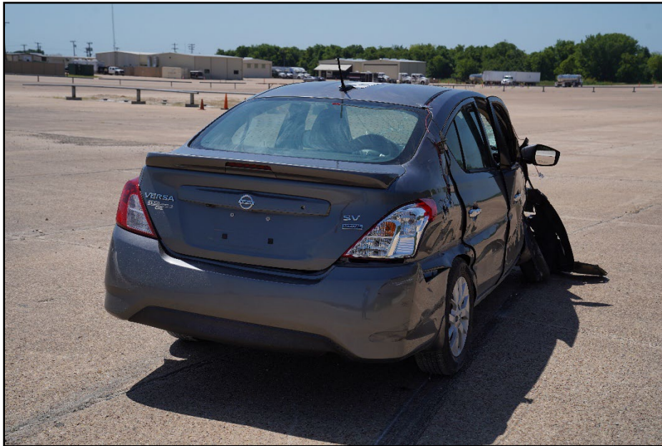
Figure 5.8. Rear Impact Side of Test Vehicle after Test 619551-01-1.
