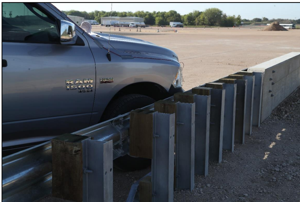
Figure 6.2. Shortened Transition/Test Vehicle Impact Location 618981-01-1.
