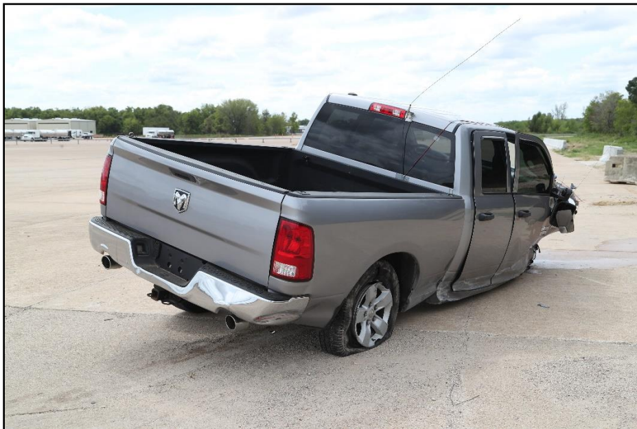
Figure 6.8. Rear Impact Side of Test Vehicle after Test 618981-01-1.
