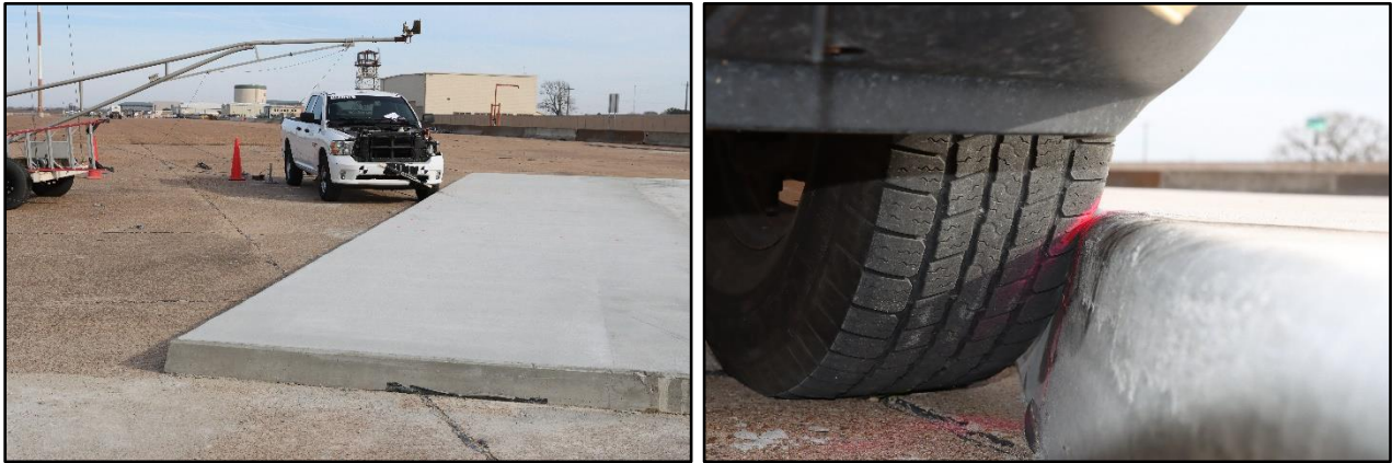
Figure 3.7. Sidewalk/Test Vehicle Geometrics for Test No. 614091-01-2
