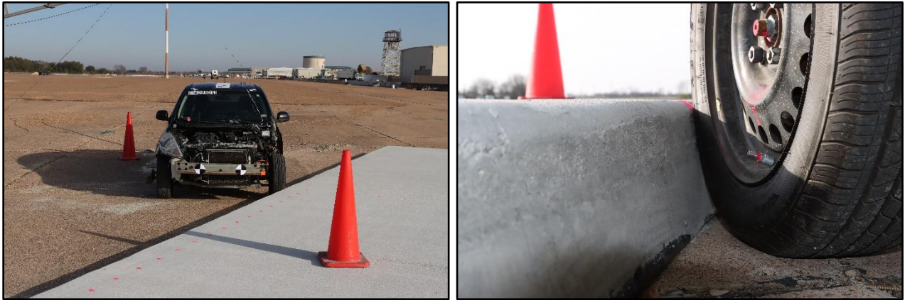
Figure 3.3. Sidewalk/Test Vehicle Geometrics for Test No. 614091-01-1
