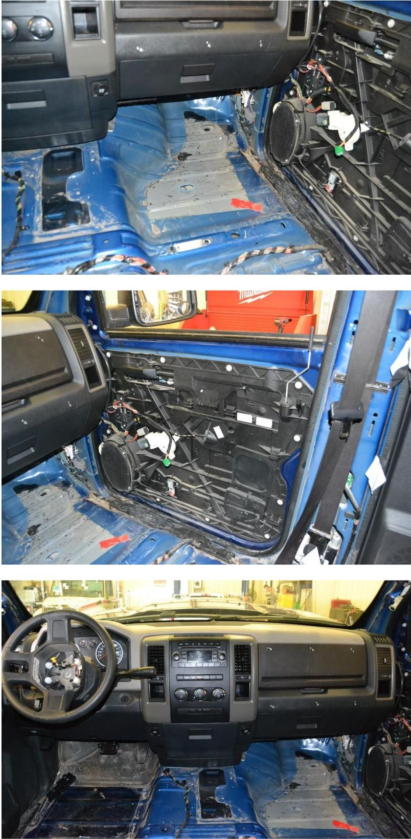
Figure 78. Occupant Compartment Vehicle Damage, Test No. NYBWT-2
