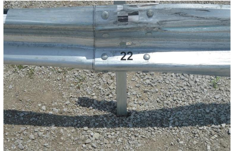
Figure 69. Rail and Post Damage, Post Nos. 19 through 22, Test No. NYBWT-2
