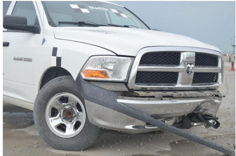
Figure 98. Vehicle Damage, Test No. NYBWT-3
