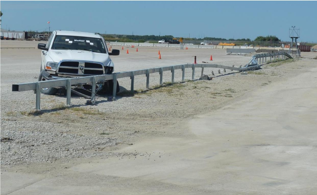
Figure 88. Vehicle Trajectory Marks and Final Position, Test No. NYBWT-3
