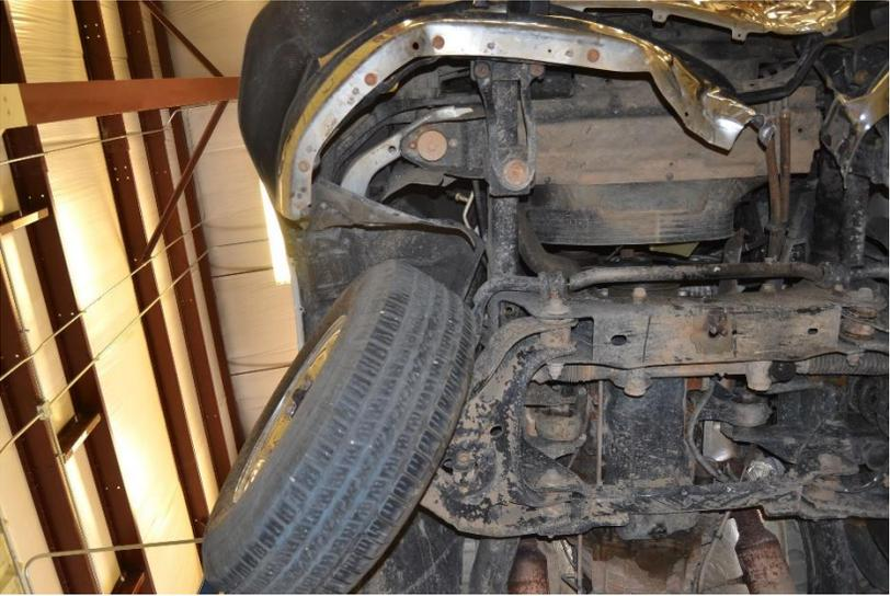
Figure 99. Undercarriage Vehicle Damage, Test No. NYBWT-3
