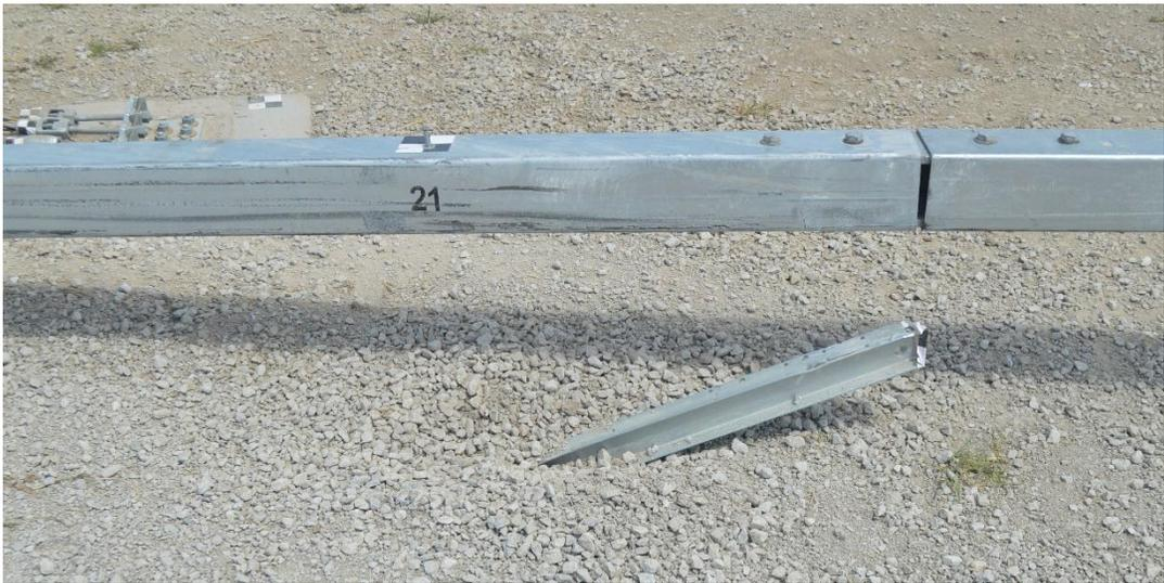
Figure 93. Damage to System at Post Nos. 19 through 21
