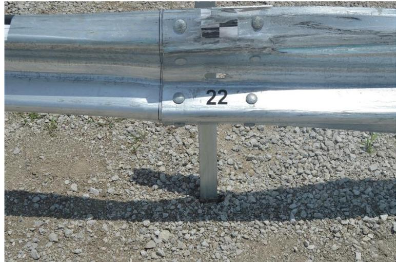
Figure 71. Rail and Post Damage, Post Nos. 19 through 22, Test No. NYBWT-2
