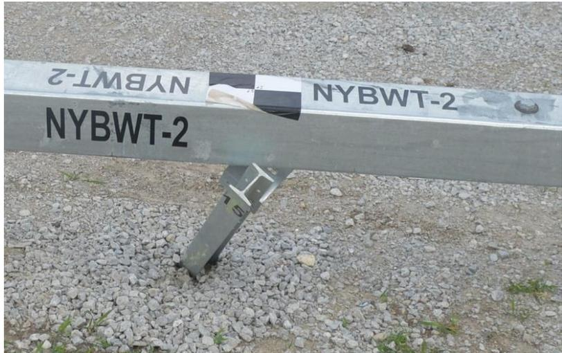
Figure 70. Backside Rail and Post Damage, Post Nos. 12 through 15, Test No. NYBWT-2
