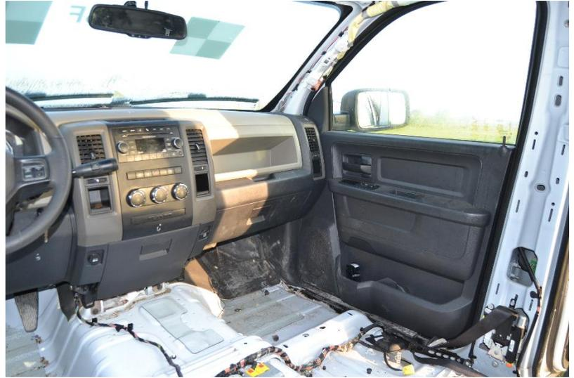
Figure 100. Occupant Compartment Damage, Test No. NYBWT-3
