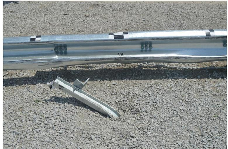
Figure 68. Rail and Post Damage, Post Nos. 15 through 18, Test No. NYBWT-2
