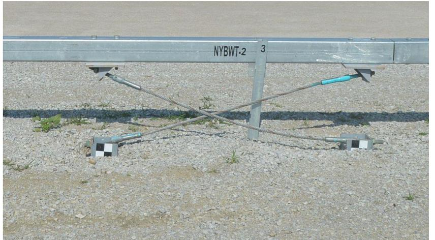
Figure 74 Anchor Damage, Test No. NYBWT-2
