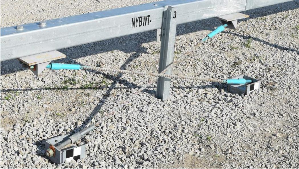
Figure 39. Anchors, Test No. NYBWT-2
