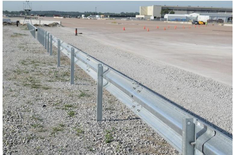
Figure 37. Box Beam and W-Beam Rails, Test No. NYBWT-2
