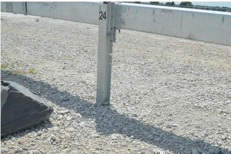
Figure 94. Damage to System at Post Nos. 22 through 24
