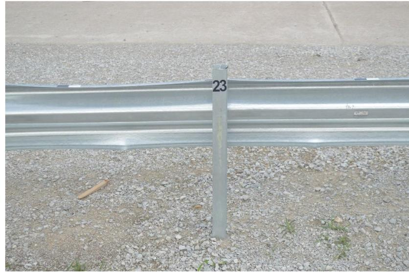
Figure 73. Backside Rail and Post Damage, Post Nos. 20 through 23, Test No. NYBWT-2
