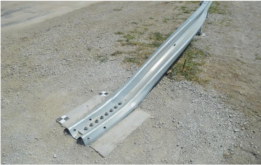
Figure 95. Anchor Damage, Test No. NYBWT-3
