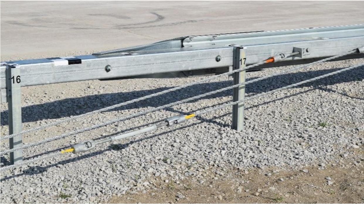
Figure 40. Transition Cover Assembly, Test No. NYBWT-2
