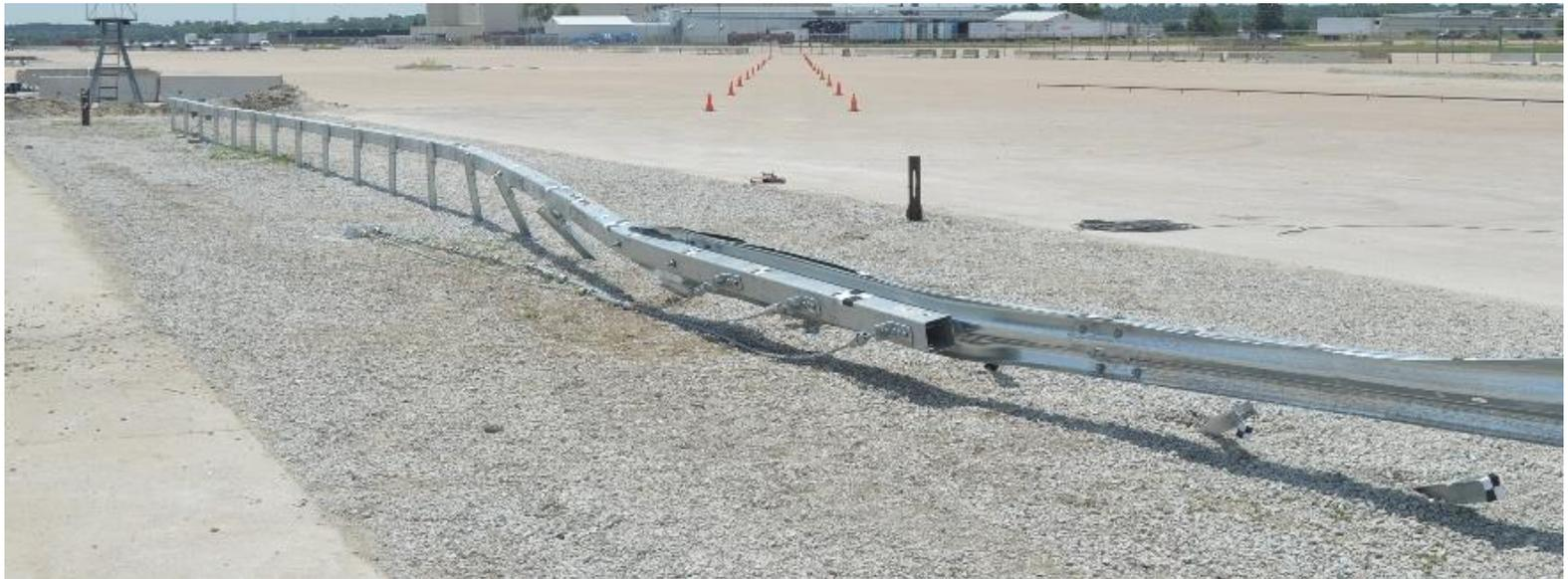
Figure 66. Overall System Damage, Test No. NYBWT-2
