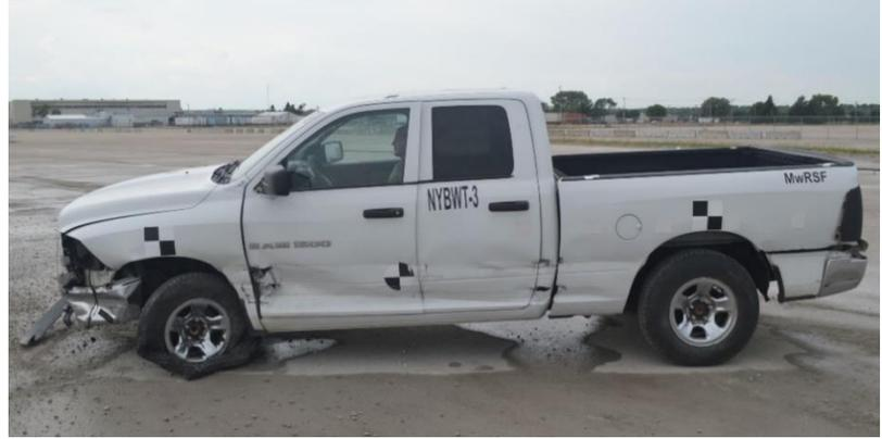
Figure 97. Vehicle Damage, Test No. NYBWT-3
