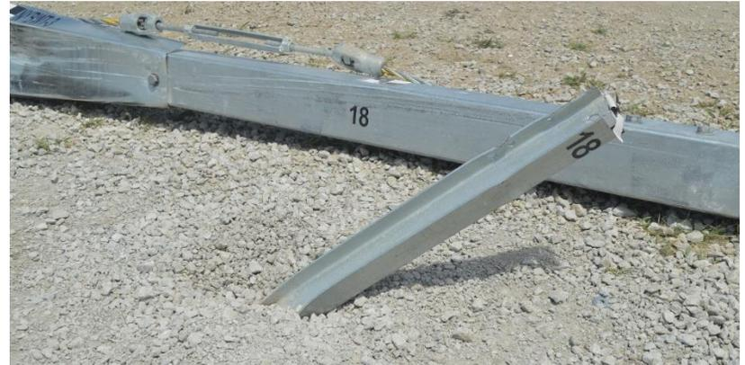
Figure 92. Damage to Post Nos. 15 through 18, Test No. NYBWT-3
