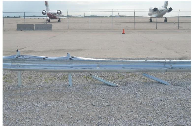
Figure 67. System Damage, Test No. NYBWT-2
