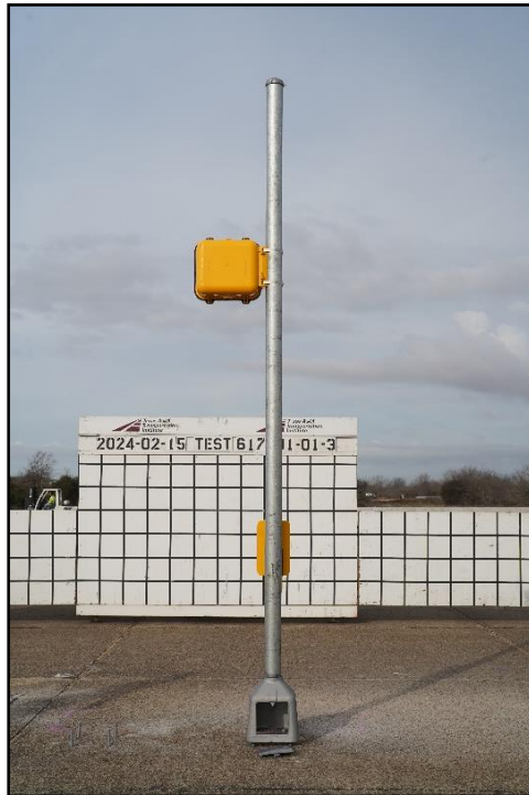
Figure 4.16. MUTCD Standard Pedestrian Signal Prior to Crash Tests 617891-01 3&4.
