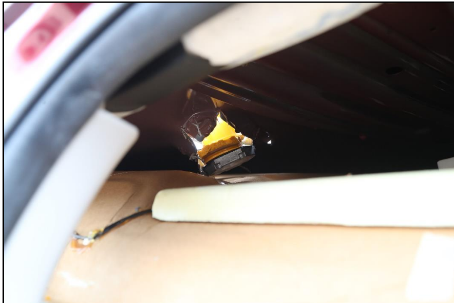
Figure 8.10. Test Article Penetration into the Test Vehicle after Test 617891-01-2.
