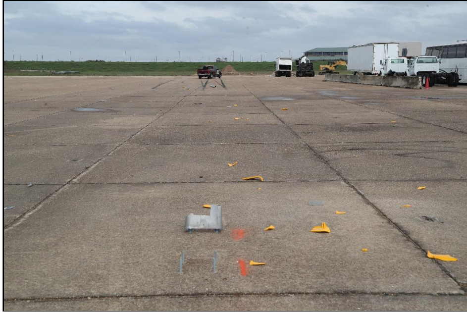
Figure 8.5. MUTCD Standard Pedestrian Signal at Impact Location after Test 617891-01-2.
