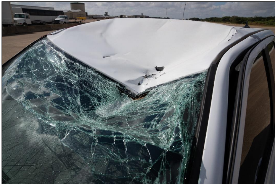
Figure 7.8. Roof and Windshield of the Test Vehicle after Test 617891-01-1.
