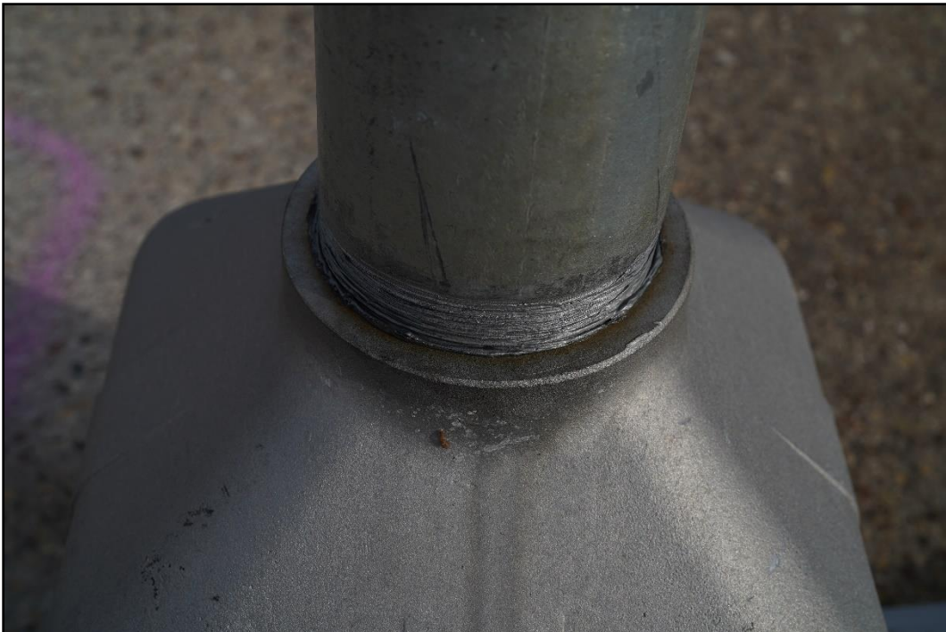
Figure 4.19. MUTCD Standard Pedestrian Signal Base Prior to Crash Tests 617891-01 3&4.
