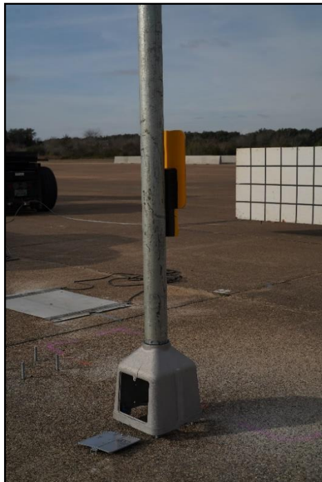
Figure 4.21. Oblique View of the MUTCD Standard Pedestrian Signal Prior to Crash Tests 617891-01 3&4.
