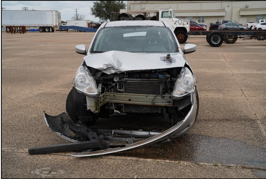
Figure 10.7. Impact Side of Test Vehicle after Test 617891-01-4.
