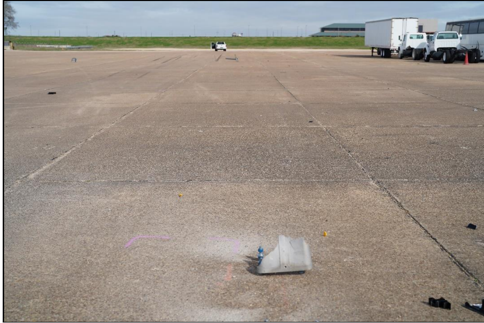
Figure 9.5. MUTCD Standard Pedestrian Signal at Impact Location after Test 617891-01-3.
