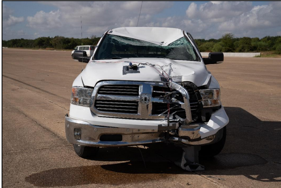
Figure 7.7. Front of the Test Vehicle after Test 617891-01-1.
