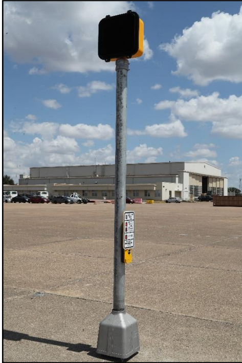
Figure 4.4. 0 Degree Angle of the MUTCD Standard Pedestrian Signal Prior to Crash Test 617891-01-1.
