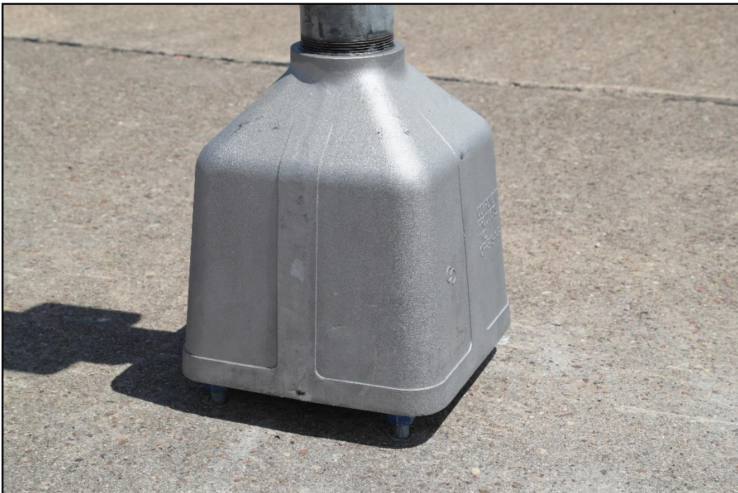
Figure 4.3. MUTCD Standard Pedestrian Signal Base Prior to Crash Test 617891-01-1.
