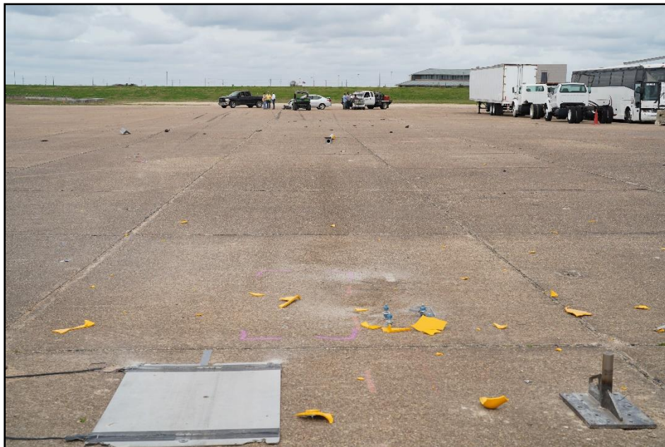
Figure 10.5. MUTCD Standard Pedestrian Signal at Impact Location after Test 617891-01-4.
