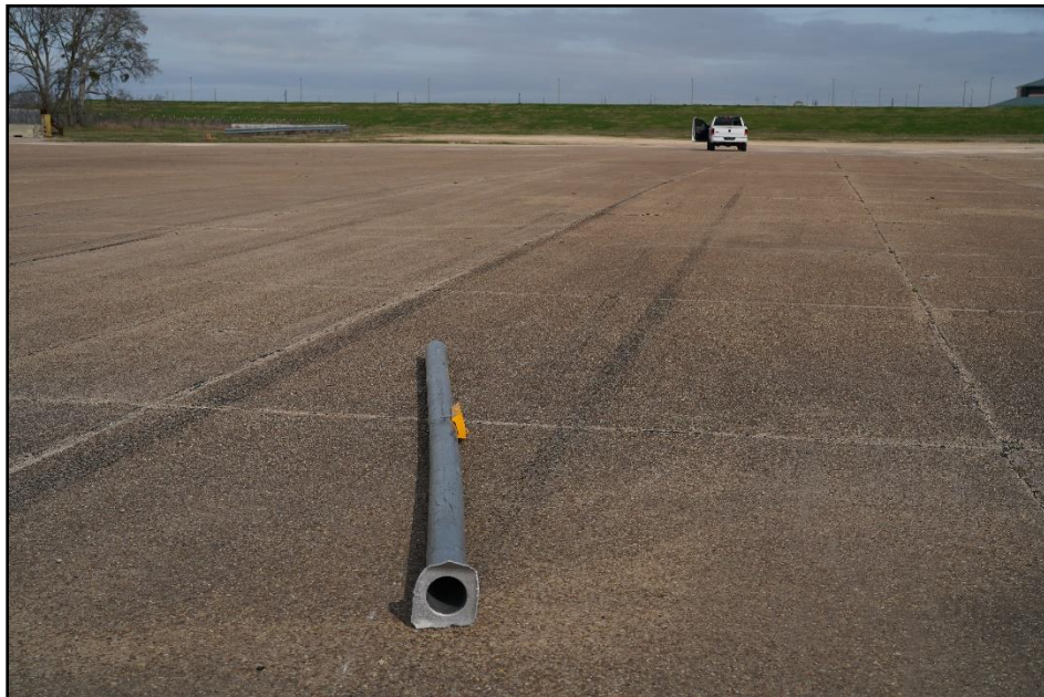
Figure 9.6. MUTCD Standard Pedestrian Signal Landing Location after Test 617891-01-3.
