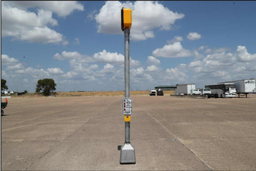
Figure 4.2. 90 Degree View of the MUTCD Standard Pedestrian Signal Prior to Crash Test 617891-01-1.
