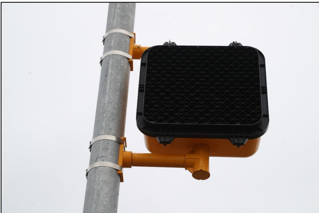
Figure 4.12. MUTCD Standard Pedestrian Signal Head Prior to Crash Test 617891-01-2.
