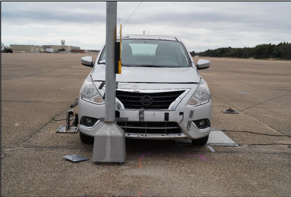
Figure 10.2. MUTCD Standard Pedestrian Signal /Test Vehicle Impact Location 617891-01-4.
