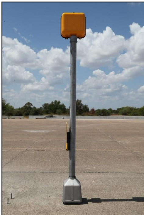
Figure 4.5. 180 Degree View of the MUTCD Standard Pedestrian Signal Prior to Crash Test 617891-01-1.
