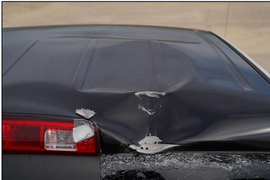
Figure 9.8. Rear Impact Side of Test Vehicle after Test 617891-01-3.
