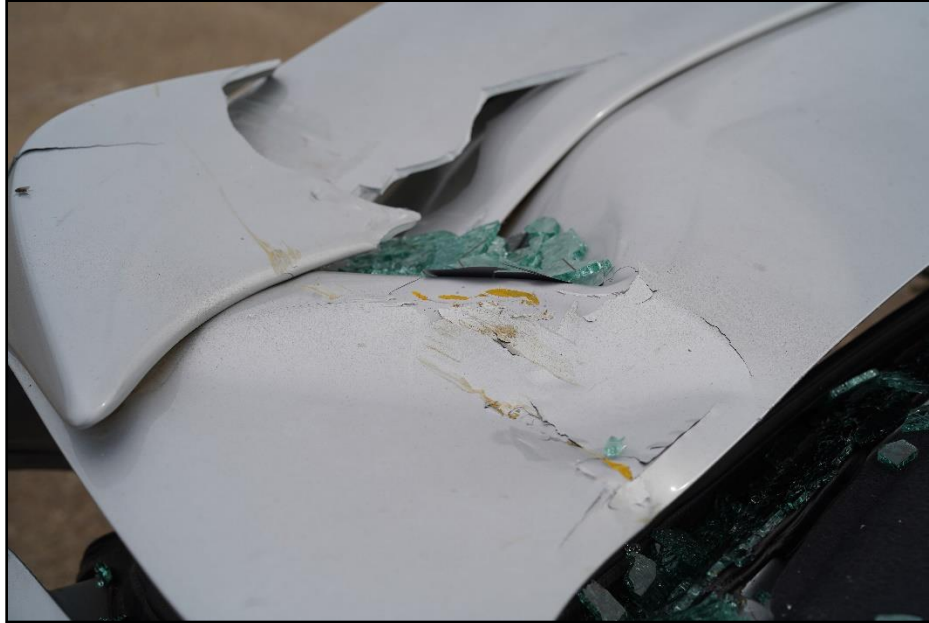
Figure 10.9. Trunk Lid of Test Vehicle after Test 617891-01-4.
