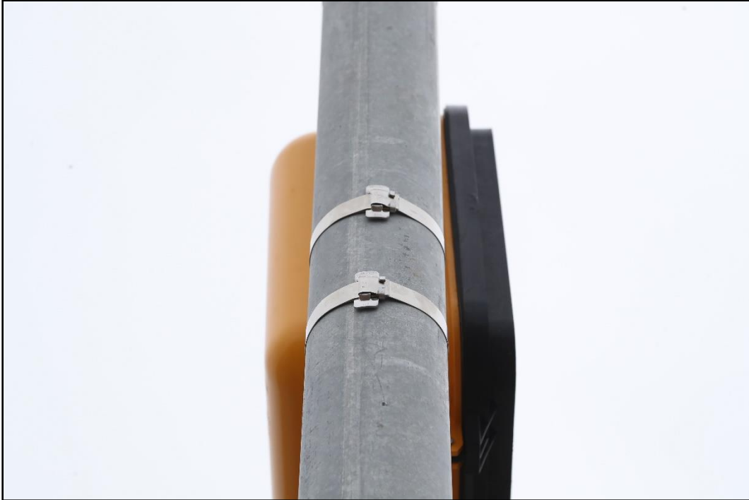
Figure 4.13. MUTCD Standard Pedestrian Signal Head Attachment Straps Prior to Crash Test 617891-01-2.
