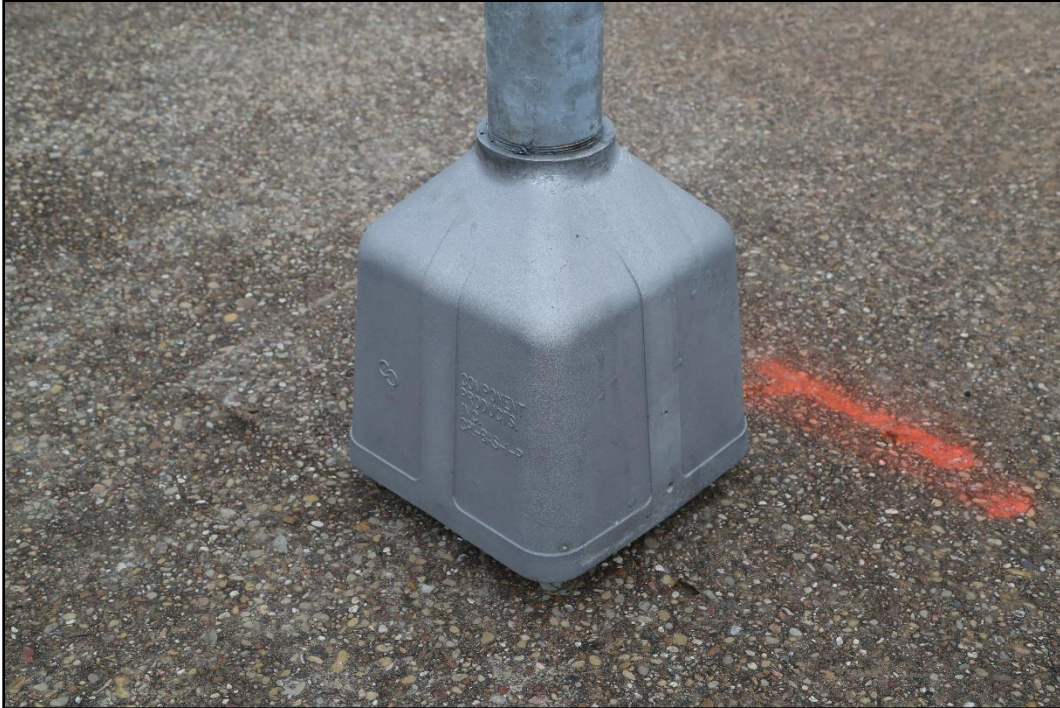
Figure 4.11. MUTCD Standard Pedestrian Signal Base Prior to Crash Test 617891-01-2.
