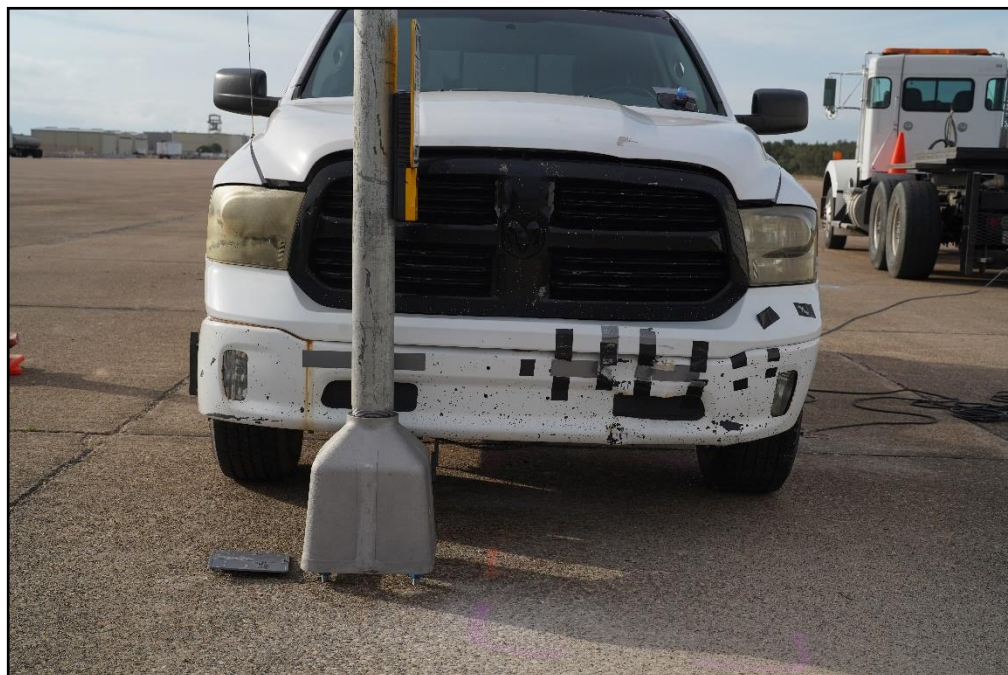
Figure 9.2. MUTCD Standard Pedestrian Signal /Test Vehicle Impact Location 617891-01-3.
