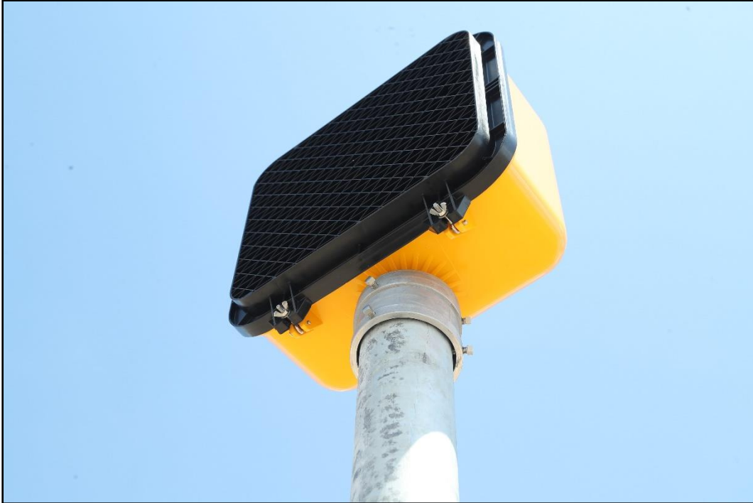
Figure 4.6. MUTCD Standard Pedestrian Signal Signal Head Prior to Crash Test 617891-01-1.
