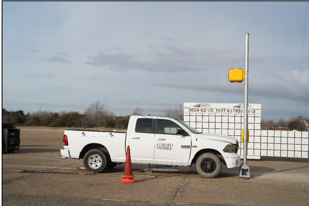
Figure 9.1. MUTCD Standard Pedestrian Signal /Test Vehicle Geometrics for Test 617891-01-3.
