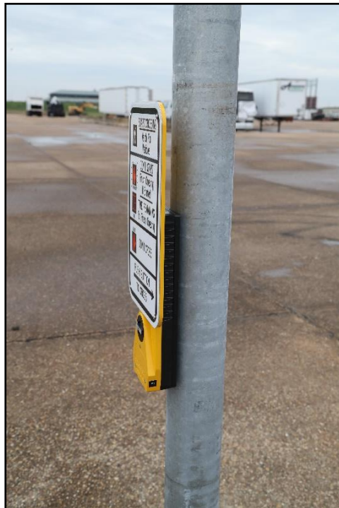
Figure 4.14. MUTCD Standard Pedestrian Signal with Audible Button Prior to Crash Test 617891-01-2.
