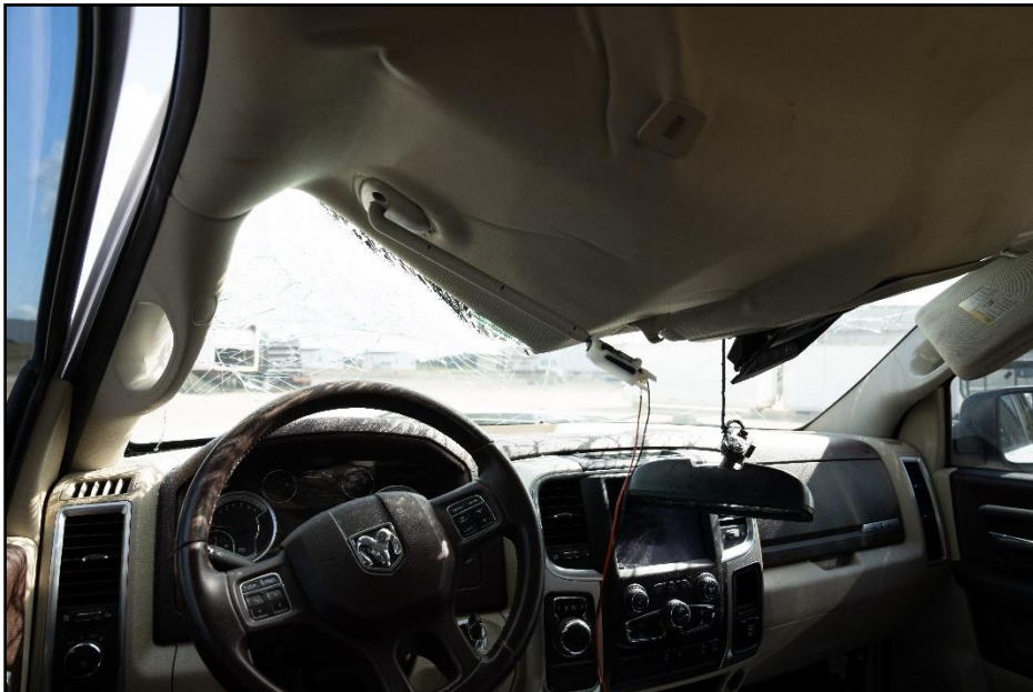
Figure 7.10. Upper Interior of Test Vehicle after Test 617891-01-1.
