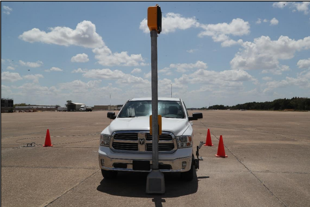
Figure 7.2. MUTCD Standard Pedestrian Signal /Test Vehicle Impact Location 617891-01-1.
