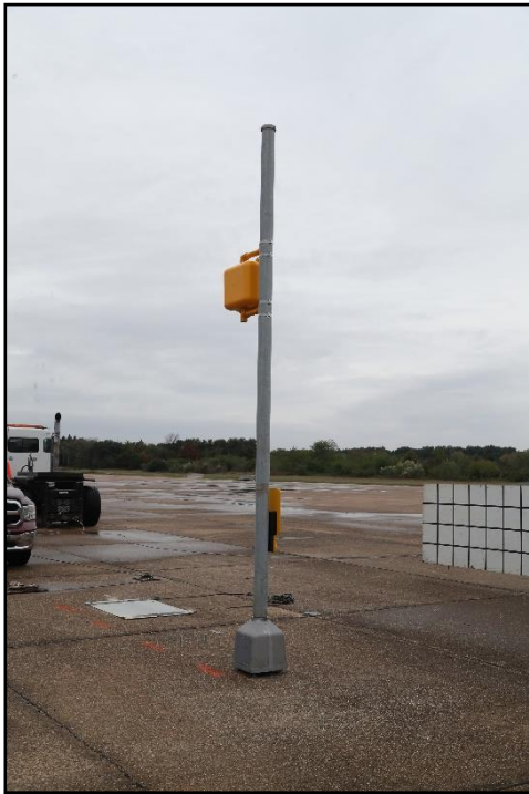
Figure 4.10. Oblique View of the MUTCD Standard Pedestrian Signal Prior to Crash Test 617891-01-2.
