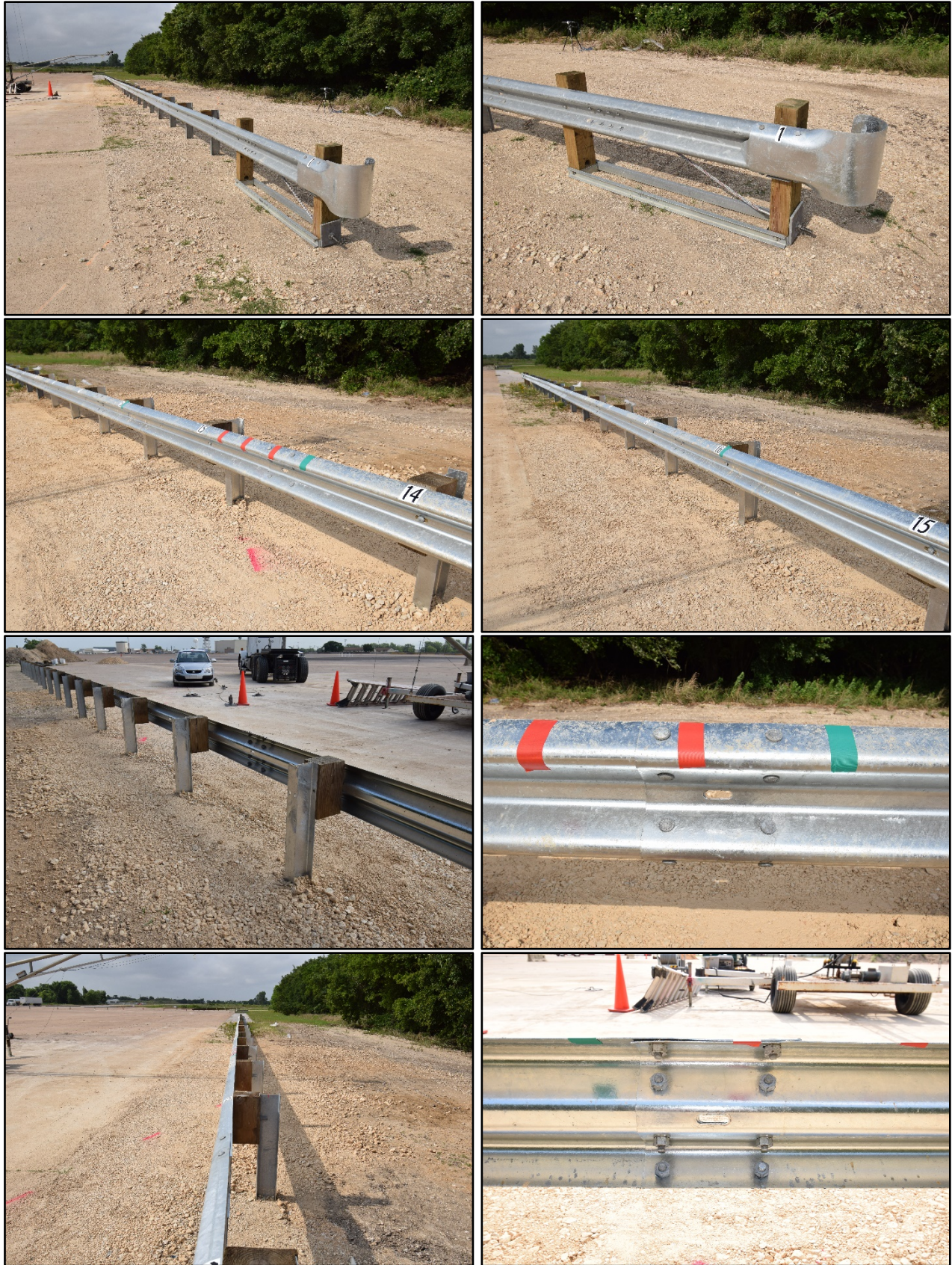
Figure 2.2. W-Beam Guiderail over Underground Structure prior to Testing.
