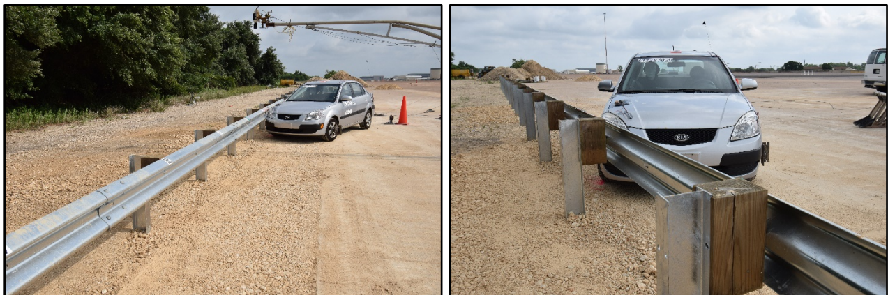
Figure 5.1. Guiderail/Test Vehicle Geometrics for Test No. 612281-02-1.
