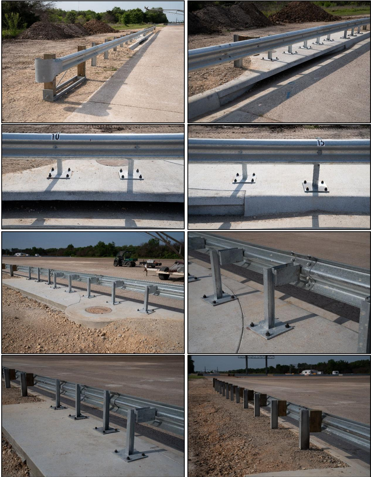
**Figure 4.2. W-Beam Guardrail with Modified Special Steel Posts for Concrete Structure Mount prior to Testing.**
