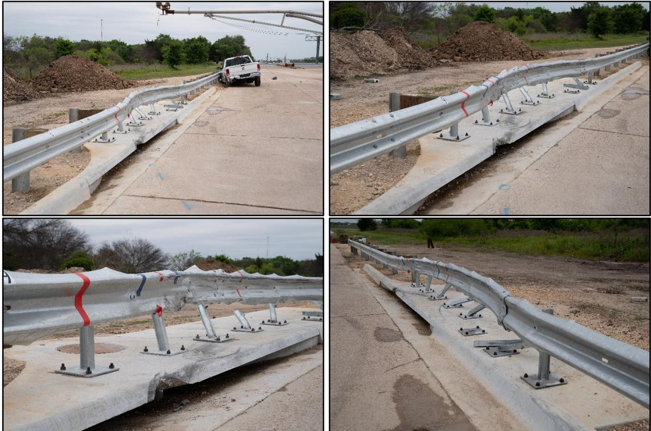
**Figure 7.3. Guardrail after Test No. 611971-01-1.**
