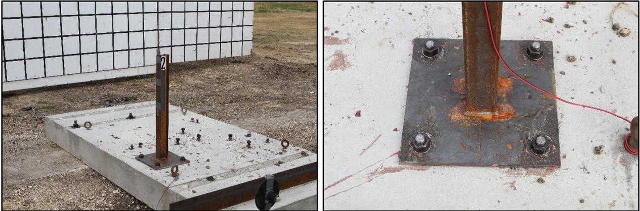
**Figure 3.8. Post before Test No. 611971-01 P2.**
