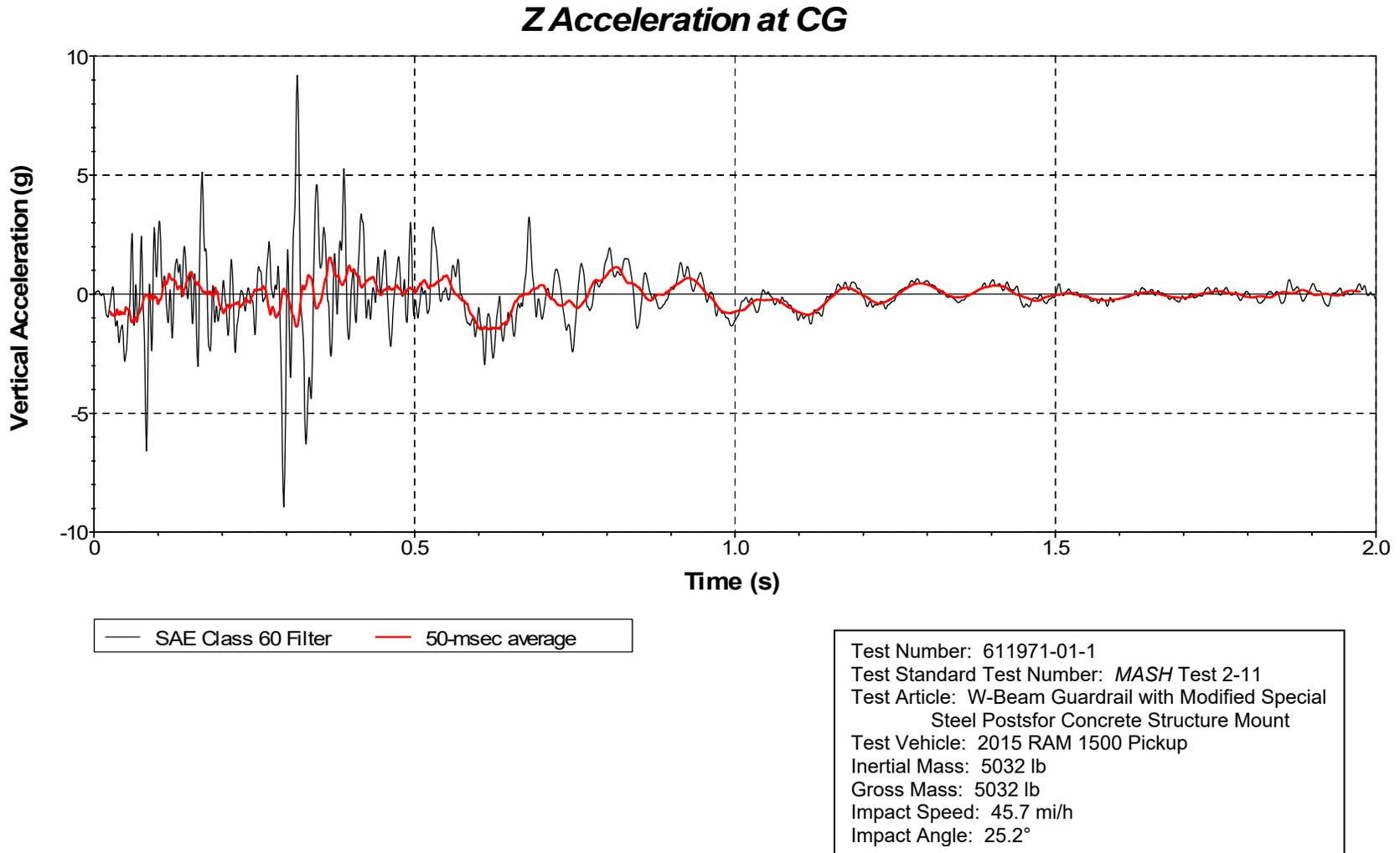
**Figure G.6. Vehicle Vertical Accelerometer Trace for Test No. 611971-01-1 (Accelerometer Located at Center of Gravity).**
