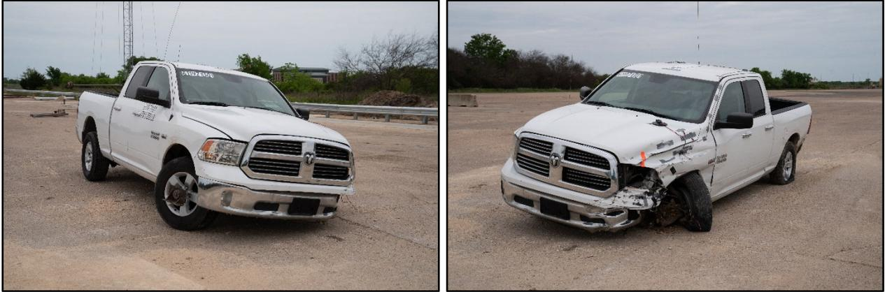
**Figure 7.5. Test Vehicle after Test No. 611971-01-1.**
