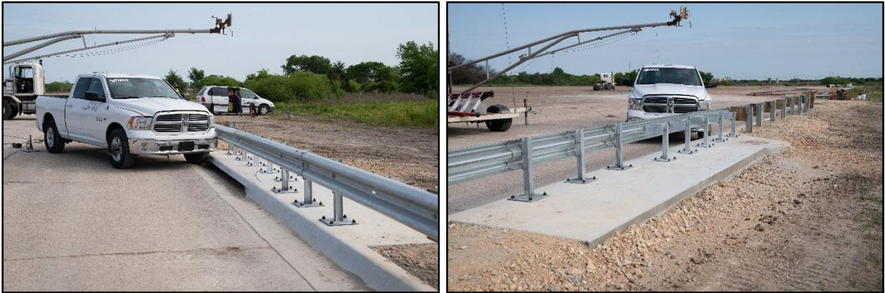
Figure 7.1. Guardrail/Test Vehicle Geometrics for Test No. 611971-01-1.
