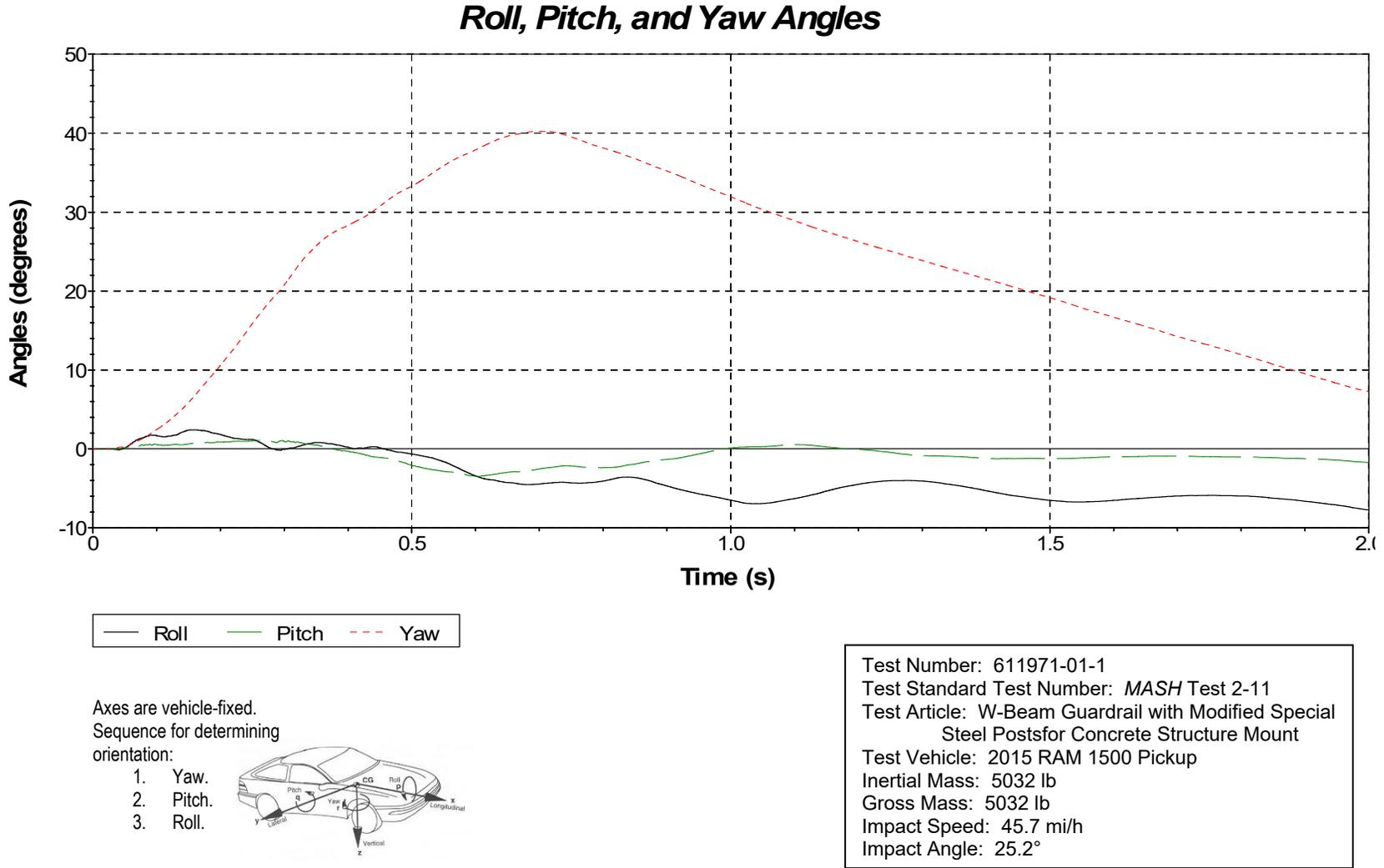
Figure G.3. Vehicle Angular Displacements for Test No. 611971-01-1.
