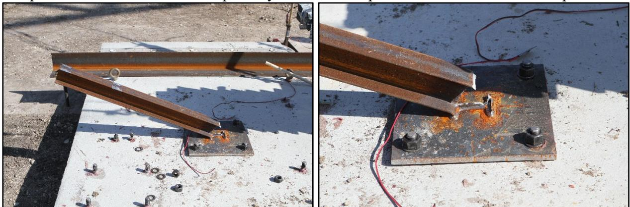
**Figure 3.15. Post after Test No. 611971-01 P5.**
