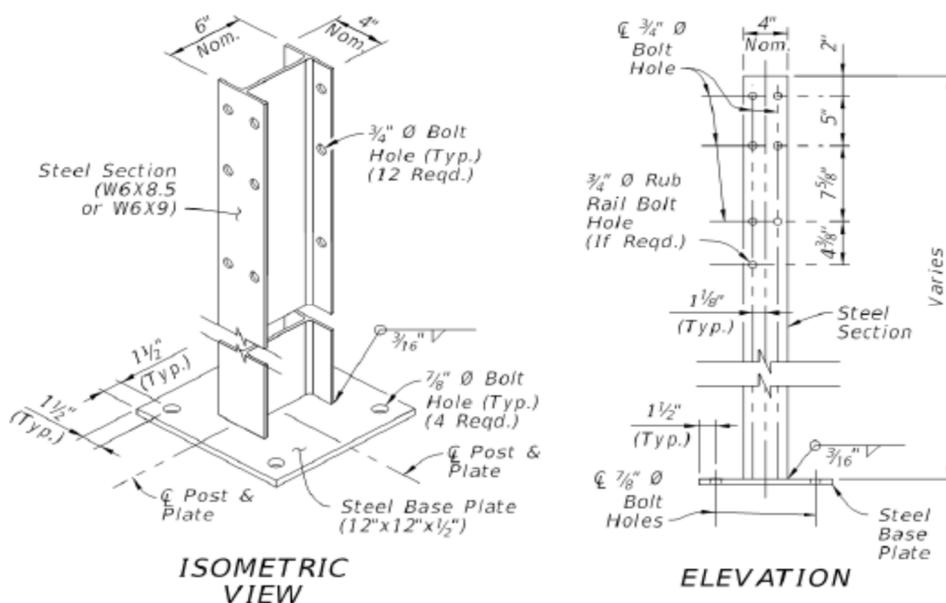
**Figure 2.1. Modified Special Steel Posts for Concrete Structure Mount.**
