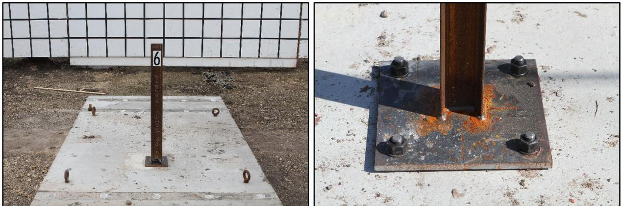
**Figure 3.14. Post before Test No. 611971-01 P5.**
