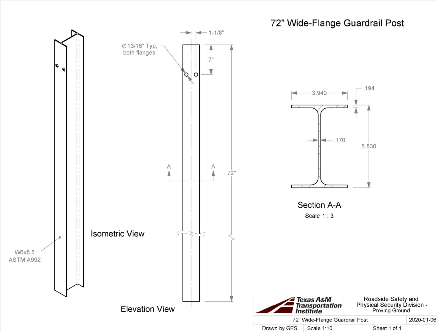
T:\Drafting Department\Solidworks\Standard Parts\Guardrail Parts and Subs\Guardrail Drawings\Post, 72" Wide Flange Guardrail
