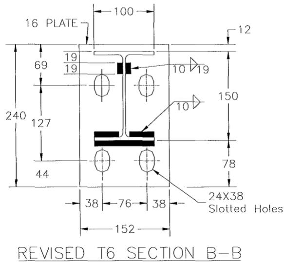
**Figure 2.9. Slotted Steel Fracture Post (Buth, Williams, Bligh, & Menges, 1999)**
