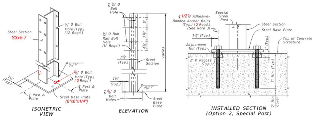
**Figure 2.8. Optimized FDOT Modified Special Steel Posts for Concrete Structure Mount (Florida Department of Transportation, 2017- 2018)**
