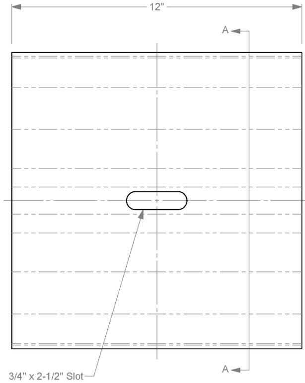
**1a.** Back-up Plate is made of 12 gauge material. See W-beam Guardrail drawing for all dimensions and material specs not shown here.
