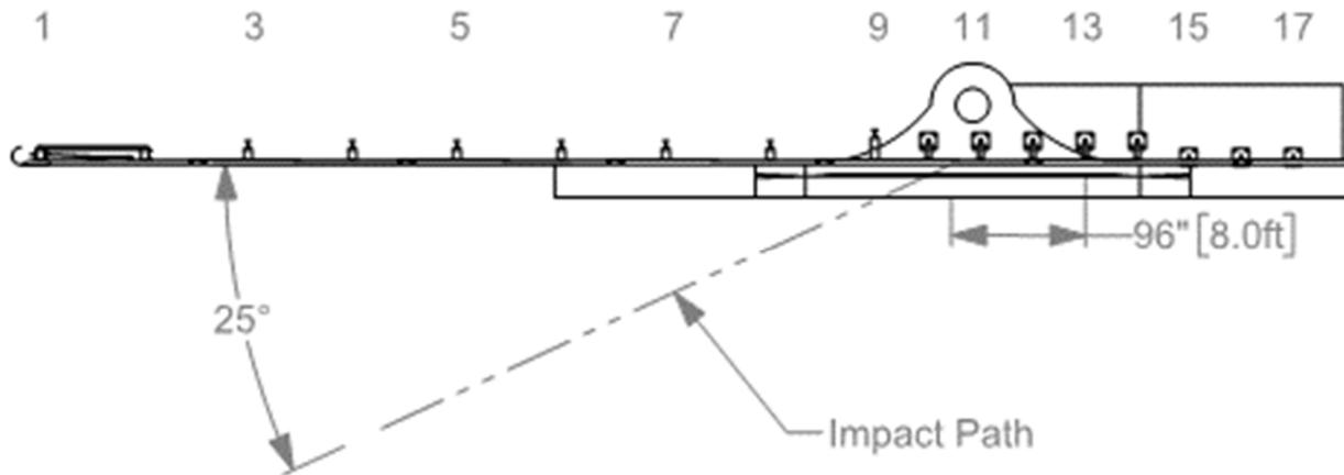
**Figure 5.1. Target CIP for *MASH* Test 2-11 on W-Beam Guardrail with Modified Special Steel Posts for Concrete Structure Mount.**
