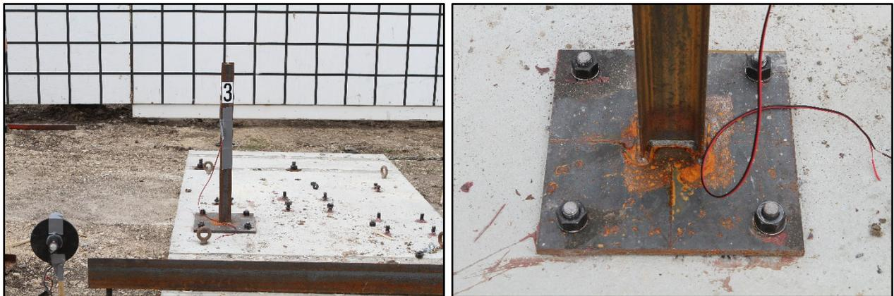
Figure 3.10. Post before Test No. 611971-01 P3.
