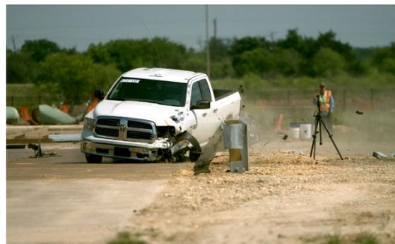
**Figure G.1. Sequential Photographs for Test No. 611971-01-1 (Overhead and Frontal Views) (Continued).**
