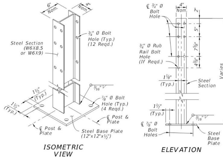
**Figure 2.5. FDOT Modified Special Steel Posts for Concrete Structure Mount (2)**
