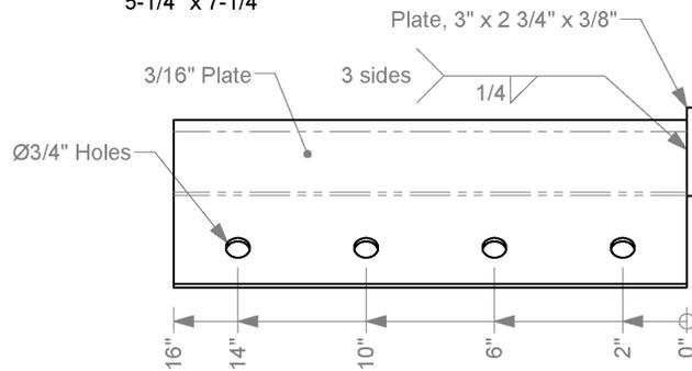
**Guardrail Anchor Bracket**
