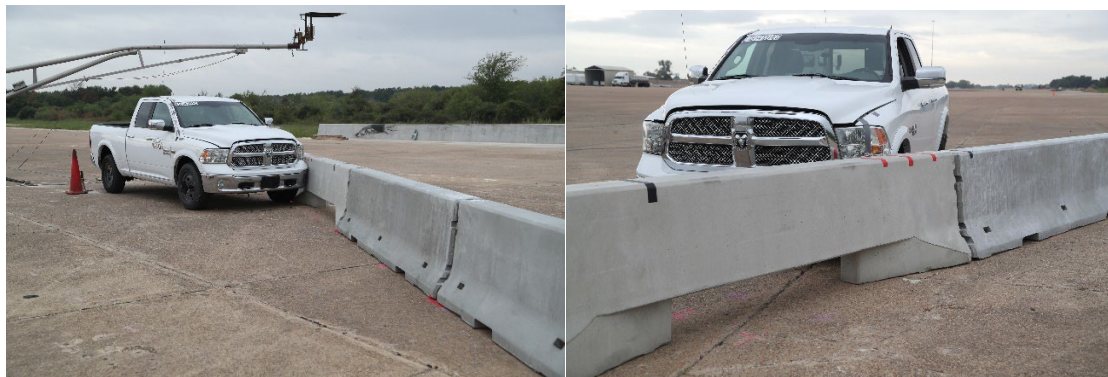
Figure 9 – Photos of MASH Test 3-11 Before Crash Test
