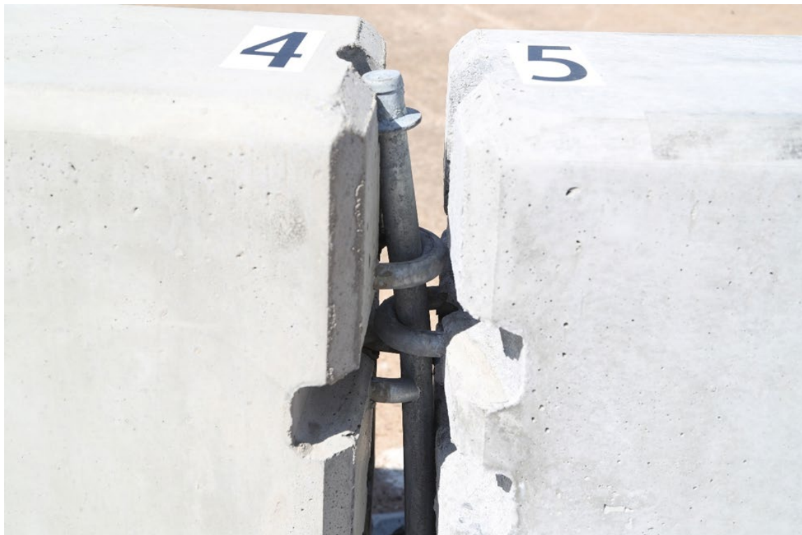
Figure 11 – Photos of Connection Between Barriers 4 & 4
