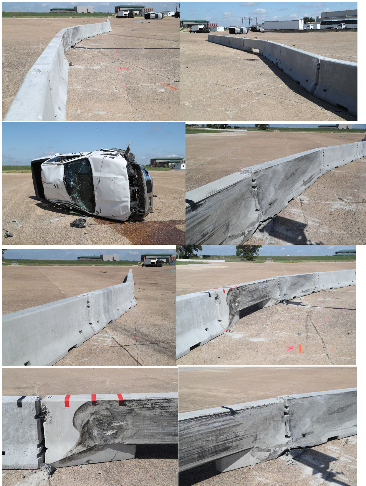
Figure 10 – Photos of MASH Test 3-11 After Crash Test
