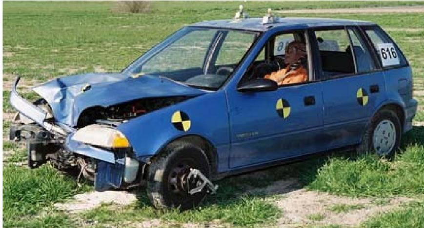
**Figure 2.8. Post-Test Image of Vehicle Damage (Second Test) (5)**
