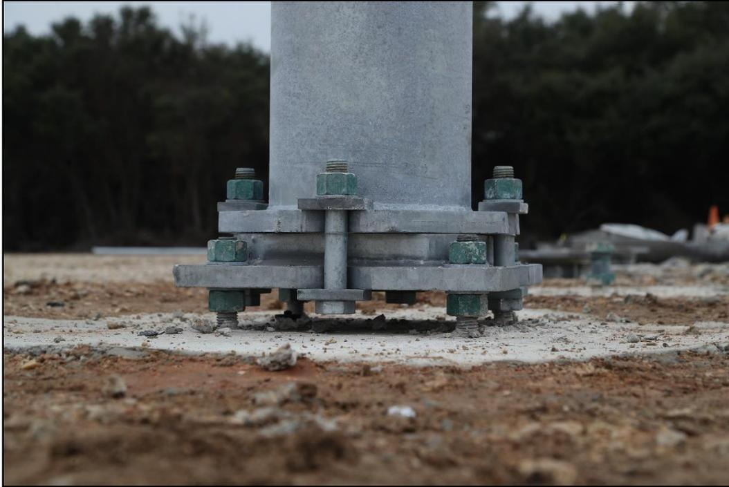
**Figure 4.9. Closeup of the Base for the Four Bolt Slip Base Support for Luminaire Poles Prior to Testing 618911-01-2.**
