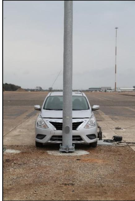
**Figure 8.1. Four Bolt Slip Base Support for Luminaire Poles/Test Vehicle Geometrics for Test 618911-01-2.**
