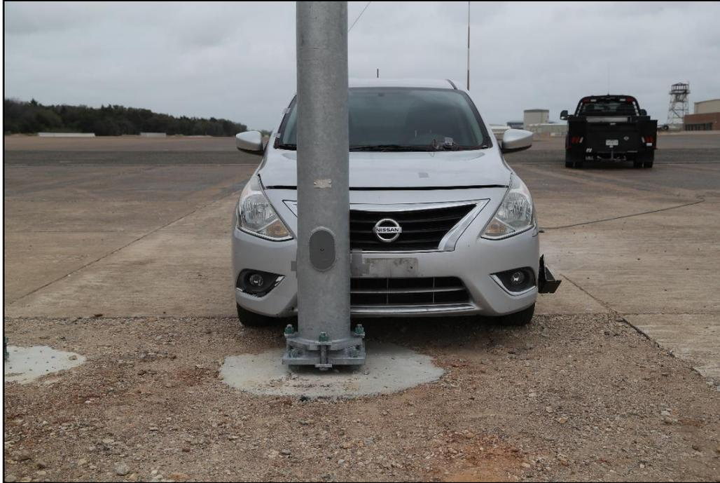
**Figure 9.1. Four Bolt Slip Base Support for Luminaire Poles/Test Vehicle Geometrics for Test 618911-01-3.**
