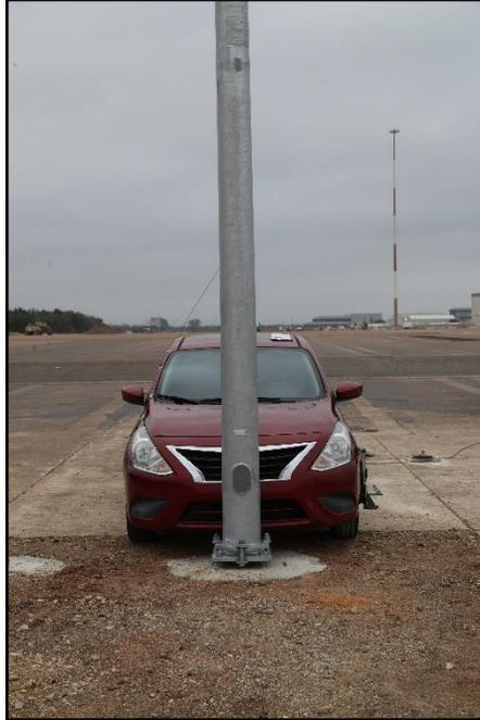
**Figure 7.1. Four Bolt Slip Base Support for Luminaire Poles/Test Vehicle Geometrics for Test 618911-01-1.**
