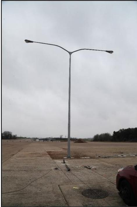
**Figure 4.2. Four Bolt Slip Base Support for Luminaire Poles Prior to Testing 618911-01-1.**
