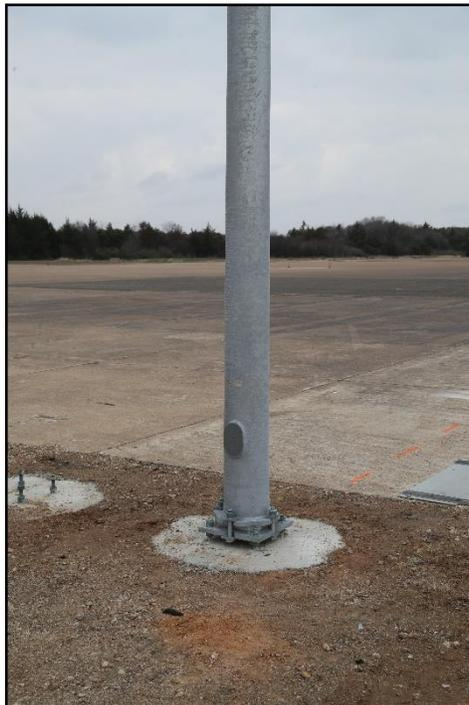
**Figure 4.10. Non-Impact Side of Four Bolt Slip Base Support for Luminaire Poles Prior to Testing 618911-01-2.**
