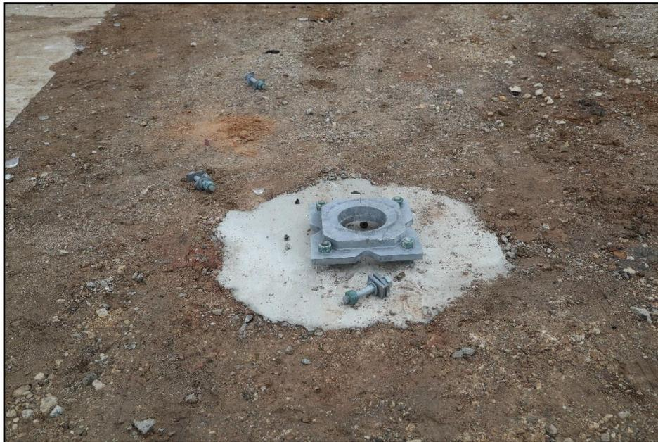
**Figure 7.5. Four Bolt Slip Base Support for Luminaire Poles at Impact Location after Test 618911-01-1.**
