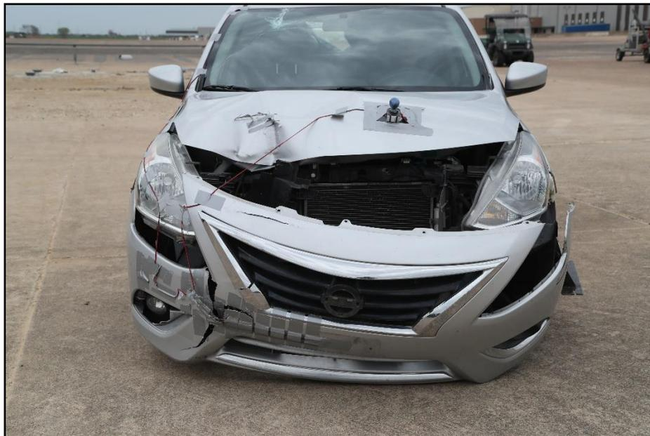
**Figure 9.7. Front of Test Vehicle after Test 618911-01-3.**
