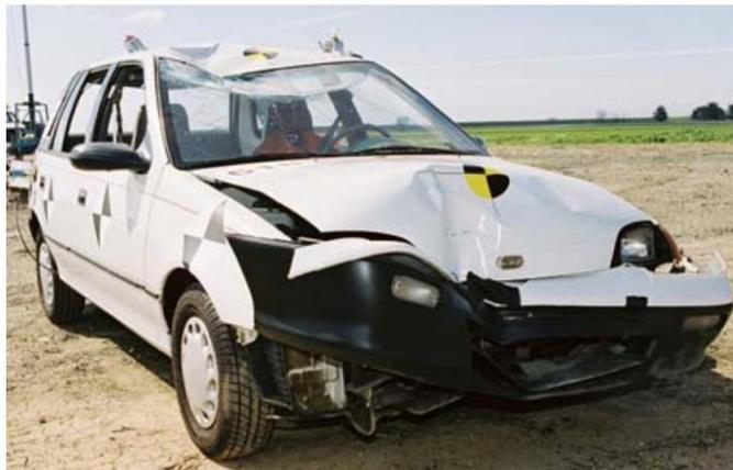
**Figure 2.7. Post-Test Image of Vehicle Damage (First Test) (5)**
