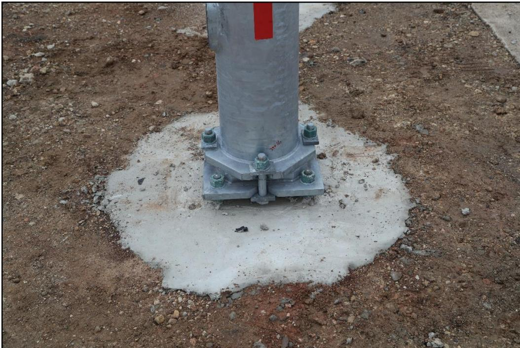
**Figure 4.5. Base and Footer of the Four Bolt Slip Base Support for Luminaire Poles Prior to Testing 618911-01-1.**
