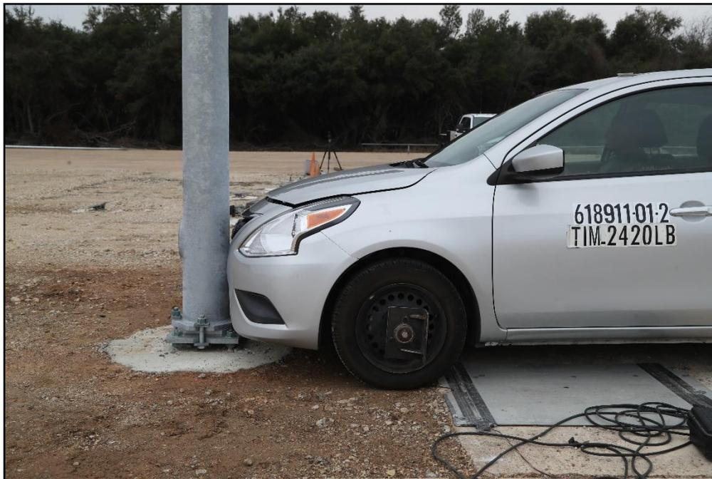
**Figure 9.2. Four Bolt Slip Base Support for Luminaire Poles/Test Vehicle Impact Location 618911-01-3.**
