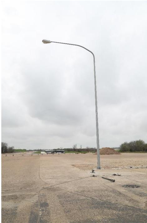
**Figure 4.12. Four Bolt Slip Base Support for Luminaire Poles Prior to Testing 618911-01-3.**
