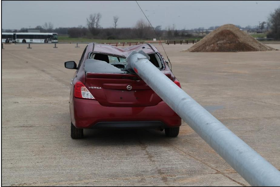
**Figure 7.8. Rear Impact Side of Test Vehicle after Test 618911-01-1.**
