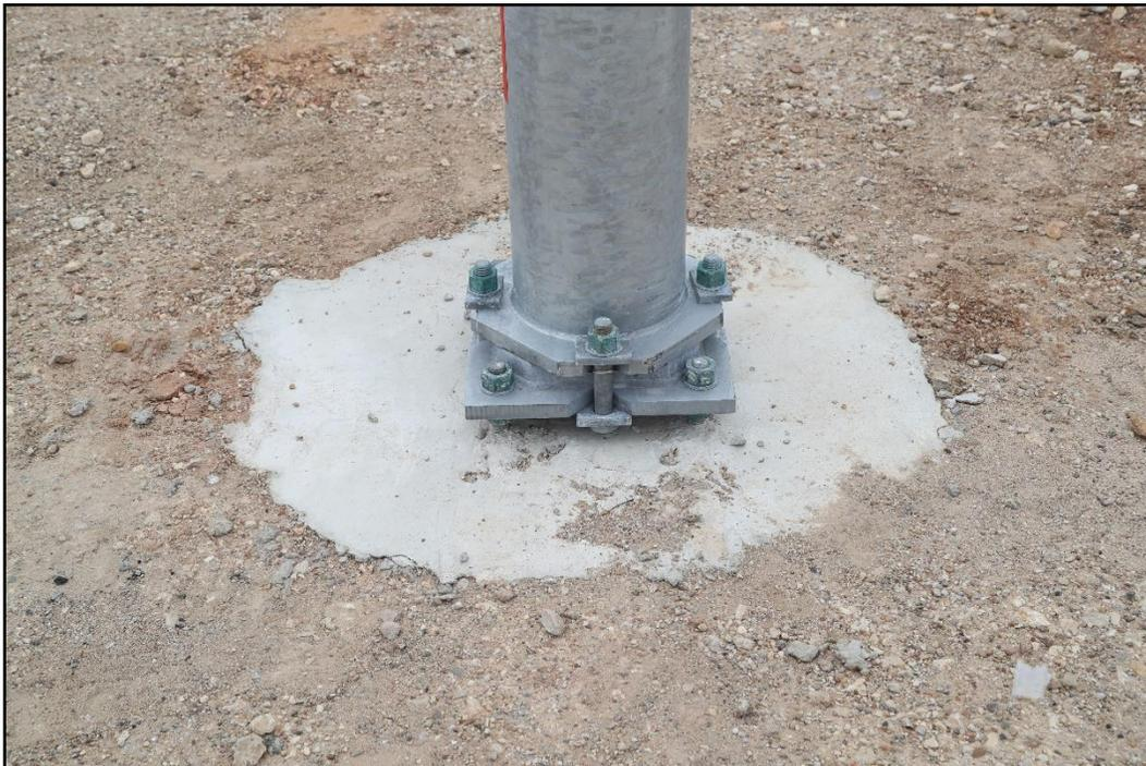
**Figure 4.13. Base and Footer of the Four Bolt Slip Base Support for Luminaire Poles Prior to Testing 618911-01-1.**
