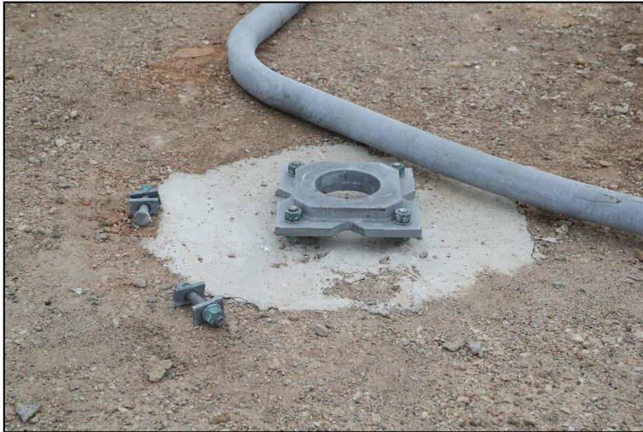
**Figure 9.5. Four Bolt Slip Base Support for Luminaire Poles at Impact Location after Test 618911-01-3.**
