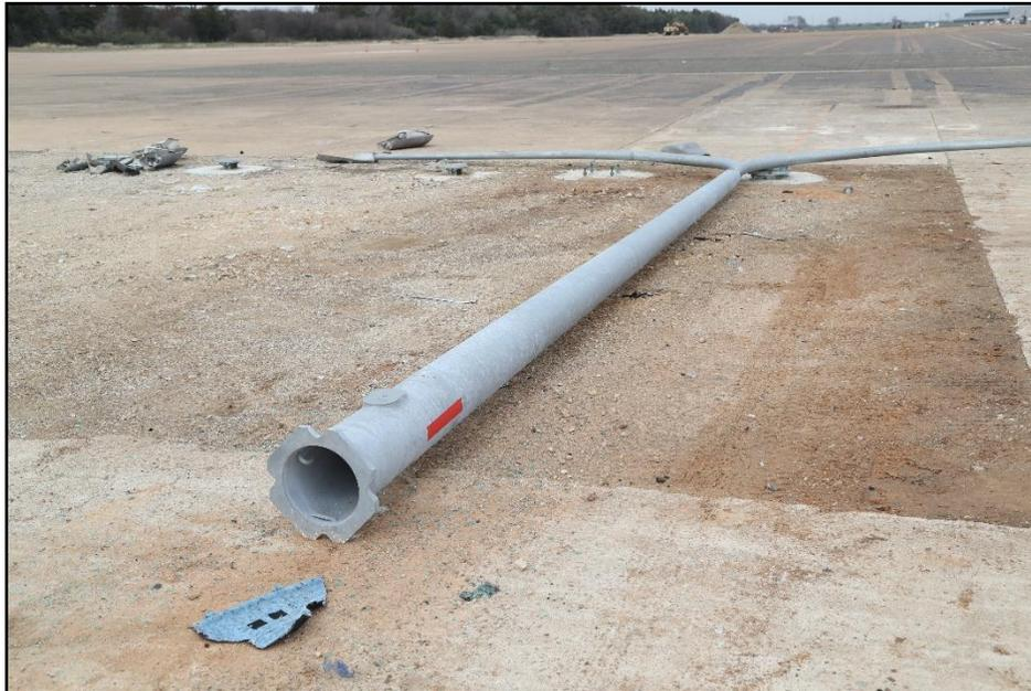
**Figure 8.5. Test Article at Impact Location after Test 618911-01-2.**
