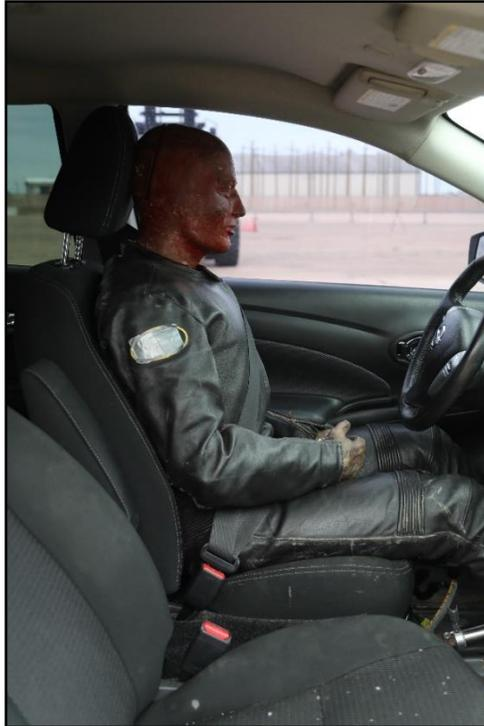
**Figure 9.10. Interior of Test Vehicle on Impact Side after Test 618911-01-3.**
