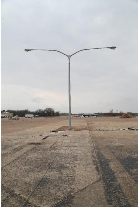
**Figure 4.7. Four Bolt Slip Base Support for Luminaire Poles Prior to Testing 618911-01-2.**
