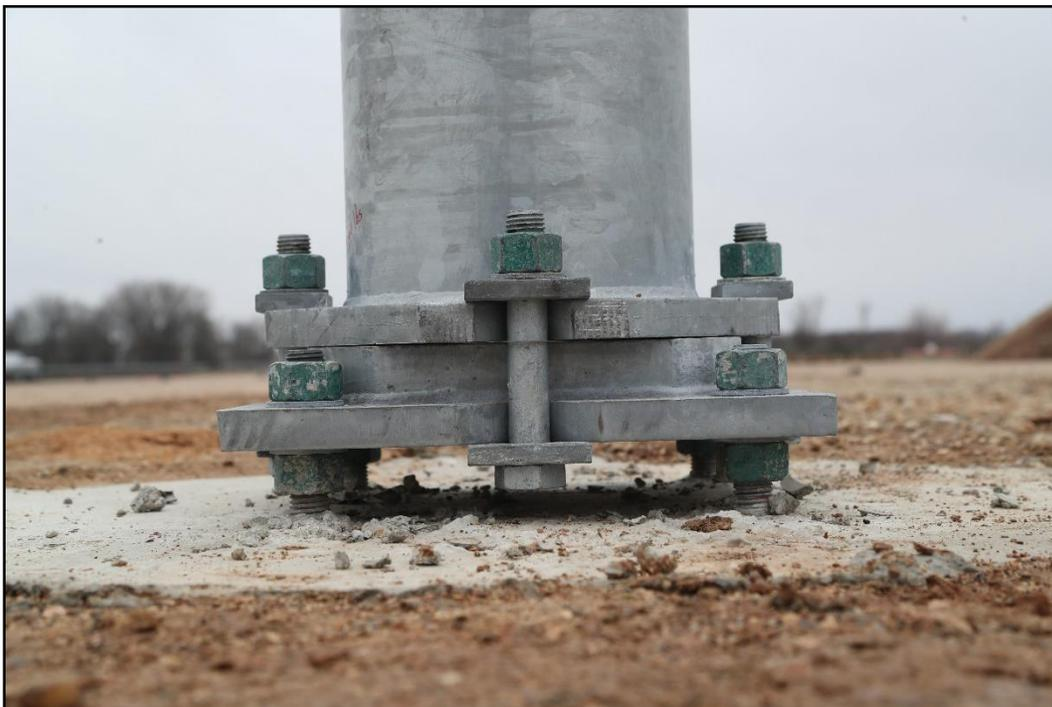
**Figure 4.3. Closeup of the Base for the Four Bolt Slip Base Support for Luminaire Poles Prior to Testing 618911-01-1.**
