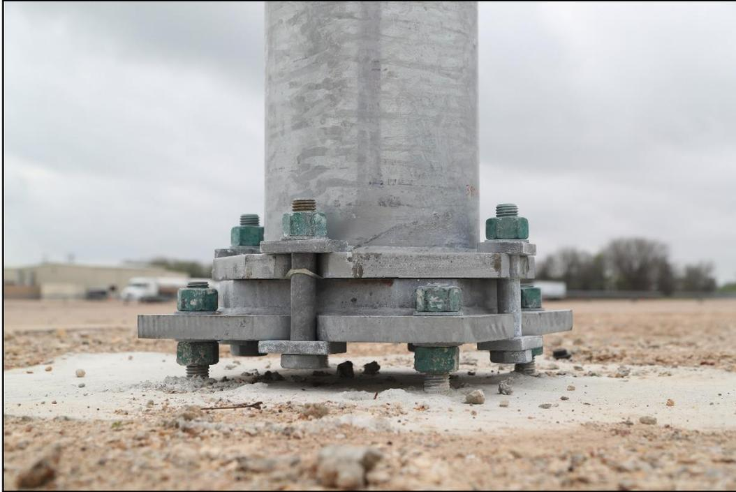
**Figure 4.14. Closeup of the Base for the Four Bolt Slip Base Support for Luminaire Poles Prior to Testing 618911-01-1.**
