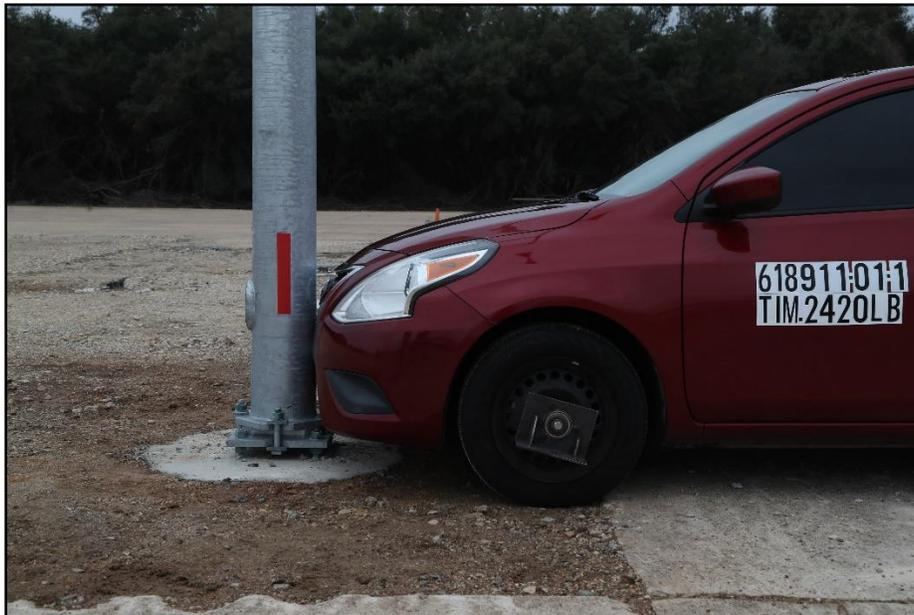
**Figure 7.2. Four Bolt Slip Base Support for Luminaire Poles/Test Vehicle Impact Location 618911-01-1.**
