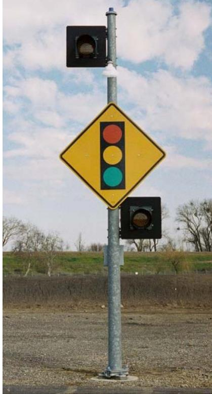
**Figure 2.6. Pre-Test Assembly of the Warning Sign with Flashing Beacons (5)**
