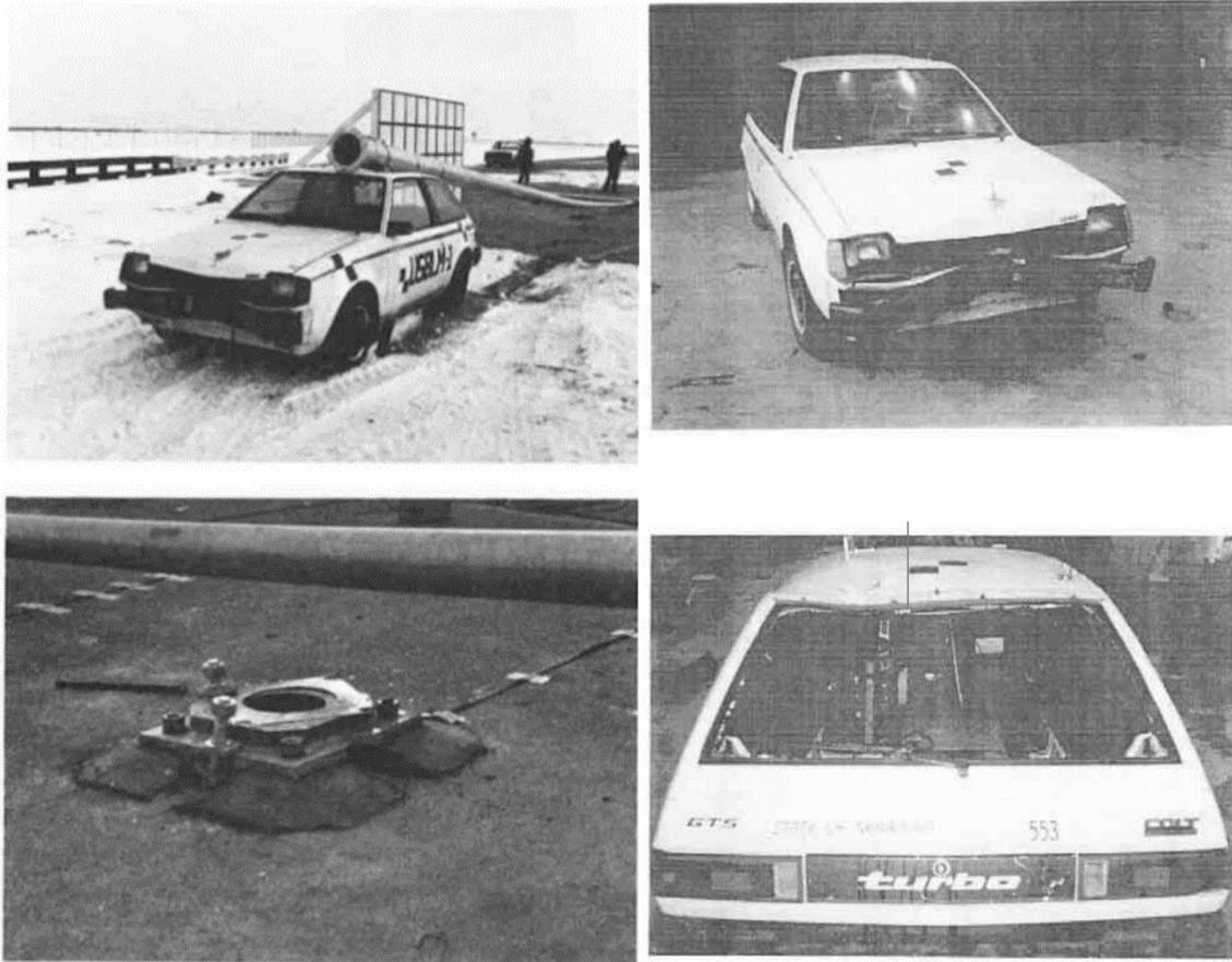
**Figure 2.3. Post-Test images of Vehicle, Luminaire, and Slip base (3)**
