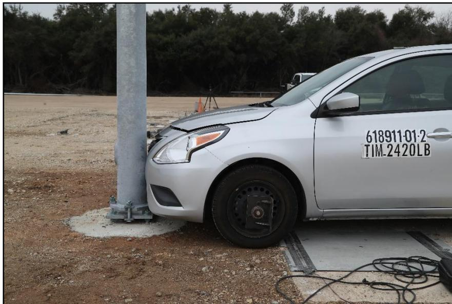
**Figure 8.2. Four Bolt Slip Base Support for Luminaire Poles/Test Vehicle Impact Location 618911-01-2.**
