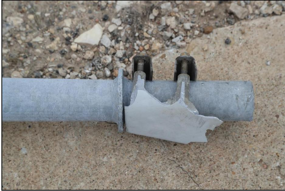
**Figure 9.6. Closeup of a Mast Arm End for Four Bolt Slip Base for Luminaire Supports after Test 618911-01-3.**
