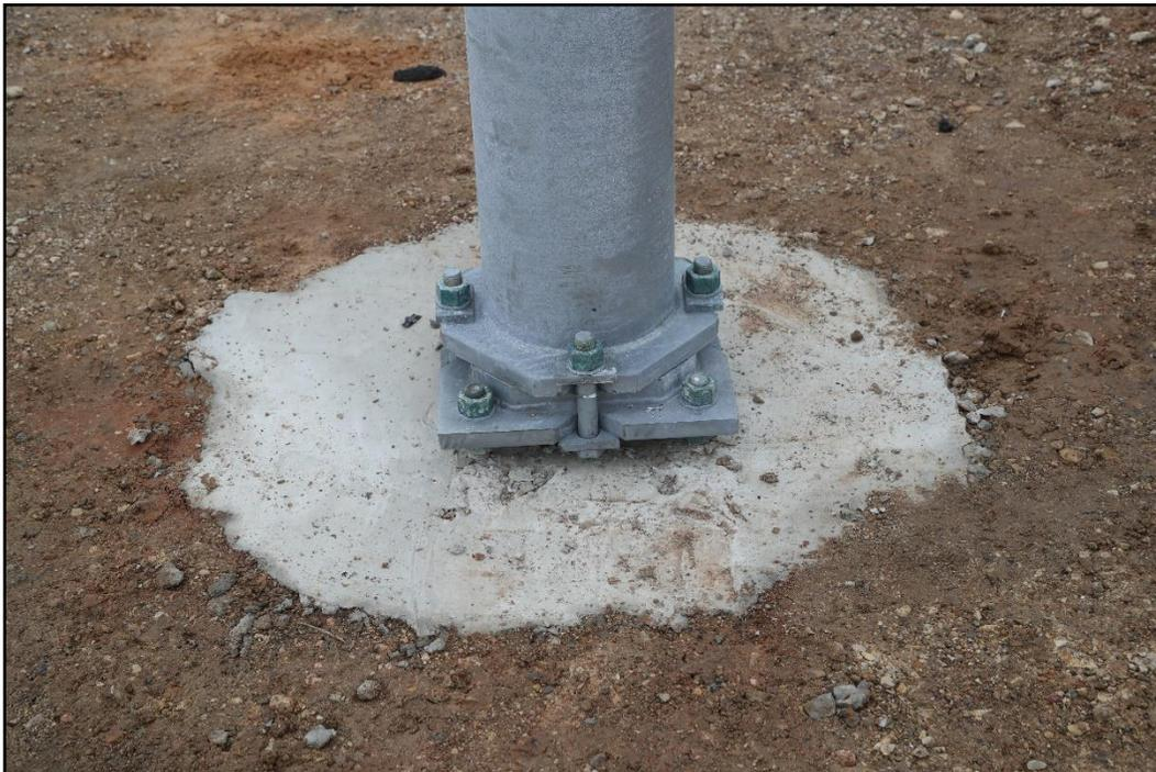
**Figure 4.8. Base and Footer of the Four Bolt Slip Base Support for Luminaire Poles Prior to Testing 618911-01-2.**
