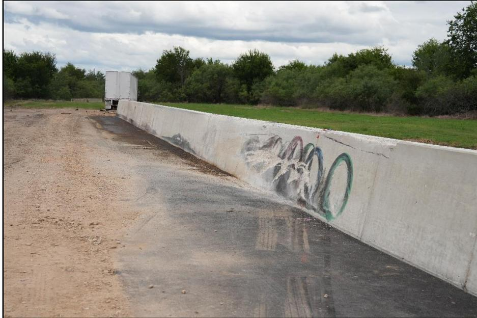
**Figure 6.7. Overall View of TL-5 Concrete Median Barrier with Shallow Embedment after Test 620331-01-1.**
