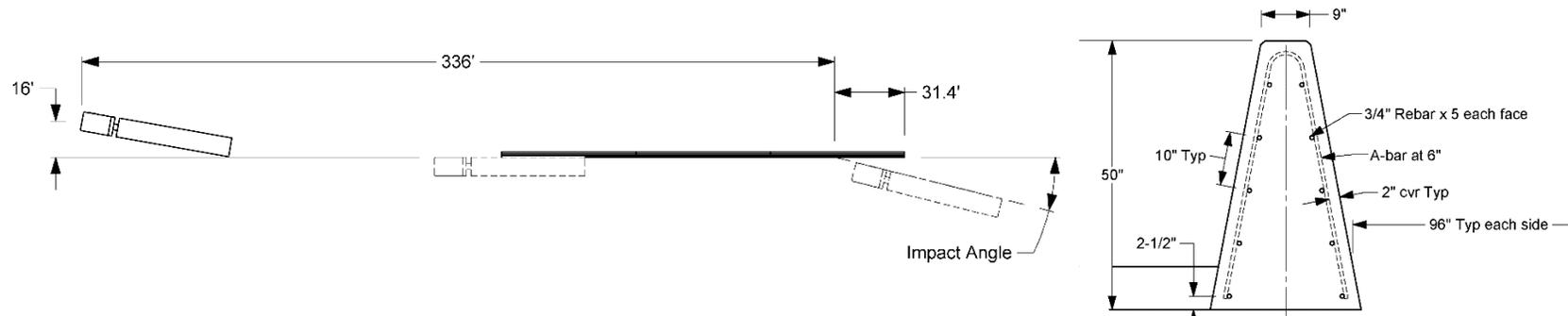
**Figure 6.17. Summary of Results for MASH Test 5-12 on TL-5 Concrete Median Barrier with Shallow Embedment.**
