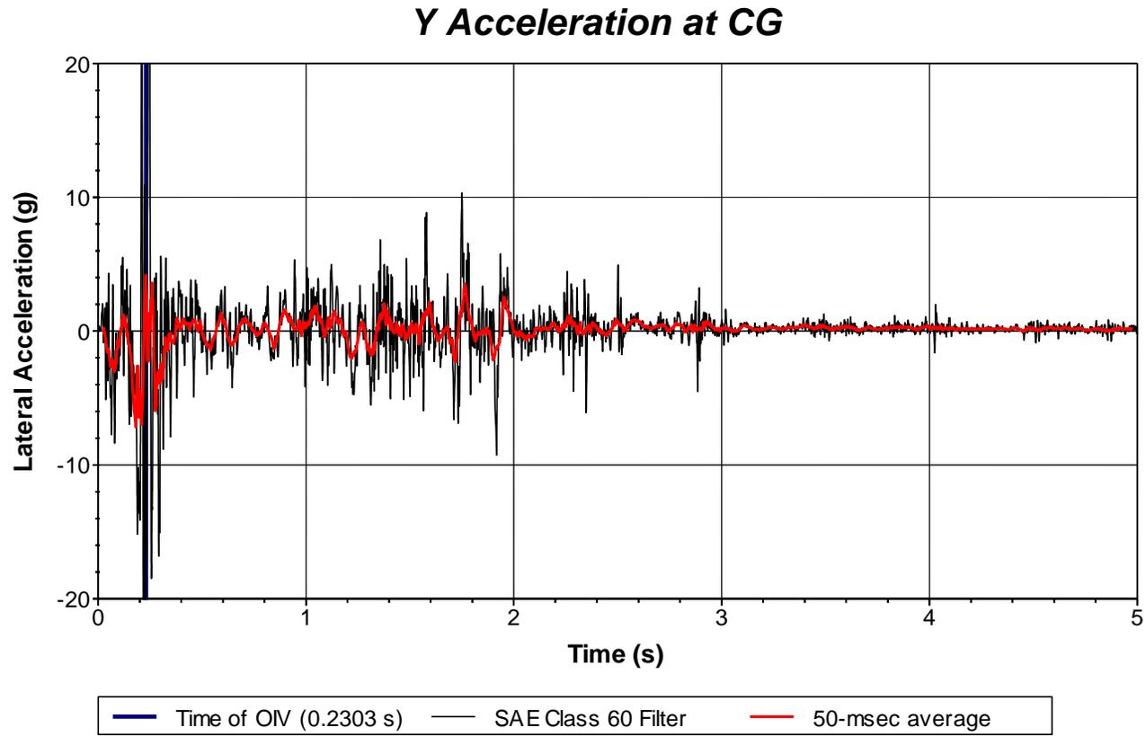
**Figure C.7. Vehicle Lateral Accelerometer Trace for Test 620331-01-1 (Accelerometer Located at Center of Gravity).**
