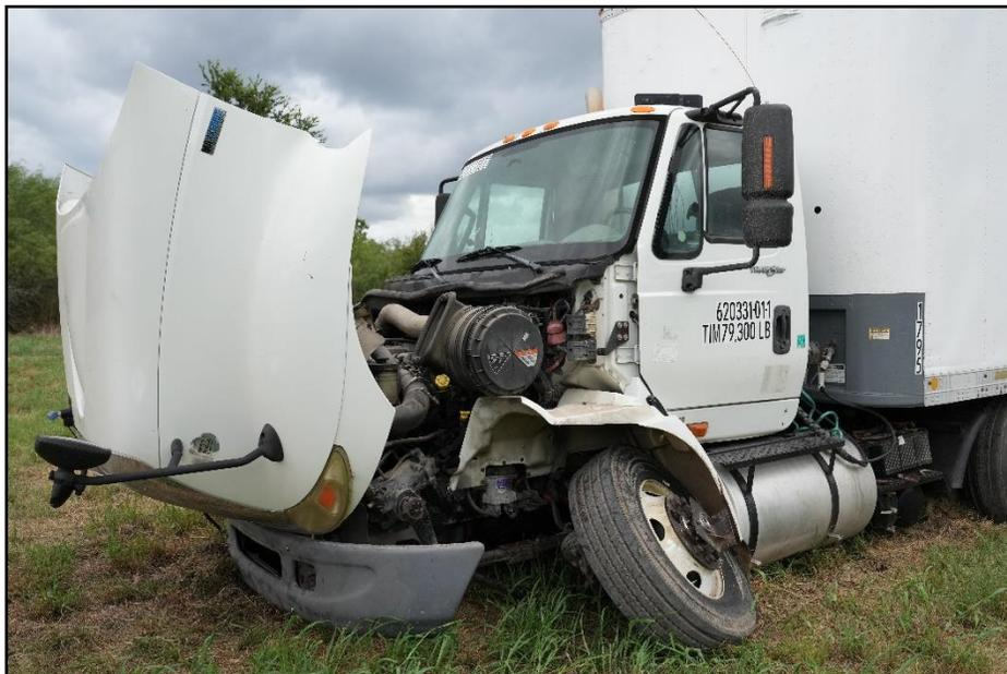
**Figure 6.14. Opposite Impact Side of Test Vehicle after Test 620331-01-1.**
