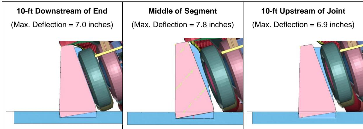
**Figure 2.4. Impact Points Shown on First Segment of the Barrier System.**
