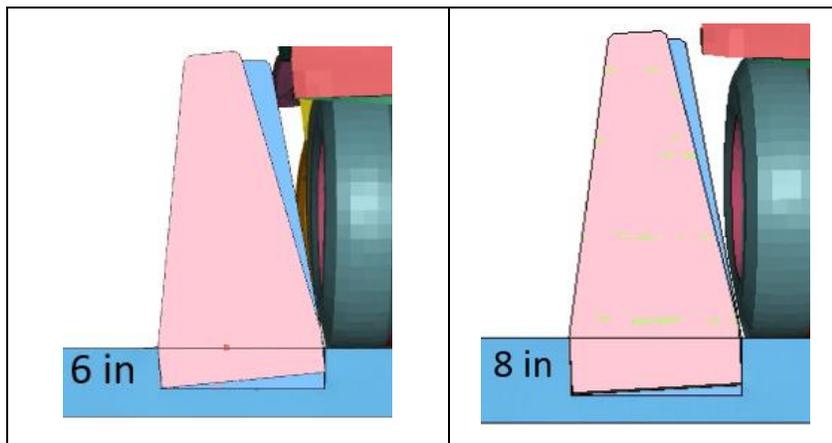
**Figure 2.6. Comparison of Permanent Barrier Deflection of 6-inch and 8-inch Embedment Depths.**
