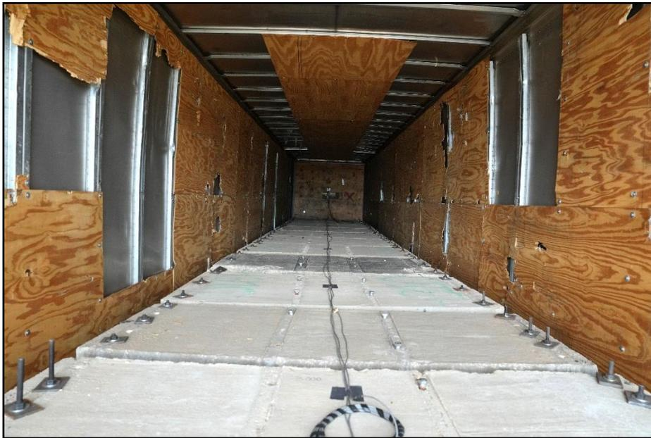
**Figure 6.16. Trailer Interior of Test Vehicle after Test 620331-01-1.**
