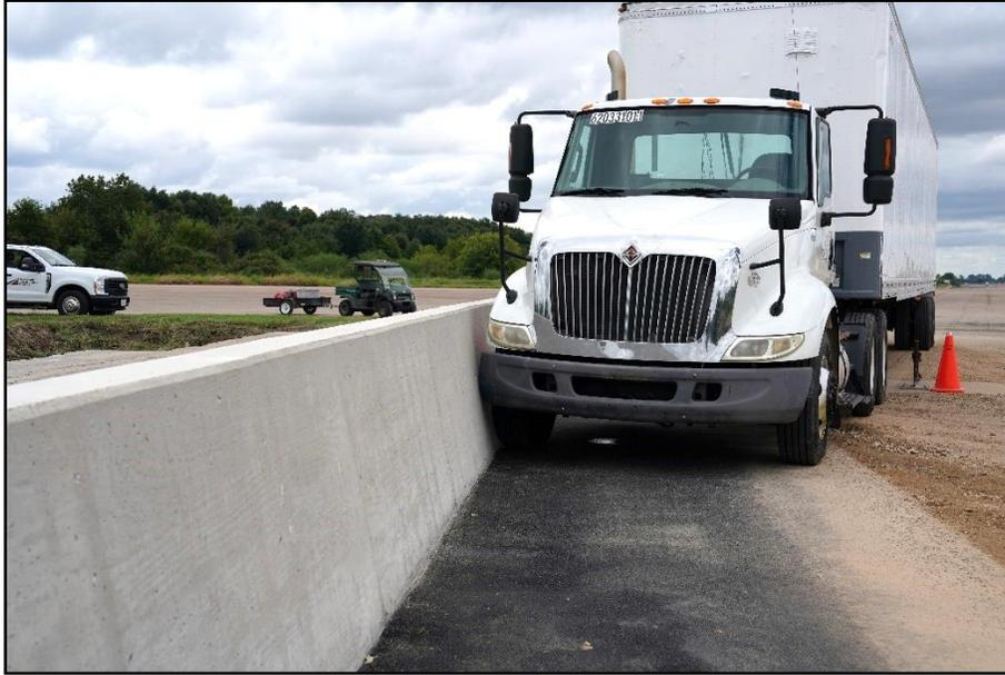
**Figure 6.1. TL-5 Concrete Median Barrier with Shallow Embedment/Test Vehicle Geometrics for Test 620331-01-1.**
