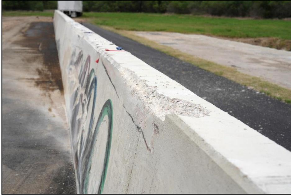
**Figure 6.9. TL-5 Concrete Median Barrier with Shallow Embedment at Impact Location after Test 620331-01-1.**
