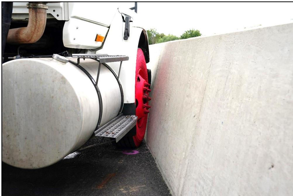
**Figure 6.2. TL-5 Concrete Median Barrier with Shallow Embedment/Test Vehicle Impact Location 620331-01-1.**
