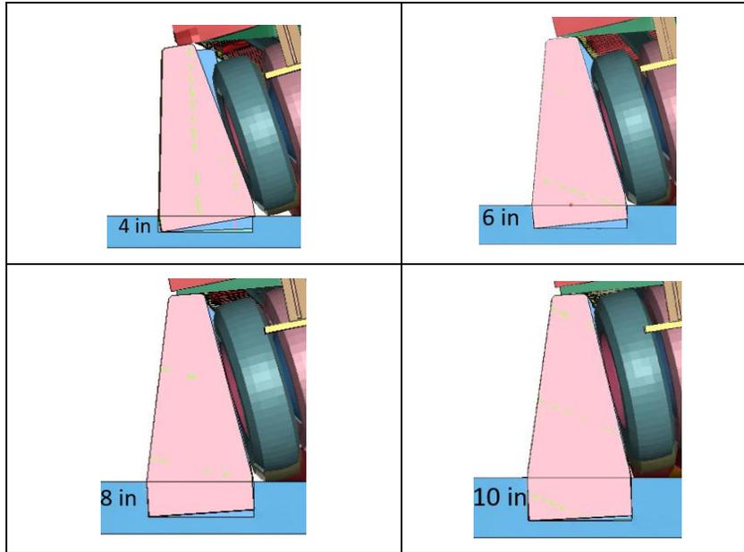
**Figure 2.5. Comparison of Maximum Dynamic Barrier Deflection for Different Embedment Depths.**
