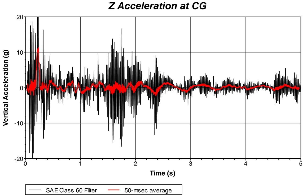
**Figure C.8. Vehicle Vertical Accelerometer Trace for Test 620331-01-1
