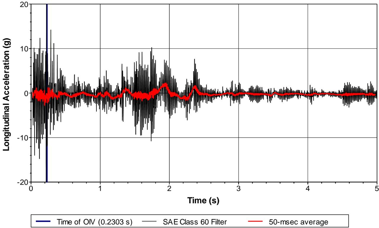
**Figure C.6. Vehicle Longitudinal Accelerometer Trace for Test 620331-01-1 (Accelerometer Located at Center of Gravity).**
