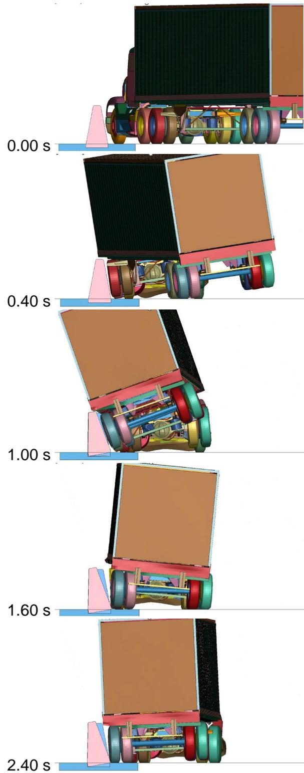
**Figure 2.3. Results of Simulation with Impact at Middle of the Segment.**
