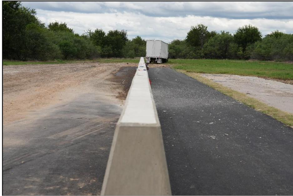
**Figure 6.12. Downstream In-line View of TL-5 Concrete Median Barrier with Shallow Embedment after Test 620331-01-1.**
