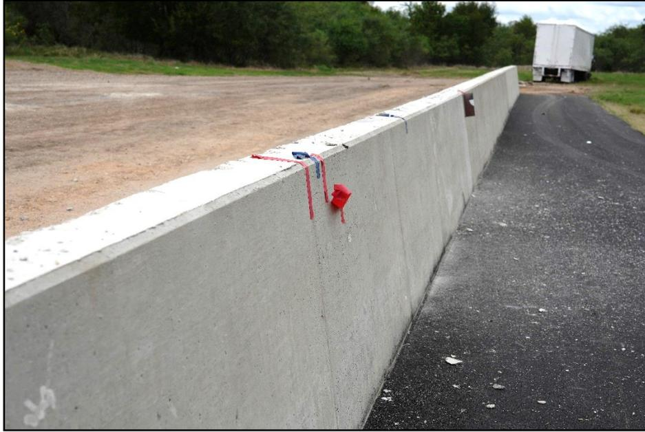
**Figure 6.11. Oblique Downstream Field Side View of TL-5 Concrete Median Barrier with Shallow Embedment at Impact Location after Test 620331-01-1.**
