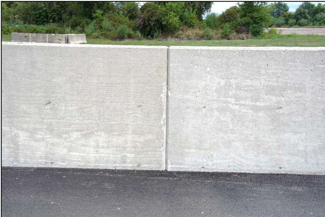
**Figure 3.5. TL-5 Concrete Median Barrier with Shallow Embedment at Unconnected Cold Joint Prior to Testing.**
