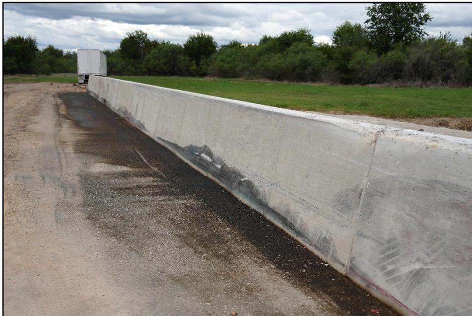
**Figure 6.10. Oblique View of Downstream Damage and Cold Joint of TL-5 Concrete Median Barrier with Shallow Embedment after Test 620331-01-1.**
