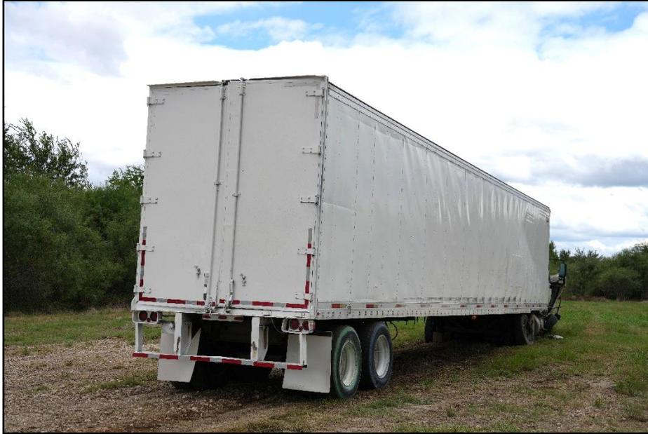
**Figure 6.15. Rear Impact of Test Vehicle after Test 620331-01-1.**
