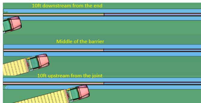
**Figure 2.2. Impact Points Shown on First Segment of the Barrier System.**
