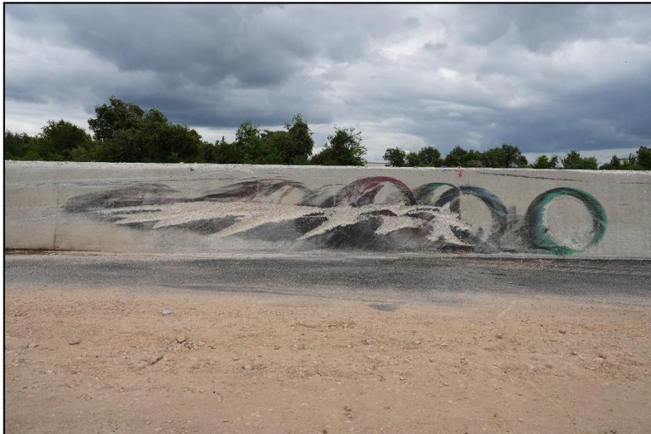
**Figure 6.8. Right Angle View of TL-5 Concrete Median Barrier with Shallow Embedment at Impact Location after Test 620331-01-1.**
