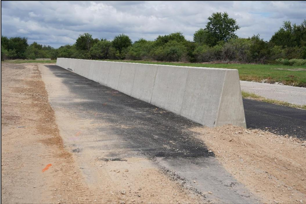
**Figure 3.2. Overall View of the TL-5 Concrete Median Barrier with Shallow Embedment Prior to Testing.**
