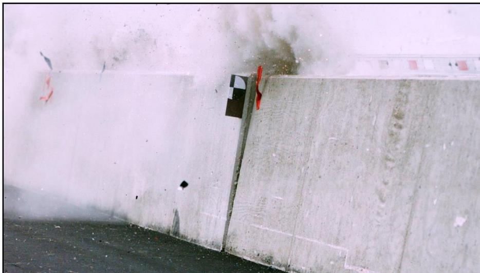
**Figure 6.6. TL-5 Concrete Median Barrier with Shallow Embedment at Maximum Deflection during Test 620331-01-1.**
