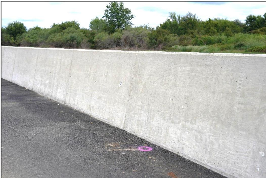
**Figure 3.3. TL-5 Concrete Median Barrier with Shallow Embedment at Impact Location Prior to Testing.**
