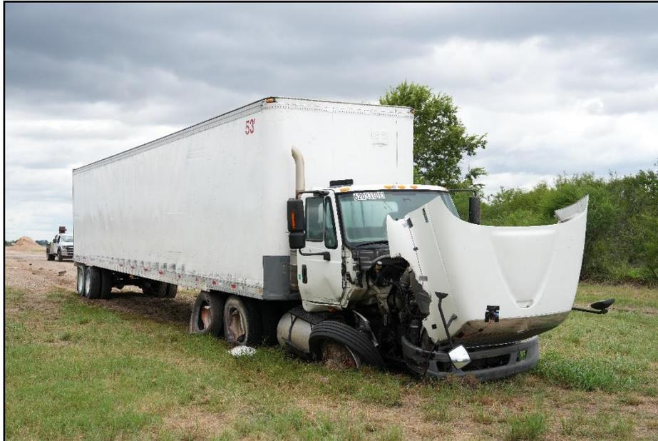
**Figure 6.13. Impact Side of Test Vehicle after Test 620331-01-1.**
