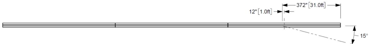
**Figure 4.1. Target CIP for *MASH* TL-5 Test on TL-5 Concrete Median Barrier with Shallow Embedment.**
