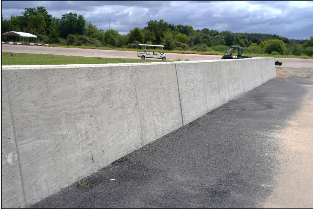
**Figure 3.4. Upstream Oblique View of the TL-5 Concrete Median Barrier with Shallow Embedment Prior to Testing.**
