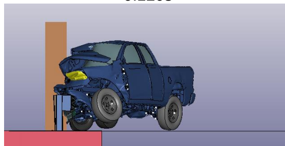
Figure 2.36. MASH Test 3-11 Simulation of Half-Post Large Gap with Fixed Object 4 inch Offset – Downstream View
