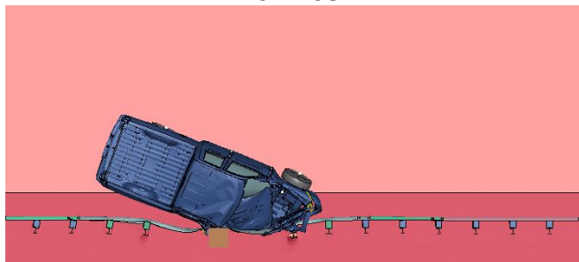
Figure 2.41. MASH Test 3-11 Simulation of Half-Post Large Gap with Fixed Object 8 inch Offset – Overhead View
