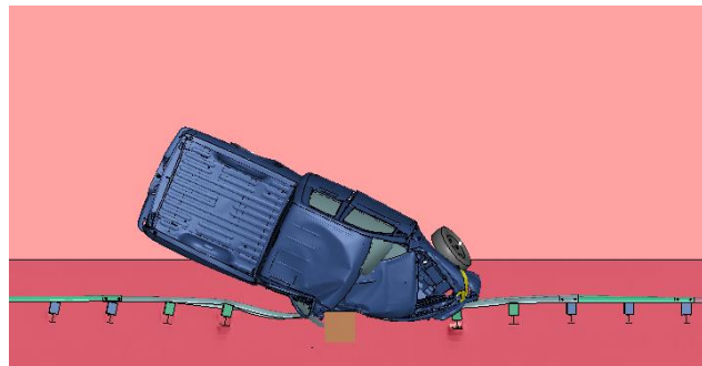
Figure 2.38. MASH Test 3-11 Simulation of Half-Post Large Gap with Fixed Object 6 inch Offset – Overhead View
