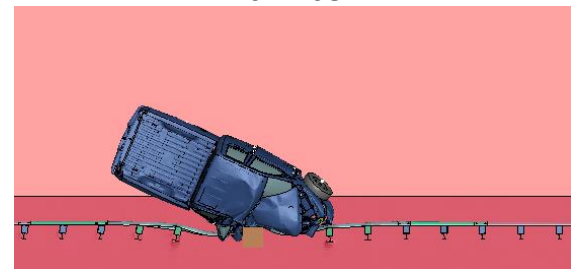
Figure 2.32. MASH Test 3-11 Simulation of Half-Post Large Gap with Fixed Object 2 inch Offset – Overhead View
