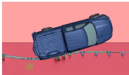
Figure 2.125. MASH Test 3-11 Simulation of Quarter-Post Large Gap with Fixed Object 30 inch Offset 4 feet Upstream Impact Variation – Overhead View
