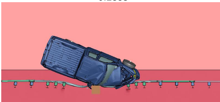
Figure 2.98. MASH Test 3-11 Simulation of Quarter-Post Large Gap with Fixed Object 8 inch Offset – Overhead View
