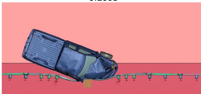
Figure 2.101. MASH Test 3-11 Simulation of Quarter-Post Large Gap with Fixed Object 10 inch Offset – Overhead View
