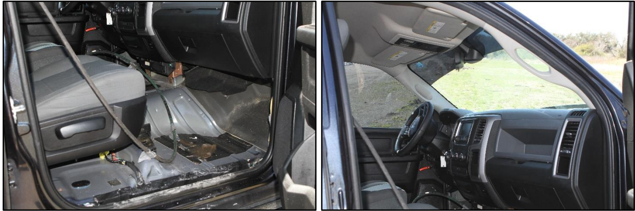
Figure 7.5 Interior of Test Vehicle after Test 614031-01-1.
