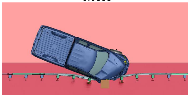
Figure 2.161. MASH Test 3-11 Simulation of Half-Post Small Gap with Fixed Object 12 inch Offset – Overhead View
