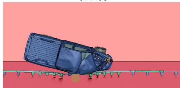
Figure 2.221. MASH Test 3-11 Simulation of Quarter-Post Small Gap with Fixed Object 6 inch Offset – Overhead View
