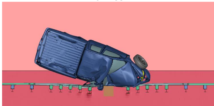
Figure 2.215. MASH Test 3-11 Simulation of Quarter-Post Small Gap with Fixed Object 2 inch Offset – Overhead View
