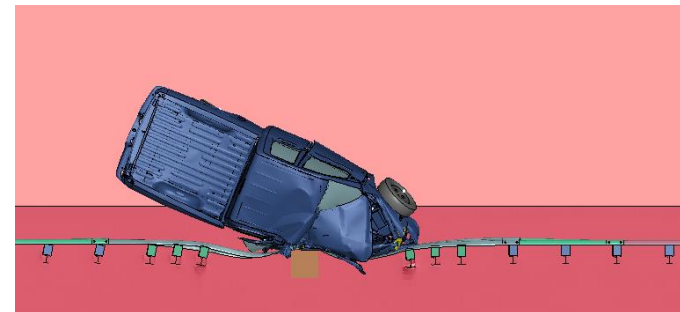
Figure 2.92. MASH Test 3-11 Simulation of Quarter-Post Large Gap with Fixed Object 4 inch Offset – Overhead View
