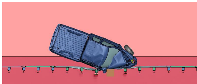
Figure 2.149. MASH Test 3-11 Simulation of Half-Post Small Gap with Fixed Object 4 inch Offset – Overhead View
