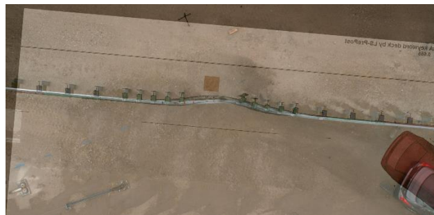
Figure 9.3. MASH Test 3-10 and Simulated MASH Test 3-10 Overlay Comparison Photos – Overhead View
