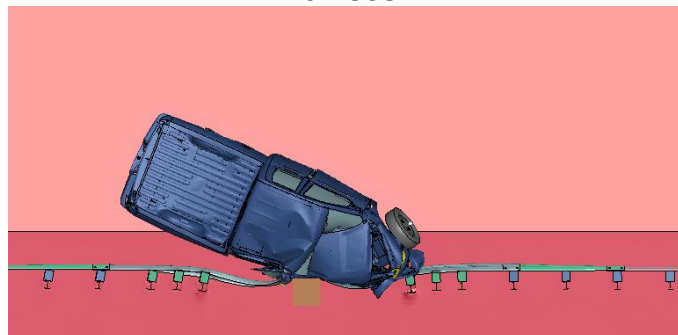
Figure 2.95. MASH Test 3-11 Simulation of Quarter-Post Large Gap with Fixed Object 6 inch Offset – Overhead View
