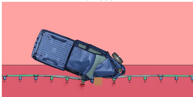
Figure 2.146. MASH Test 3-11 Simulation of Half-Post Small Gap with Fixed Object 2 inch Offset – Overhead View
