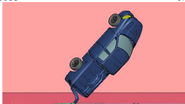
Figure 2.134. MASH Test 3-11 Simulation of Quarter-Post Large Gap with Fixed Object 30 inch Offset 2 feet Downstream Impact Variation – Overhead View
