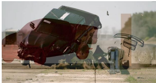
Figure 9.2. MASH Test 3-11 and Simulated MASH Test 3-11 Overlay Comparison Photos – Downstream View
