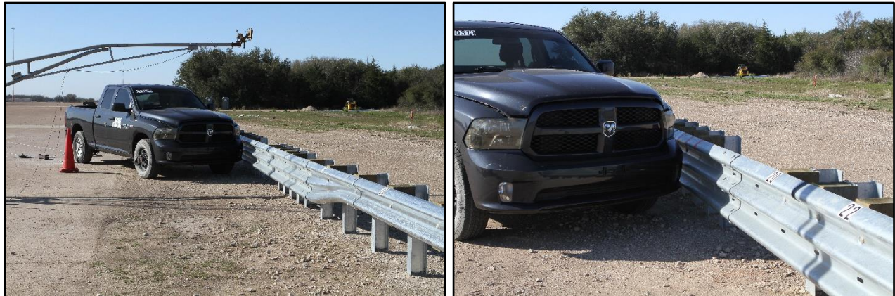
Figure 7.1 Thrie-Beam Guardrail System at a Fixed Object/Test Vehicle Geometrics for Test 614031-01-1.
