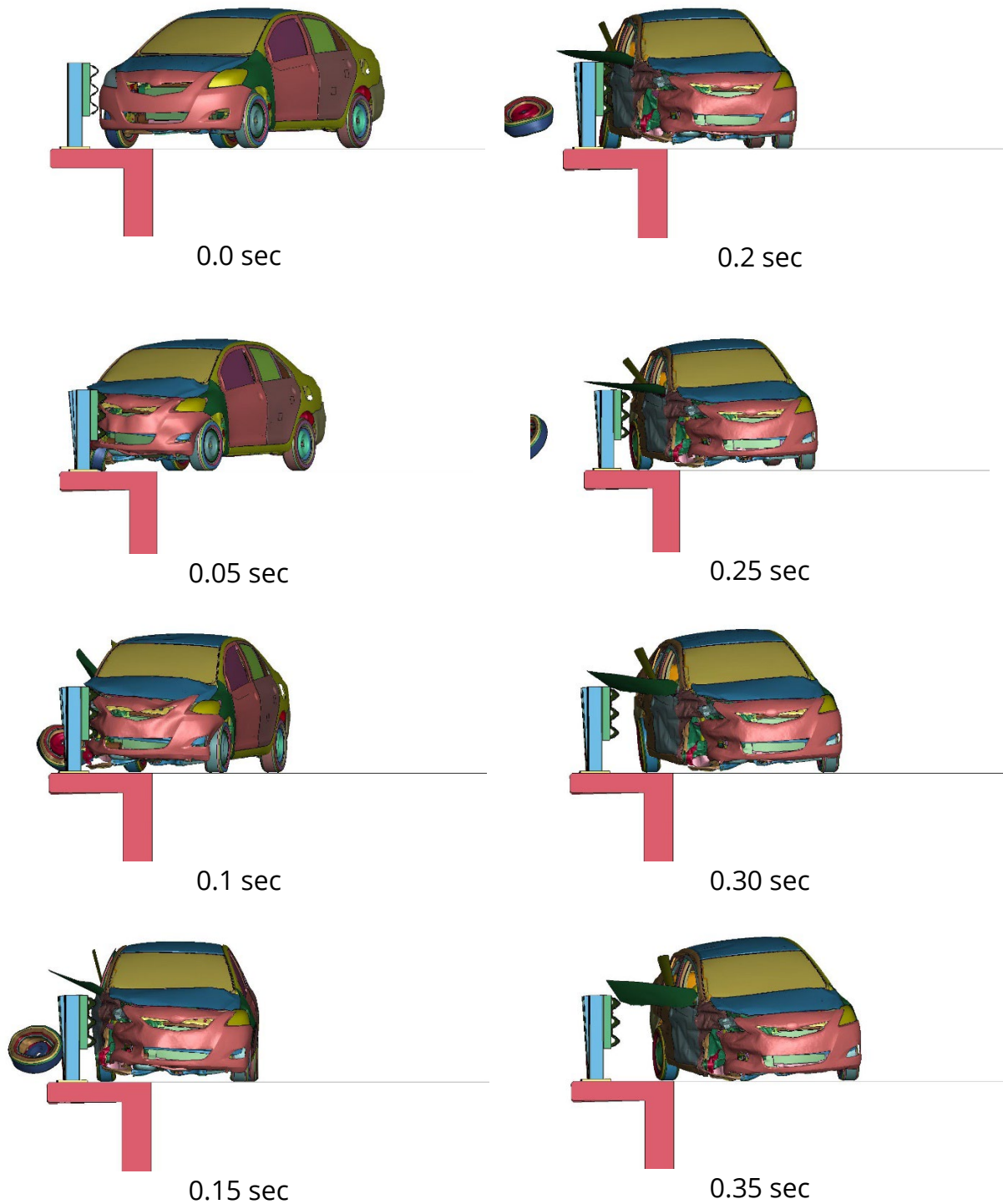
Figure 3.12. FE Simulation Sequential Images for Thrie-beam System without Curb – MASH Test 3-10.
