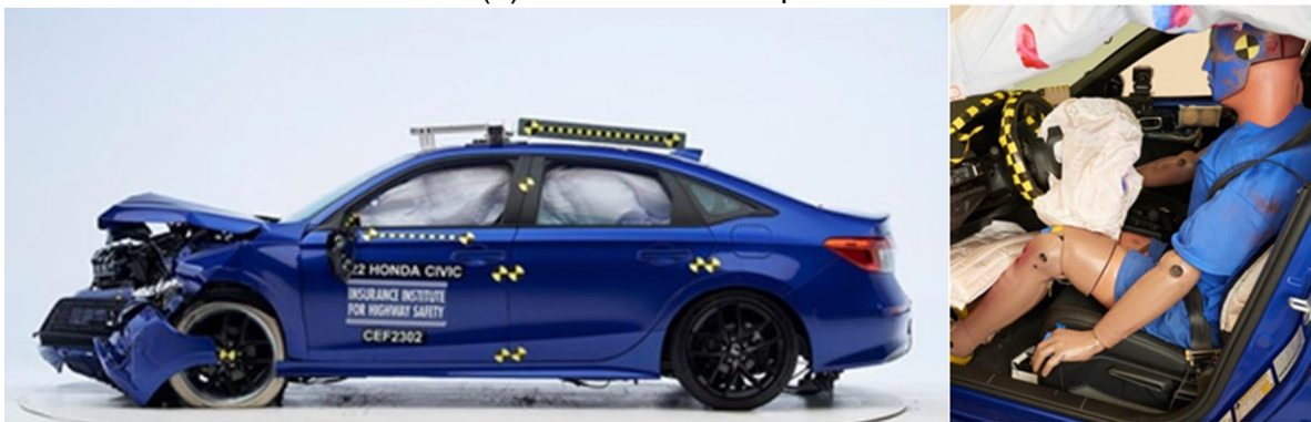
(b) Vehicle damage after impact
