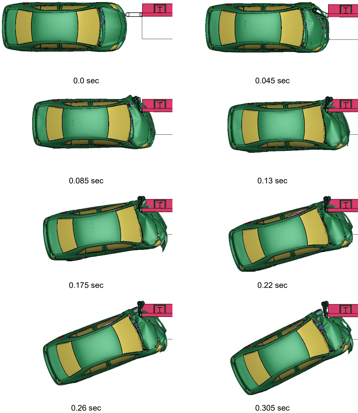
Figure 5.10. Sequential Images Impacting Attenuator Option 1 with Small Car
