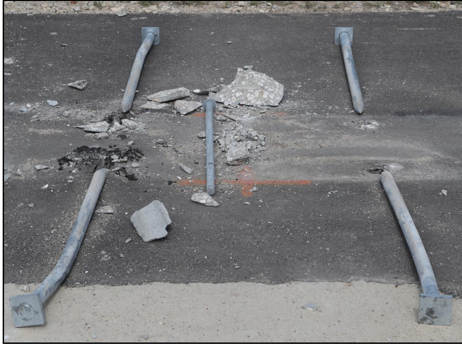
Figure 5.11. Anchoring Pins, Connection Pin, and Asphalt Damage at Joint between Barrier Segments 8 and 9 Post-Disassembly after Test 622421-01-1.
