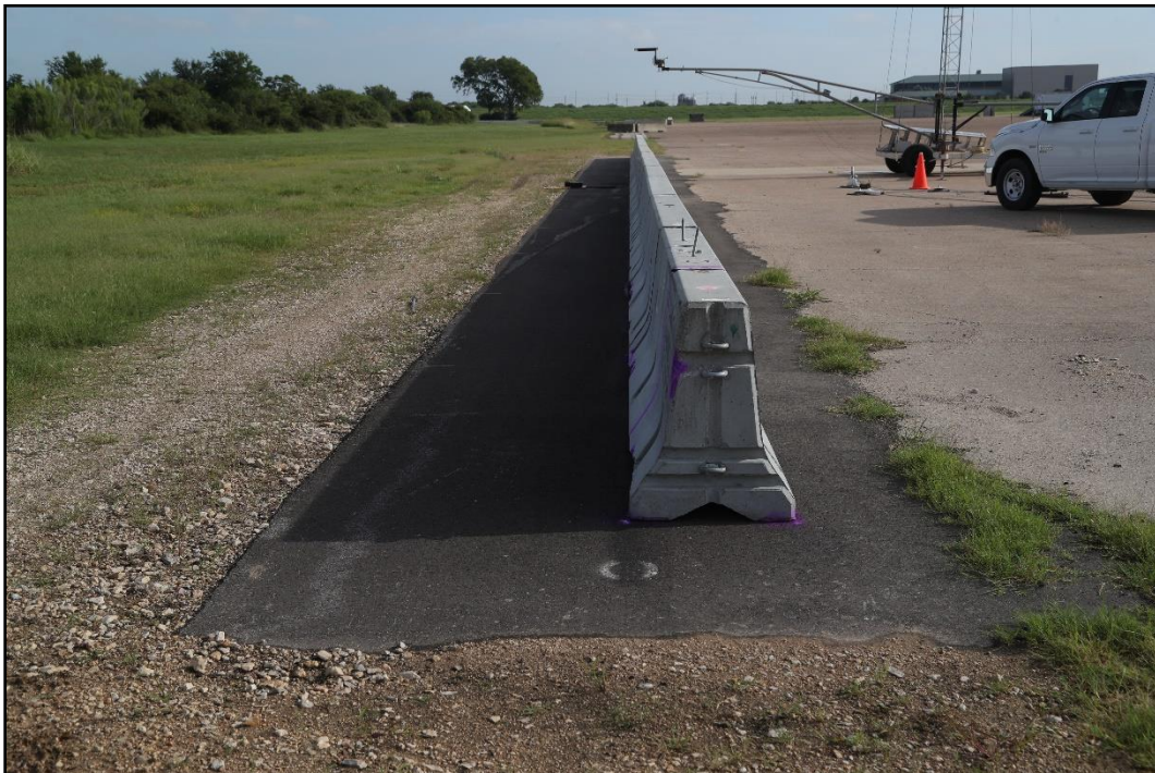
Figure 2.3. Downstream In-Line View of the Free-Standing-to-Anchored PCB Transition System Prior to Testing.
