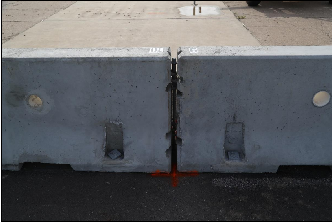
Figure 2.6. Field Side View of the Transition System at Joint Between Segments 9 and 10 Prior to Testing.
