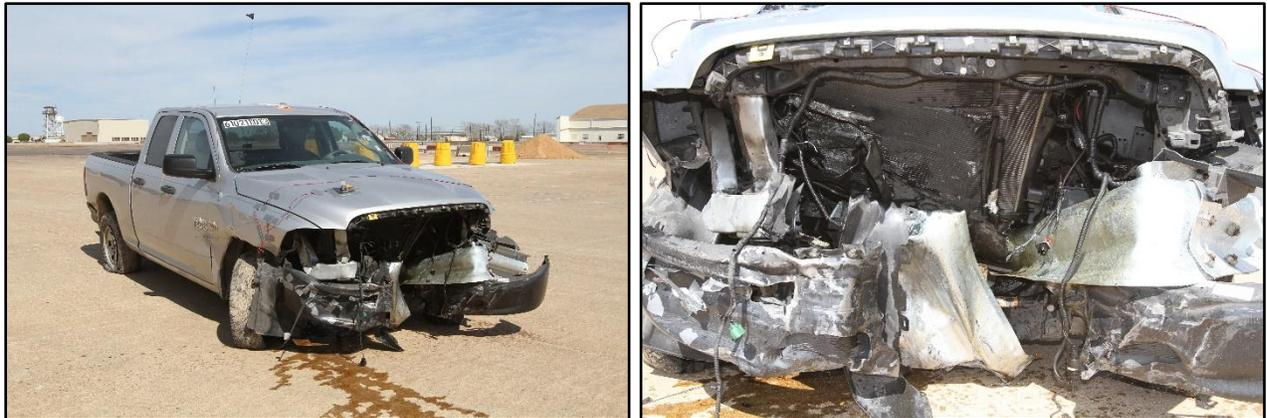
**Figure 5.6. Test Vehicle after Test No. 610211-01-3.**
