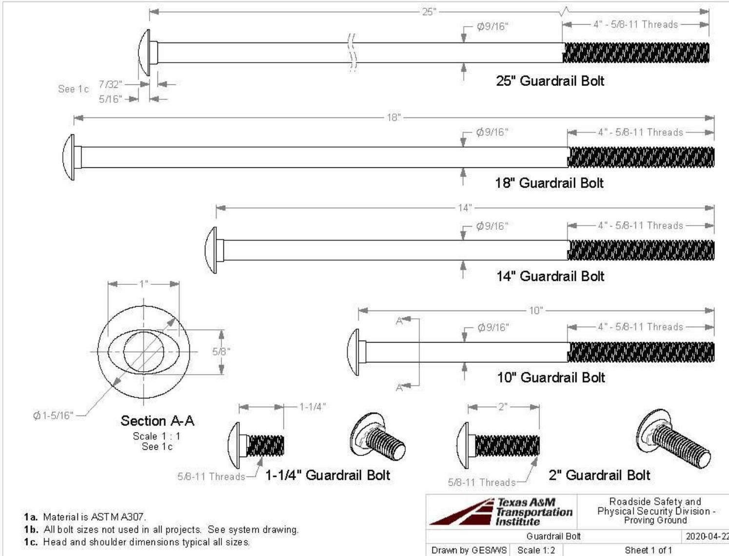
T:\Drafting Department\Solidwork.s\Standard Parts\Guardrail Parts and Subs\Guardrail Drawings\Guardrail Bolt
