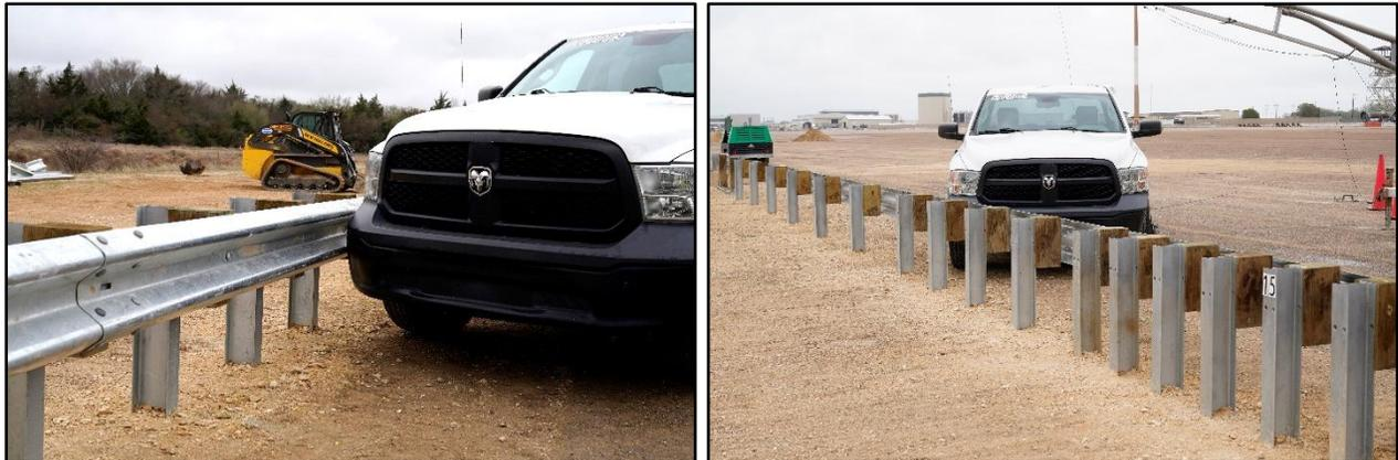
**Figure 6.18. Transition/Test Vehicle Geometrics for Test No. 610211-01-5.**
