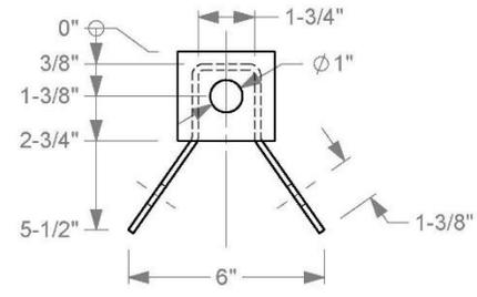
**Guardrail Anchor Bracket**
