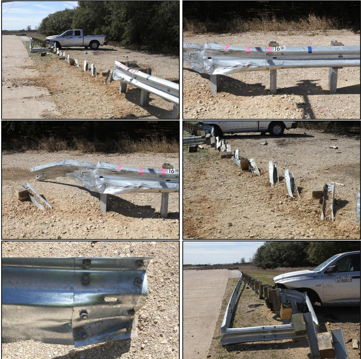
Figure 5.5. MGS with Half Post Spacing after Test No. 610211-01-3.
