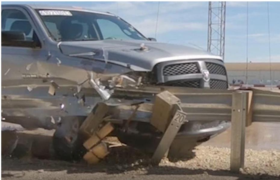
**Figure 5.9. Rear View of Rail Rupture.**
