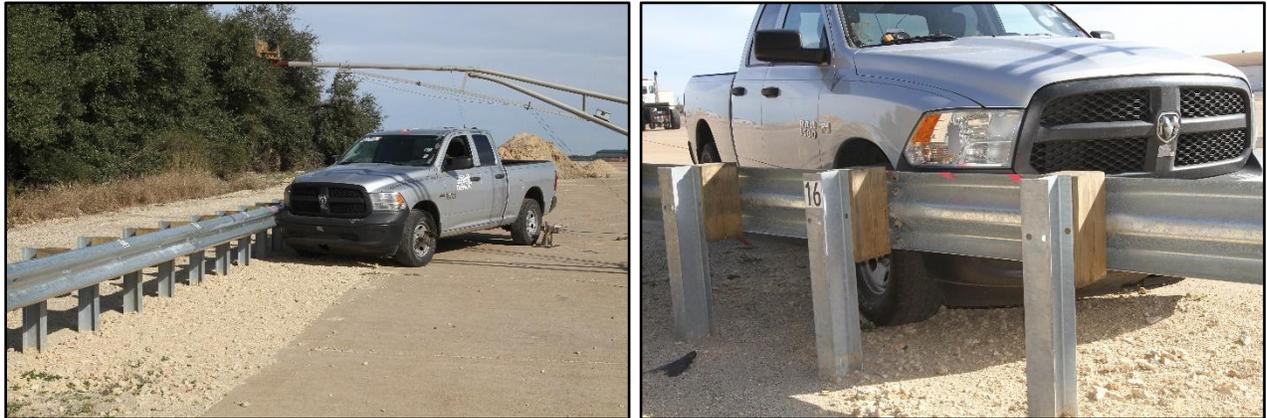
**Figure 5.3. MGS with Half Post Spacing/Test Vehicle Geometrics for Test No. 610211-01-3.**
