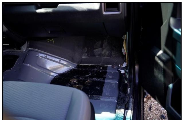
**Figure 5.23. Interior of Test Vehicle after Test No. 610211-01-6.**
