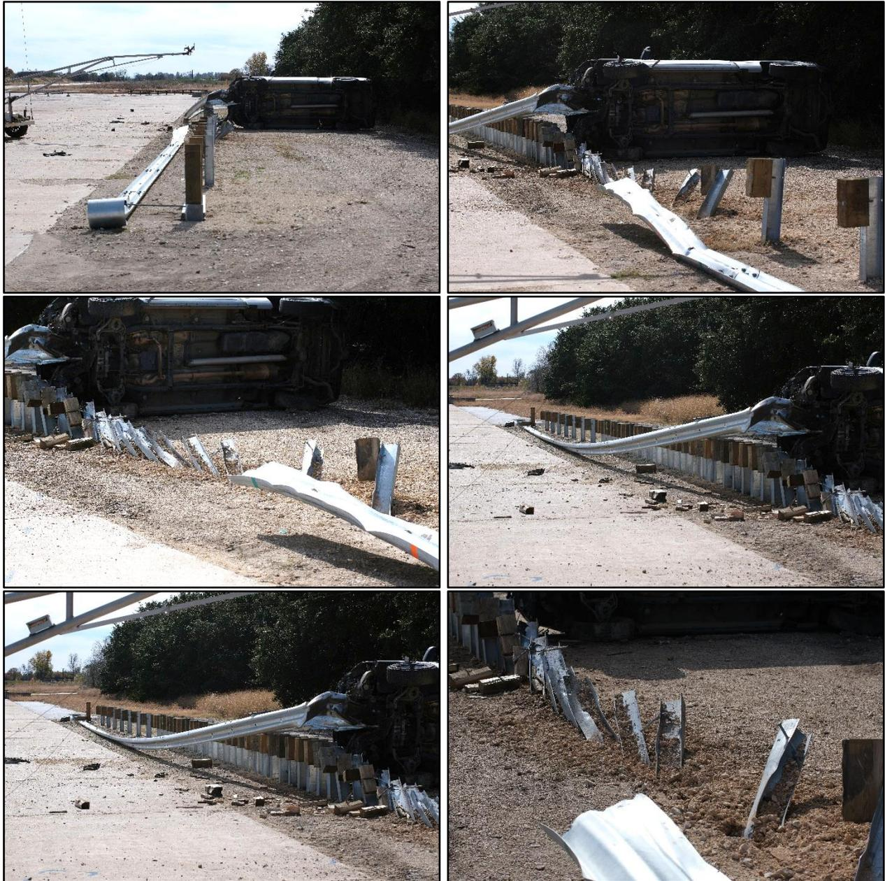
**Figure 6.5. Transition from Full to Quarter Post Spacing after Test No. 610211-01-4.**
