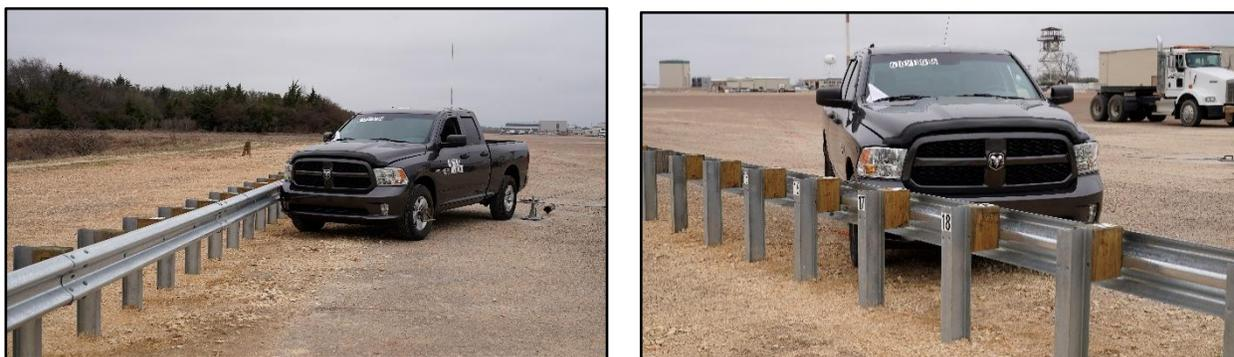
**Figure 5.19. Guardrail/Test Vehicle Geometrics for Test No. 610211-01-6.**
