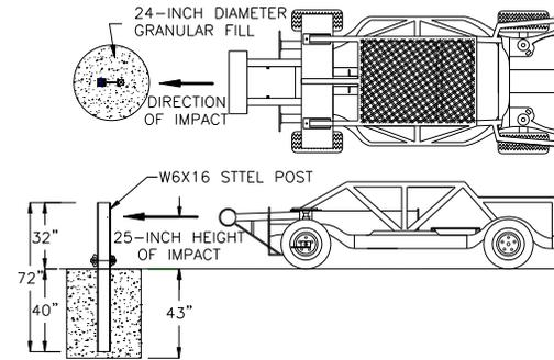
**Static Load Test Installation Details**
