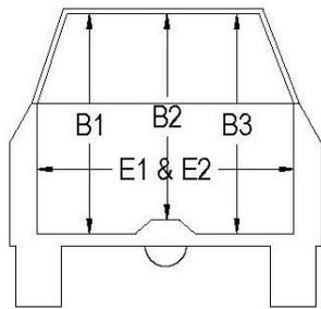
**OCCUPANT COMPARTMENT DEFORMATION MEASUREMENT**
