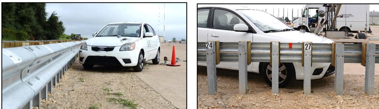
**Figure 4.3. Guardrail/Test Vehicle Geometrics for Test No. 610211-01-1.**
