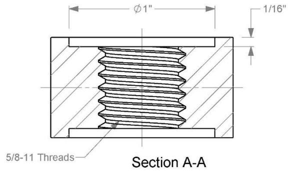
1a. Material is ASTM A 563 Grade A.
