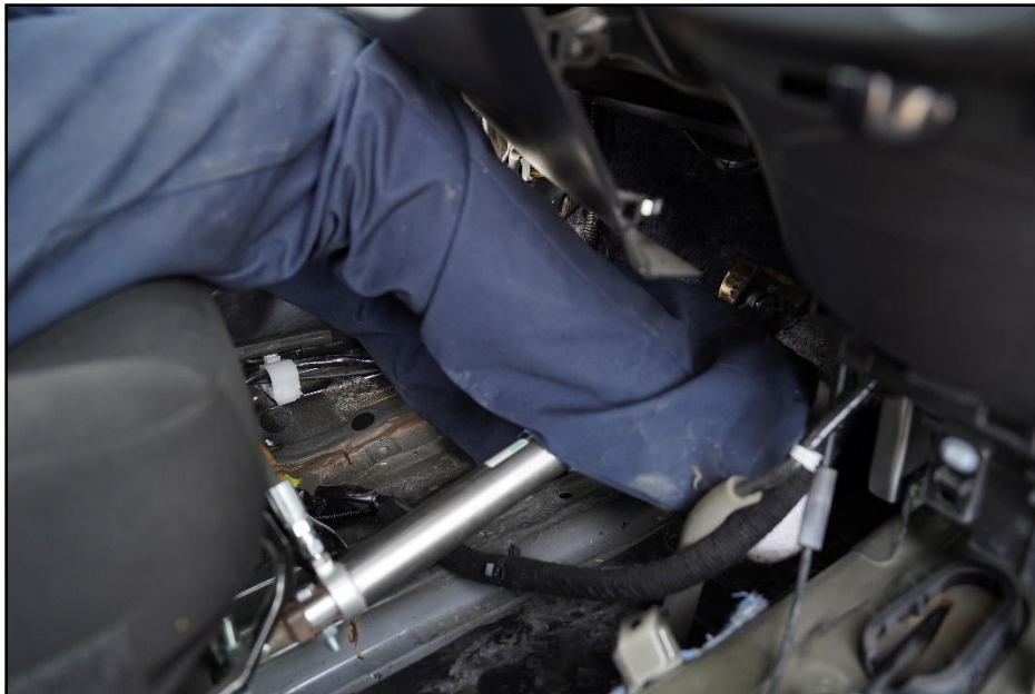
Figure 7.11. Interior of Test Vehicle on Impact Side after Test 620281-01-1.
