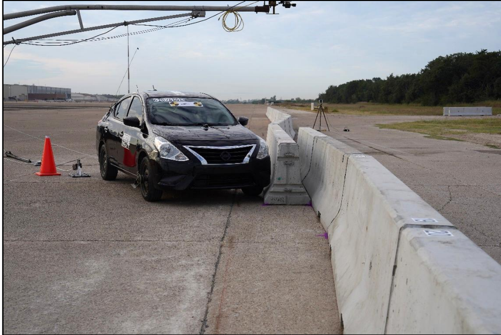
Figure 7.2. Overlapping Precast Portable Concrete Barriers/Test Vehicle Geometrics for Test 620281-01-1.
