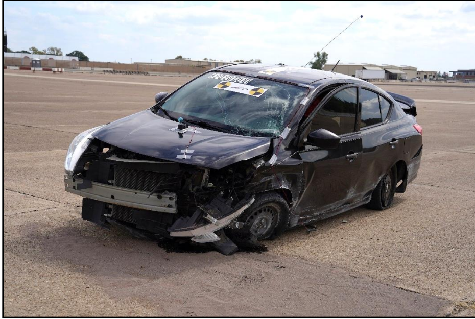
Figure 7.8. Impact Side of Test Vehicle after Test 620281-01-1.
