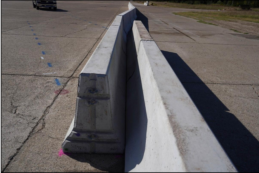
Figure 4.6. In-line View of the Overlapping Precast Portable Concrete Barriers at the Overlap prior to Testing.
