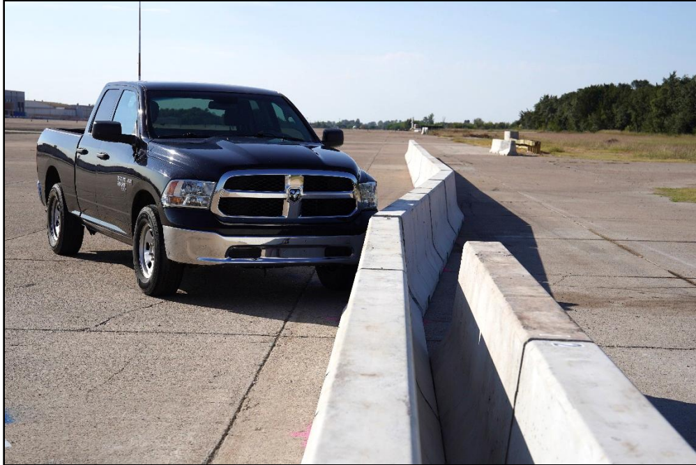
Figure 8.2. Overlapping Precast Portable Concrete Barriers/Test Vehicle Geometrics for Test 620281-01-2.
