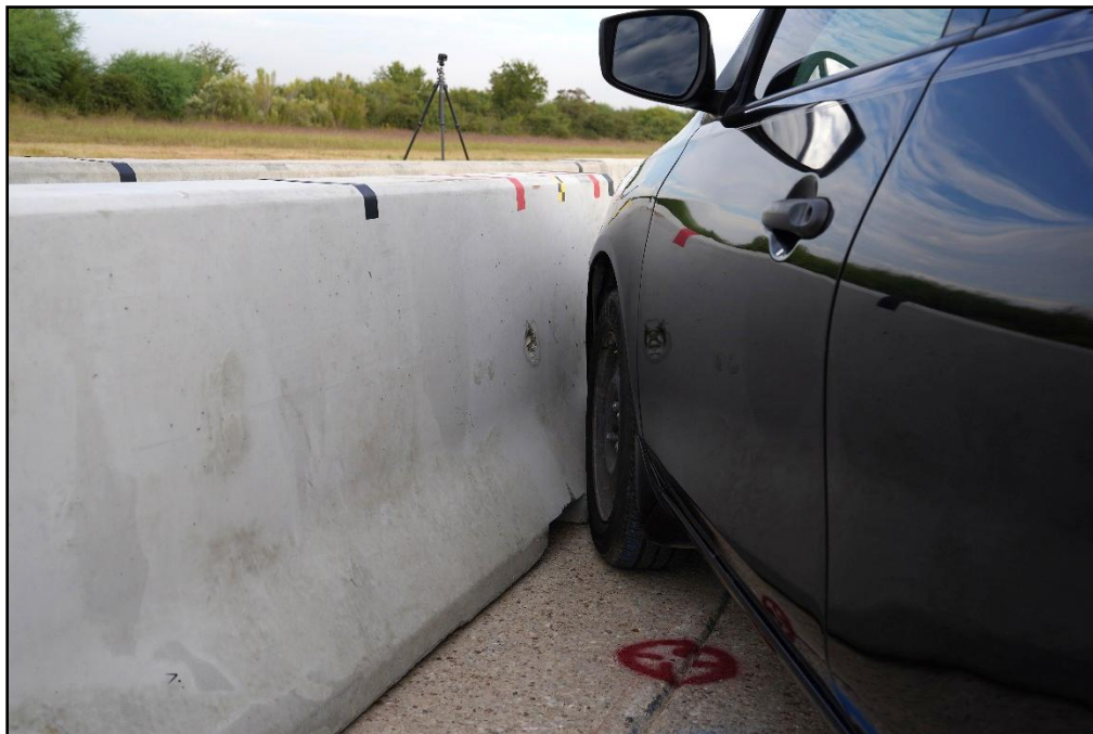
Figure 7.3. Overlapping Precast Portable Concrete Barriers/Test Vehicle Impact Location 620281-01-1.
