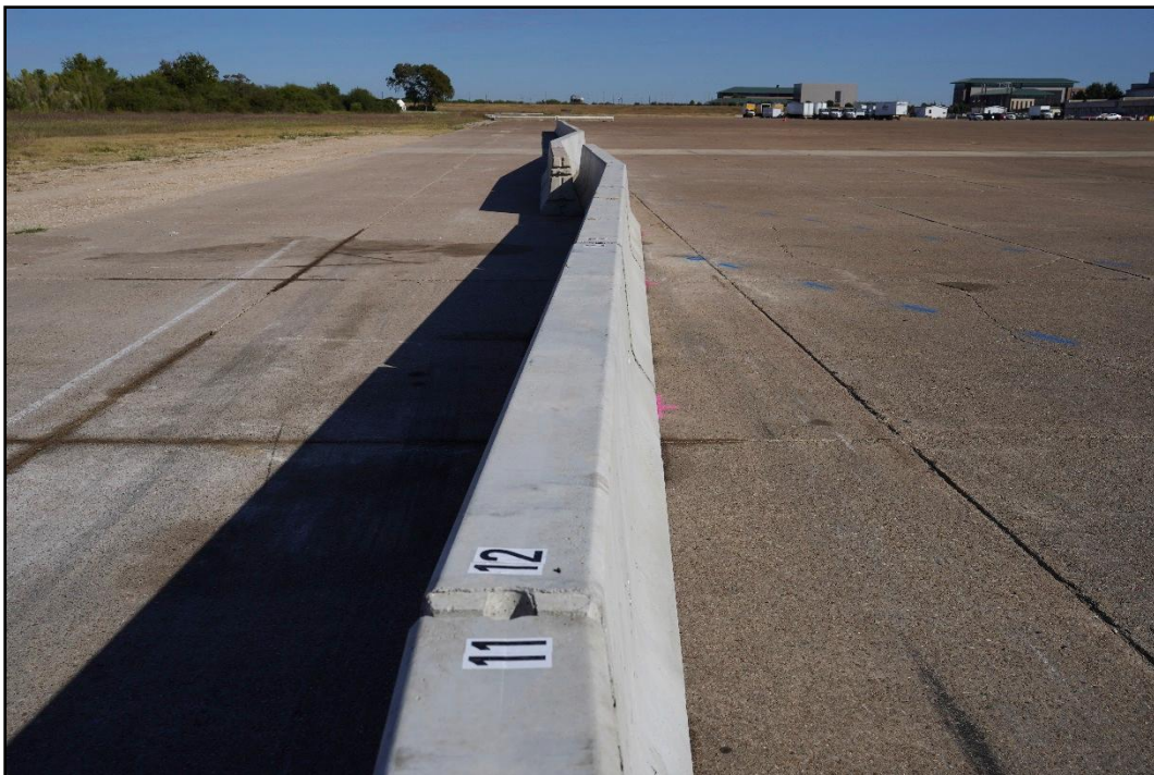
Figure 4.3. In-line View of the Overlapping Precast Portable Concrete Barriers prior to Testing.
