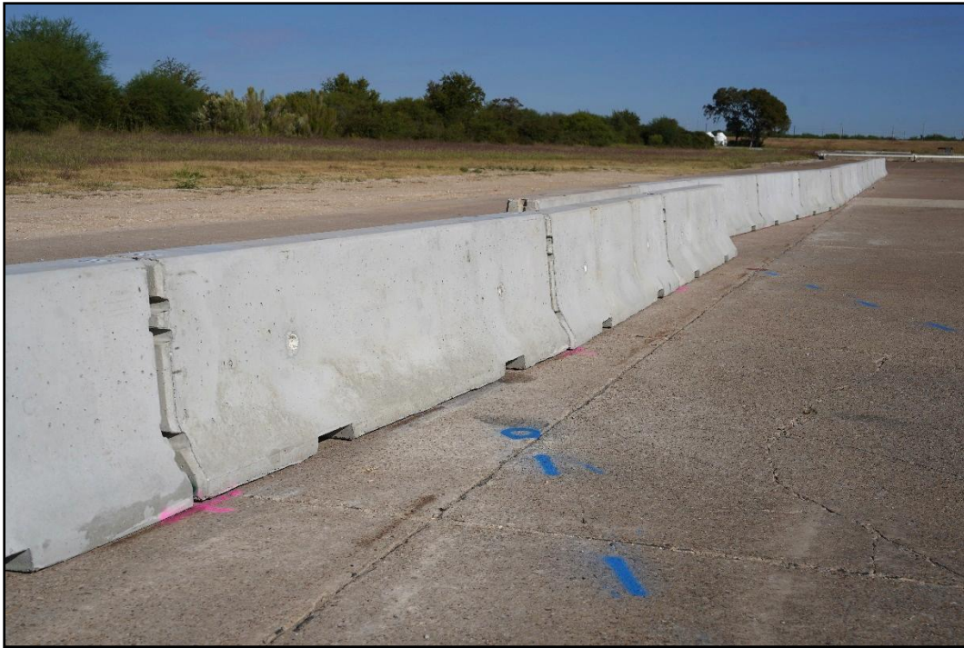
Figure 4.2. Overlapping Precast Portable Concrete Barriers prior to Testing.
