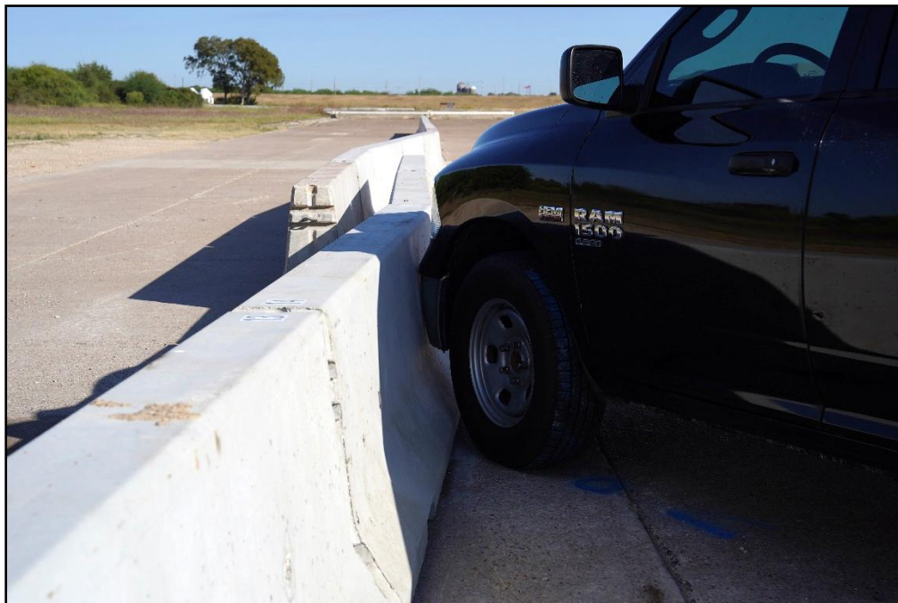
Figure 8.3. Overlapping Precast Portable Concrete Barriers/Test Vehicle Impact Location 620281-01-2.
