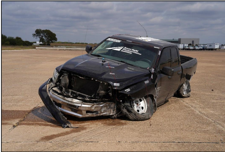
Figure 8.8. Impact Side of Test Vehicle after Test 620281-01-2.
