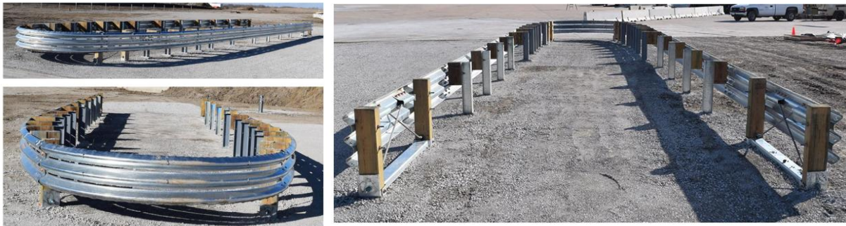
Figure 2.4. MwRSF Thrie-beam Bullnose Median Barrier System [7]
