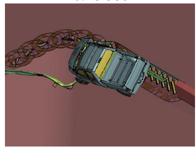
Figure 4.4. Sequential images for Test 3-33 with Nested Nose Rails
