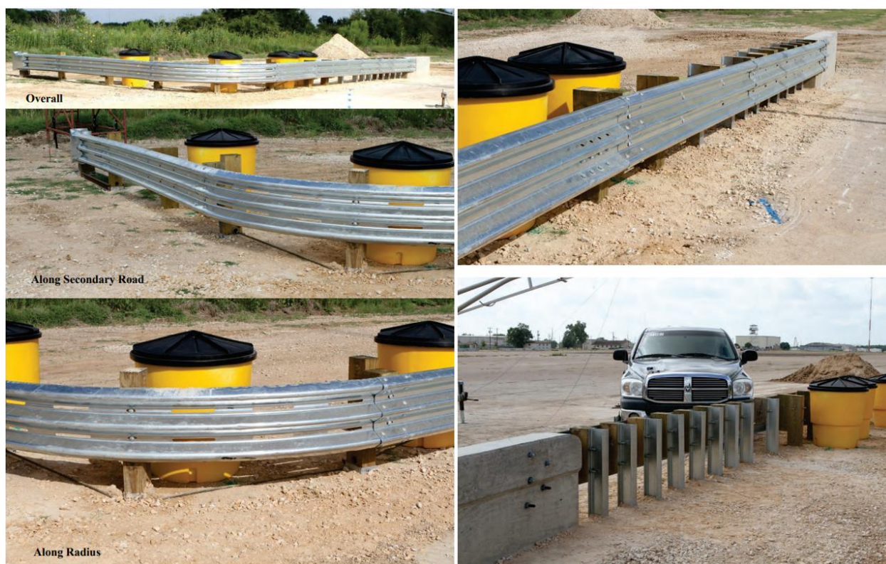
Figure 2.2. TXDOT Short-Radius Guardrail MASH TL-3 setup [5]
