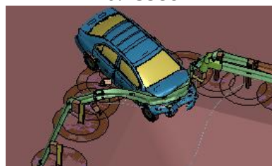
Figure 4.15. Sequential Images for Passenger Car impacting SRGS with 4-ft Flat Bench Section at 15- and 25-Degrees
