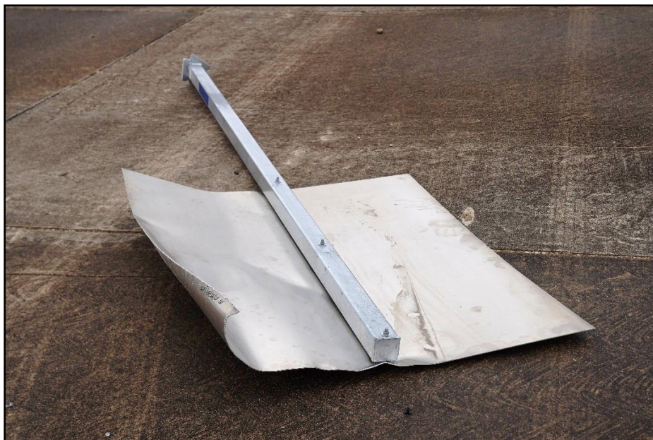
Figure 7.7. 3 × 3 Square Tube Slip Base Sign Support System at Resting Position after Test 621201-01-2.
