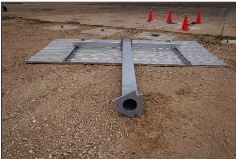
Figure 9.7. 8 × 8 Square Tube Slip Base Sign Support System at Resting Position after Test 621201-01-3.
