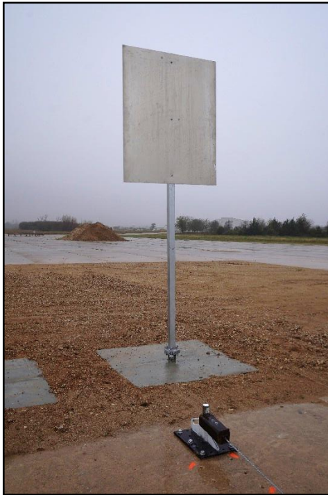
Figure 5.2. 3 × 3 Square Tube Slip Base Sign Support System prior to Testing.
