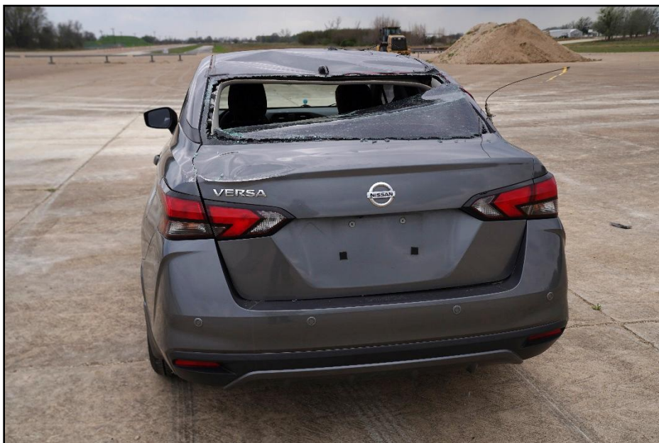
Figure 9.9. Rear Impact Side of Test Vehicle after Test 621201-01-3.
