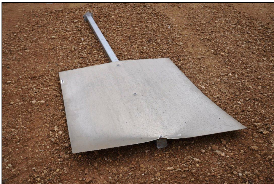
Figure 6.7. 3 × 3 Square Tube Slip Base Sign Support System at Resting Position after Test 621201-01-1.
