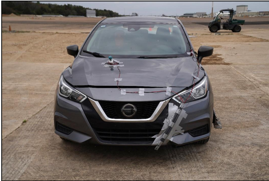
Figure 9.8. Impact Side of Test Vehicle after Test 621201-01-3.
