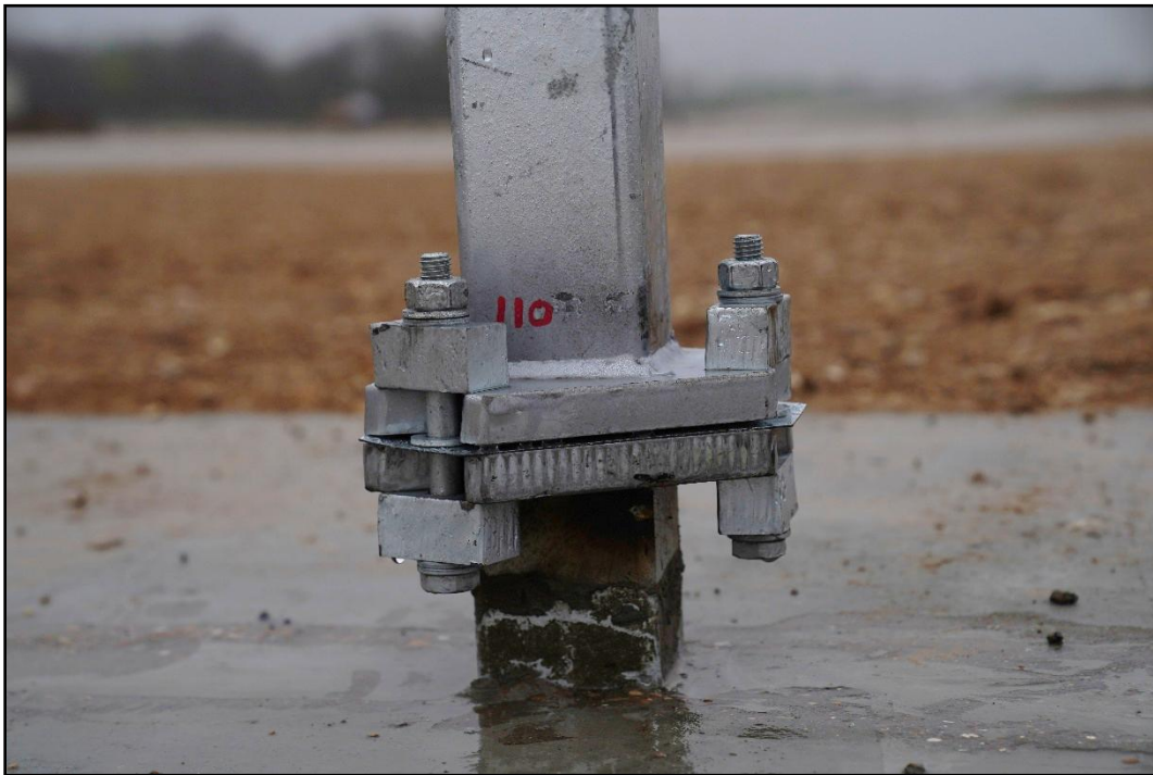
Figure 5.5. Slip Base Assembly prior to Testing.
