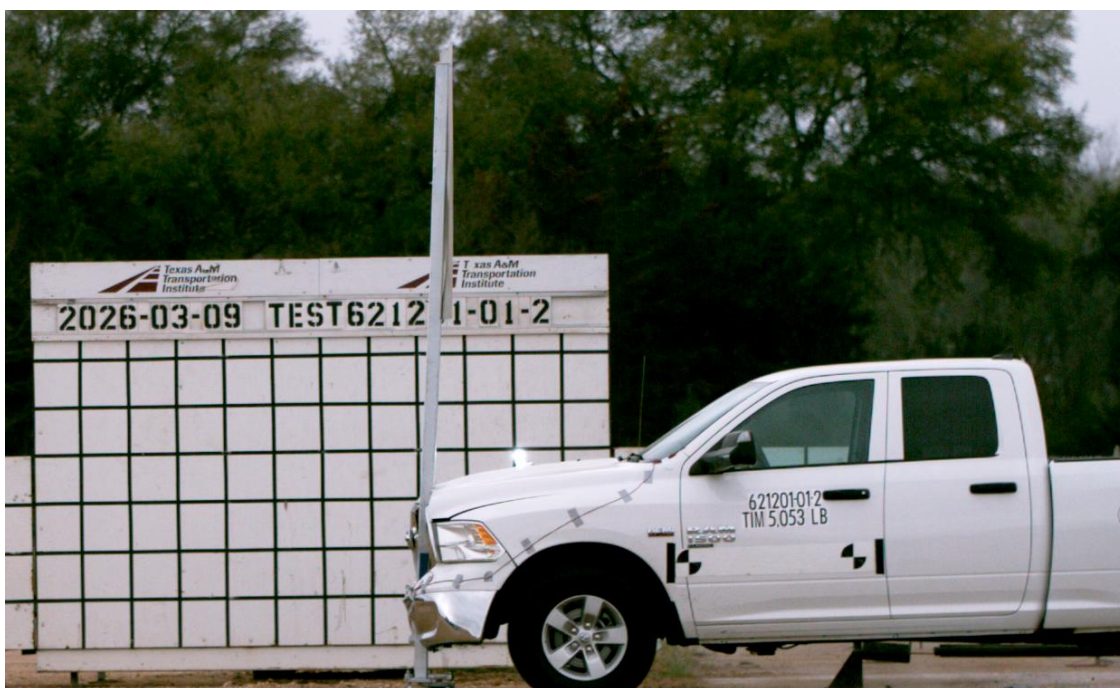
Figure 10.1. Engagement of Pickup Truck Hood with Post.
