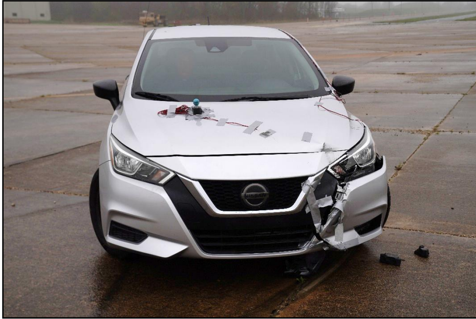
Figure 6.8. Impact Side of Test Vehicle after Test 621201-01-1.
