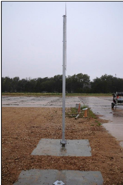
Figure 5.3. Right Angle View of the 3 × 3 Square Tube Slip Base Sign Support System prior to Testing.
