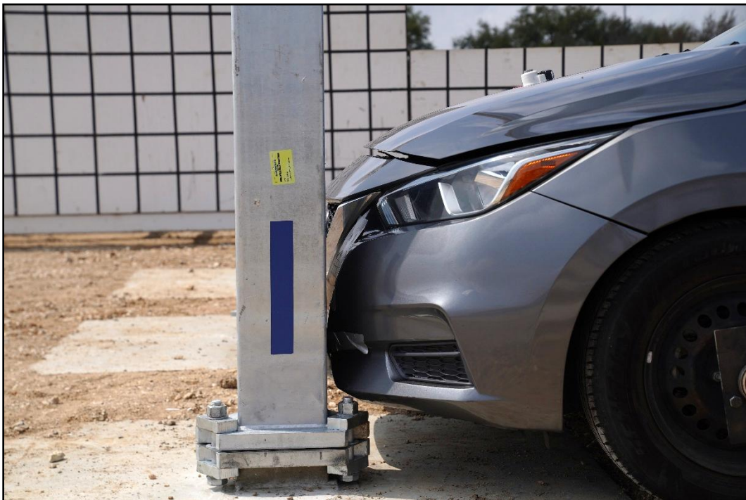
Figure 8.3. 8 × 8 Square Tube Slip Base Sign Support System Base prior to Testing.
