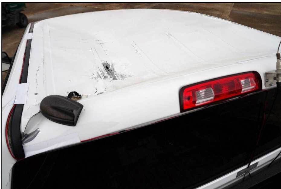
Figure 7.9. Rear Impact Side of Test Vehicle after Test 621201-01-2.
