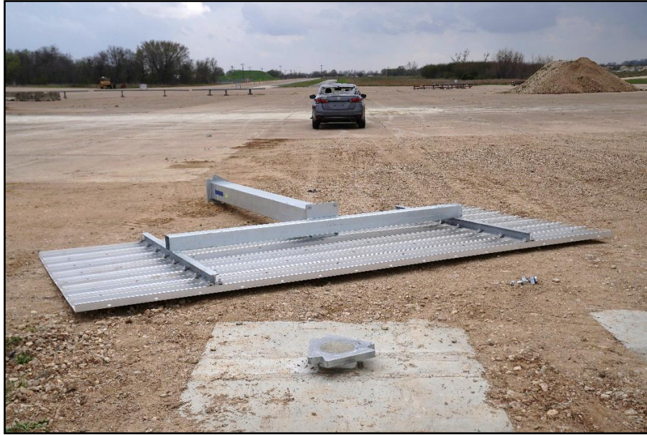
Figure 9.6. 8 × 8 Square Tube Slip Base Sign Support System at Impact Location after Test 621201-01-3.
