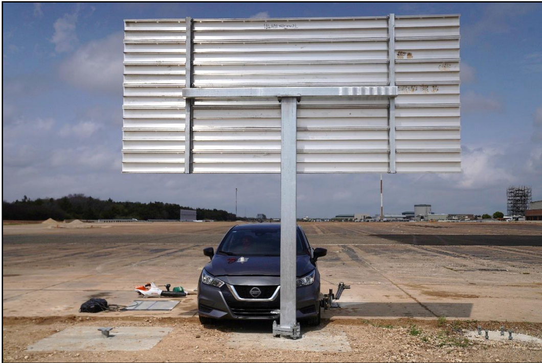
Figure 8.2. 8 × 8 Square Tube Slip Base Sign Support System prior to Testing.
